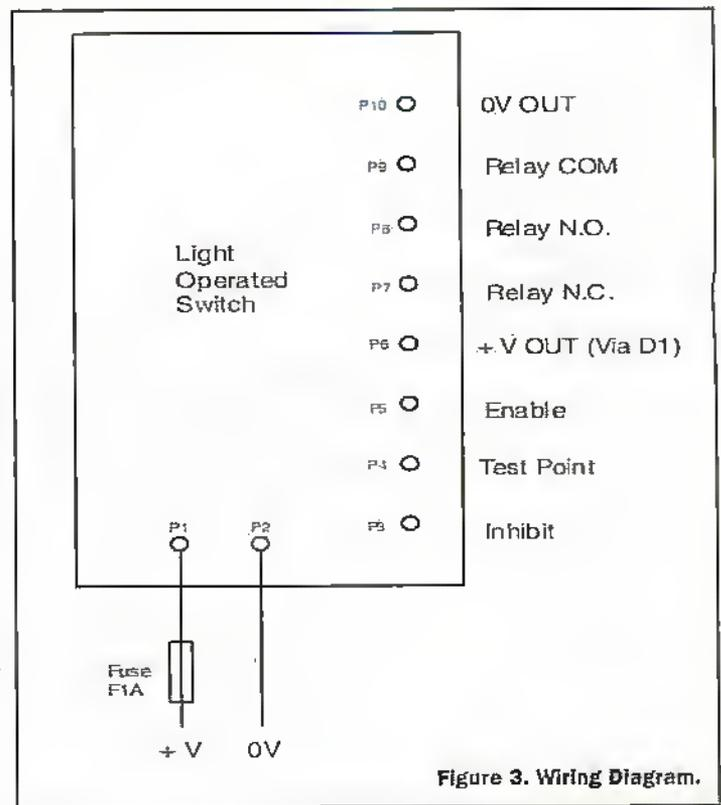
Figure 3. Wiring Diagram.
