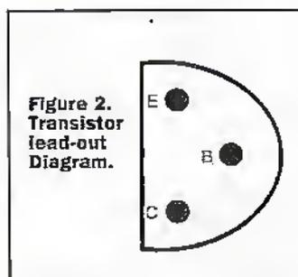
Figure 2. Transistor lead-out Diagram.
