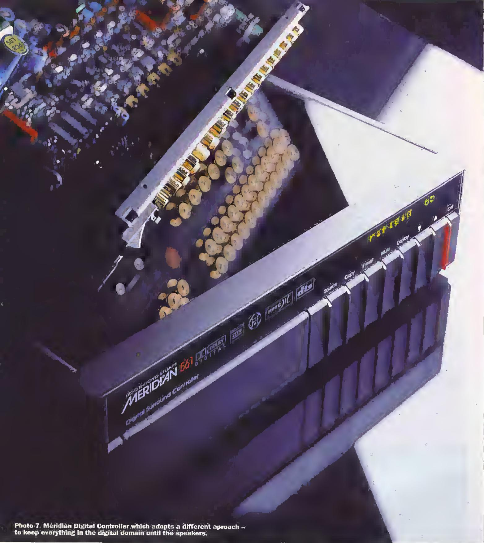
Photo 7. Meridian Digital Controller which adopts a different approach – to keep everything in the digital domain until the speakers.
