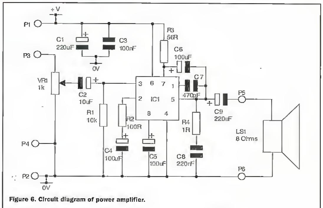
Figure 6. Circuit diagram of power amplifier.
