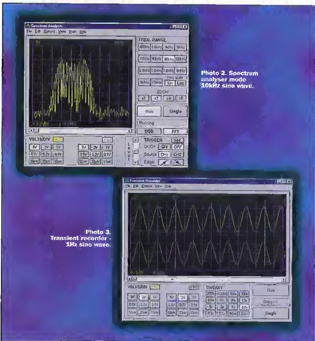
Photo 2. Spectrum analyser mode 10kHz sine wave.
