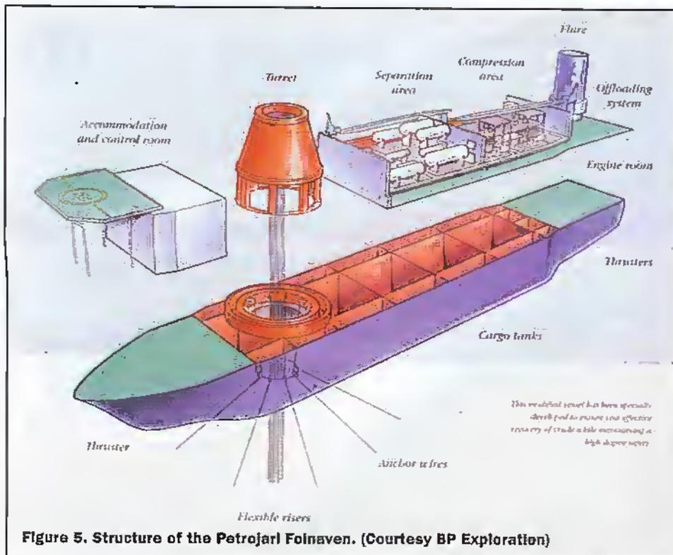
Figure 5. Structure of the Petrojarl Foinaven. (Courtesy BP Exploration)
