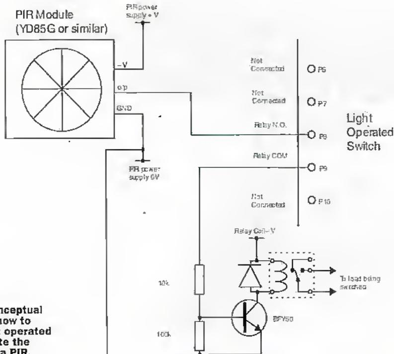
**Figure 7. Conceptual example of how to use the light operated switch to gate the output from a PIR.**
