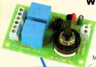
Up to 3 different time intervals (2 - 10 - 15 seconds) can be selected for the windshield wipers of your car. It can also be used for automatic slide projection. Manual includes installation instructions for most cars.
