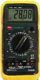
True RMS digital multimeter with 4 1/2 LCD display. 10 different functions and 32 ranges. Data hold function. DC and AC voltage measurements : DC (max. 1000V) en AC (max. 700V). DC and AC current measurements : max. 10A. Resistance (up to 200Mohm) and continuity measurements. Diode- and transistor test. Capacitance measurements up to 20µF. Frequency measurements up to 20kHz. With protection holster.
