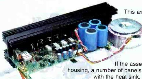
This amplifier is the mono version of the K4020 amplifier, but comes without a housing. Heat sink and transformer are included. Ideally suited for installation in disco bars and active speaker systems.
