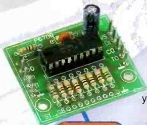
This transmitter K6700 allows you to open or to close 8 (extendible up to 16) different contacts from just two wires. For use with K6701. For use in model building, model trains, or wherever you want to establish several connections with only two wires. Connection of several receivers on one transmitter is possible (several transmitters on one receiver is NOT possible !)
