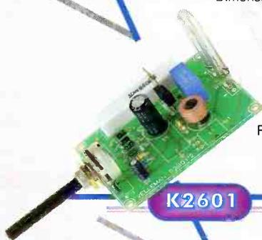
Flashing light effects for discos. Make your own snapshots and "lightning" light effects. Flash frequency adjustable from 2 to 20Hz.
