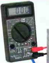
Automatic polarity indication. Low battery indication. Transistor and diode test. DC current max. 10A. AC voltage max. 600V. Max. resistance measurements : 2Mohm
