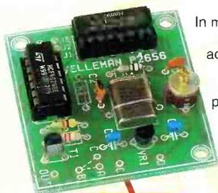
In many clocks and circuits mains frequency is used as the time base, because of its high accuracy. If these devices are to be supplied by batteries (e.g. in the event of power failure) another time base should be provided to prevent the clock from stopping. This kit provides the standard 50Hz mains frequency, 100Hz (for devices operating with hundreds of seconds) or 400Hz signals (selectable).
