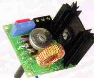
Due to its small size, this small dimmer easily replaces an existing switch, permitting you to vary the brightness of a light or group of lights. The dimmer may also be used to adjust the speed of a motor, vacuum cleaner, or any other motor with carbon brush. A mains suppresser is provided eliminating undesirable RFI. It is not suitable for halogen lamps.
