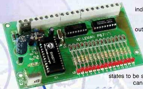
The receiver has 15 independent outputs. Each output can be operated separately and every output carries the option of being used as a change-over switch or pulse contact. The receiver is built around a microprocessor, allowing two output states to be stored in memory, which can be recalled at all times.
