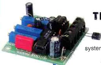
This kit has been developed especially to be combined with the K6000 or K6002 to build a temperature regulation and control system. The advantage of a separate sensor lies in the fact that the distance between the actual controller and the sensor is of no importance.
