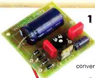
This small power supply provides a regulated voltage adjustable between 1.5 and 35 Volts at 1 Amp. With the LM317 regulator remarkably better ripple and regulation characteristics are given than with conventional regulators. Current limiter and thermal overload protection are included in the chip. Supplied without heat sink.
