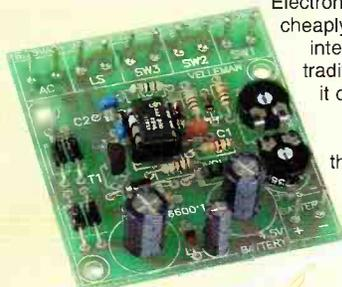
Electronic tones can be generated simply and cheaply using the device. This kit is primarily intended for use as a replacement for the traditional mechanical doorbell. Of course, it can also be used for many other types of applications. The number of tones may be selected up to a maximum of three, each of which is output one after the other. This can be used to help locate the place being called. Volume and tone can also be set. The existing bell transformer can be used as a power supply.
