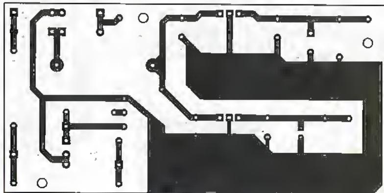
Figure 6. PSU PCB foil.
