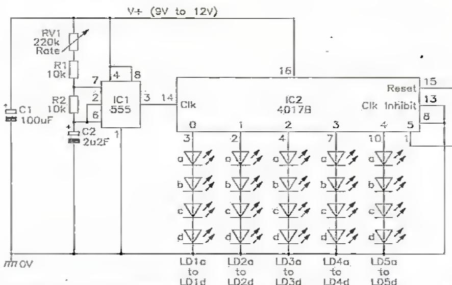
Figure 15. This 4-bank, 5-step, 20-LED chaser must be used with supply voltages of at least 9V.
