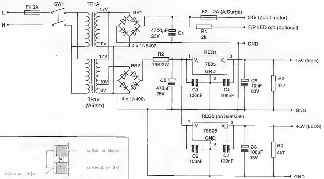
Figure 5. Circuit diagram for PSU.
