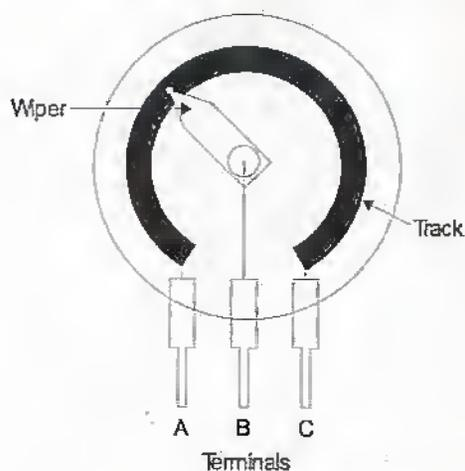
Figure 1. Simplified diagram of a typical rotary potentiometer.
