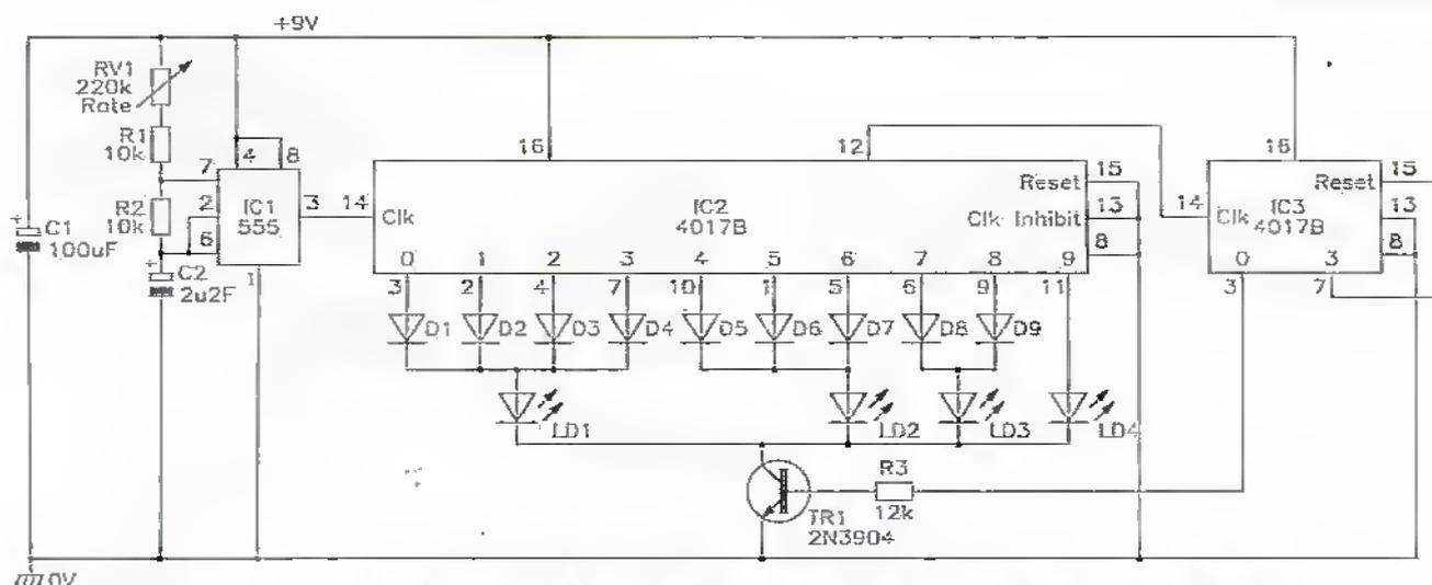
Figure 17. 4-LED Intermittent accelerator display in which acceleration occurs for ten clock steps in every thirty.
