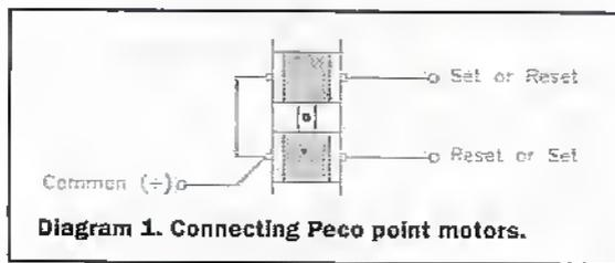
Diagram 1. Connecting Peco point motors.
