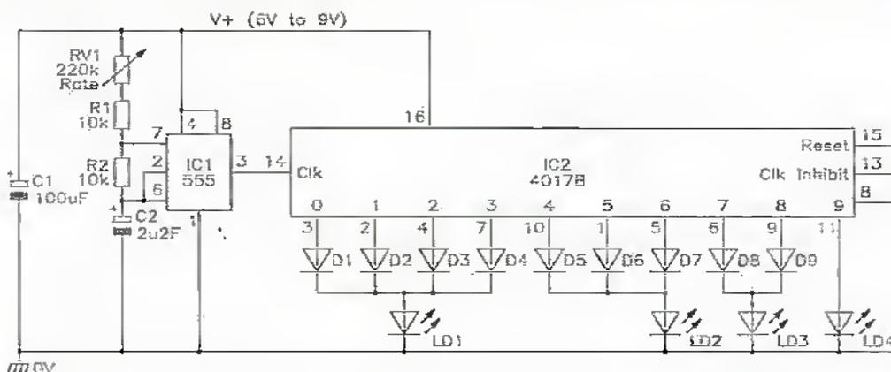
Figure 14. 4-LED continuous accelerator display in which the pattern seems to accelerate from left to right.
