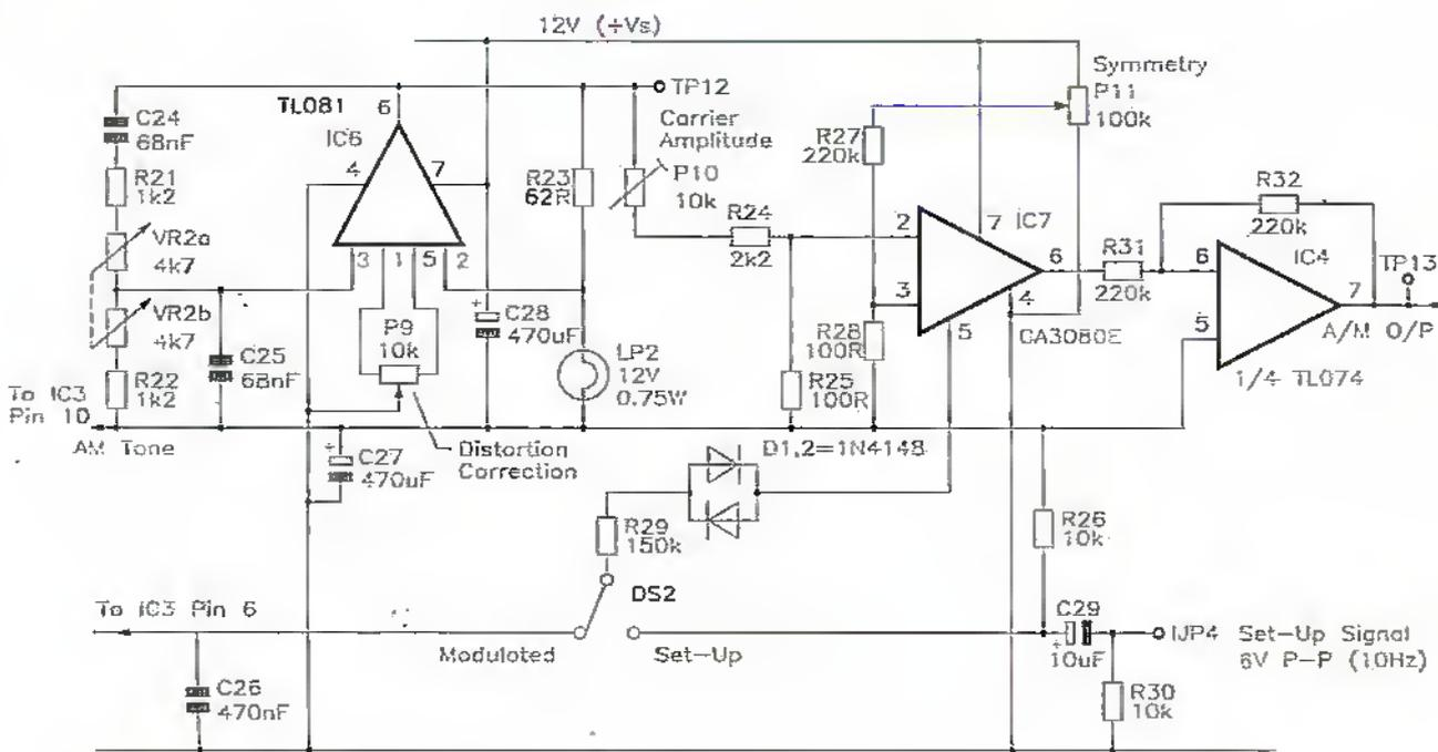
Figure 4. Amplitude modulated channel.
