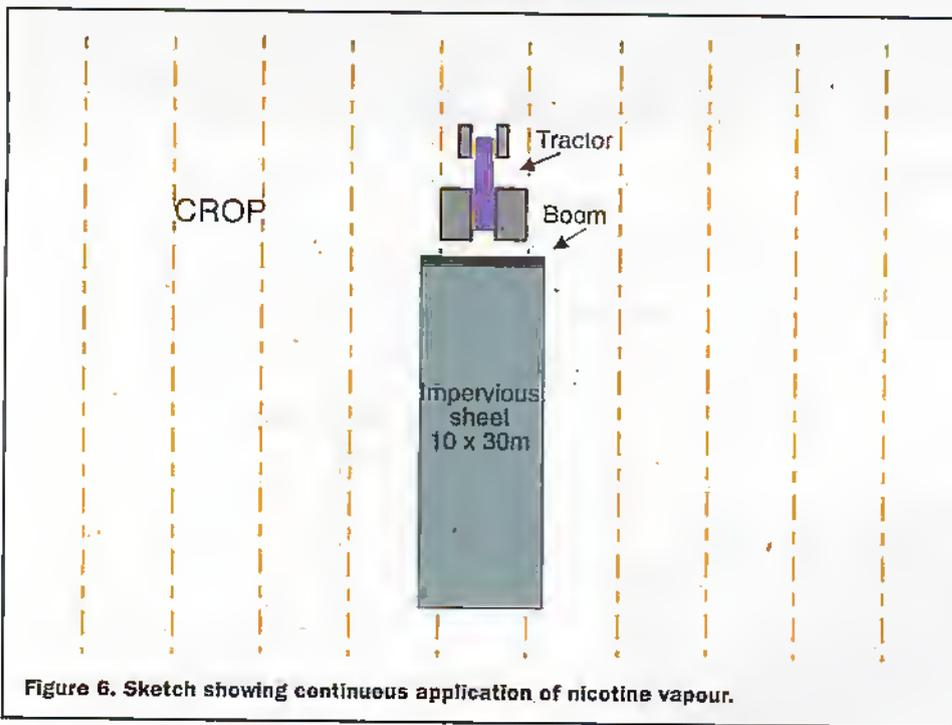
Figure 6. Sketch showing continuous application of nicotine vapour.
