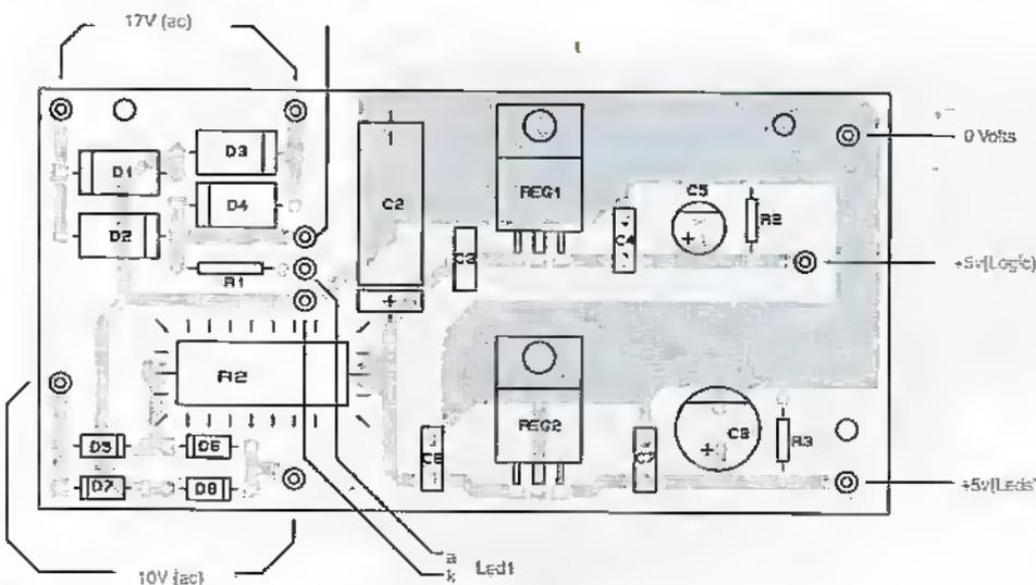
Figure 7. Component layout for PSU.
