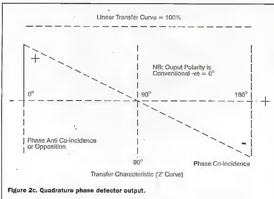
Figure 2c. Quadrature phase detector output.
