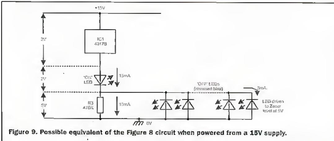
Figure 9. Possible equivalent of the Figure 8 circuit when powered from a 15V supply.
