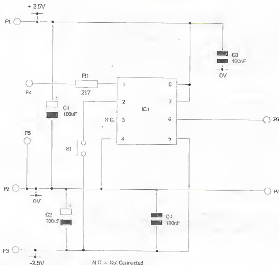
Figure 7. A simple volume control circuit using single button control.
