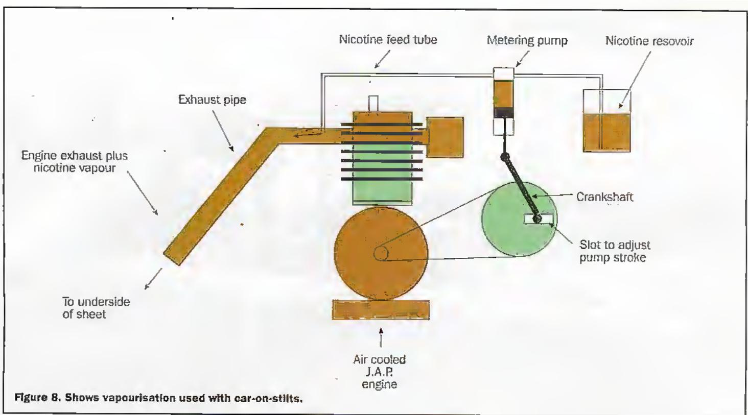
Figure 8. Shows vapourisation used with car-on-stilts.
