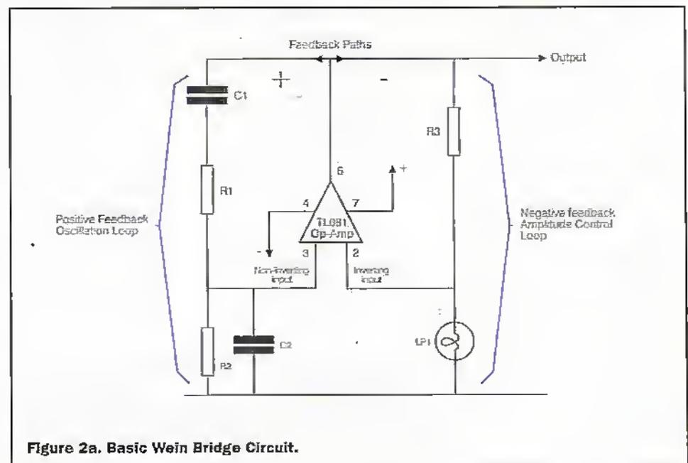
Figure 2a. Basic Wein Bridge Circuit.
