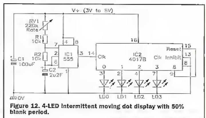
Figure 12. 4-LED intermittent moving dot display with 50% blank period.
