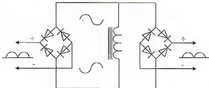
Figure 2e (iii) Double balanced bridge analogy.
