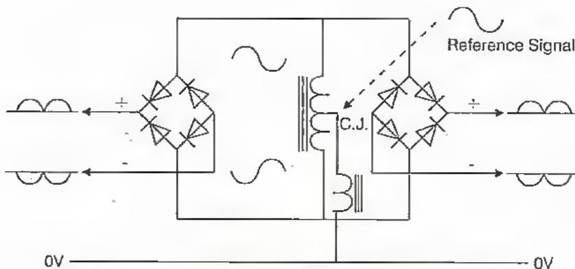
Figure 2e (iv) Double phase detector analogy.
