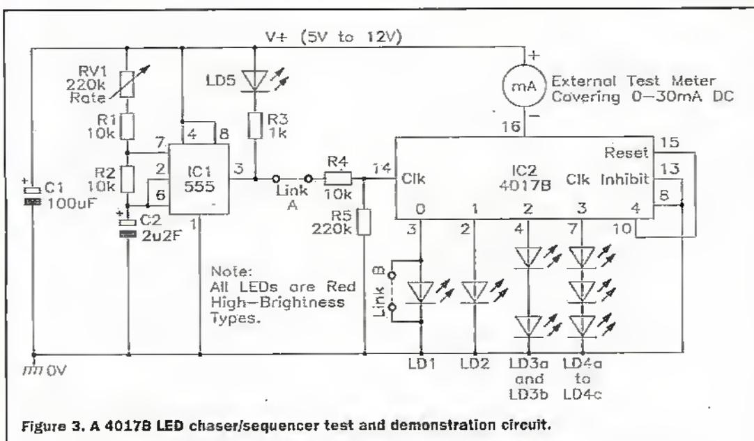
Figure 3. A 4017B LED chaser/sequencer test and demonstration circuit.
