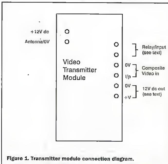
Figure 1. Transmitter module connection diagram.
