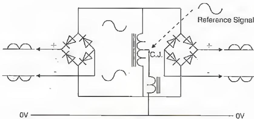
Figure 2e (iv) Double phase detector analogy.
