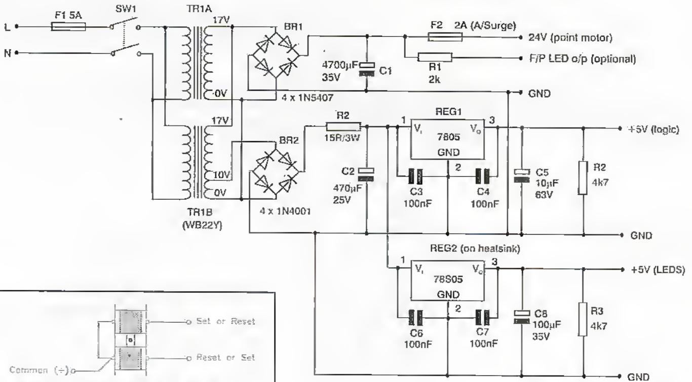
Figure 5. Circuit diagram for PSU.
