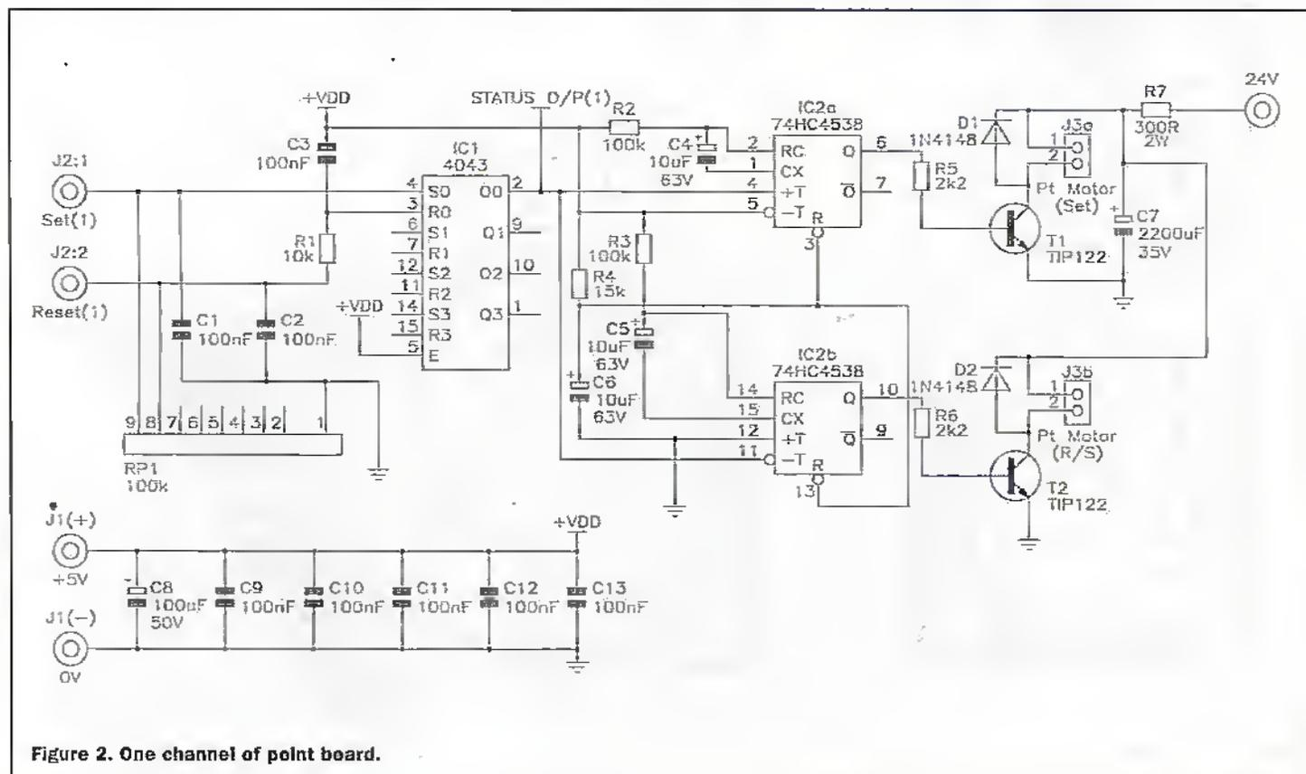
Figure 2. One channel of point board.
