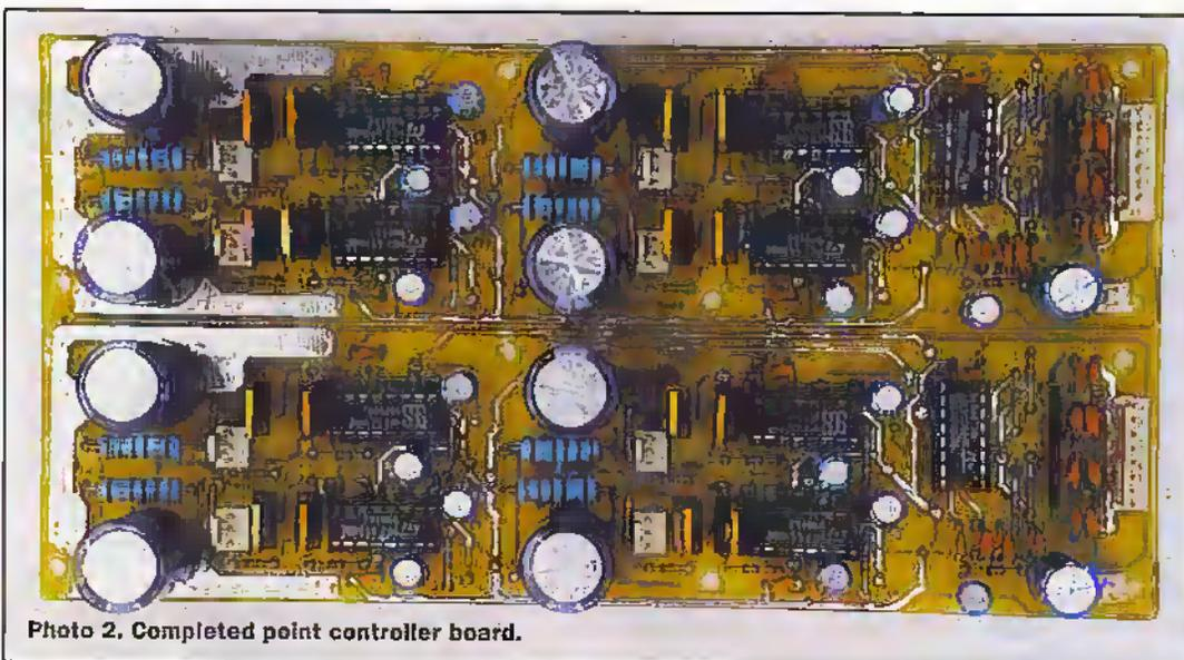
Photo 2. Completed point controller board.
