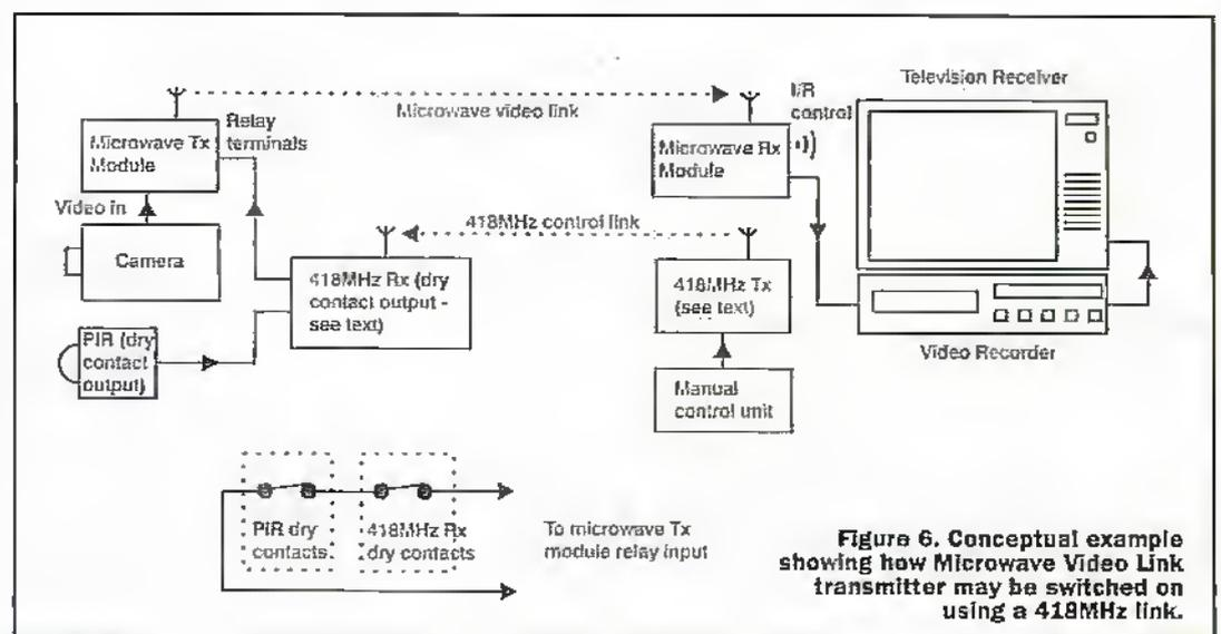
**Figure 6.** Conceptual example showing how Microwave Video Link transmitter may be switched on using a 418MHz link.
