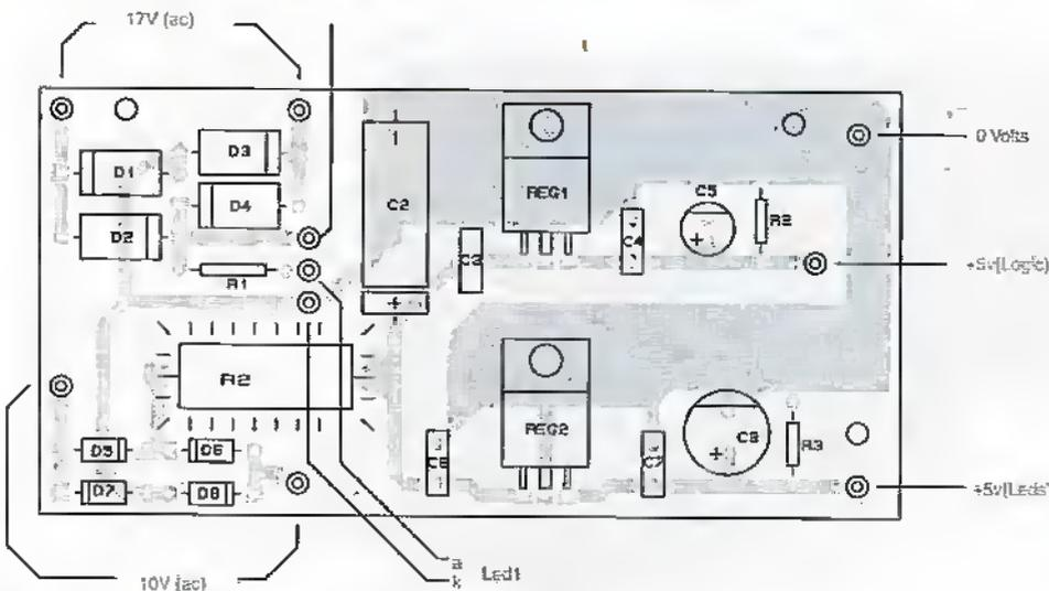
Figure 7. Component layout for PSU.
