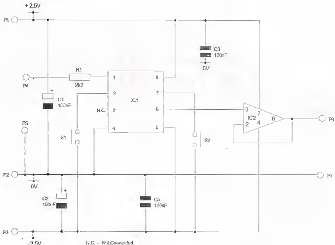
Figure 6. Using an op-amp to buffer the output.
