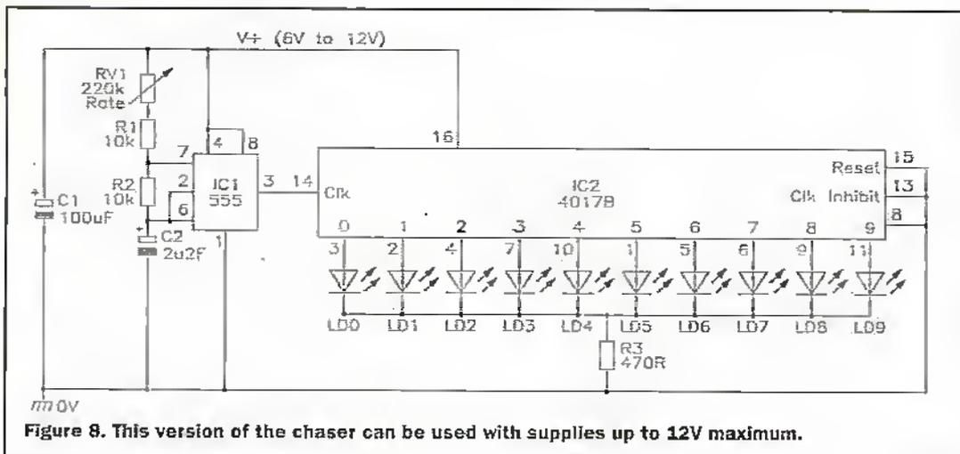
Figure 8. This version of the chaser can be used with supplies up to 12V maximum.
