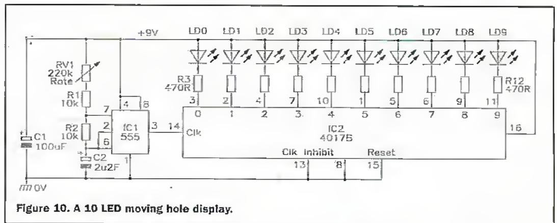
Figure 10. A 10 LED moving hole display.
