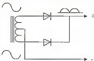
Figure 2e (i) Basic full wave rectifier analogy.
