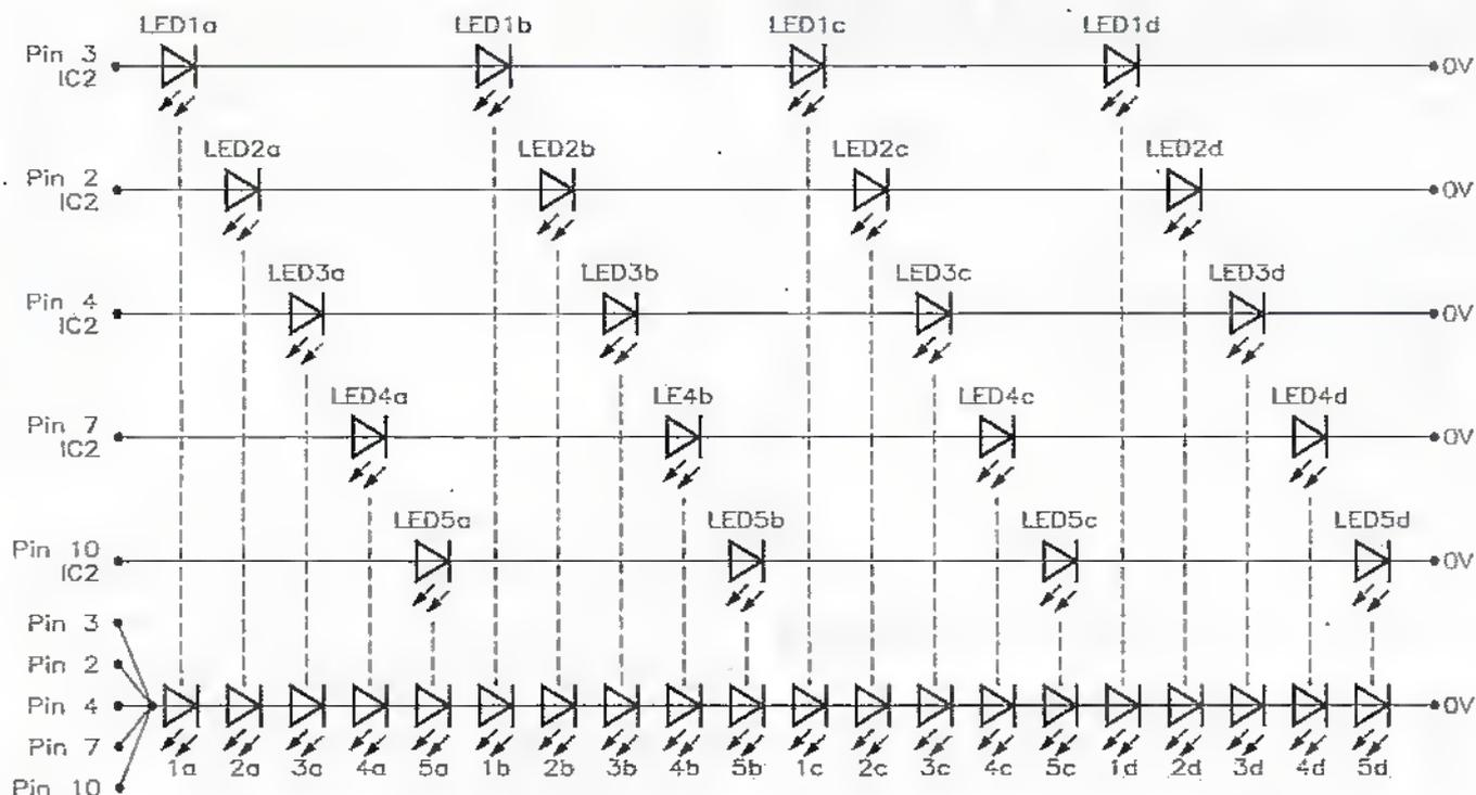
Figure 16. Basic method of constructing a 5-strand, 20-LED light rope display for use with the Figure 15 circuit.
