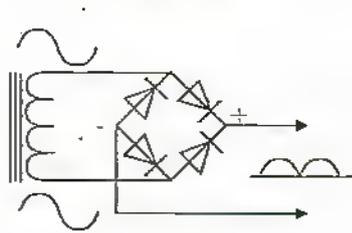
Figure 2e (ii) Full wave bridge analogy.
