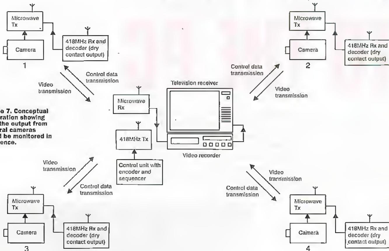
**Figure 7. Conceptual illustration showing how the output from several cameras could be monitored in sequence.**
