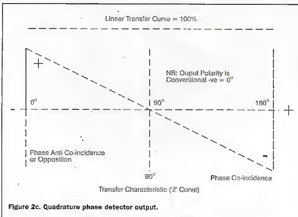
Figure 2c. Quadrature phase detector output.
