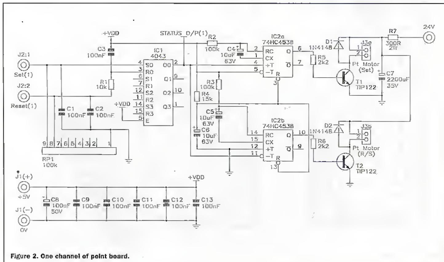
Figure 2. One channel of point board.
