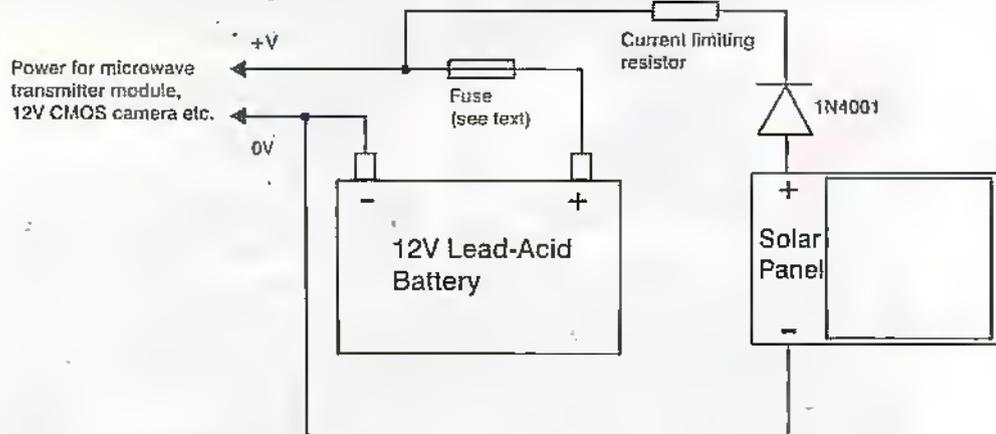
**Figure 8. Typical example of lead acid battery supply charged by solar panel.**
