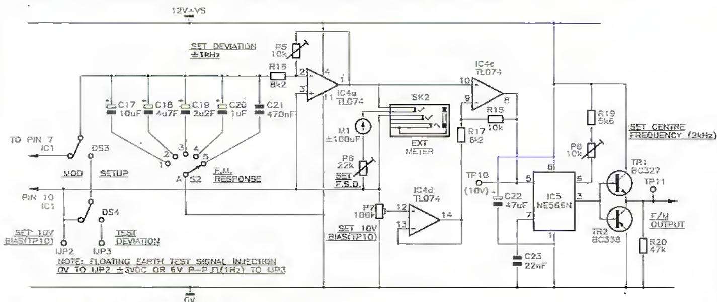
Figure 3. Frequency modulated channel.
