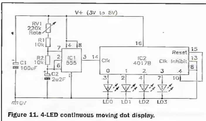
Figure 11. 4-LED continuous moving dot display.
