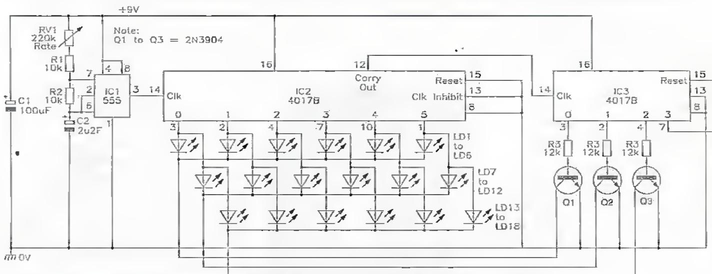
Figure 18. Multiplexed 6 LED x 3 line moving dot display. The dot moves intermittently along the lines.
