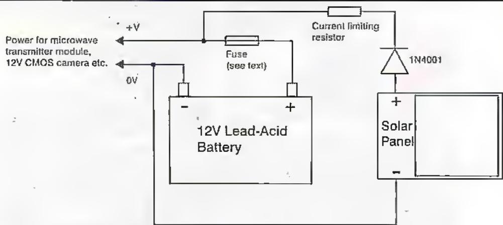
**Figure 8. Typical example of lead acid battery supply charged by solar panel.**
