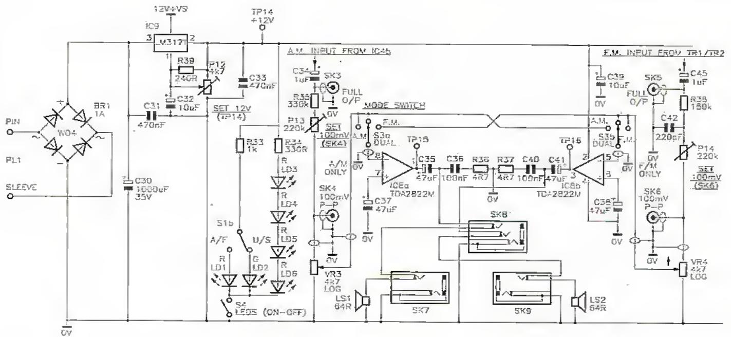
Figure 5. Power supply and output amplifier circuit.
