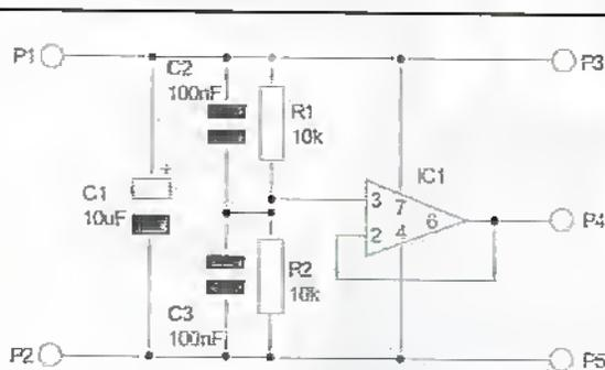
Figure 8. Using an op-amp to produce a centre reference voltage.
