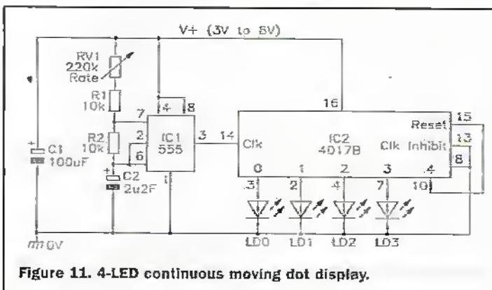
Figure 11. 4-LED continuous moving dot display.
