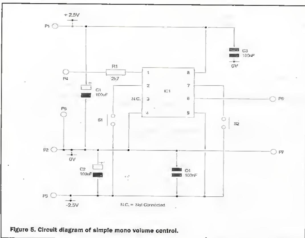
Figure 5. Circuit diagram of simple mono volume control.
