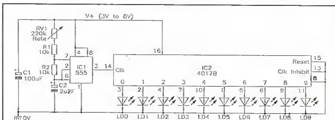
Figure 6. 10 LED chaser/sequencer can be used with supply voltages up to only 8V and produces a moving dot display.
