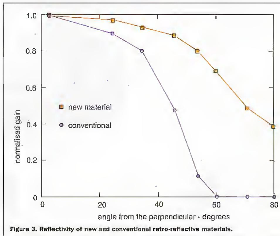
Figure 3. Reflectivity of new and conventional retro-reflective materials.
