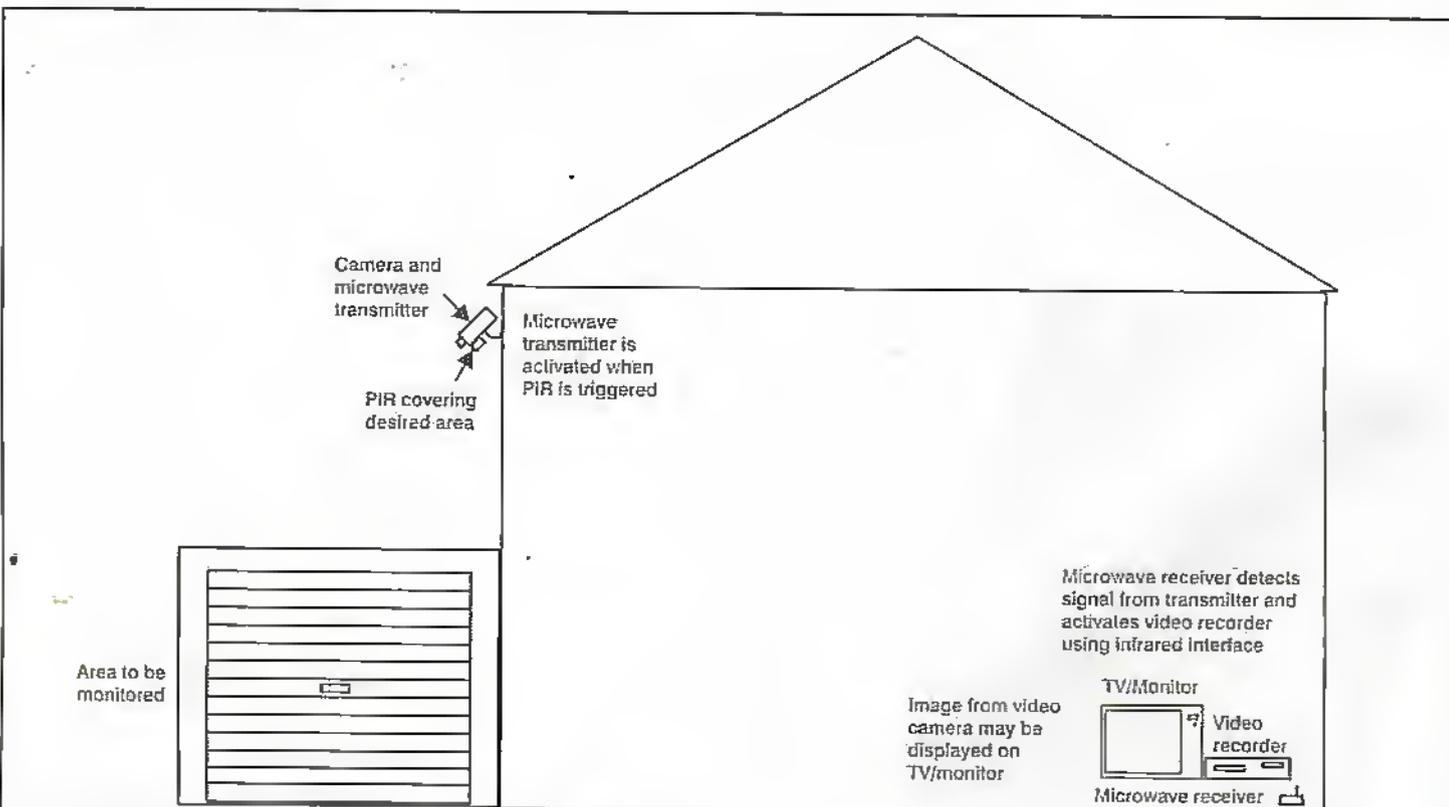
Figure 3. A typical application for the Microwave Video Link.
