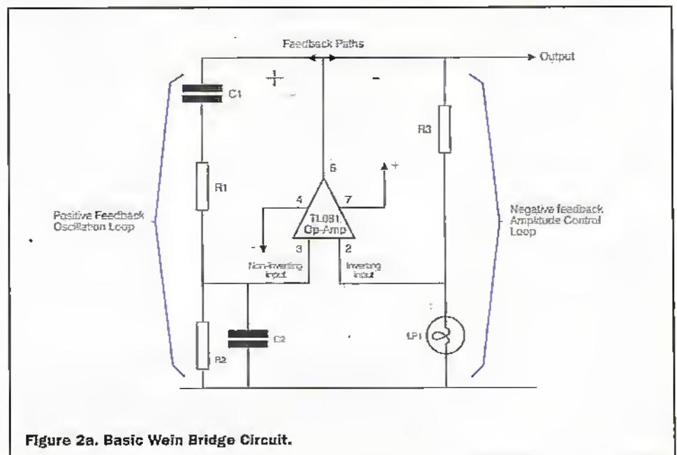
Figure 2a. Basic Wein Bridge Circuit.
