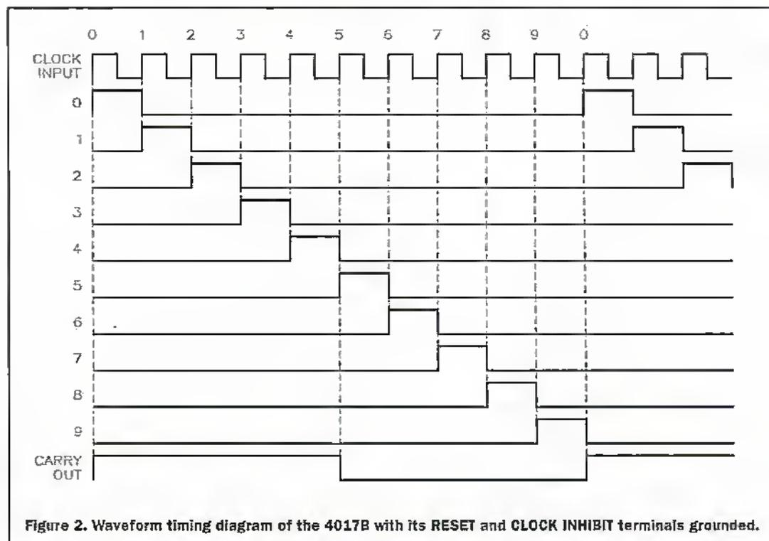
Figure 2. Waveform timing diagram of the 4017B with its RESET and CLOCK INHIBIT terminals grounded.
