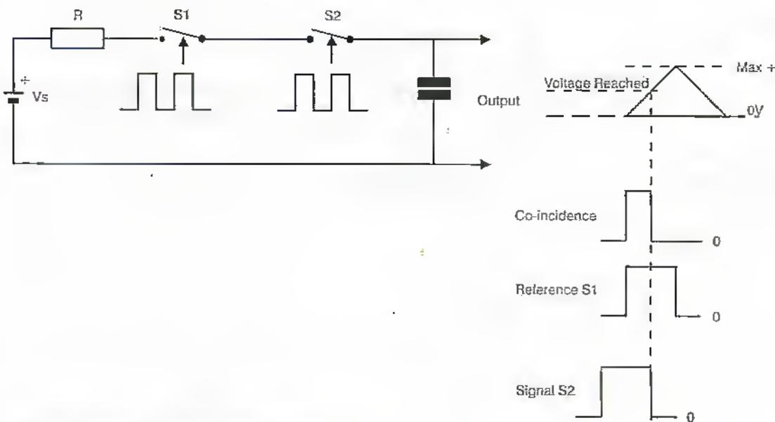
Figure 2d. Basic operation of a quadrature detector.
