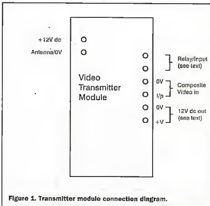
Figure 1. Transmitter module connection diagram.
