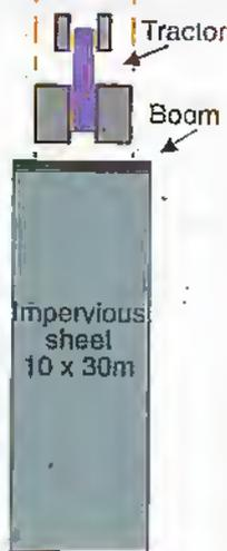
Figure 6. Sketch showing continuous application of nicotine vapour.
