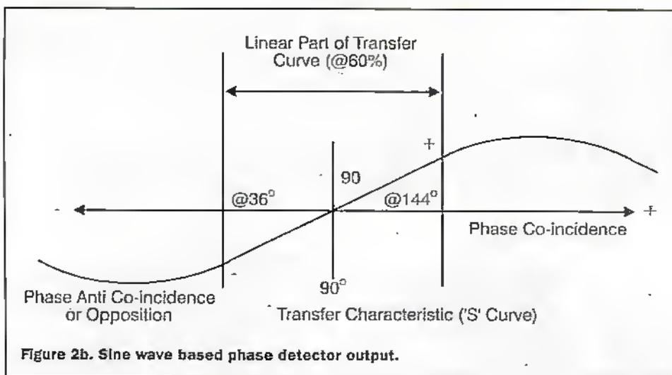
Figure 2b. Sine wave based phase detector output.
