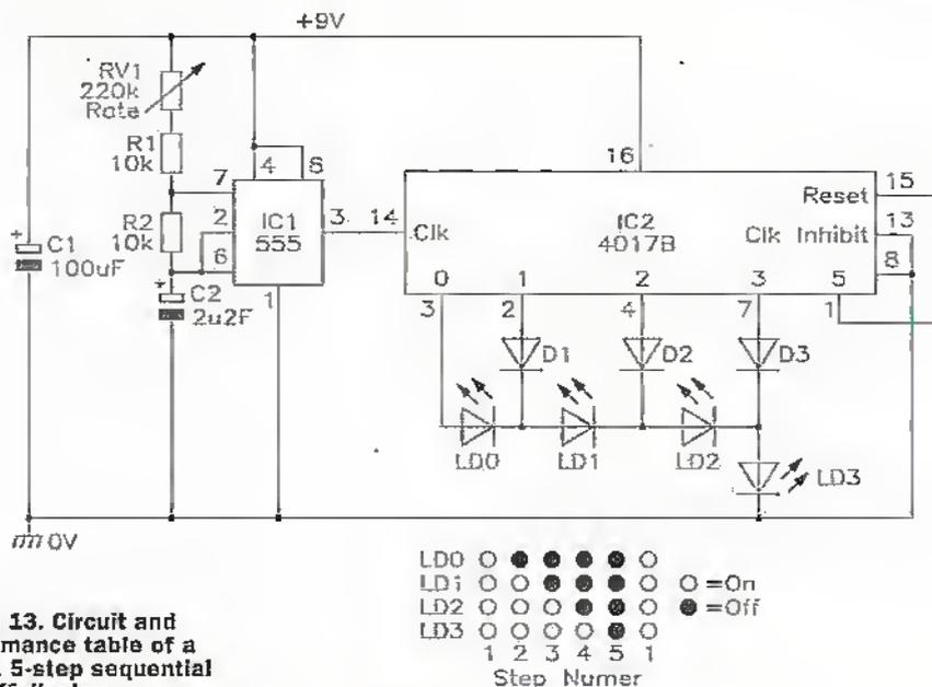
Figure 13. Circuit and performance table of a 4-LED, 5-step sequential turn off display.
