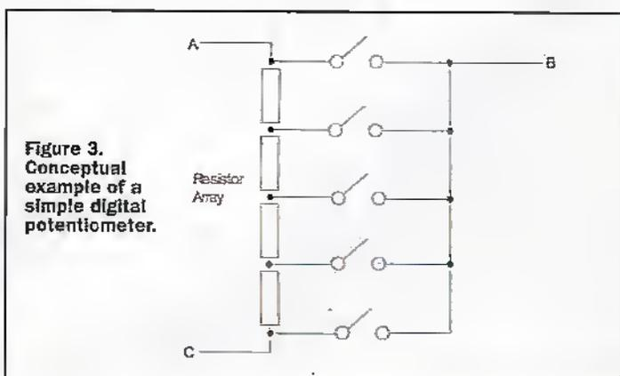
Figure 3. Conceptual example of a simple digital potentiometer.
