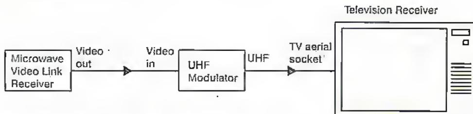
Figure 4. Using a UHF modulator to enable a composite video signal to be displayed on a standard television receiver.
