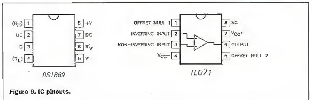
viewed from above, is pin 1 (see Figure 9). Although it is possible to solder directly to the IC's, it is sensible to use a DIL socket. This makes life so much easier, should it be necessary to replace the IC, and prevents the possibility of damaging the device during soldering due to overheating.
