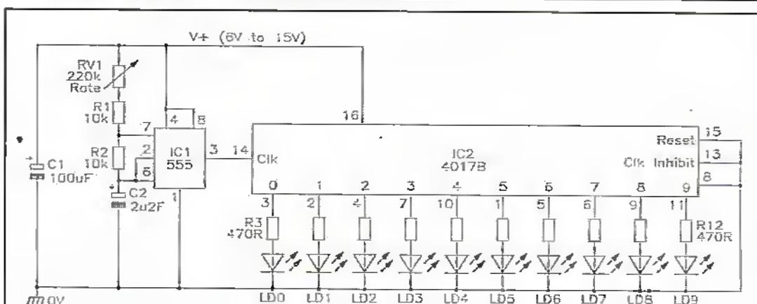
Figure 7. This version of the 10 LED chaser can be used with any supply up to 15V.
