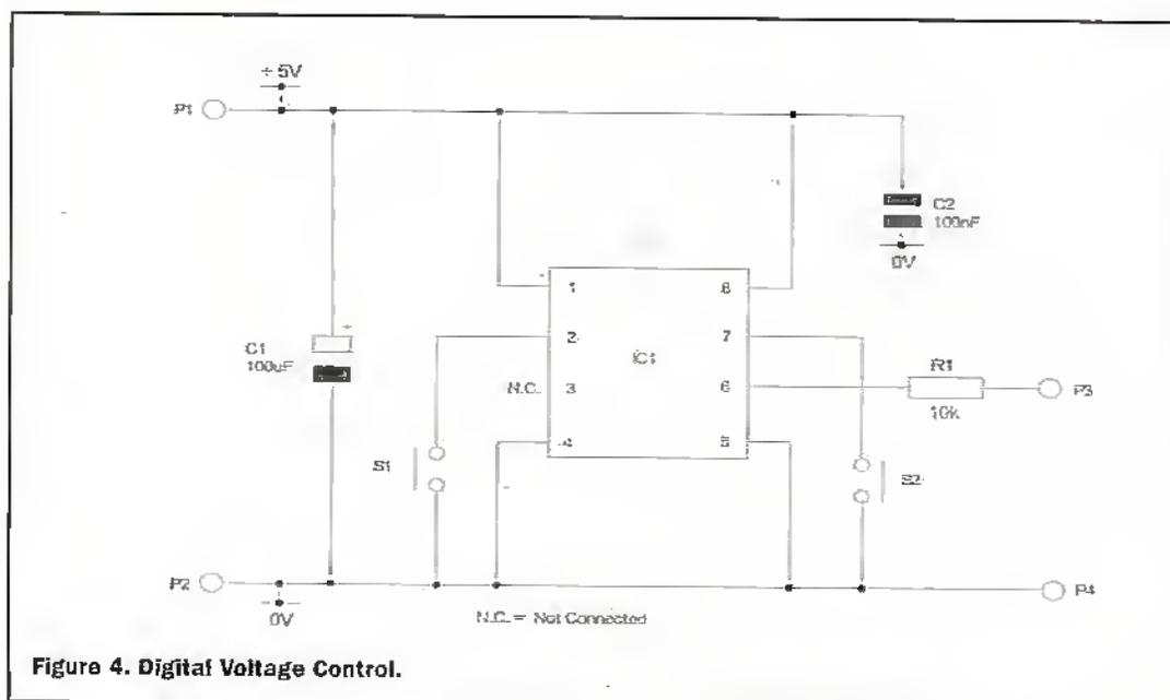
Figure 4. Digital Voltage Control.
