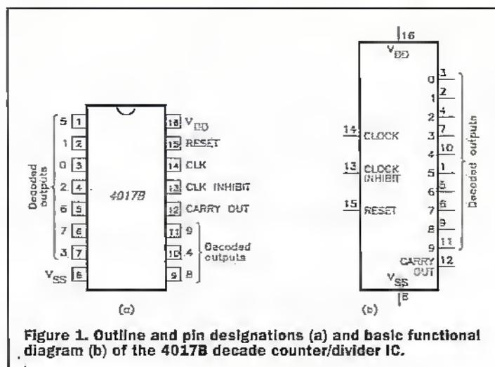
Figure 1. Outline and pin designations (a) and basic functional diagram (b) of the 4017B decade counter/divider IC.
