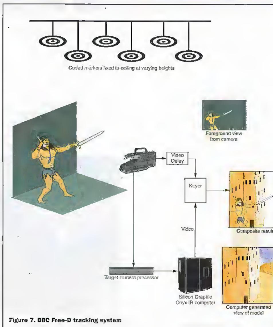
Figure 7. BBC Free-D tracking system
