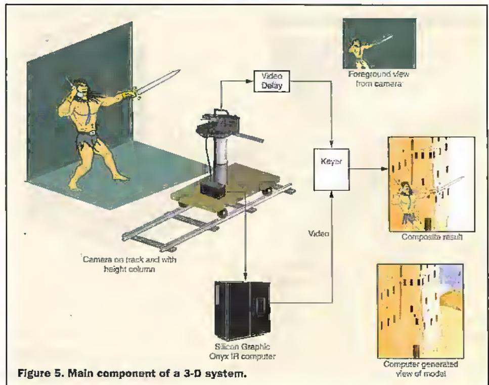
Figure 5. Main component of a 3-D system.
