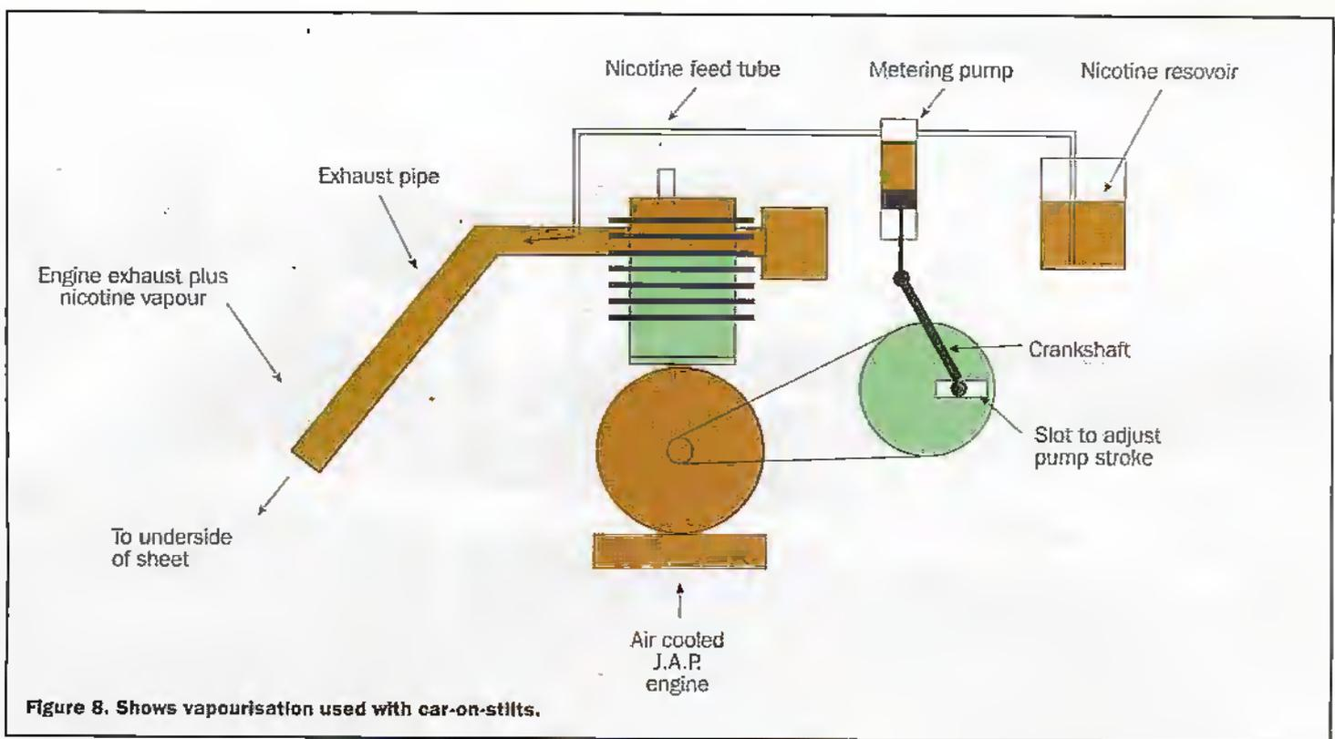
Figure 8. Shows vapourisation used with car-on-stilts.
