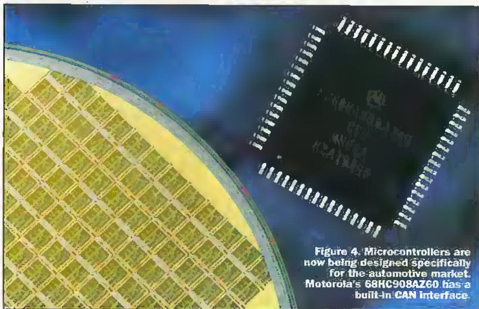
Figure 4. Microcontrollers are now being designed specifically for the automotive market. Motorola's 68HC908AZ60 has a built-in CAN interface.
