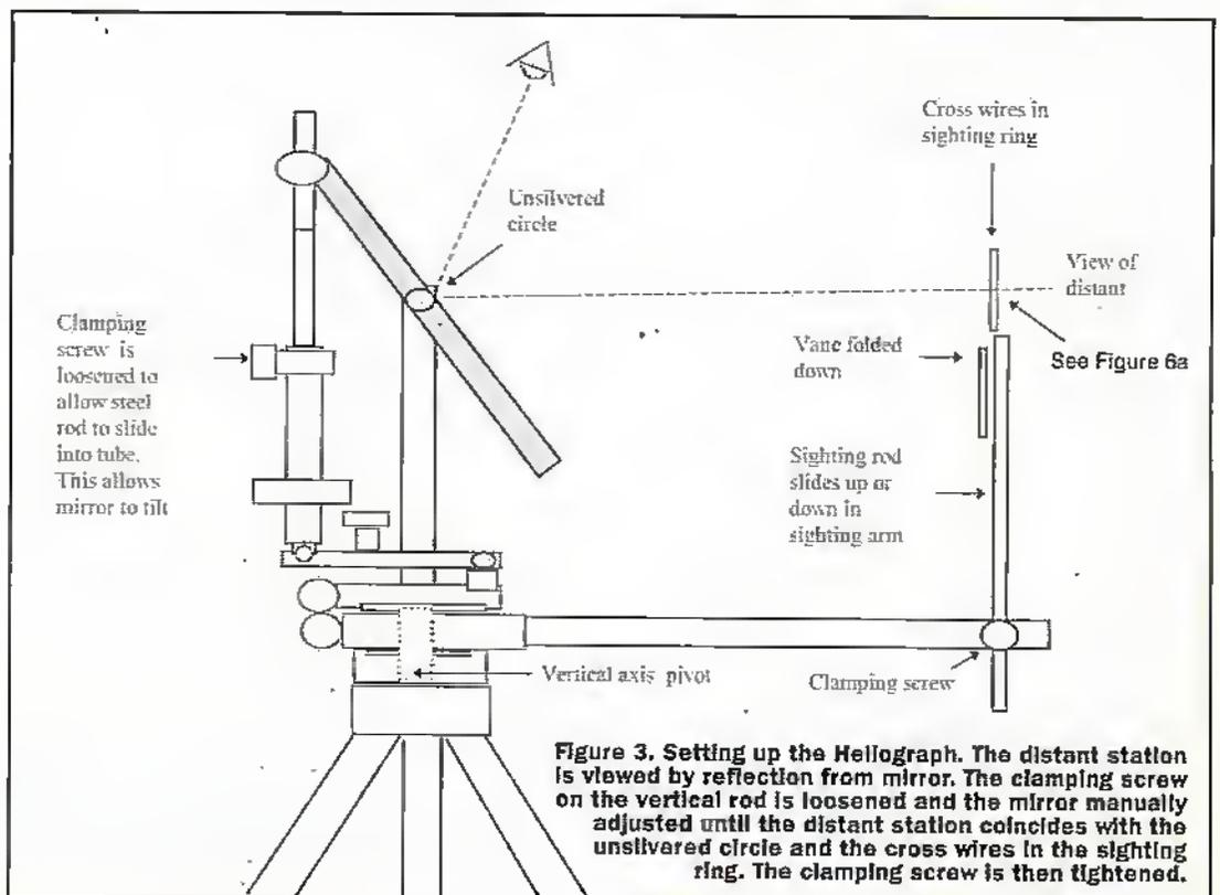
**Figure 3.** Setting up the Heliograph. The distant station is viewed by reflection from mirror. The clamping screw on the vertical rod is loosened and the mirror manually adjusted until the distant station coincides with the unsilvered circle and the cross wires in the sighting ring. The clamping screw is then tightened.
