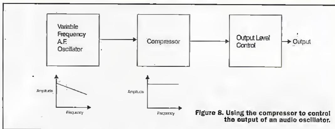
Figure 8. Using the compressor to control the output of an audio oscillator.
