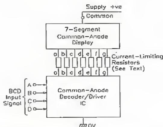
Figure 7. Method of driving a common-anode LED display.
