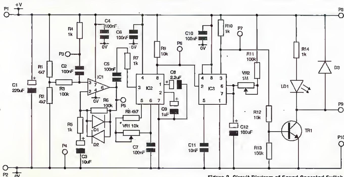
Figure 2. Circuit Diagram of Sound Operated Switch.
