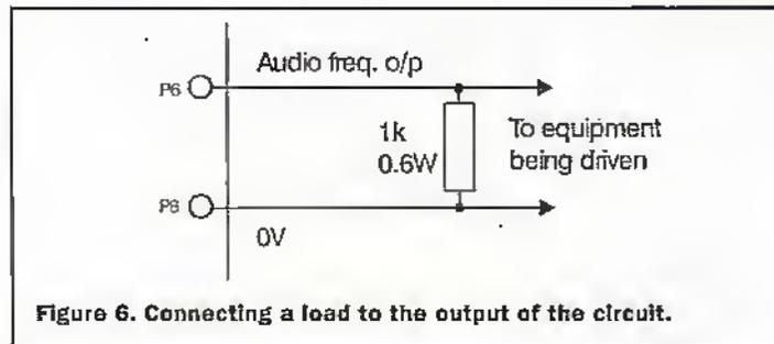
Figure 6. Connecting a load to the output of the circuit.
