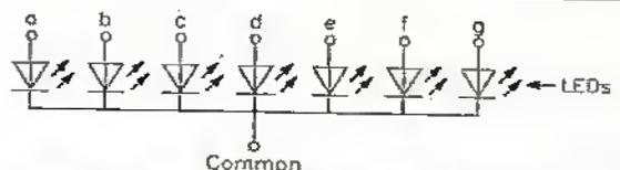
Figure 4. Schematic diagram of a common-cathode 7-segment LED display.
