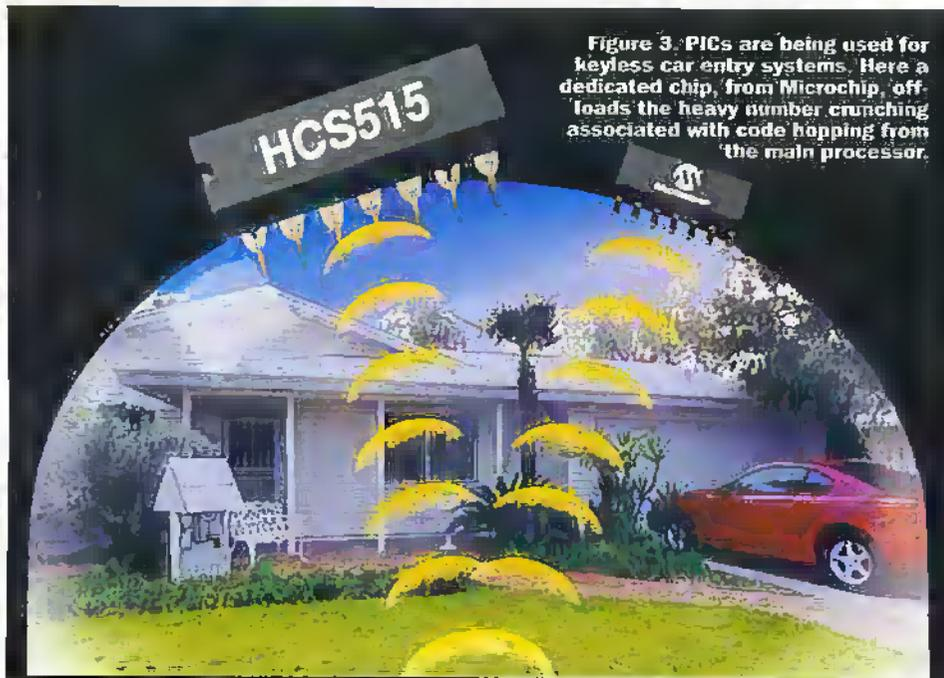
**Figure 3:** PICs are being used for keyless car entry systems. Here a dedicated chip, from Microchip, off-loads the heavy number crunching associated with code hopping from the main processor.
