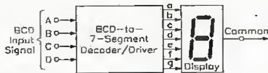
Figure 5. Basic connections of a BCD-to-7-segment decoder/driver IC.
