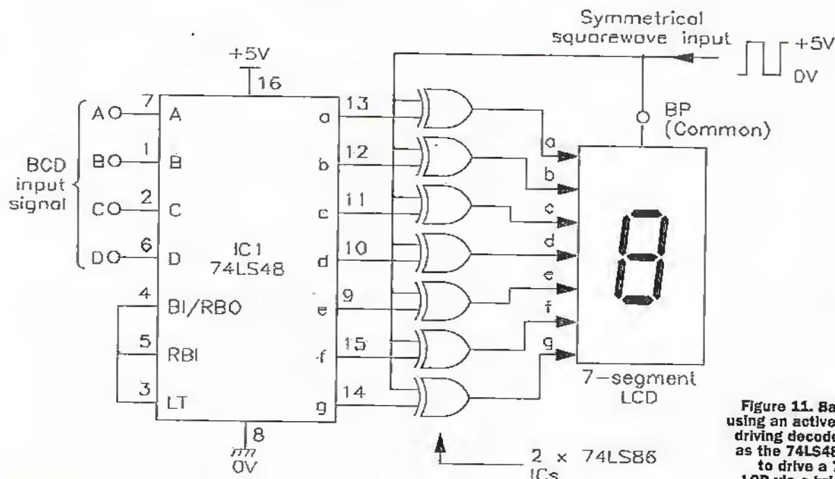
Figure 11. Basic way of using an active-high LED-driving decoder IC (such as the 74LS48 TTL type) to drive a 7-segment LCD via a bridge-driven 7-section EX-OR array.
