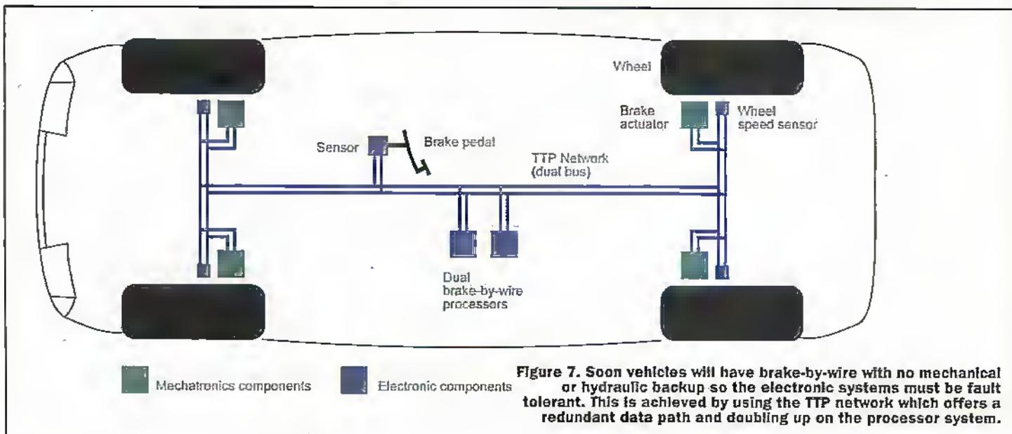
**Figure 7. Soon vehicles will have brake-by-wire with no mechanical or hydraulic backup so the electronic systems must be fault tolerant. This is achieved by using the TTP network which offers a redundant data path and doubling up on the processor system.**
