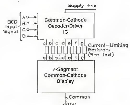
Figure 8. Method of driving a common-cathode LED display.
