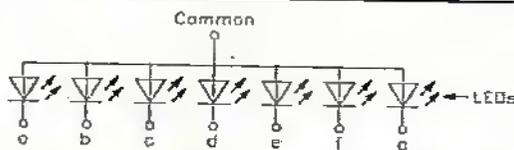
Figure 3. Schematic diagram of a common-anode 7-segment LED display.
