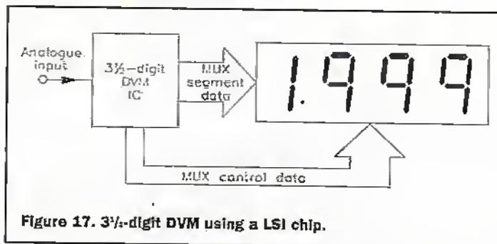
Figure 17. 3 1/2-digit DVM using a LSI chip.
