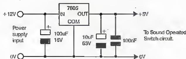
**Figure 7.** Example of how to use a voltage regulator.
