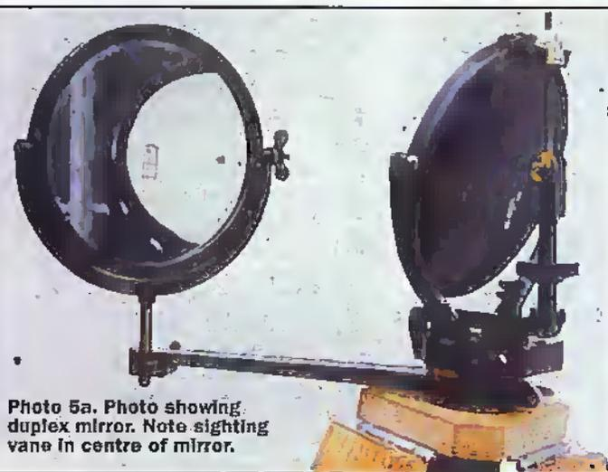
Photo 5a. Photo showing duplex mirror. Note sighting vane in centre of mirror.
