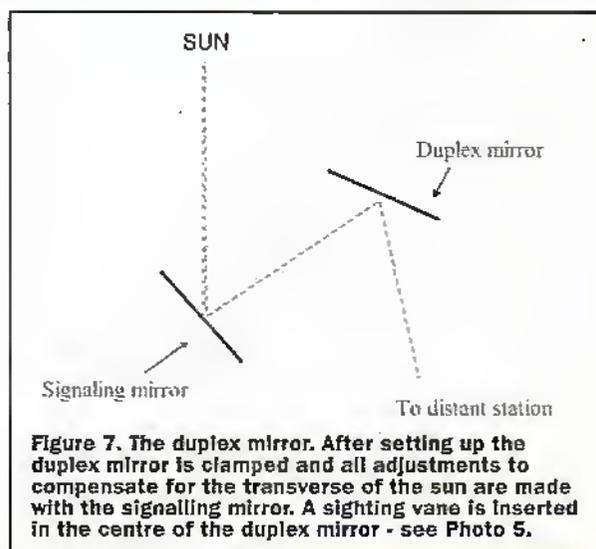
Figure 7. The duplex mirror. After setting up the duplex mirror is clamped and all adjustments to compensate for the transverse of the sun are made with the signalling mirror. A sighting vane is inserted in the centre of the duplex mirror - see Photo 5.
