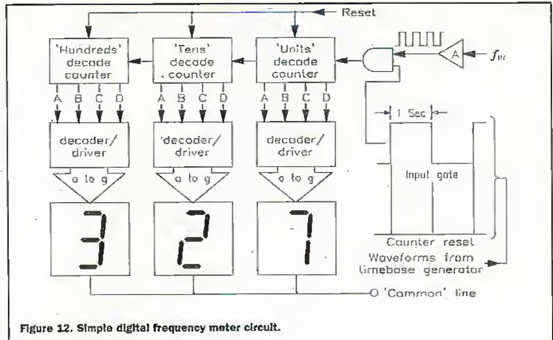
Figure 12. Simple digital frequency meter circuit.
