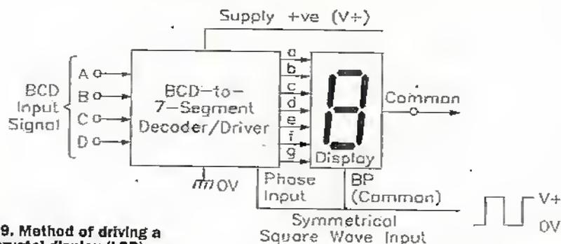
Figure 9. Method of driving a liquid-crystal display (LCD).
