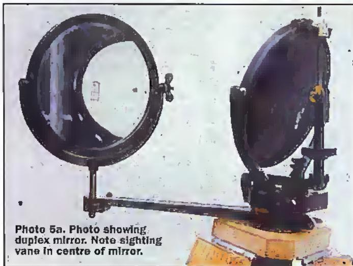
Photo 5a. Photo showing duplex mirror. Note sighting vane in centre of mirror.
