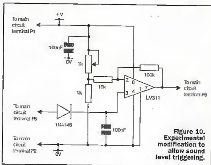
Figure 10. Experimental modification to allow sound level triggering.
