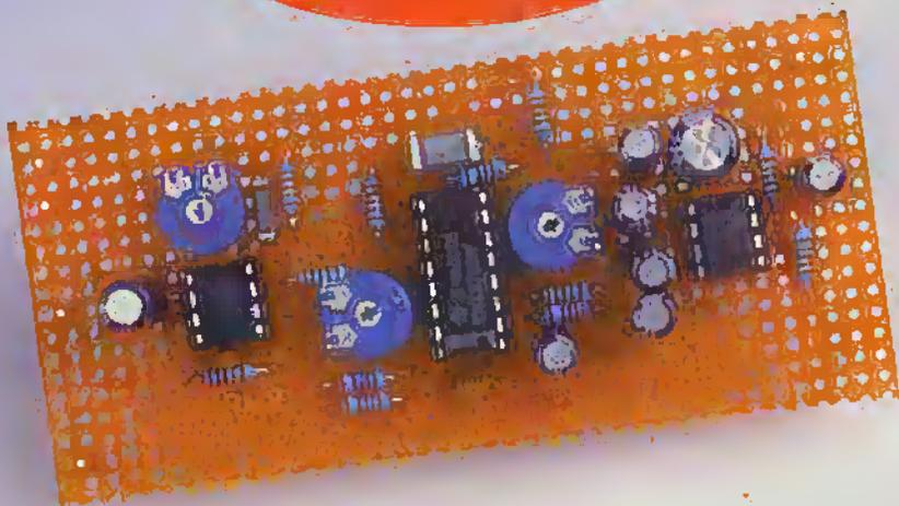
easy to use and is capable of good results. The circuit is designed as a general purpose building block that can be adapted for use in a variety of different applications. The block diagram of the unit is shown in Figure 2 for reference. The circuit uses two stages of compression to maintain a stable output level over a wide range of input voltages.
