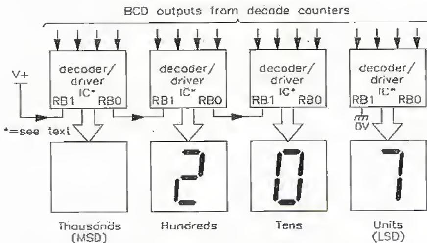
Figure 18. Ripple-blanking used to give leading-zero suppression in a 4-digit counter.
