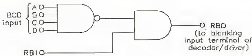
Figure 20. DIY ripple-blanking logic (active-high type).
