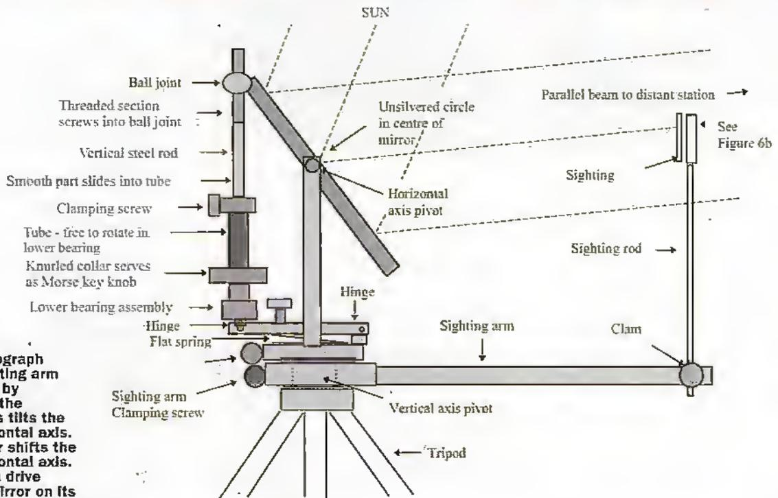
Figure 1. The Heliograph together with sighting arm and rod. Keying is by pressing down on the knurled collar. This tilts the mirror on its horizontal axis. Rotating the collar shifts the mirror on its horizontal axis. Rotating the worm drive knob, shifts the mirror on its vertical axis.
