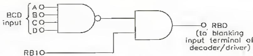
Figure 20. DIY ripple-blanking logic (active-high type).
