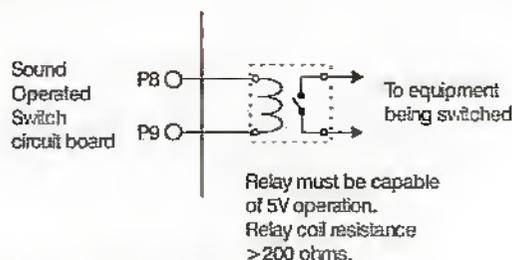
**Figure 8.** Connecting a relay.
