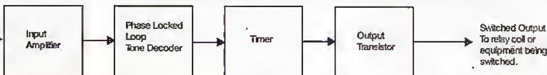
Figure 1. Block Diagram of Sound Operated Switch.
