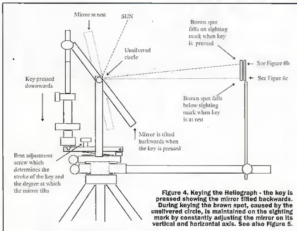
Figure 4. Keying the Heliograph - the key is pressed showing the mirror tilted backwards. During keying the brown spot, caused by the unsilvered circle, is maintained on the sighting mark by constantly adjusting the mirror on its vertical and horizontal axes. See also Figure 5.
