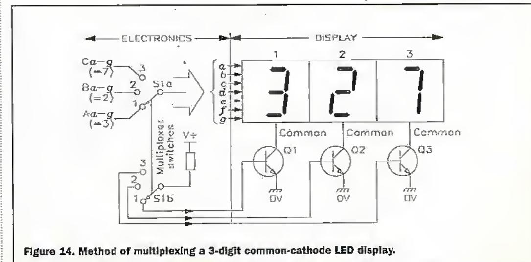
Figure 14. Method of multiplexing a 3-digit common-cathode LED display.
