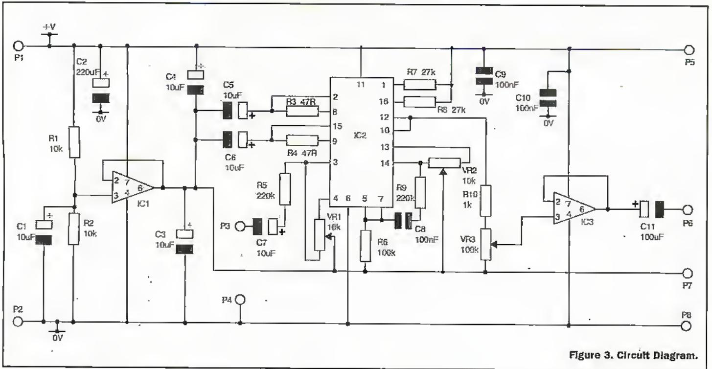
Figure 3. Circuit Diagram.
