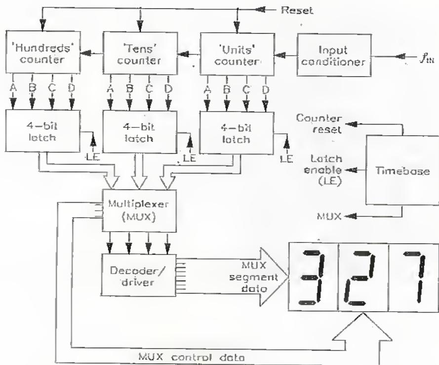
Figure 15. Realistic implementation of the multiplexing technique in a 3-digit frequency meter.
