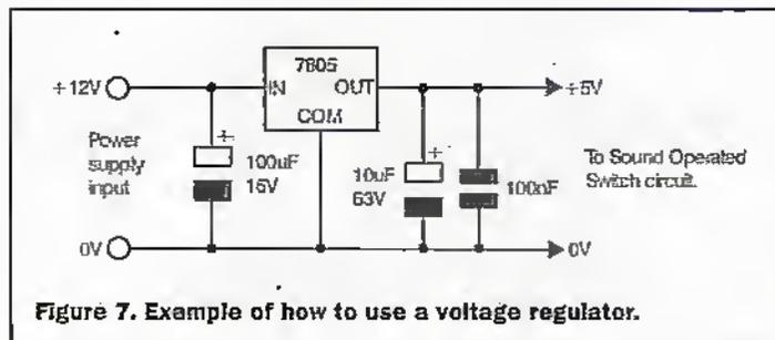
**Figure 7.** Example of how to use a voltage regulator.
