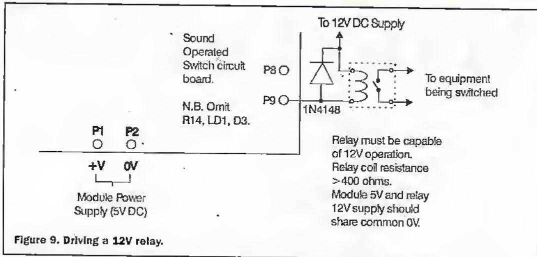
Figure 9. Driving a 12V relay.
