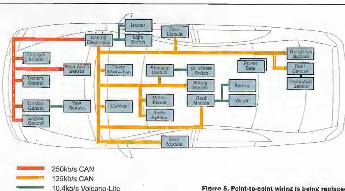
Figure 5. Point-to-point wiring is being replaced by vehicle networks. Volvo's S80 has three separate networks.
