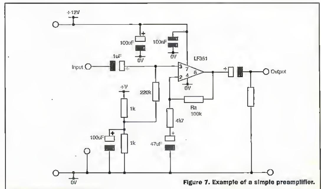
Figure 7. Example of a simple preamplifier.
