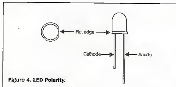
Figure 4. LED Polarity.
