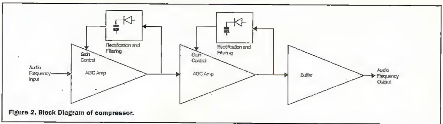
Figure 2. Block Diagram of compressor.
