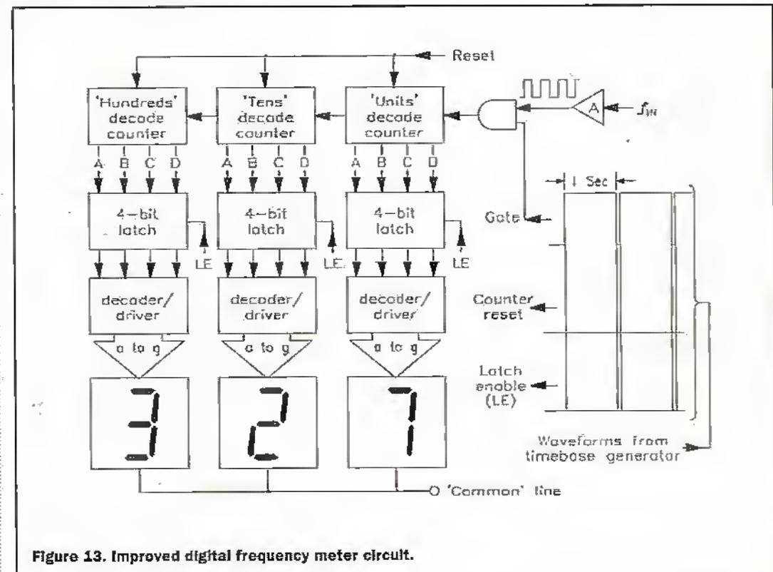
Figure 13. Improved digital frequency meter circuit.
