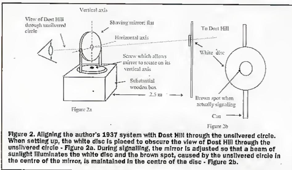
**Figure 2.** Aligning the author's 1937 system with Dost Hill through the unsilvered circle. When setting up, the white disc is placed to obscure the view of Dost Hill through the unsilvered circle - Figure 2a. During signaling, the mirror is adjusted so that a beam of sunlight illuminates the white disc and the brown spot, caused by the unsilvered circle in the centre of the mirror, is maintained in the centre of the disc - Figure 2b.
