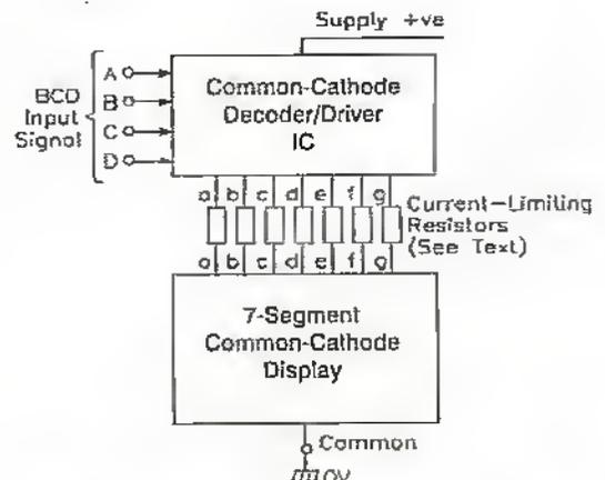
Figure 8. Method of driving a common-cathode LED display.
