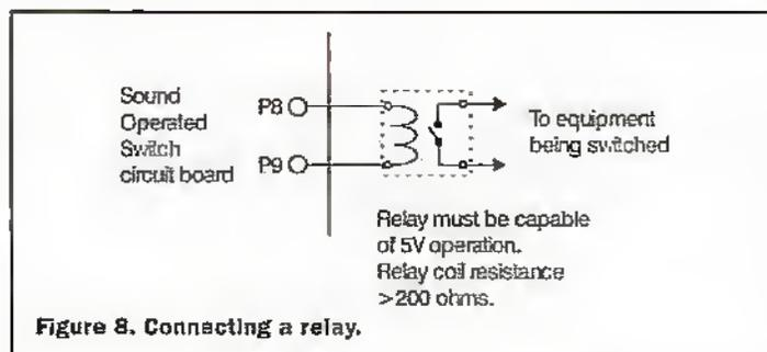
**Figure 8.** Connecting a relay.
