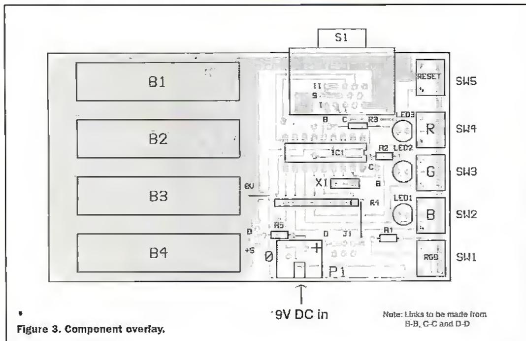
Figure 3. Component overlay.
