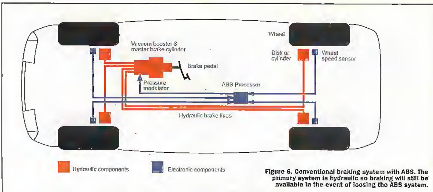
**Figure 6. Conventional braking system with ABS. The primary system is hydraulic so braking will still be available in the event of losing the ABS system.**
