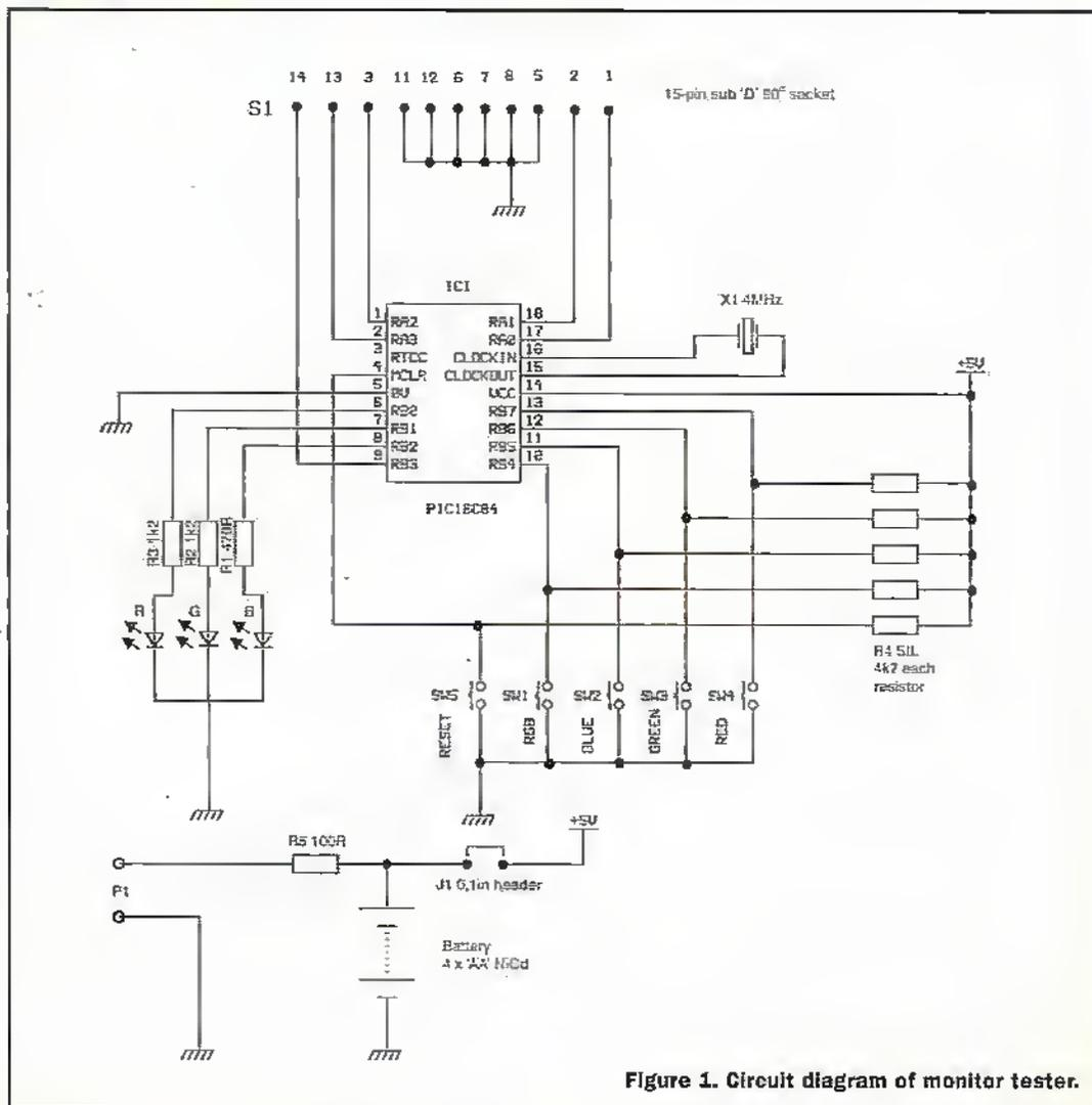
Figure 1. Circuit diagram of monitor tester.
