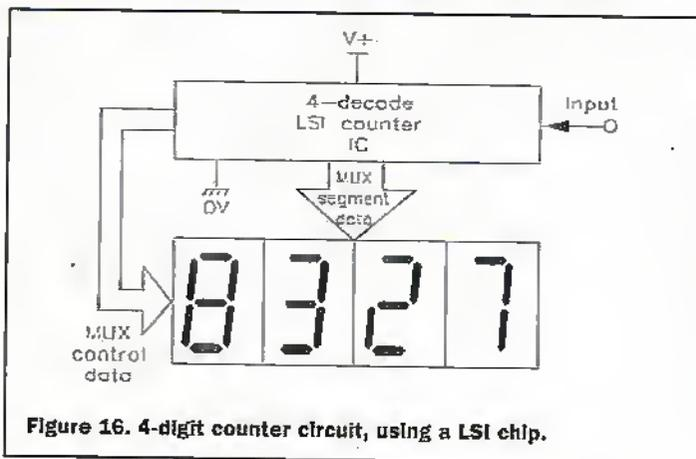
Figure 16. 4-digit counter circuit, using a LSI chip.
