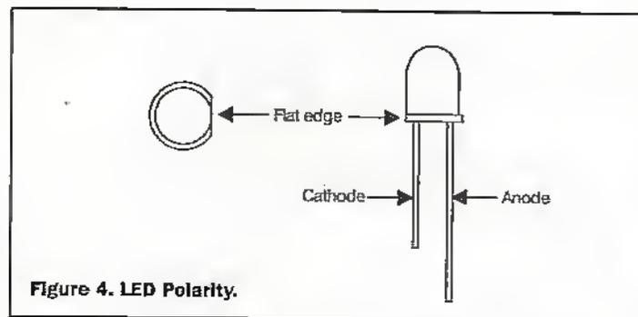
Figure 4. LED Polarity.
