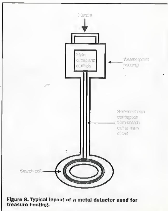
Figure 8. Typical layout of a metal detector used for treasure hunting.
