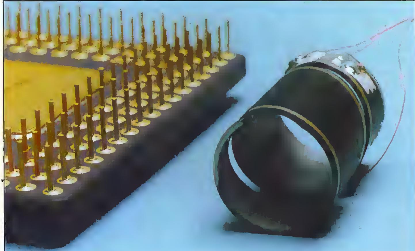
Photo 5. The electronic spring which contracts on the application of a voltage will form the basis of the transducer in the DLS.
