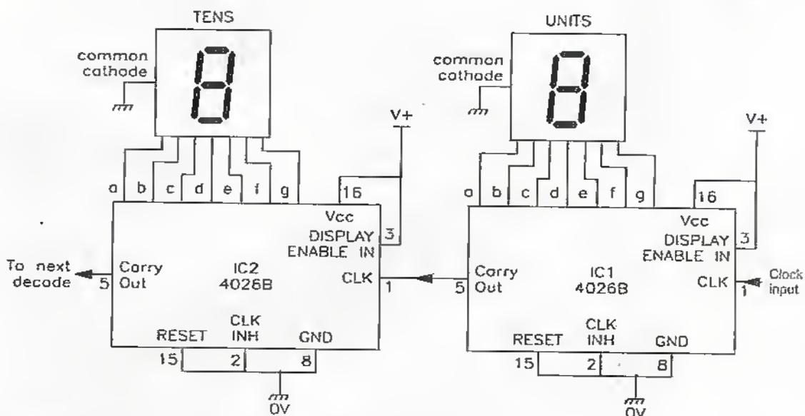
Figure 15. Basic method of cascading 4026B ICs.
