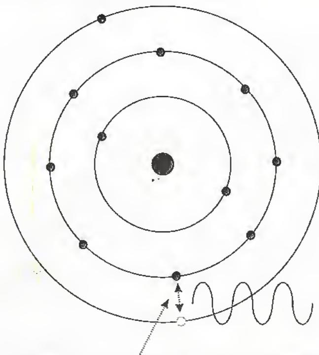
If an electron absorbs enough energy to 'jump' from one shell, or energy level to another, it will 'fall back' to its original level, emitting energy at a frequency which is a measure of that energy.
