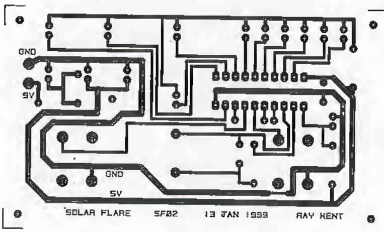
Figure 3. PCB track layout.
