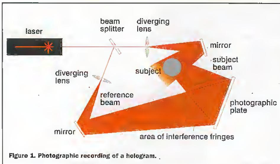
two beams are made to coincide on a very high resolution film. This pattern can be recorded photographically. See Figure 1.
