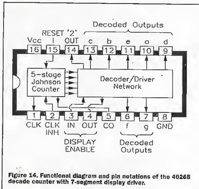
Figure 14. Functional diagram and pin notations of the 4026B decade counter with 7-segment display driver.
