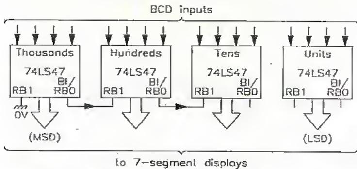
Figure 3. Method of applying leading-zero suppression to the first three digits of a 4-digit display using 74LS47 ICs.
