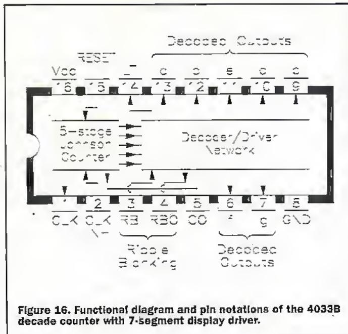
Figure 16. Functional diagram and pin notations of the 4033B decade counter with 7-segment display driver.
