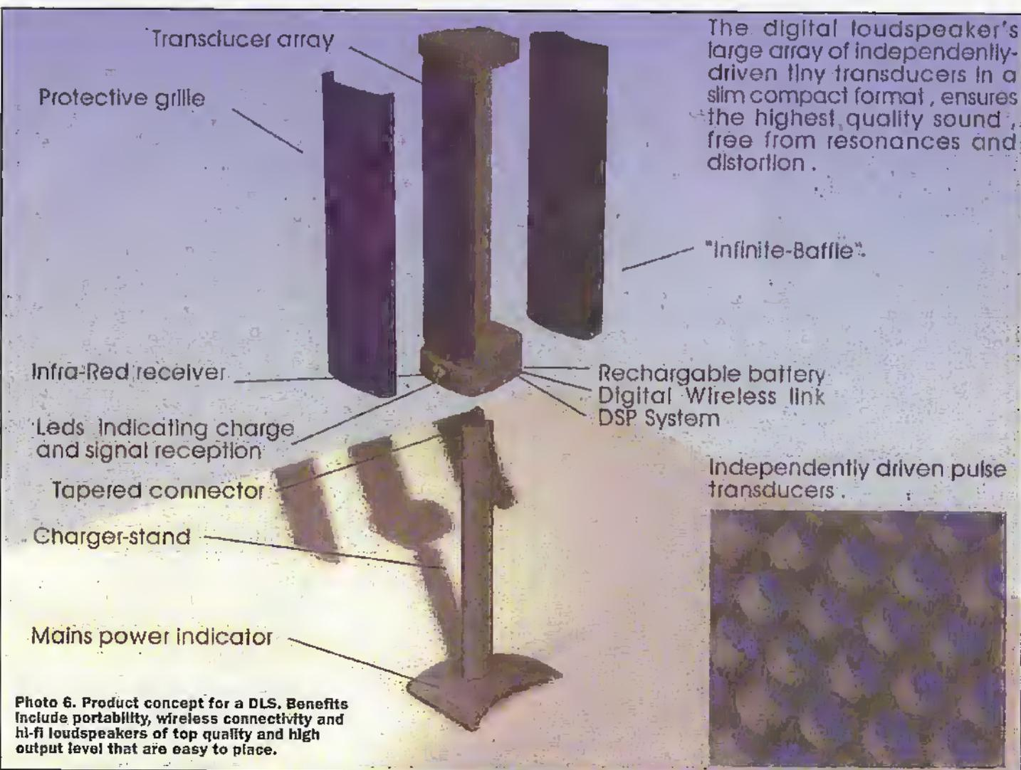
The digital loudspeaker's large array of independently-driven tiny transducers in a slim compact format, ensures the highest quality sound, free from resonances and distortion.
