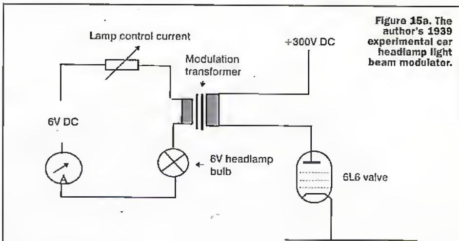
Figure 15a. The author's 1939 experimental car headlamp light beam modulator.
