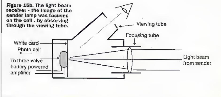
Figure 15b. The light beam receiver - the image of the sender lamp was focused on the cell by observing through the viewing tube.
