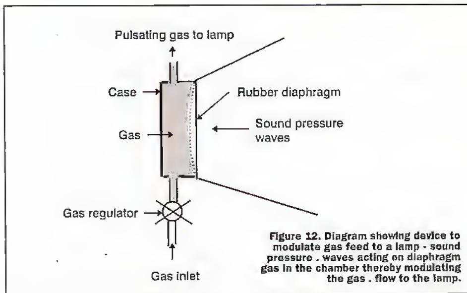
Figure 12. Diagram showing device to modulate gas feed to a lamp - sound pressure waves acting on diaphragm gas in the chamber thereby modulating the gas flow to the lamp.
