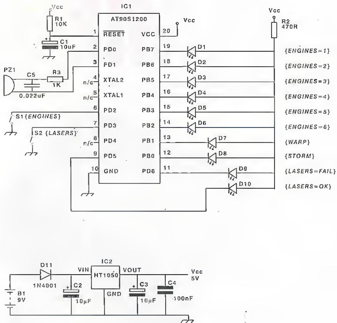
Figure 1. Complete circuit for 'Solar Flare'.
