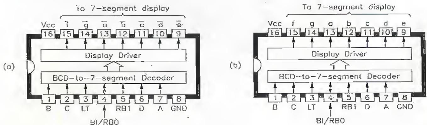
Figure 1. Functional diagram of the (a) 74LS47 and (b) 74LS48 BCD-to-7-segment decoder/driver ICs.
