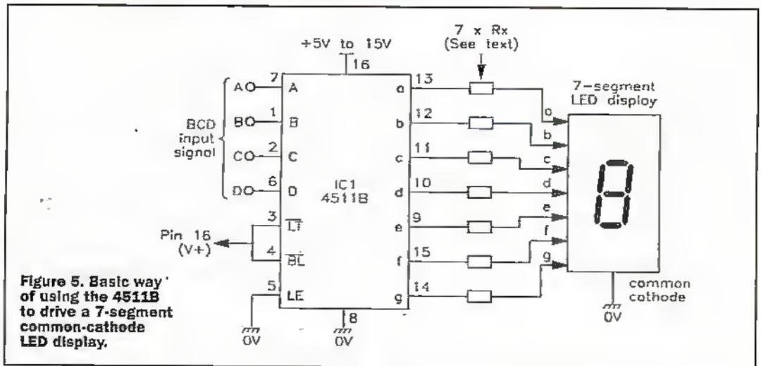
Figure 5. Basic way of using the 4511B to drive a 7-segment common-cathode LED display.
