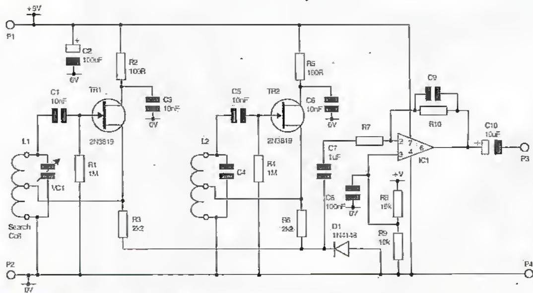
Figure 2. Illustrative example of Beat Frequency metal detector circuit.
