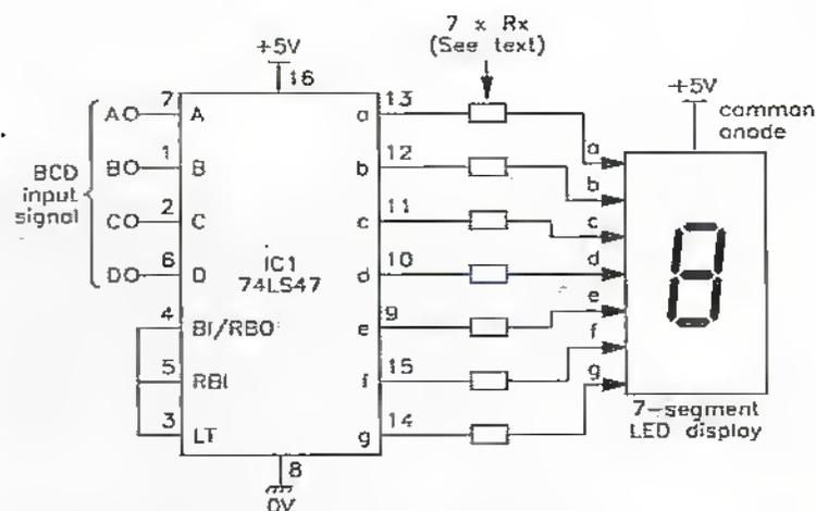
Figure 2. Basic way of using a 74LS47 IC to drive a common-anode LED display.
