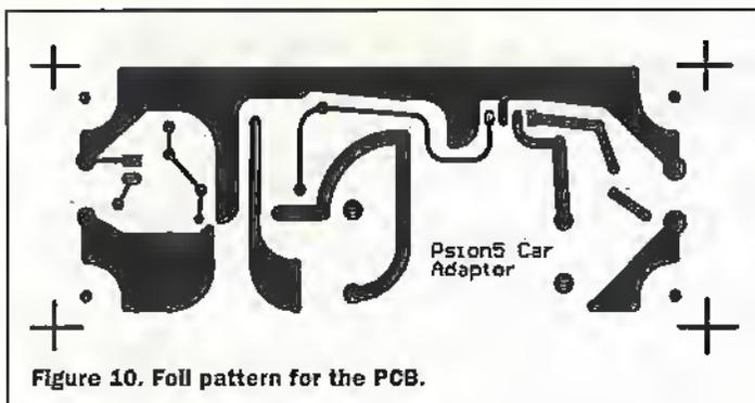
Figure 10. Foil pattern for the PCB.
