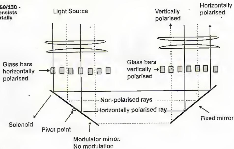
**Figure 16b. With maximum modulation - modulator mirror now moved so that rays horizontally polarised by the first polariser are blocked by the second polariser. N.B. The rays actually converge on to a single very small mirror, in an arrangement similar to Figure 9a. Drawings are shown for clarity.**
