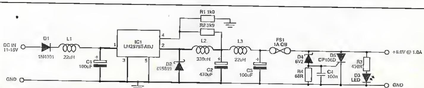
**Figure 9. Putting it all together. Note the critical paths marked with extra thick lines.**
