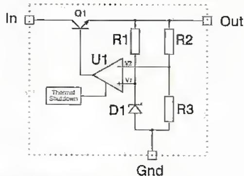
Figure 1. Three terminal regulator: unsung hero of the electronics age.
