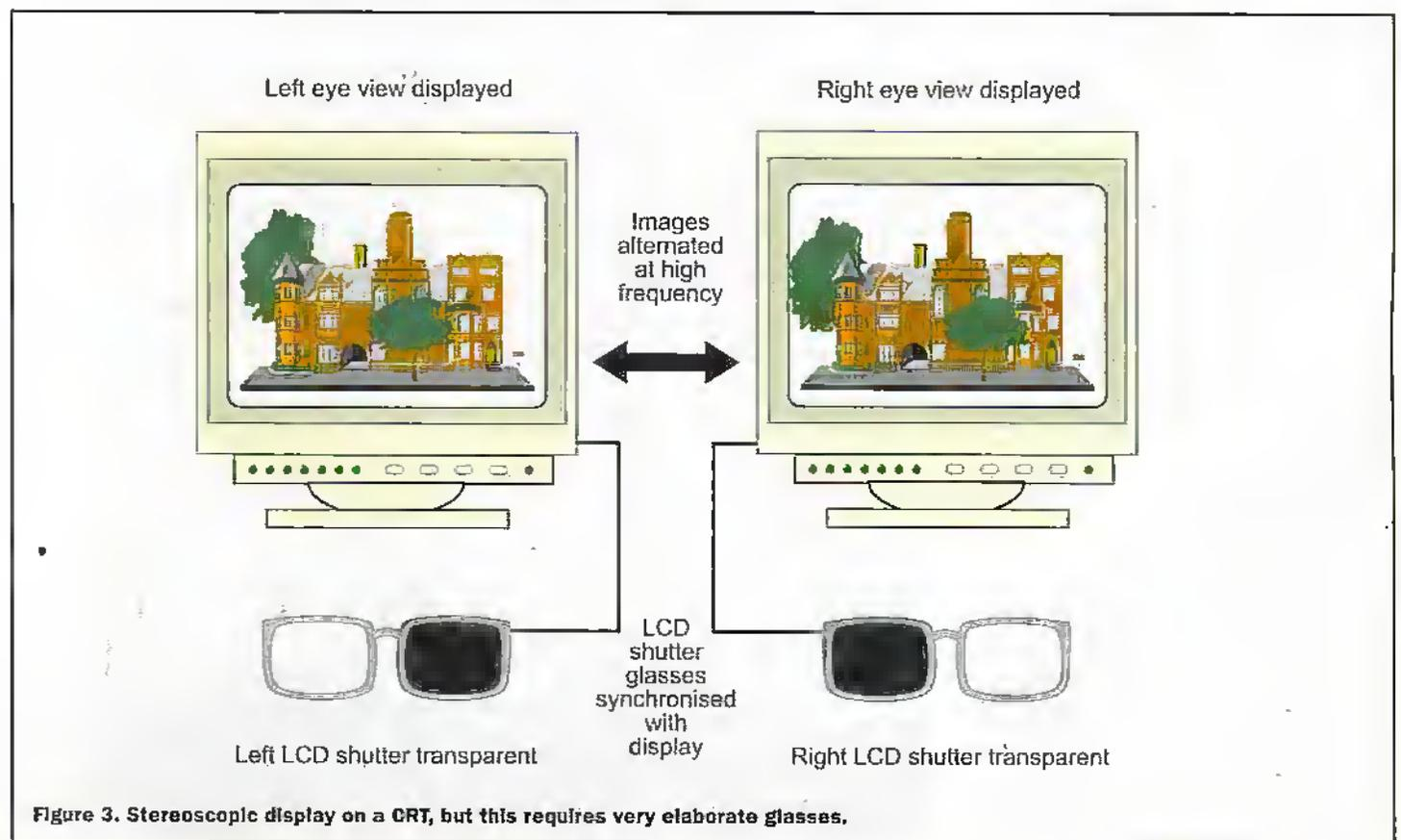
Figure 3. Stereoscopic display on a CRT, but this requires very elaborate glasses.
