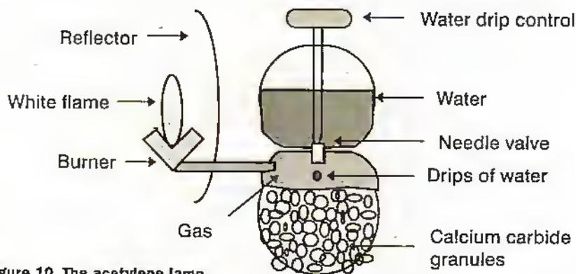
**Figure 10.** The acetylene lamp.
