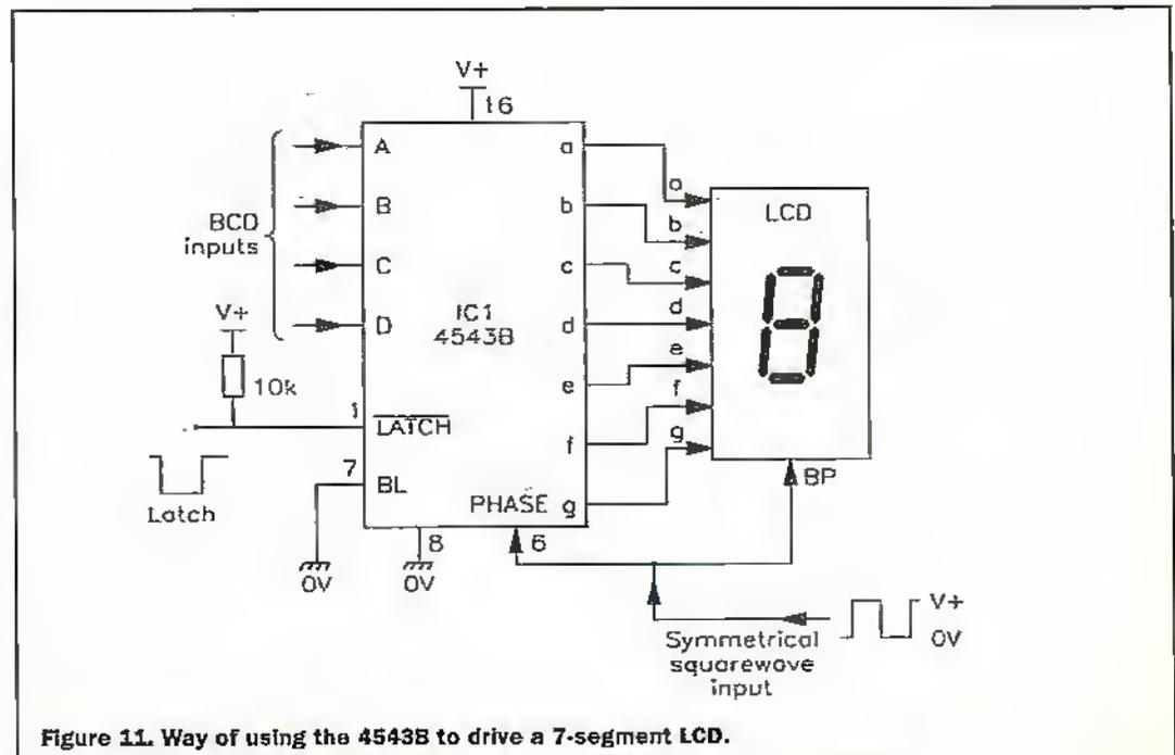
Figure 11. Way of using the 4543B to drive a 7-segment LCD.
