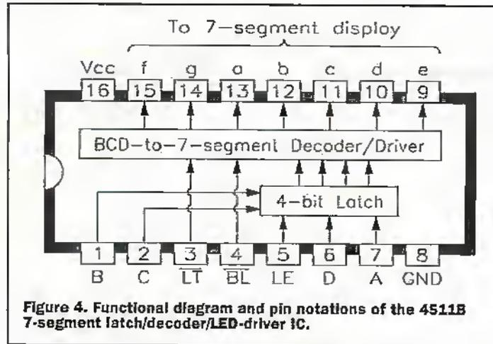
Figure 4. Functional diagram and pin notations of the 4511B 7-segment latch/decoder/LED-driver IC.
