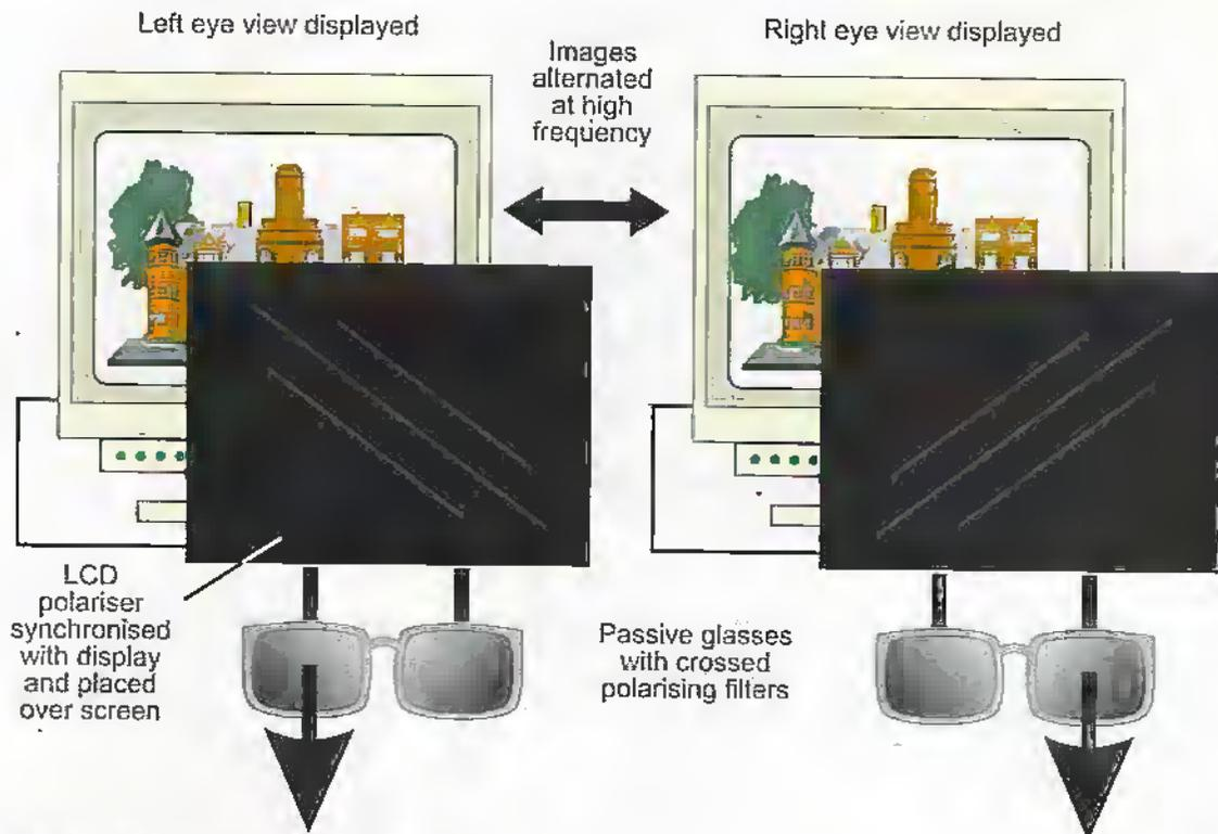
Figure 4. Stereoscopic display using passive glasses.
