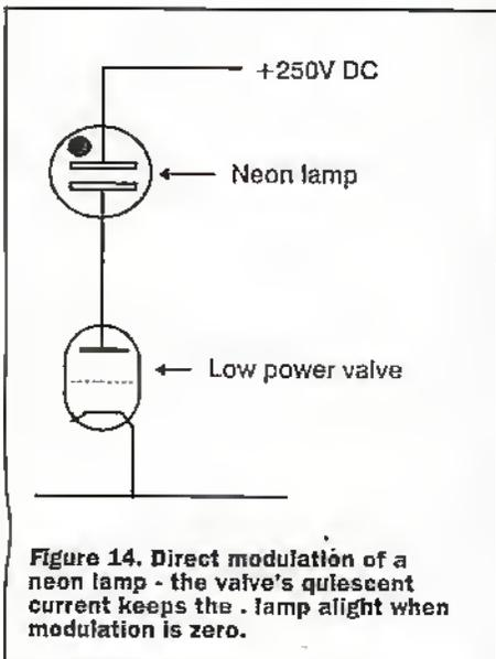
Figure 14. Direct modulation of a neon lamp - the valve's quiescent current keeps the lamp alight when modulation is zero.
