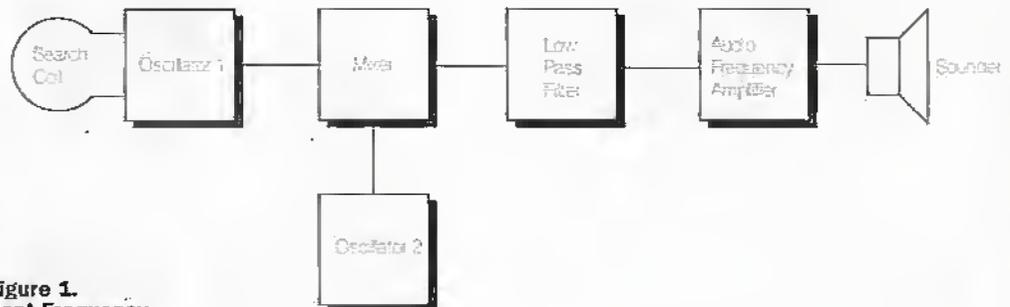
Figure 1. Beat Frequency metal detector block diagram.
