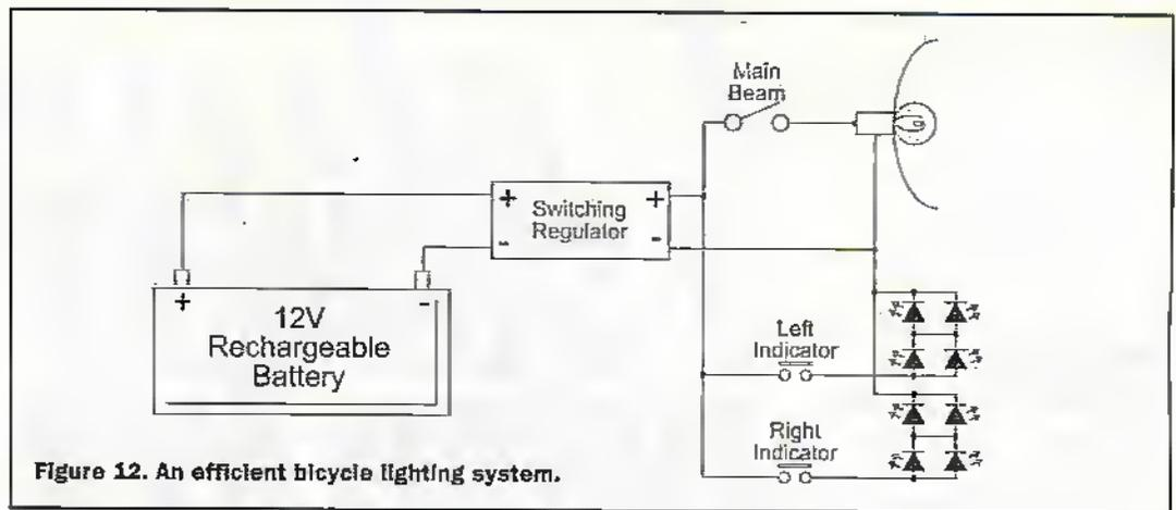
Figure 12. An efficient bicycle lighting system.
