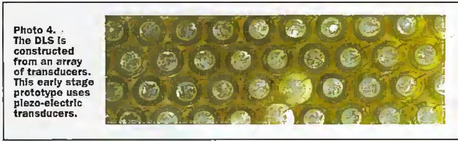
Photo 4. The DLS is constructed from an array of transducers. This early stage prototype uses piezo-electric transducers.
