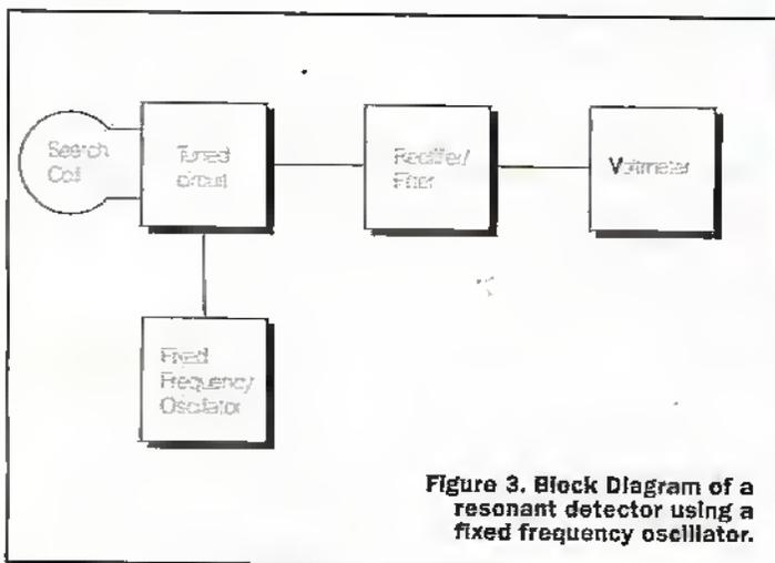
Figure 3. Block Diagram of a resonant detector using a fixed frequency oscillator.
