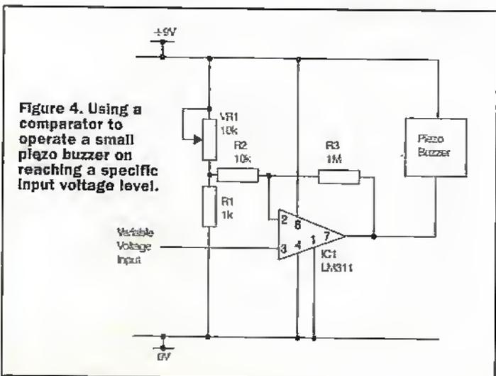
Figure 4. Using a comparator to operate a small piezo buzzer on reaching a specific input voltage level.
