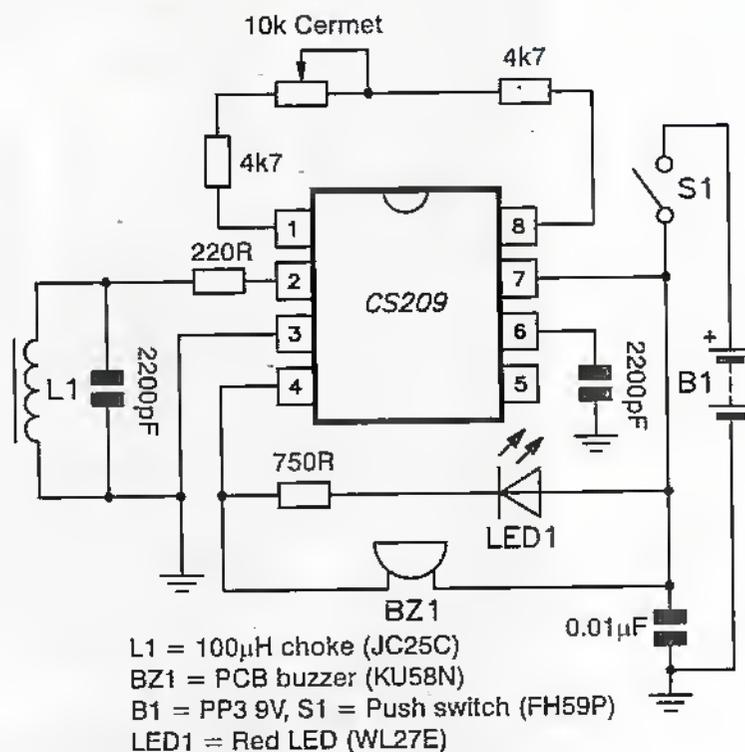
Figure 5. Example of a simple IC based metal detector circuit.
