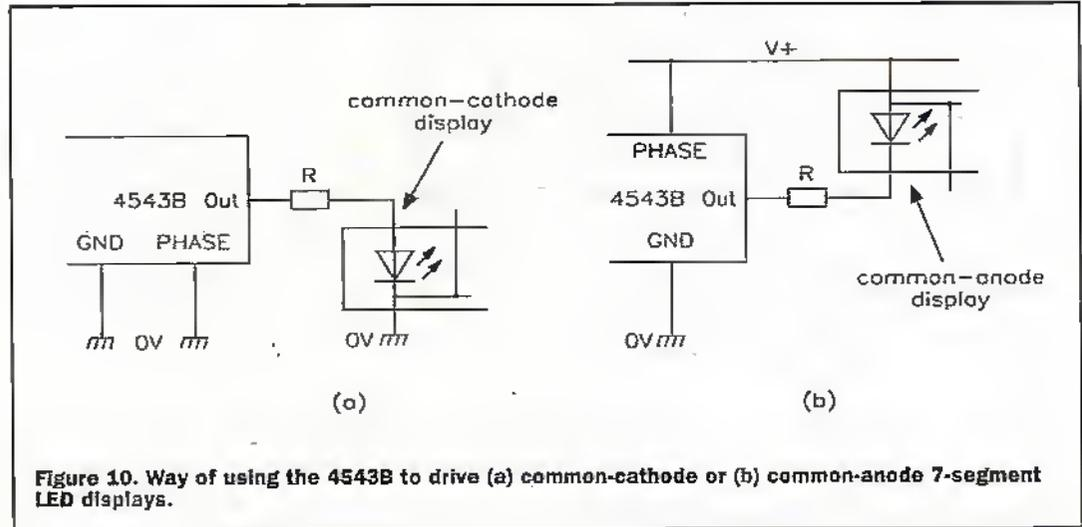
Figure 10. Way of using the 4543B to drive (a) common-cathode or (b) common-anode 7-segment LED displays.
