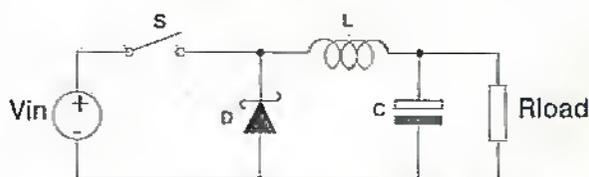
Figure 2. The four basic components of a buck converter.
