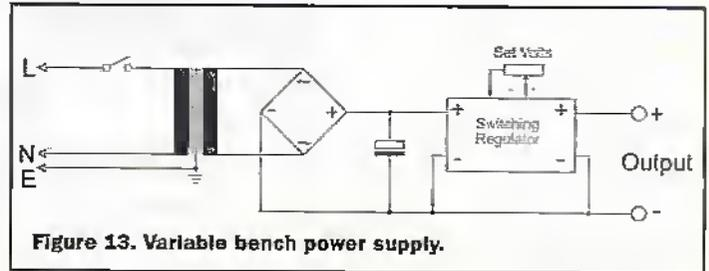
Figure 13. Variable bench power supply.
