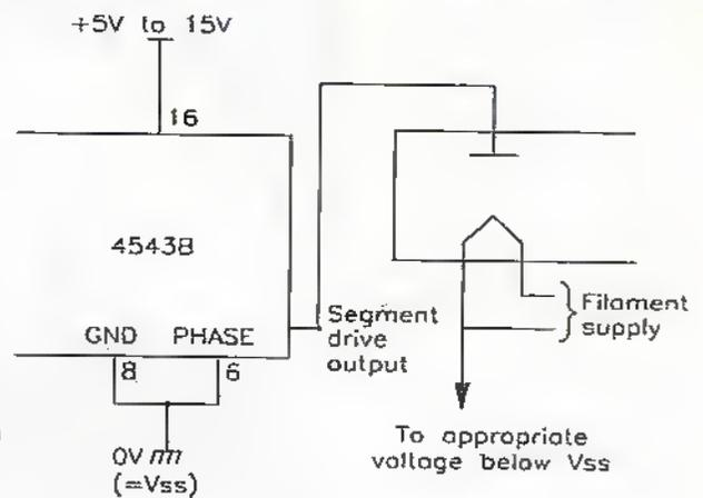
Figure 13. Driving a fluorescent readout with a 4543B.
