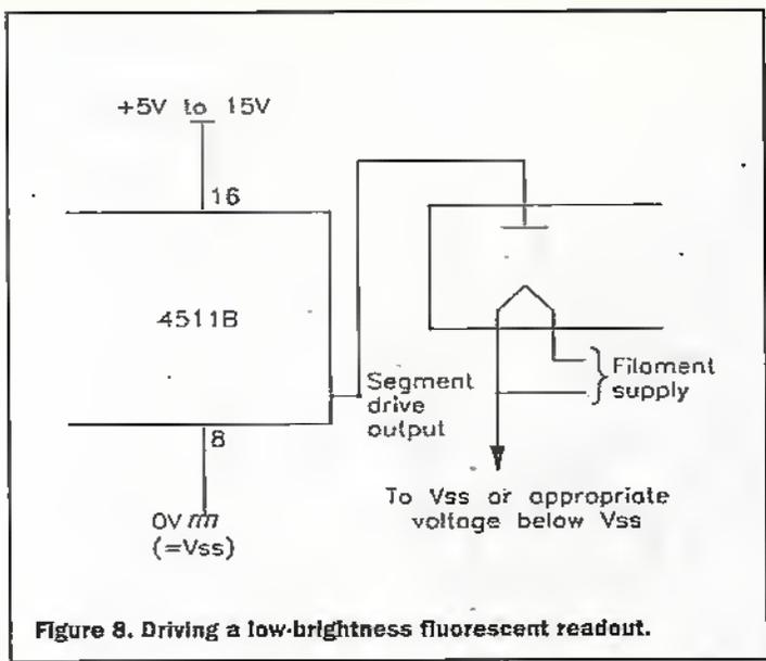
Figure 8. Driving a low-brightness fluorescent readout.
