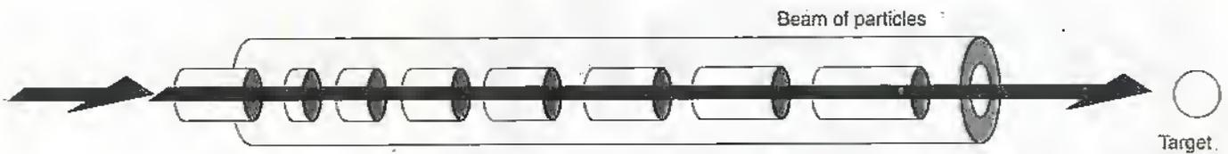
Figure 2. The Linear Accelerator, or Linac, of 1939.
