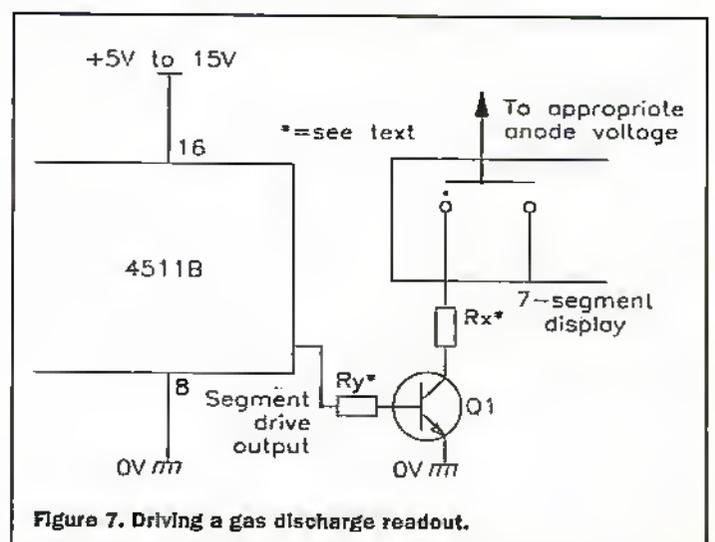
Figure 7. Driving a gas discharge readout.
