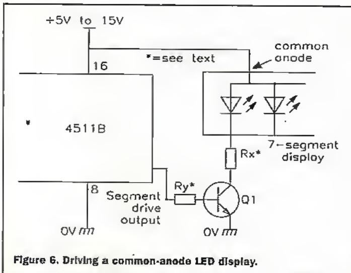
Figure 6. Driving a common-anode LED display.
