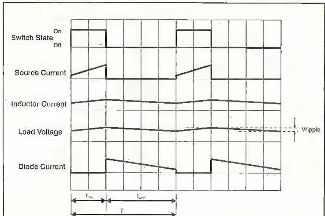
Figure 3. The Buck converter switching cycle. Ripple is due to non-ideal components.
