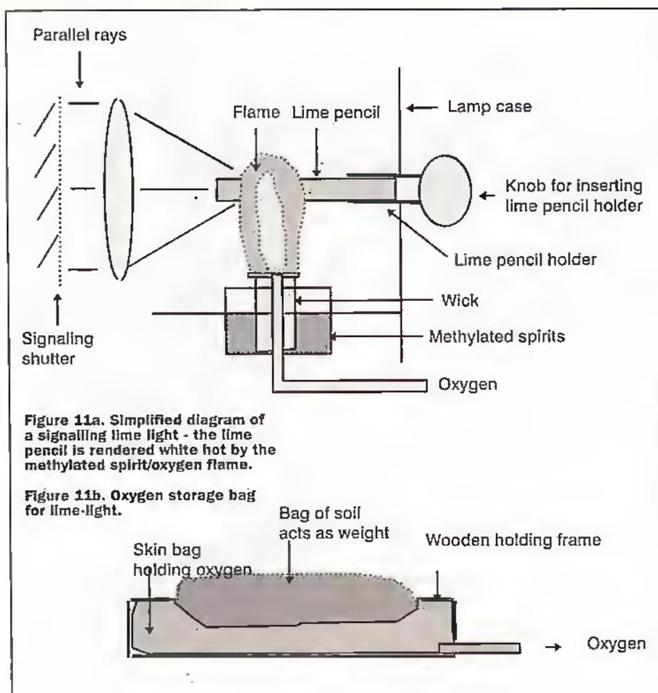
Figure 11a. Simplified diagram of a signalling lime light - the lime pencil is rendered white hot by the methylated spirit/oxygen flame.
