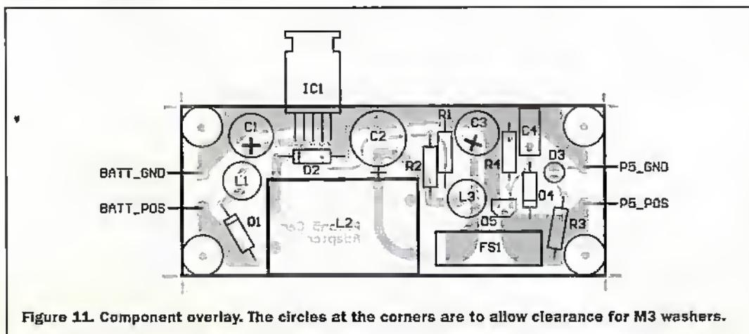
Figure 11. Component overlay. The circles at the corners are to allow clearance for M3 washers.
