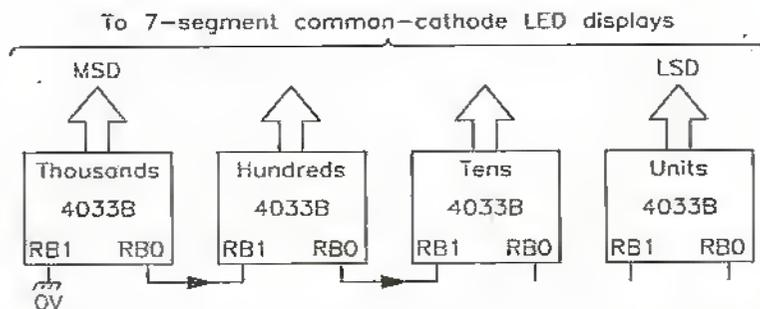
Figure 18. Method of modifying the Figure 17 circuit to give automatic leading-zero suppression.
