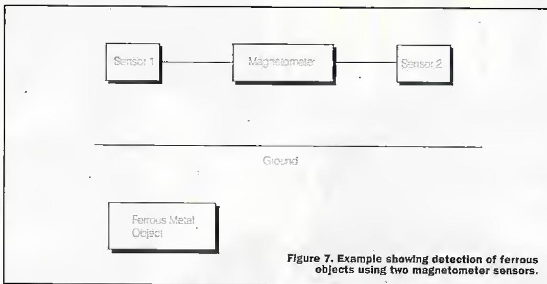
Figure 7. Example showing detection of ferrous objects using two magnetometer sensors.
