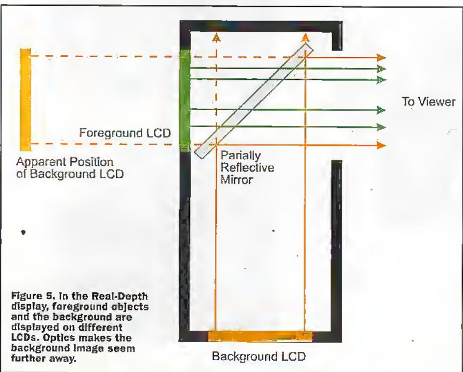
**Figure 5.** In the Real-Depth display, foreground objects and the background are displayed on different LCDs. Optics makes the background image seem further away.
