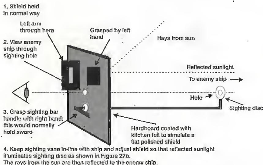
Figure 27a. The Author's simulation of a shield that could have been used by the ancient Greeks to concentrate sunlight on the Persian Ships.
