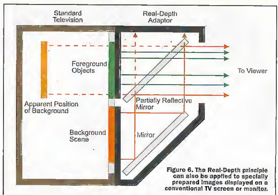
Figure 6. The Real-Depth principle can also be applied to specially prepared images displayed on a conventional TV screen or monitor.
