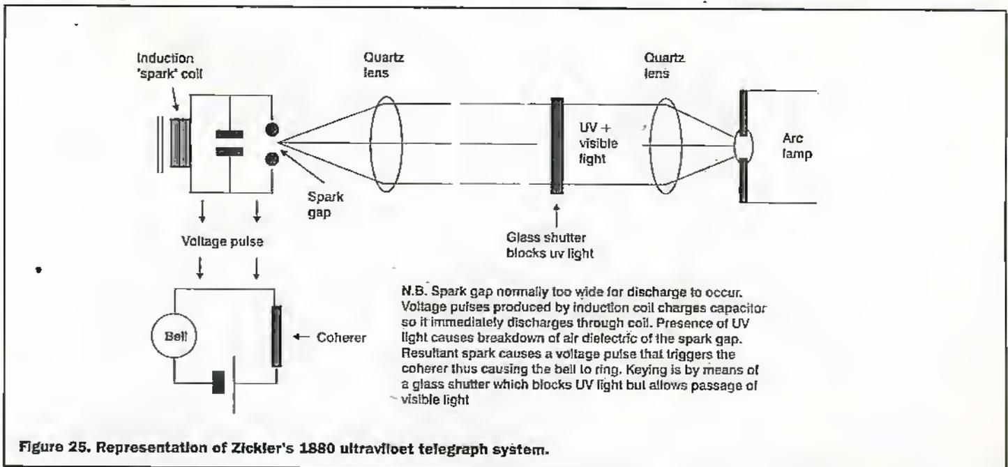
Figure 25. Representation of Zickler's 1880 ultraviolet telegraph system.
