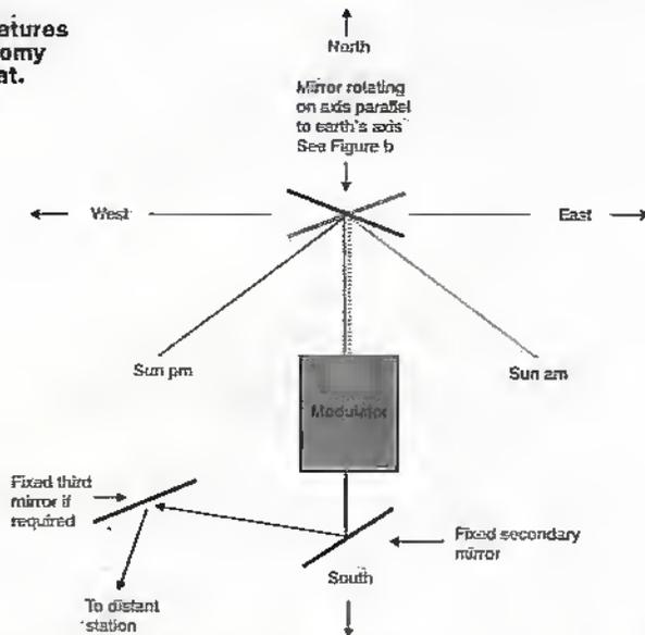
Diagram shows sunlight directed on to modulator, and set up for northern hemisphere. Modulated light can be reflected in any direction by fixed secondary mirrors.
