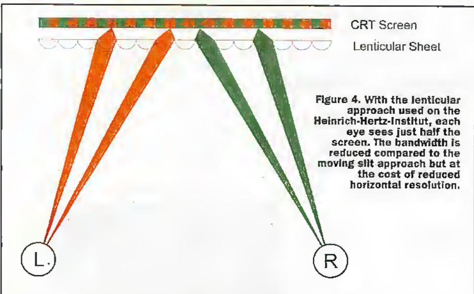
**Figure 4.** With the lenticular approach used on the Heinrich-Hertz-Institut, each eye sees just half the screen. The bandwidth is reduced compared to the moving slit approach but at the cost of reduced horizontal resolution.
