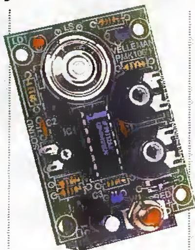
The circuit can be literally constructed in under 10 minutes. But before starting construction it is worth deciding whether you wish the sensor probes to be remote from the board and sounder. This can be up to two metres and so does provide some flexibility in any application, and Velleman thoughtfully provided a convenient 'break' point on the board so that the sensor
