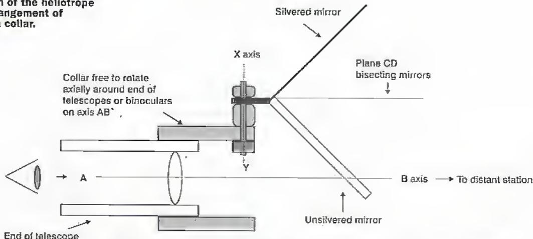
Although offset, the view through the telescope is taken to run longitudinally through plane CD, the offset is too small to have any significant effect on alignment with the distant station
