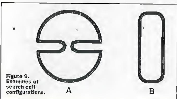
Figure 9. Examples of search coil configurations.
