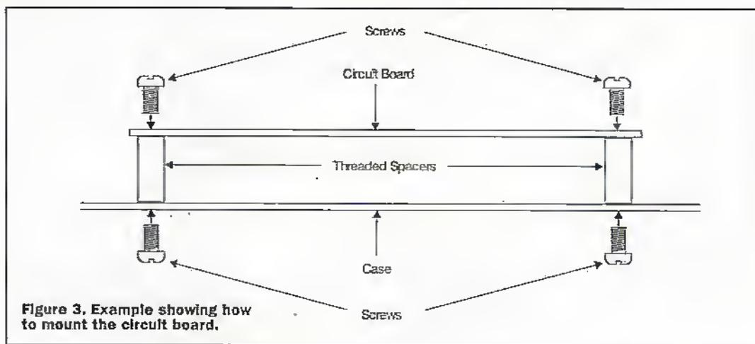
Figure 3. Example showing how to mount the circuit board.
