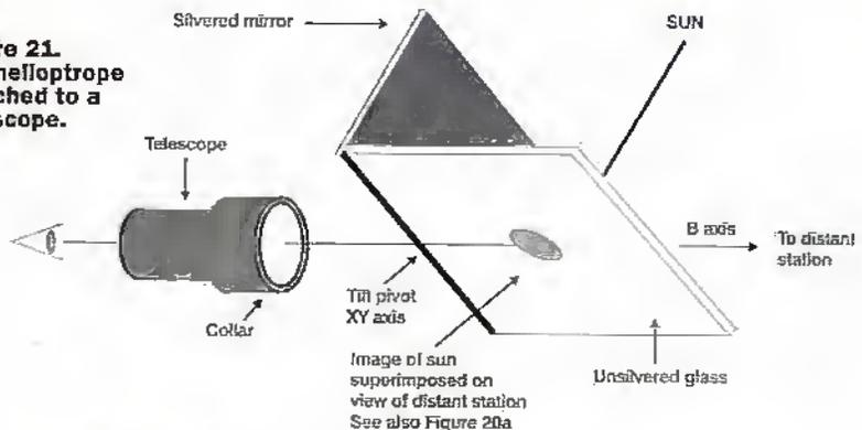
When faint image of the sun is superimposed on the view of distant station, the reflected beam is aligned with the distant station.
