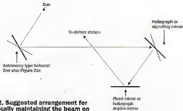
**Figure 22. Suggested arrangement for automatically maintaining the beam on the distant station.**
