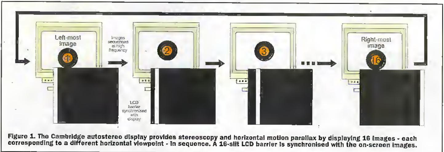
Figure 1. The Cambridge autostereo display provides stereoscopy and horizontal motion parallax by displaying 16 images - each corresponding to a different horizontal viewpoint - in sequence. A 16-slit LCD barrier is synchronised with the on-screen images.
