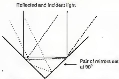
When light falls equally on the two mirrors at an angle within the 'V' it is reflected at 180° within the same plane as the incident light.
