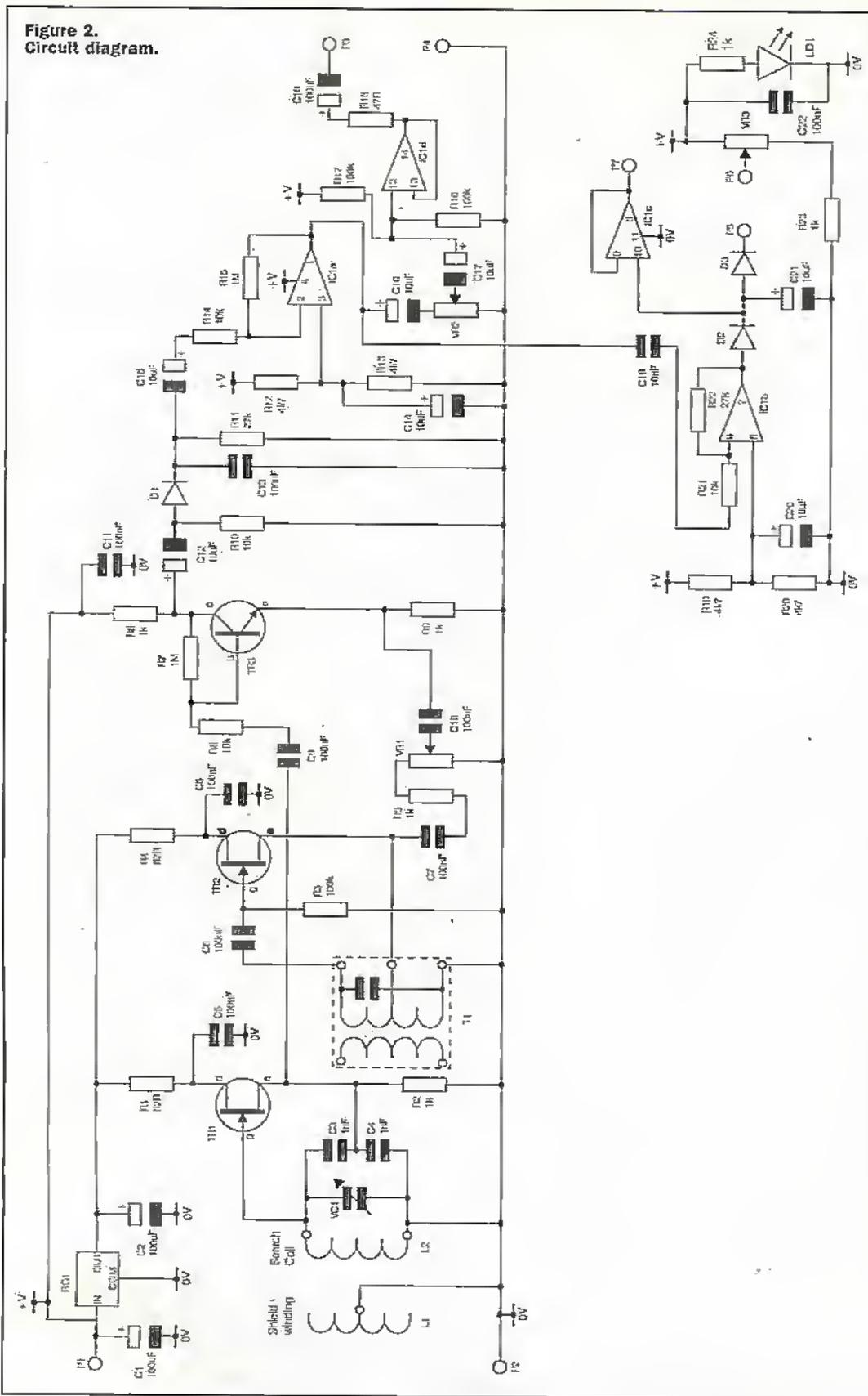
provide a reference level for the device whereas R14 and R15 set the amplifier gain. The output is fed to volume control VR2 via coupling capacitor C16 and then on to a buffer stage formed by IC1d and associated components. C18 acts as a DC blocking capacitor at the output.
