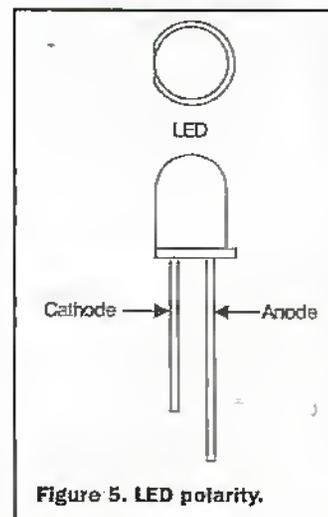
Figure 5. LED polarity.
