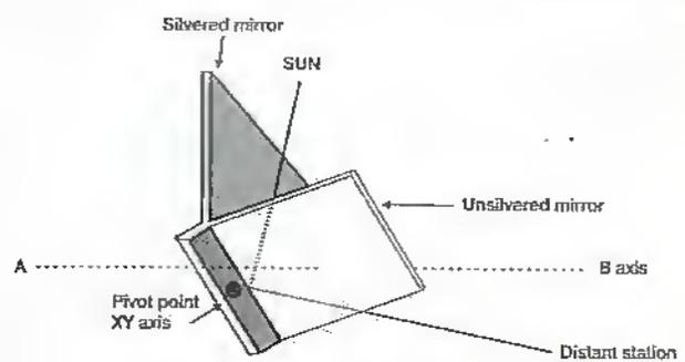
Rotating mirror on axis AB also rotates plane CD. Mirrors are rotated on axis AB until CD corresponds to plane of the sun and distant station. Mirrors are then tilted on axis XY until light from the sun is reflected to distant station.
