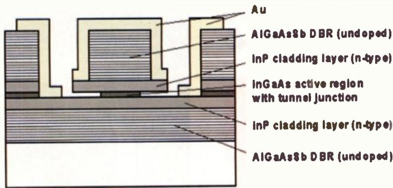
**Figure 3.** Schematic of intracavity contacted design.
