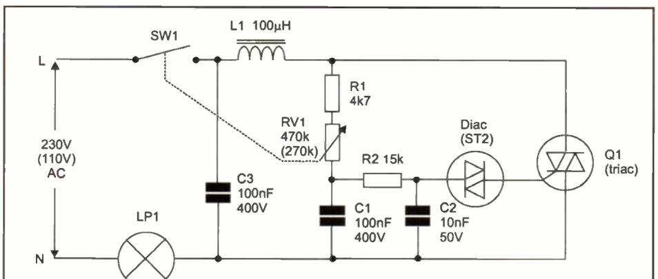
**Figure 12.** Improved diac-type lamp dimmer with gate slaving.
