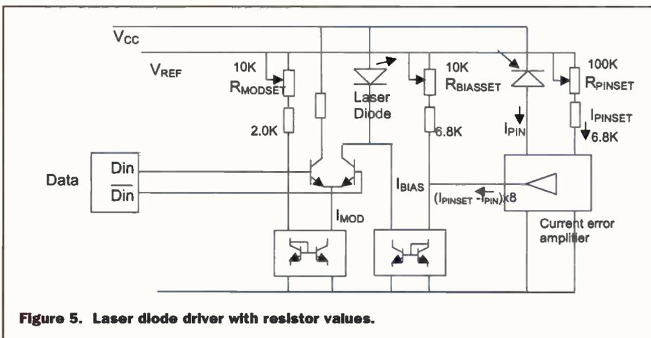
**Figure 5. Laser diode driver with resistor values.**
