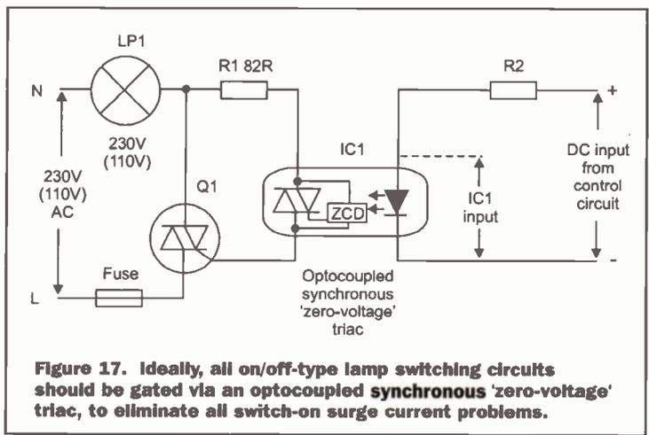
**Figure 17. Ideally, all on/off-type lamp switching circuits should be gated via an optocoupled synchronous 'zero-voltage' triac, to eliminate all switch-on surge current problems.**
