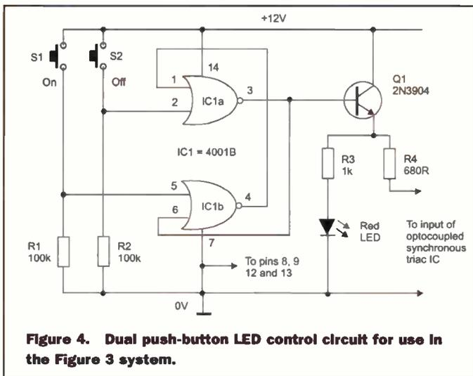
**Figure 4. Dual push-button LED control circuit for use in the Figure 3 system.**
