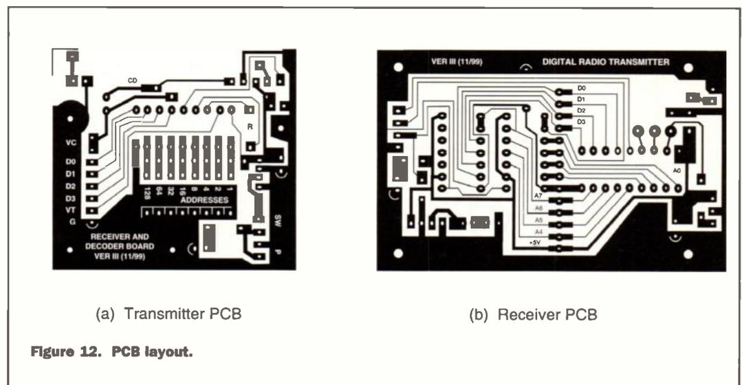
Figure 12. PCB layout.
