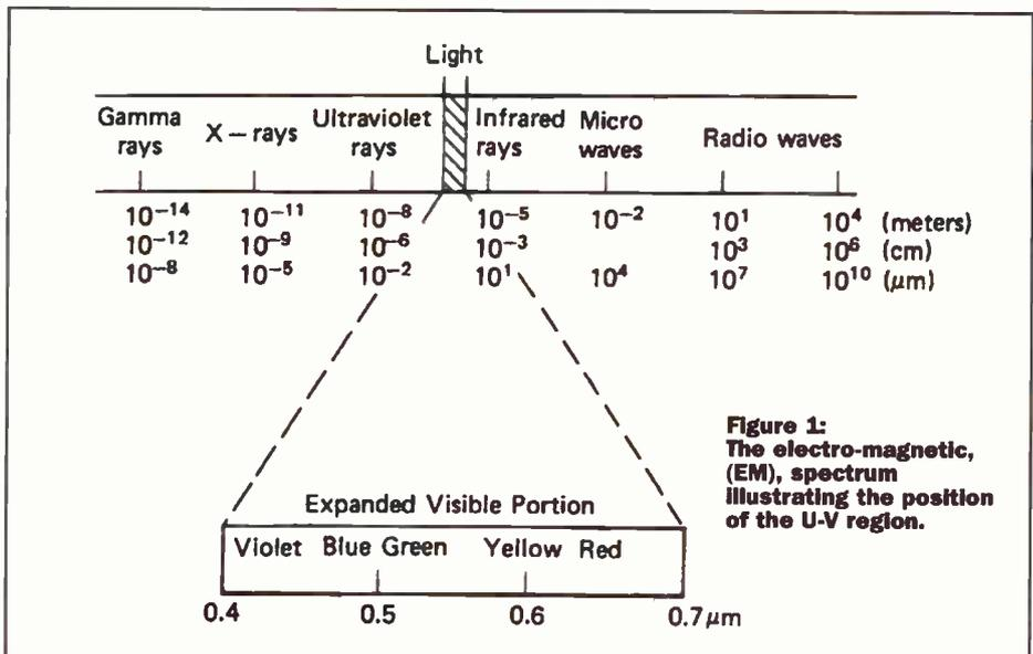
**Figure 1:** The electro-magnetic, (EM), spectrum illustrating the position of the U-V region.
