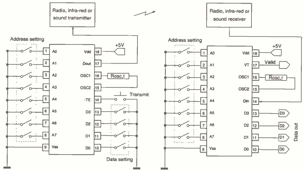
Figure 7. Typical application of the data encoder and decoder pairs.
