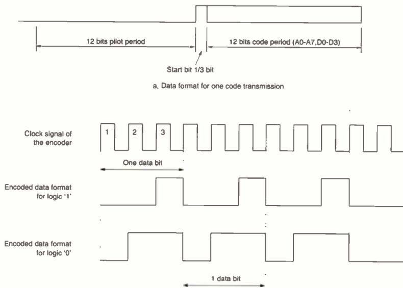
Figure 9. Encoded serial data format.
