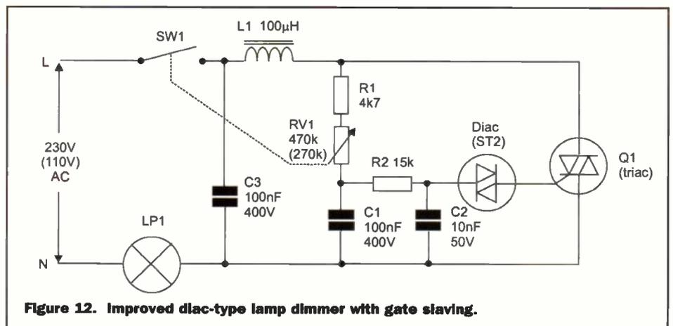
**Figure 12.** Improved diac-type lamp dimmer with gate slaving.
