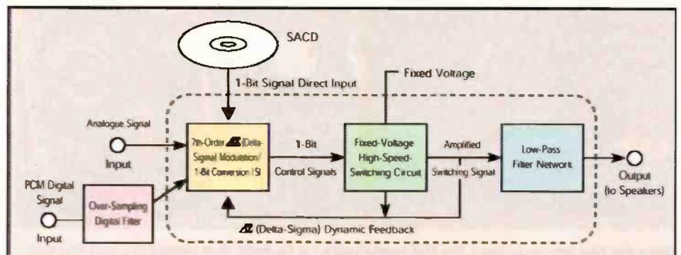
**Block diagram, showing one channel of the Sharp SM-SX1 digital amplifier.**
