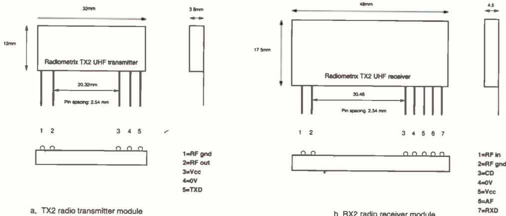
Figure 3. Pin-out of Radiometrix TX2 and RX2 modules.
