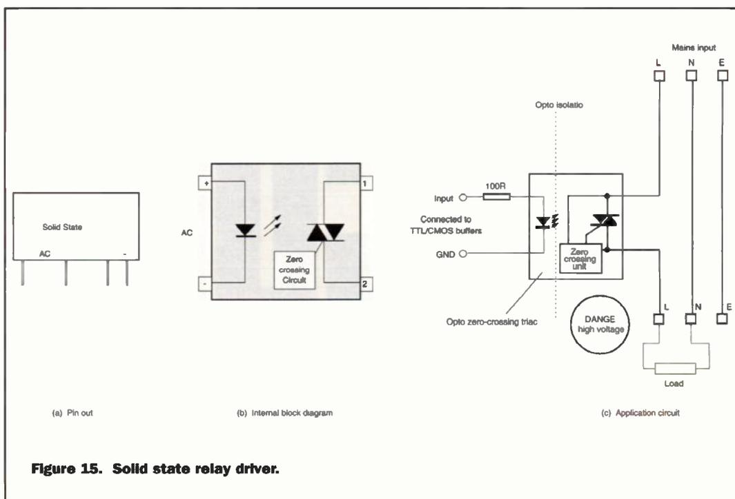
Figure 15. Solid state relay driver.
