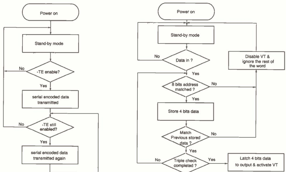
Figure 8. Flow chart of the operation of the encoder and decoder.
