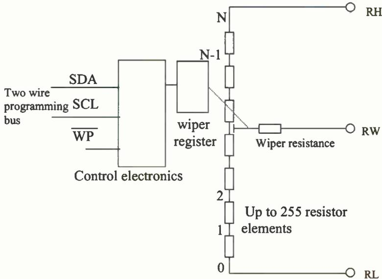
**Figure 7. Block Diagram of Xicor Digitally Controlled Potentiometer**
