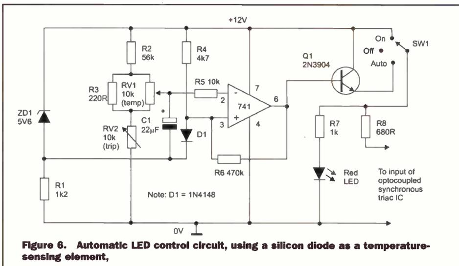
**Figure 6. Automatic LED control circuit, using a silicon diode as a temperature-sensing element,**
