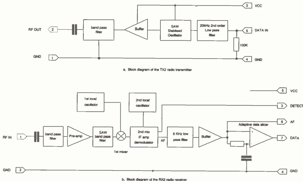
Figure 4. Internal block diagrams of TX2 and RX2.
