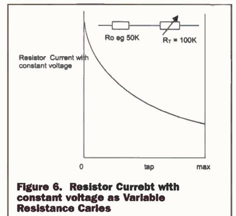
**Figure 6. Resistor Current with constant voltage as Variable Resistance Carries**
