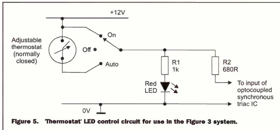
**Figure 5. Thermostat LED control circuit for use in the Figure 3 system.**
