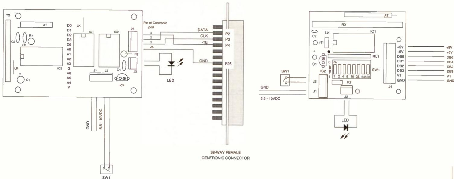
Figure 13. PCB artwork of the radio transmitter and the receiver.
