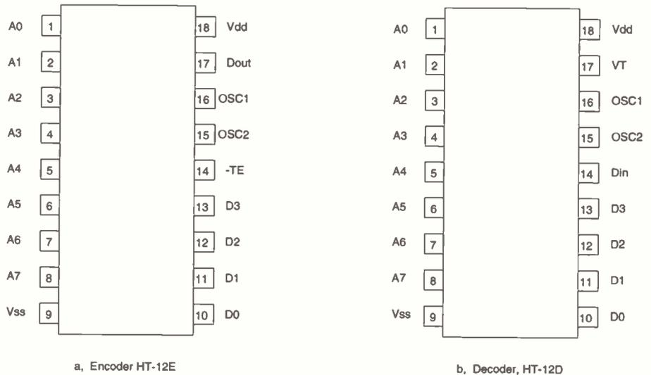
Figure 6. Data encoder (HT-12E) and decoder pairs (HT-12D).
