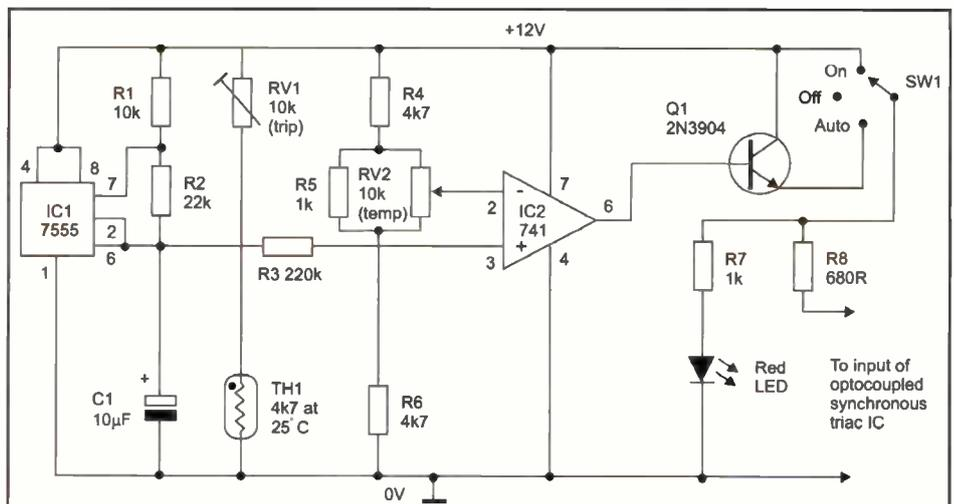
**Figure 10.** Fully automatic 'burst-fire' LED control circuit for use in the Figure 3 heater control system.
