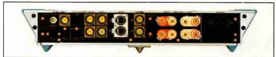
**Round the back of the Sharp SM-SX1 digital amplifier, showing all the various analogue and digital connections.**
