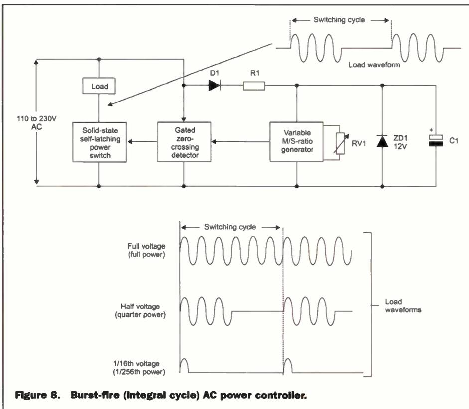
**Figure 8. Burst-fire (Integral cycle) AC power controller.**
