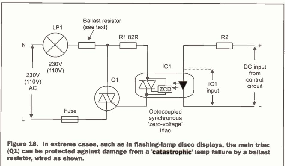
**Figure 18. In extreme cases, such as in flashing-lamp disco displays, the main triac (Q1) can be protected against damage from a 'catastrophic' lamp failure by a ballast resistor, wired as shown.**
