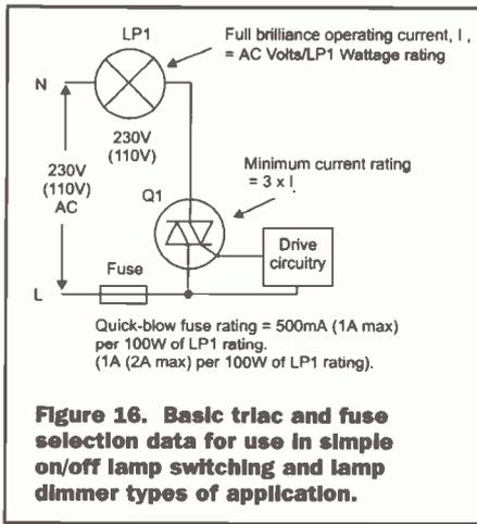
**Figure 16. Basic triac and fuse selection data for use in simple on/off lamp switching and lamp dimmer types of application.**
