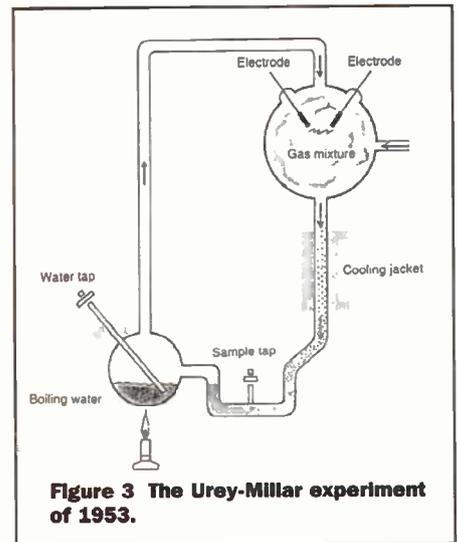
Figure 3 The Urey-Millar experiment of 1953.
