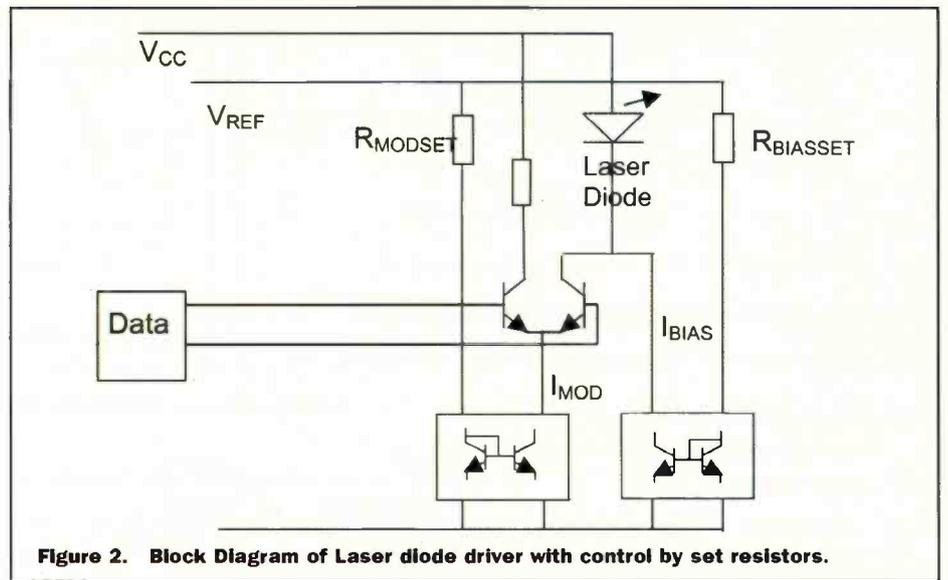
Figure 2. Block Diagram of Laser diode driver with control by set resistors.
