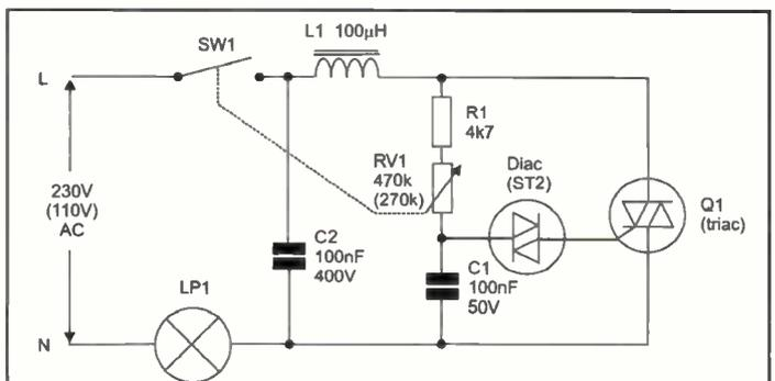
**Figure 11.** Practical circuit of a simple diac-type lamp dimmer with RFI suppression.
