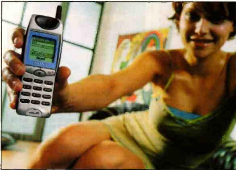
**Cellphones equipped with WAP microbrowsers are proving popular, despite the inconsistency of the services that can be accessed. Here's the latest CMD-J5 model from Sony. This WAP-compatible handset features a voice recorder (as its LCD screen demonstrates), compatibility with HTML (yes, really!) and a thumbwheel for site navigation.**
