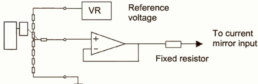
**Figure 8. Block Diagram of Digital Controlled Potentiometer with Buffer to Give Wider Range or More Resolution of Control Current.**
