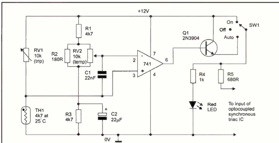
**Figure 7. Automatic LED control circuit, using a NTC thermistor as a temperature-sensing element, for use in the Figure 3 system.**
