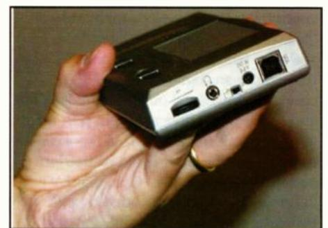
A side view of the Hango Personal Jukebox, showing the USB interface - across which MP3 tracks are transferred from a PC - and power/headphone sockets. No S/PDIF output for your hi-fi, though... Photo courtesy of Adrian Caspersz.
