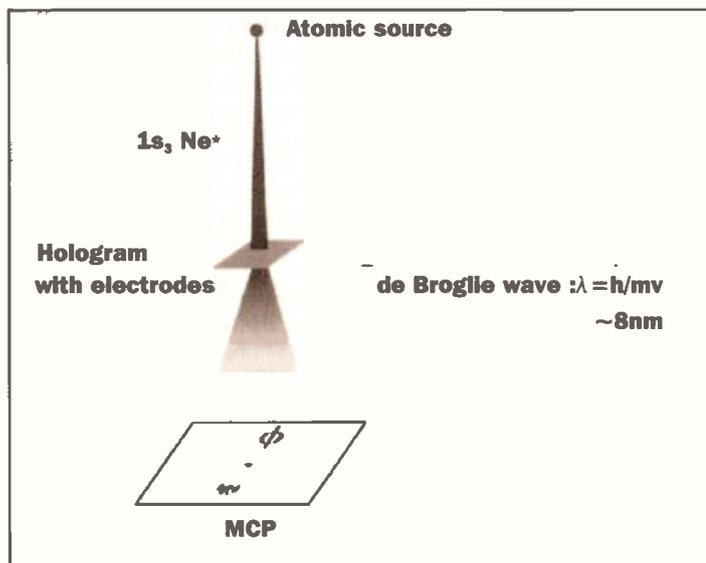
**Figure 1. Schematic diagram of experimental setup. The atomic source, the hologram, and the screen of microchannel plate (MCP) were placed vertically.**
