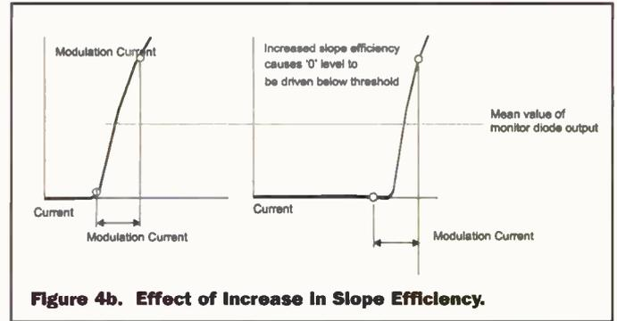
**Figure 4b. Effect of Increase in Slope Efficiency.**
