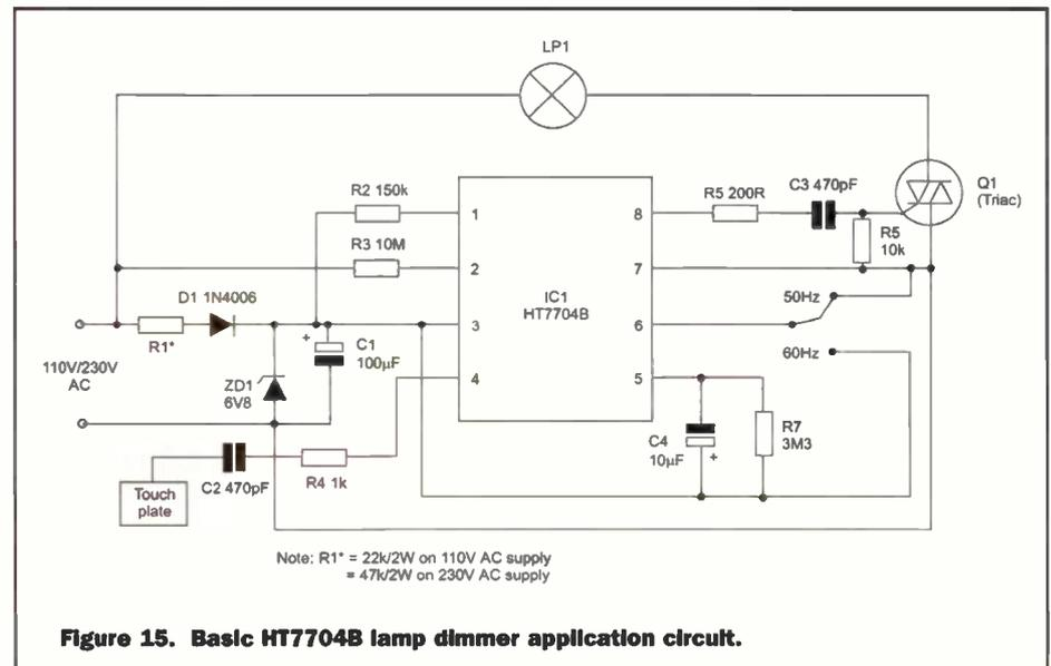
**Figure 15. Basic HT7704B lamp dimmer application circuit.**
