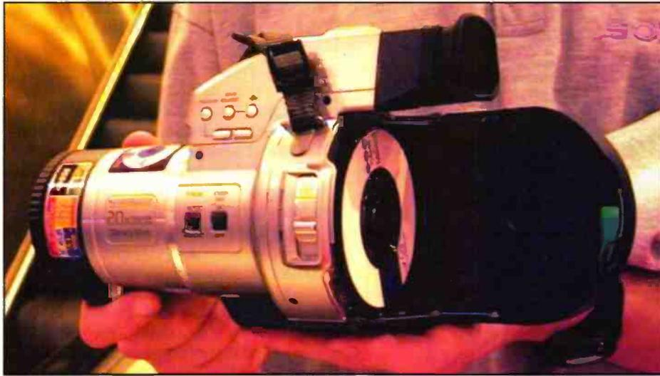
One of the most interesting digital stills cameras on view was the Sony MVC-CD1000., which dispenses with traditional flash memory or floppy discs. Instead, images are stored on a special 8cm CD-R that has a capacity of 156MB capacity. Once the disc has been burnt, it can be read by a PC. We applaud Sony's efforts, but surely CD-RW would have been a more logical storage medium? Other features include a 10x optical zoom and a 2.1 megapixel resolution.
