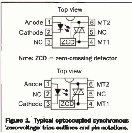
Figure 1. Typical optocoupled synchronous 'zero-voltage' triac outlines and pin notations.
