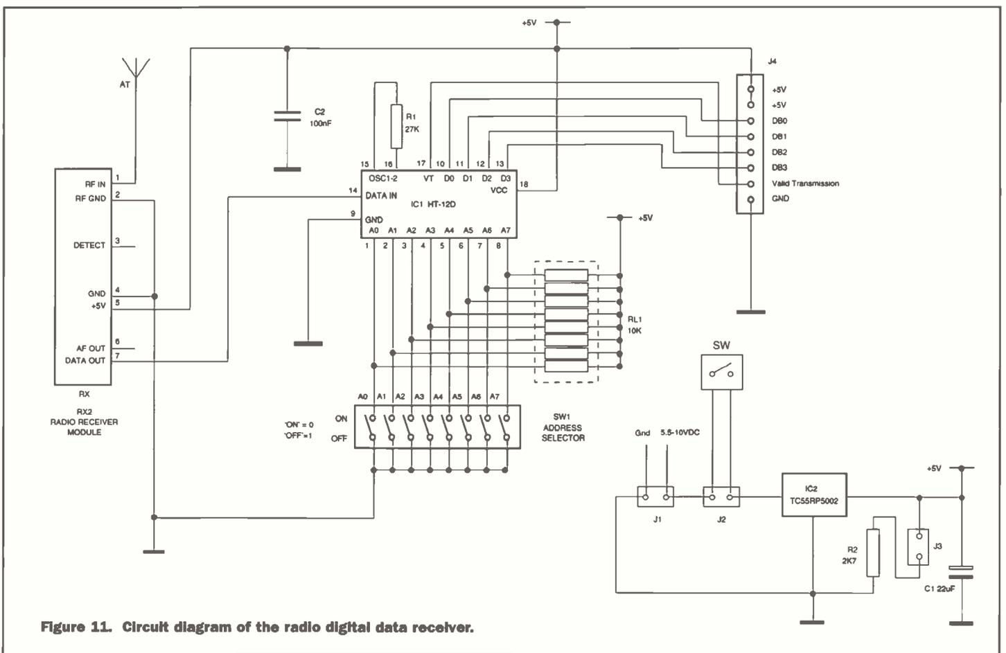
Figure 11. Circuit diagram of the radio digital data receiver.
