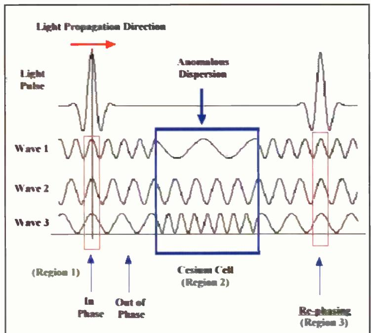
**Figure 1.** A "snapshot" of a propagating light pulse. A light pulse is made of many component waves (waves 1 through 3). Inside an anomalous dispersion region (region-2), the waves propagate in an unusual way. The result is that the waves are "rephased" again at a distant place along its propagation direction to produce the incoming pulse. The effect is greatly exaggerated here for the purpose of illustration.
