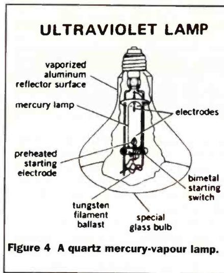
Figure 4 A quartz mercury-vapour lamp.
