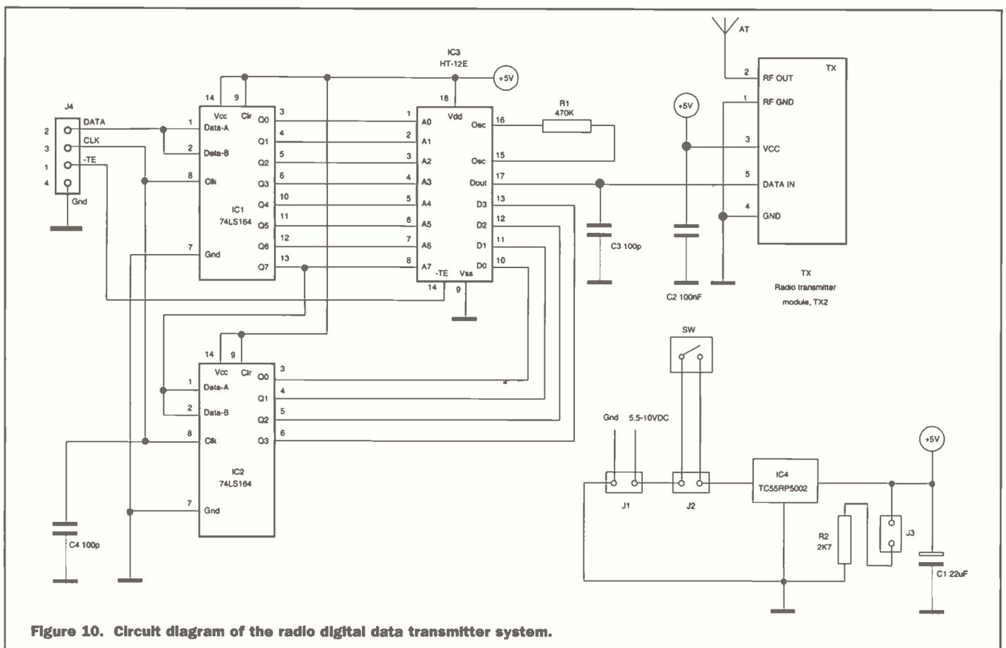
Figure 10. Circuit diagram of the radio digital data transmitter system.
