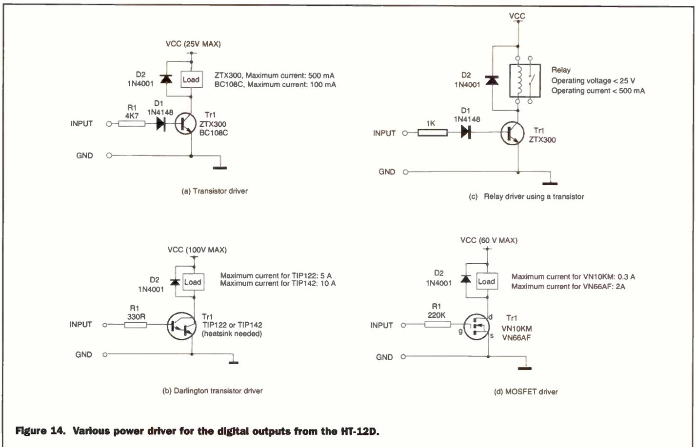
Figure 14. Various power driver for the digital outputs from the HT-12D.
