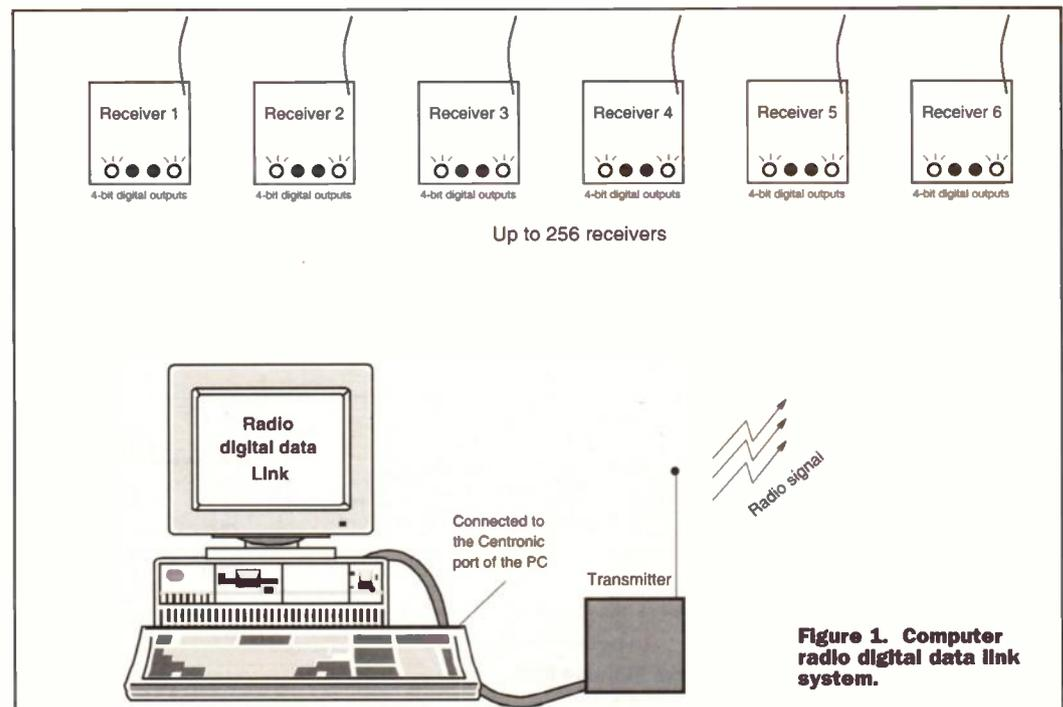
Figure 1. Computer radio digital data link system.
