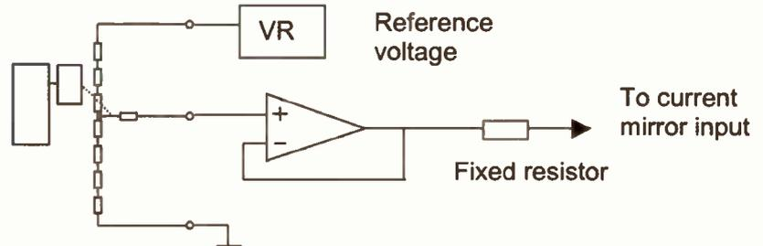
**Figure 8. Block Diagram of Digital Controlled Potentiometer with Buffer to Give Wider Range or More Resolution of Control Current.**
