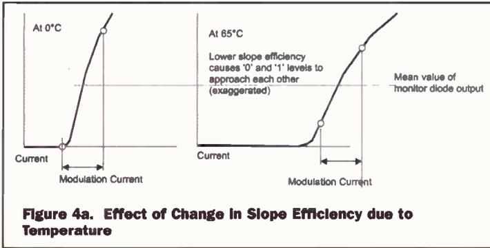
**Figure 4a. Effect of Change in Slope Efficiency due to Temperature**
