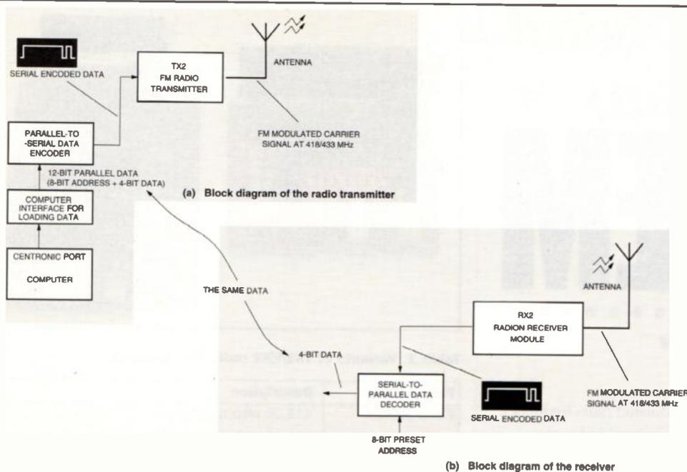
Figure 2. Block Diagram of the transmitter and receiver.
