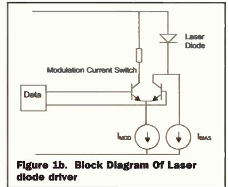
Figure 1b. Block Diagram Of Laser diode driver
