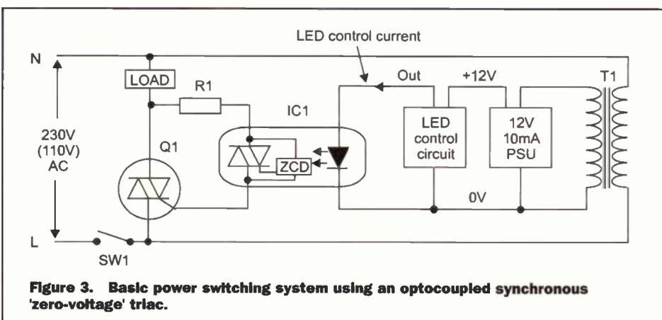
Figure 3. Basic power switching system using an optocoupled synchronous 'zero-voltage' triac.
