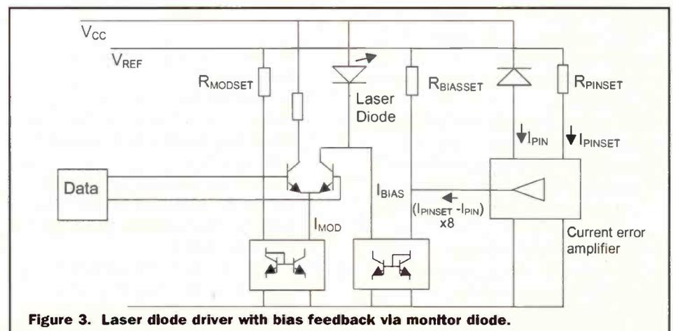
Figure 3. Laser diode driver with bias feedback via monitor diode.
