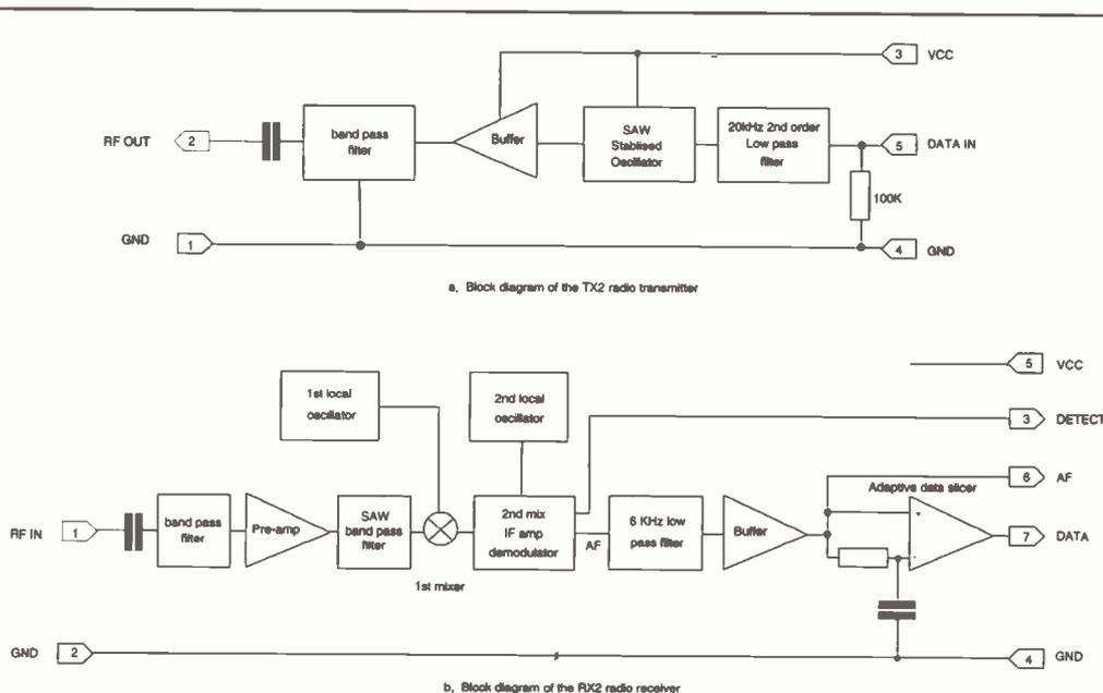
Figure 4. Internal block diagrams of TX2 and RX2.
