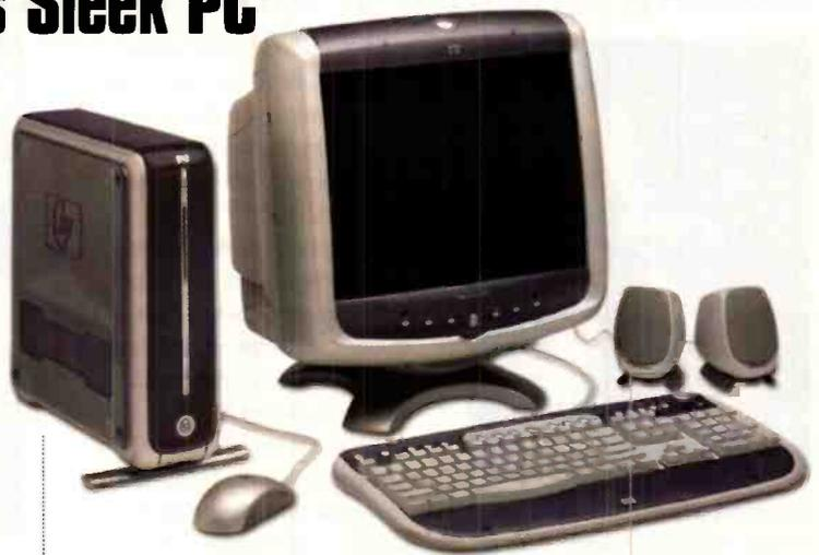
up to 11 MB for video memory, a 20 GB hard drive, CD-RW, 10/100 BT Ethernet card, v.90 56K modem, Polk Audio stereo
