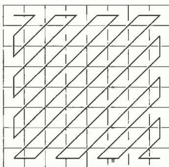
Data stream to VCL and run-length encoding:
