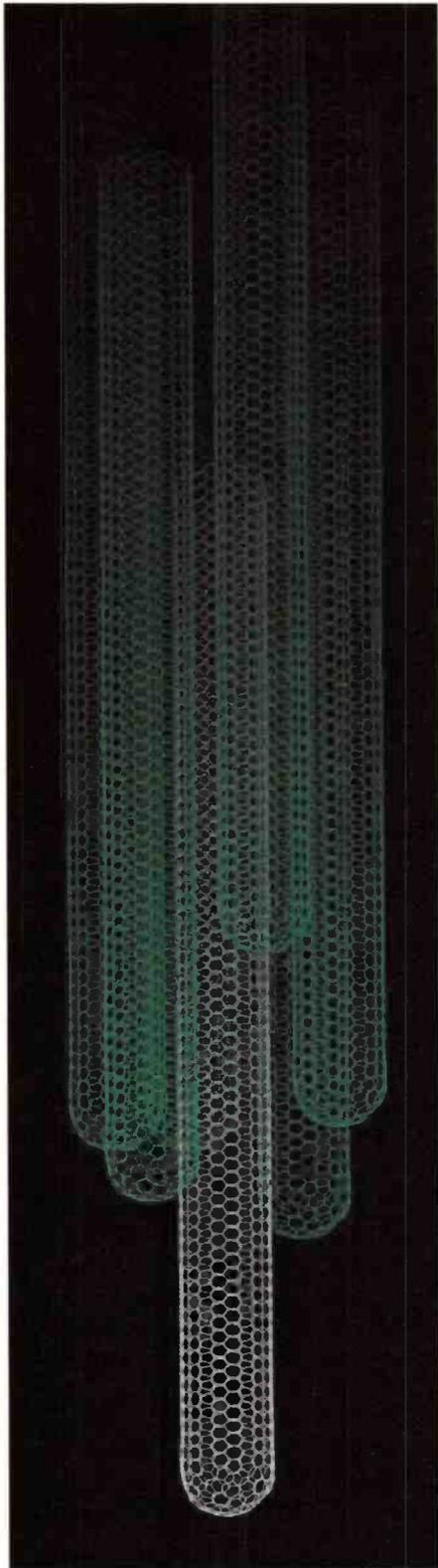
**Simulated image of collection of single-wall carbon nanotubes.**
