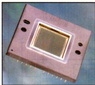
**Figure 9. The Kodak KAI-4000M 4 Million Pixel Image Sensor.** Courtesy Kodak.
