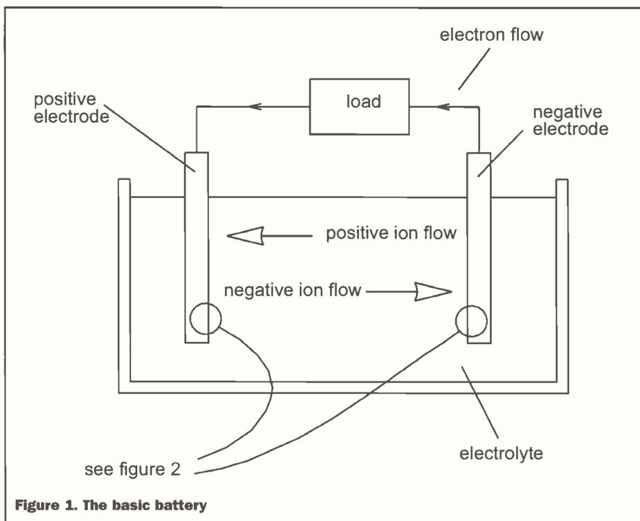
**Figure 1. The basic battery**
