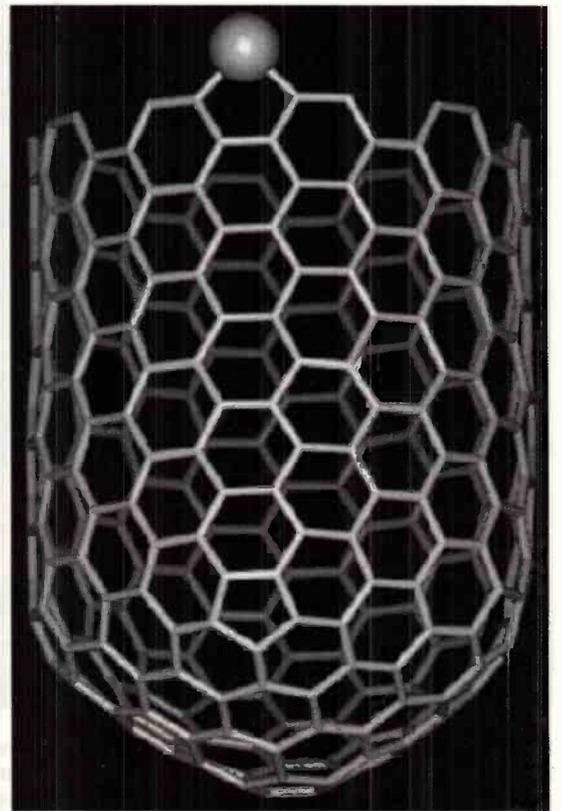
**Simulated image of collection of single-wall carbon nanotubes.** Courtesy Rice University
