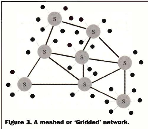
**Figure 3. A meshed or 'Gridded' network.**
