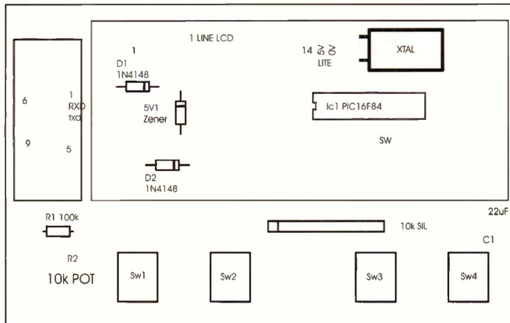
Figure 2. Component overlay
