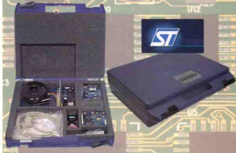
Complete development environment for ST72141 Motor Control Device
