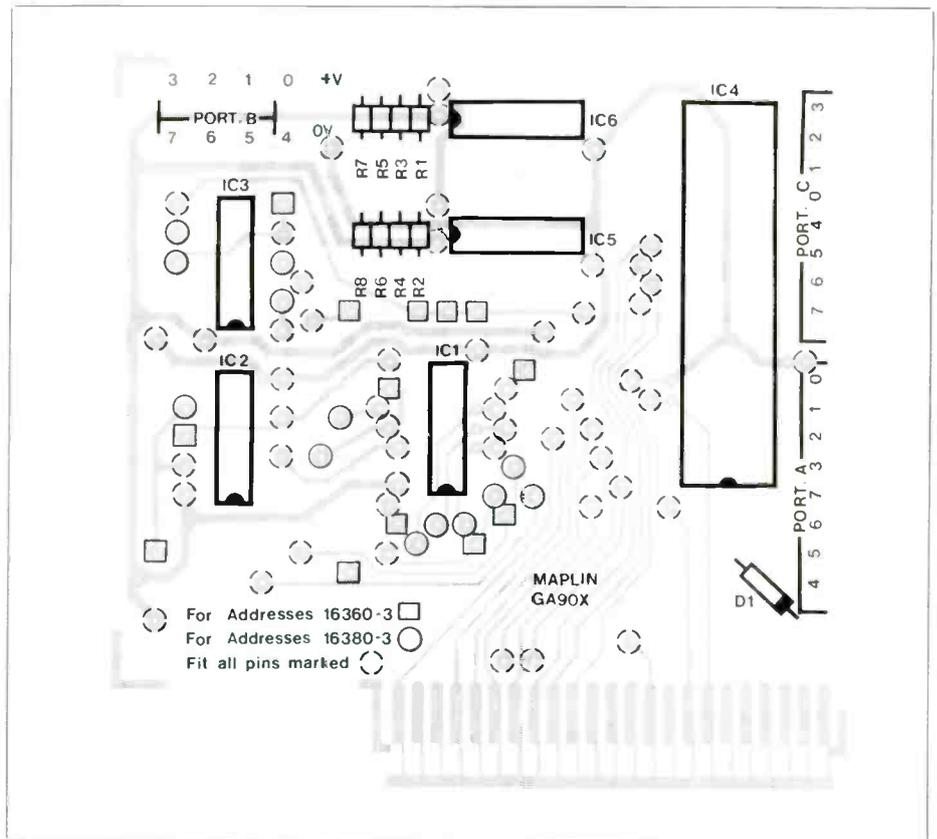
Figure 2. Component layout of I/O Port pcb.
