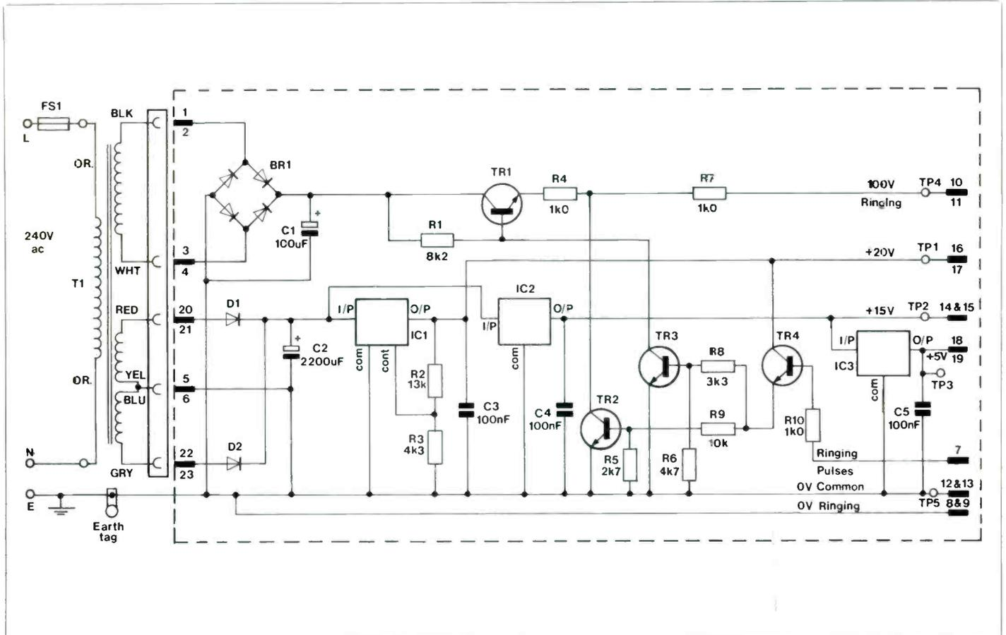
Figure 9. PSU circuit.
