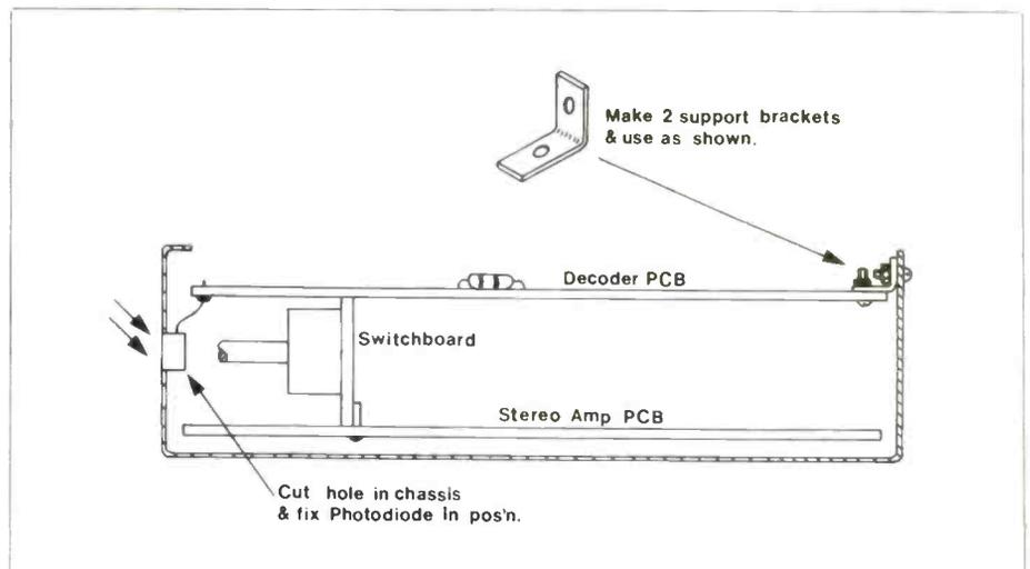
Figure 7. Mounting Decoder in 25W Mosfet Amplifier.
