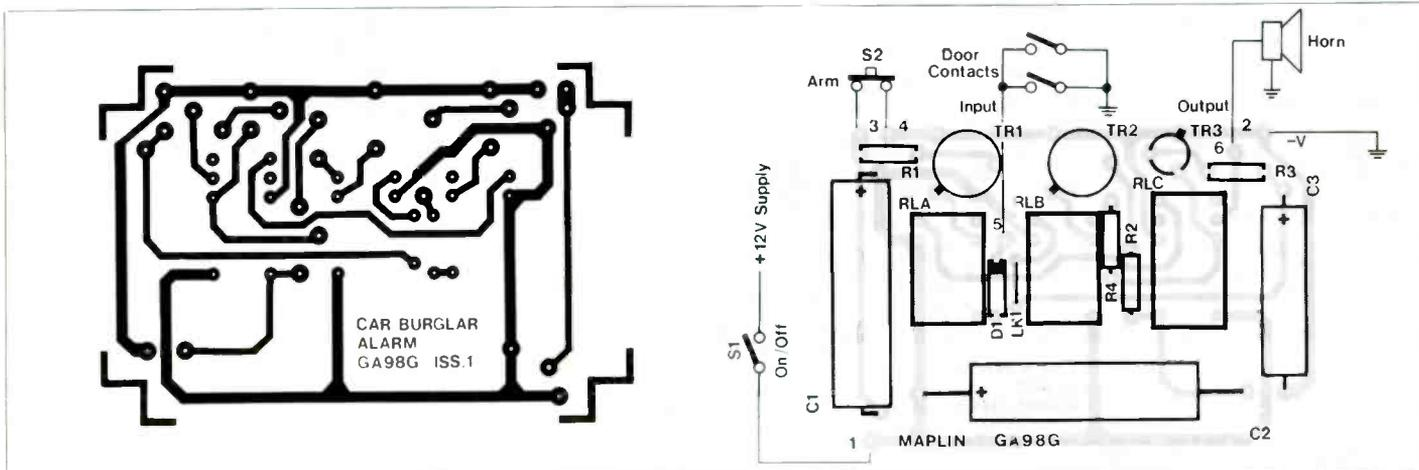
Figure 2. Track layout and component diagram.
