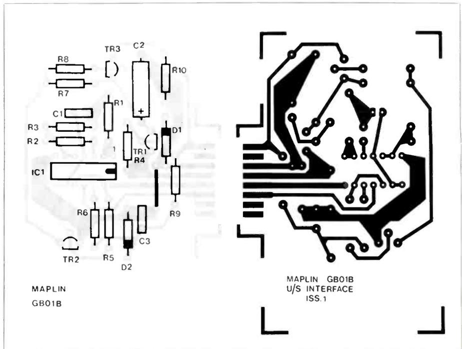
Figure 4. Component layout of the Ultrasonic Interface.
