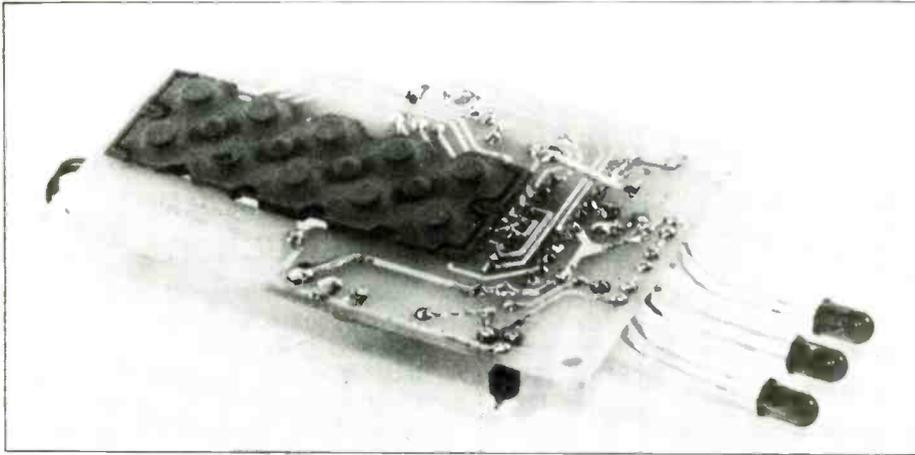
apparent. Press any one of S1 to S10 contacts, and the reading should drop 200mv to 6.7v. These readings can vary slightly, but serve to give an indication that all is well.
