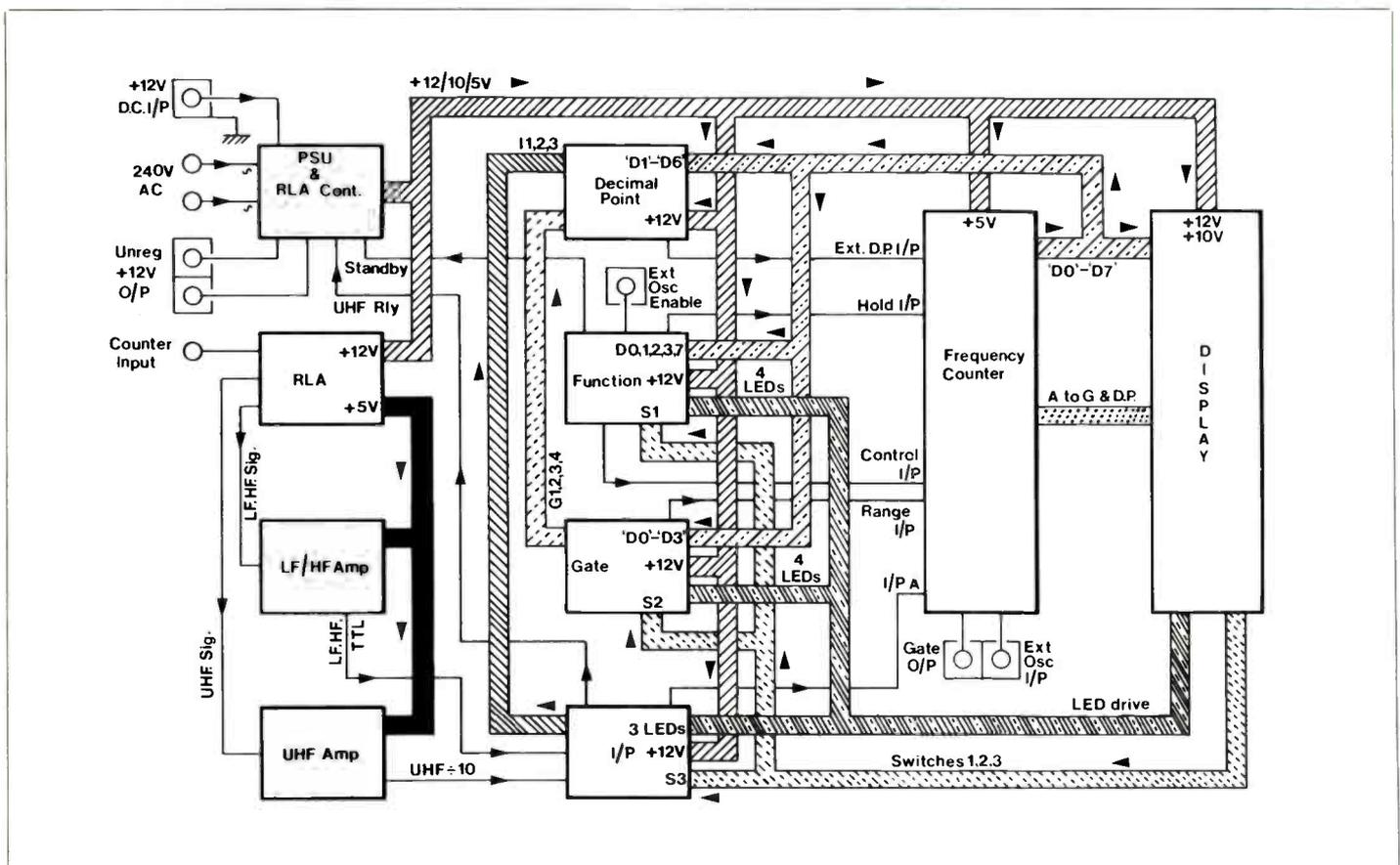
Figure 1. Block schematic of counter.
