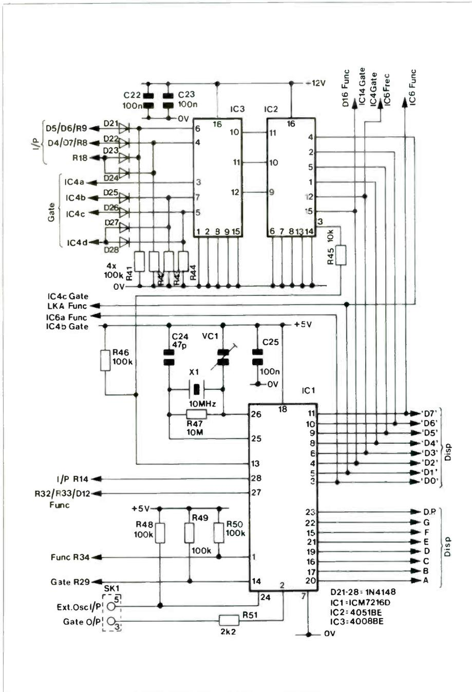
Figure 2. Frequency counter and decimal point logic counter.
