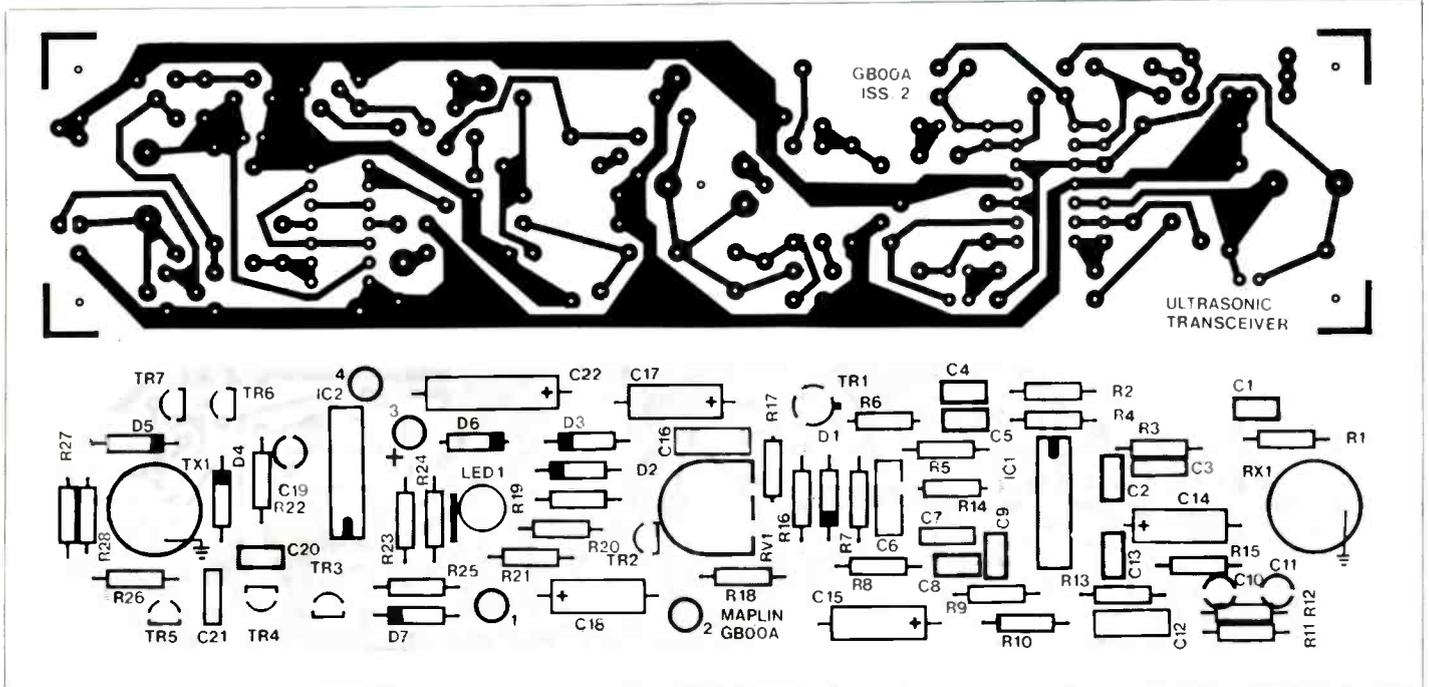
Figure 2. Component layout of the Ultrasonic Transceiver.
