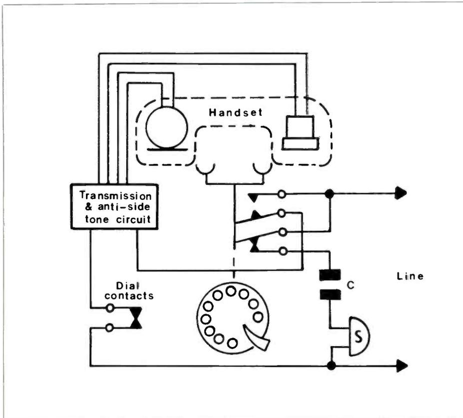
Figure 1. Block diagram of a typical telephone.
