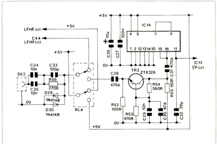
Figure 7. UHF input and relay circuit.
