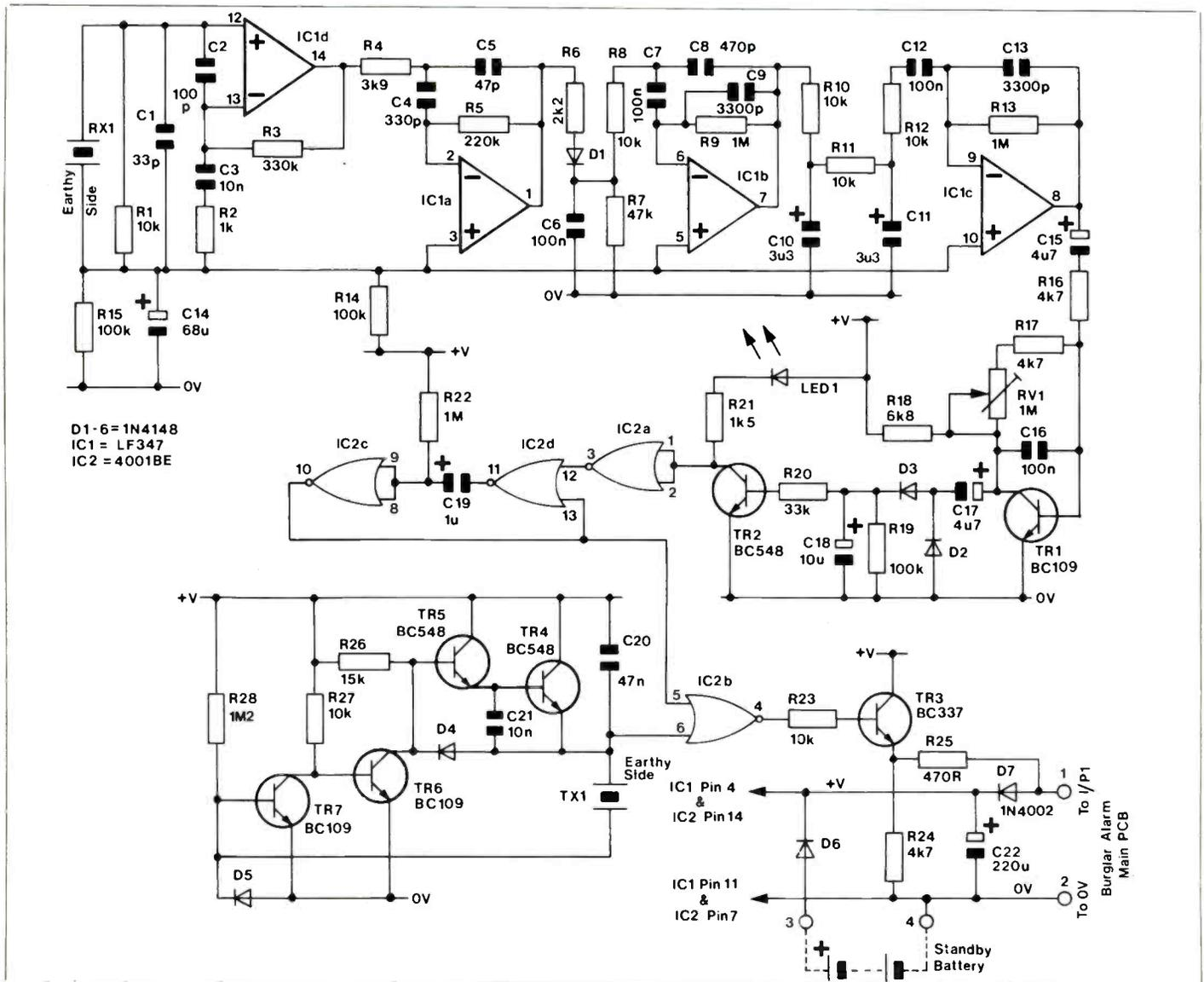
Figure 1. Circuit diagram of the Ultrasonic Transceiver.
