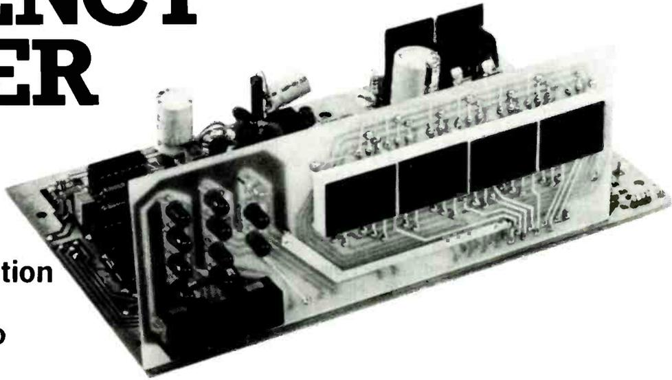
This frequency counter offers a superior specification for the first time in kit form. The design is based on the Intersil ICM7216D, and includes electronically switched ranges for greater reliability and ease of construction. Provision has been made for possible future extensions, so this kit can be considered truly flexible.
