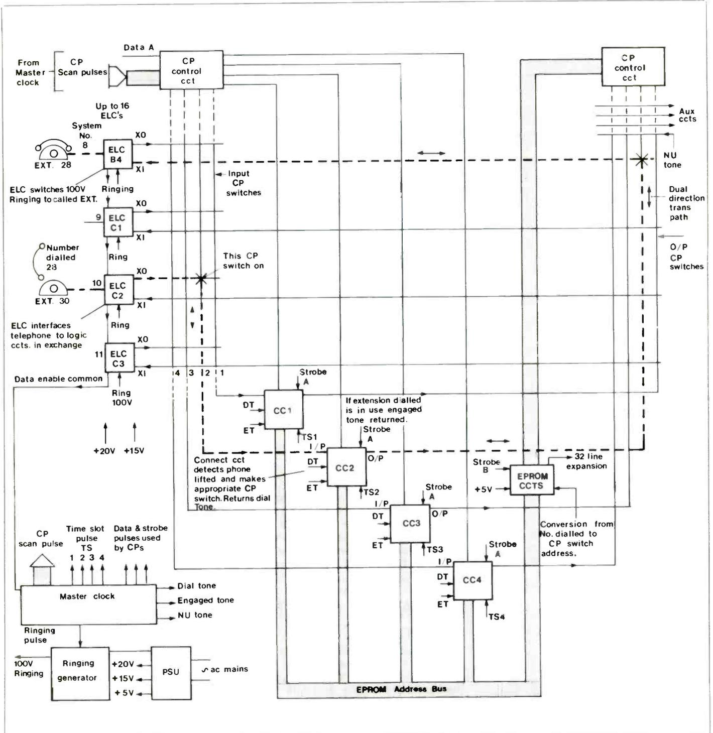
Figure 4a. Block diagram of the complete system.
