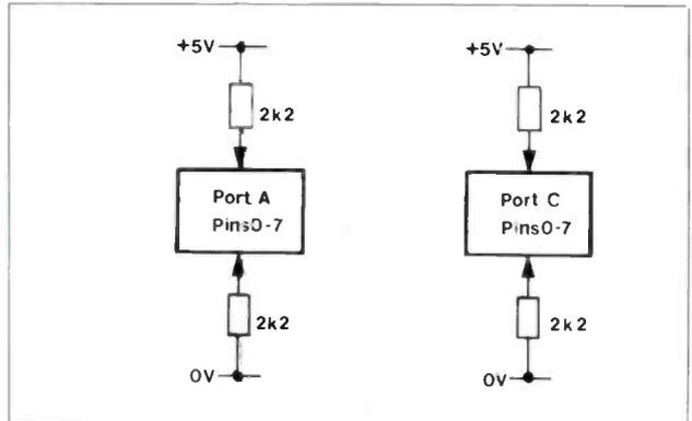
Figure 4. Test resistor connections.
