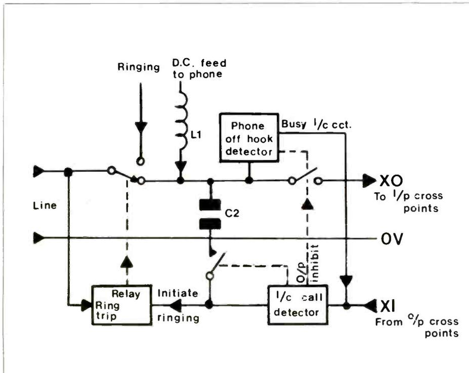
Figure 2. Block diagram of an Extension Line Circuit (ELC).
