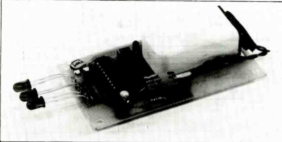
mately 150Hz. Scope measurements can be made on pin 2 of IC1 with the 'treble cut' key S7 operated.
