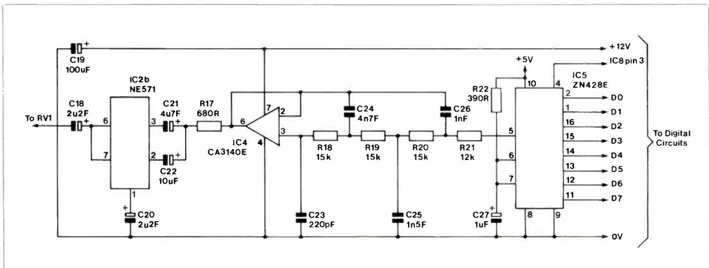
Figure 3. Digital to Analogue Converter Stage Circuit
