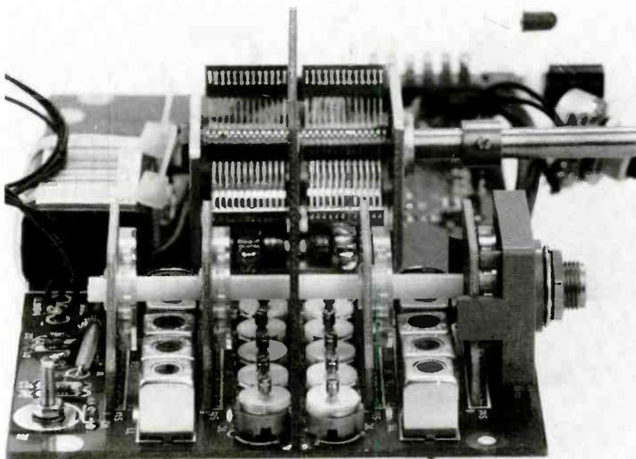
The power source for the active aerial is an internal PP3 battery or, an external DC power supply of between +7 volts and +15 volts can be used. This means the active aerial can be used virtually anywhere, i.e. at home, in the car or on a boat.
