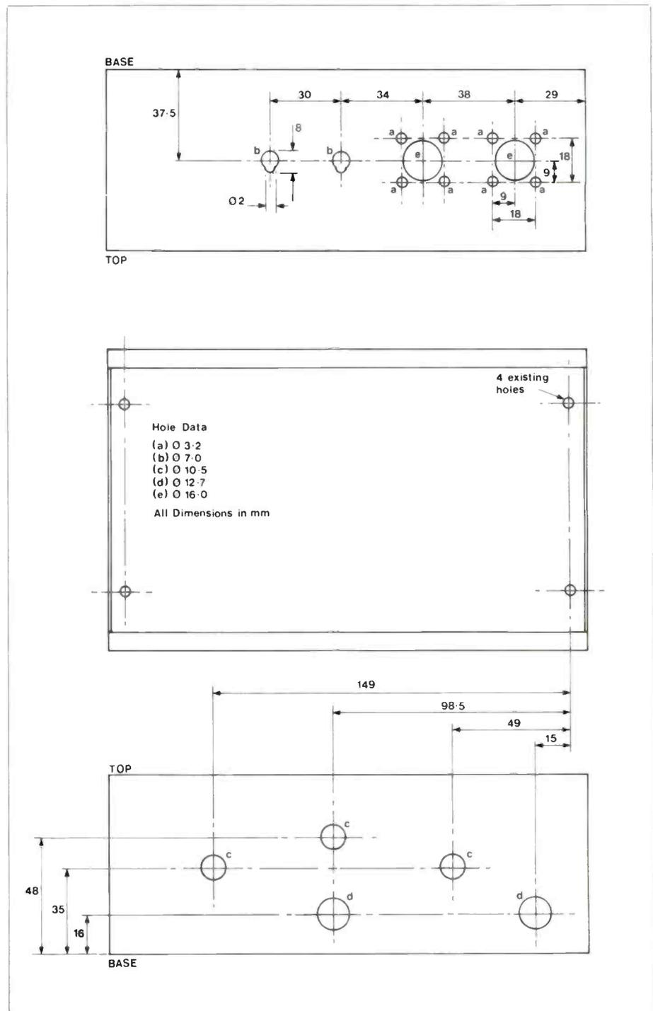
Figure 5. Tuner Case Drilling
