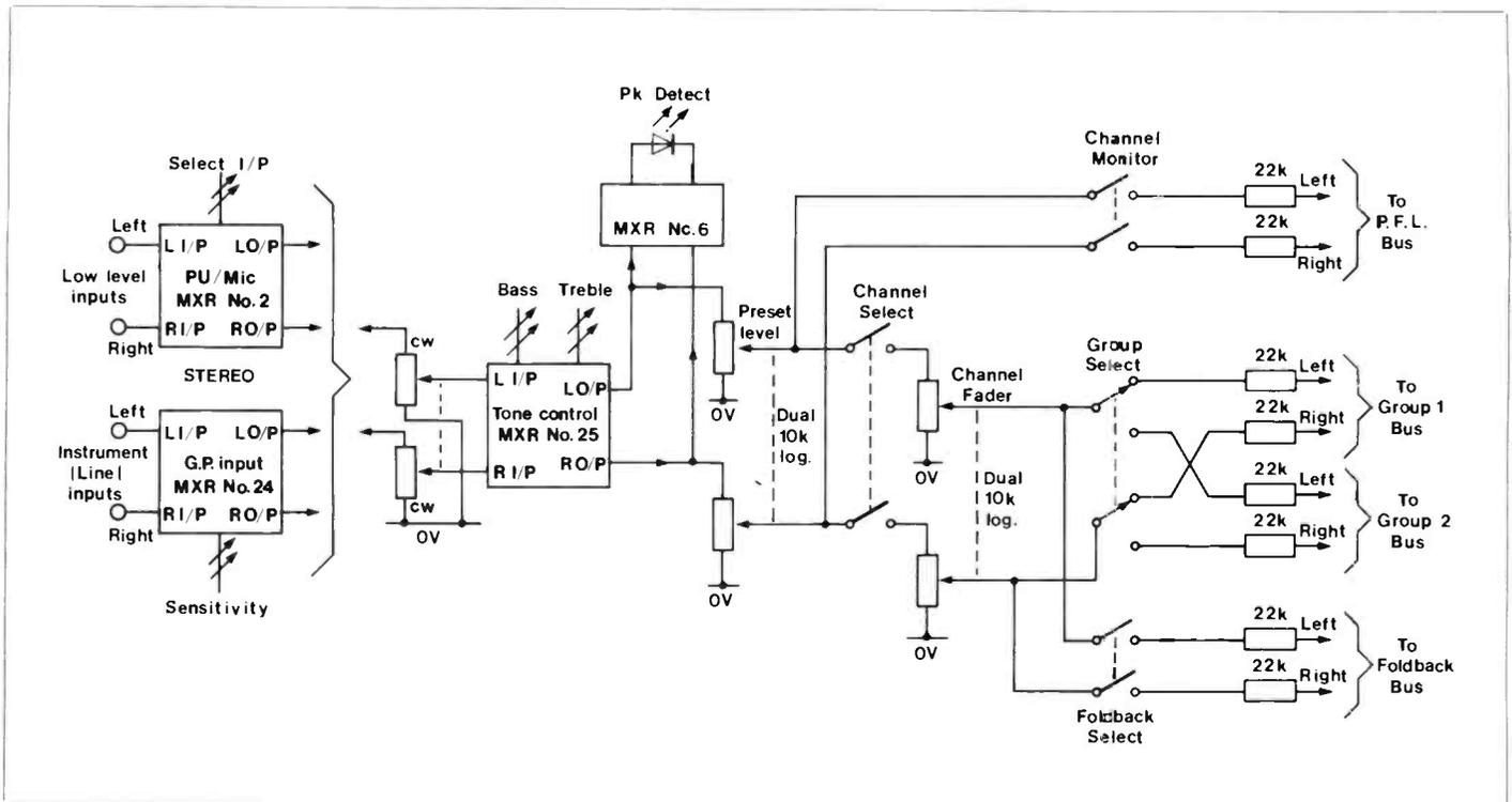
Figure 37. Typical Stereo System
