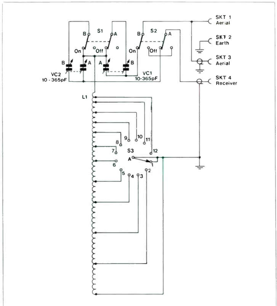
Figure 1. Tuner Circuit
