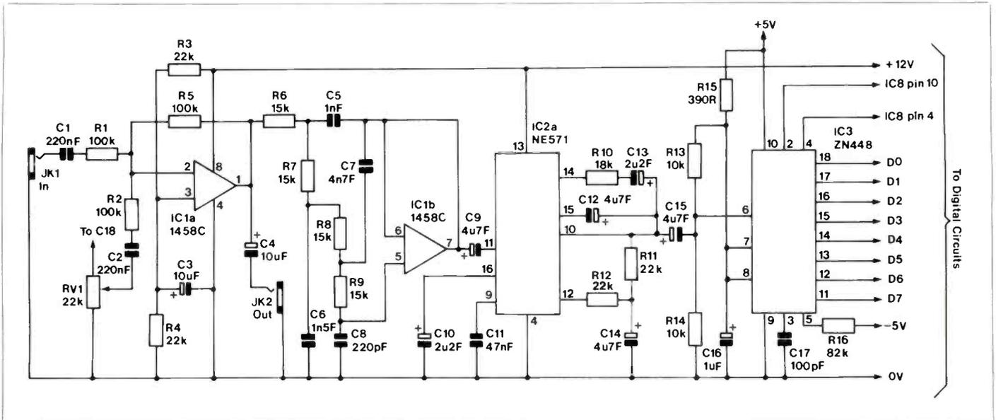
Figure 2. Analogue to Digital Converter Stage Circuit
