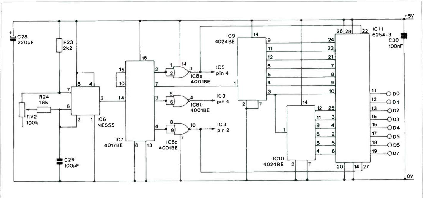
Figure 4. Clock, Control and Memory Stage Circuit
