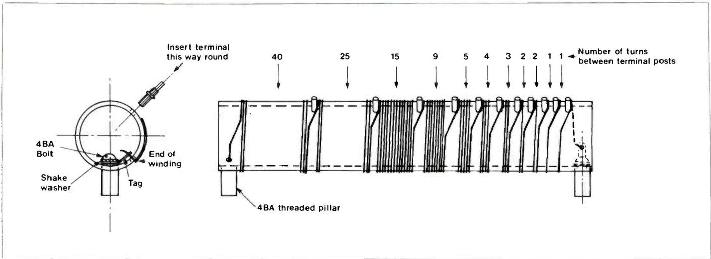
Figure 8. Coil Winding
