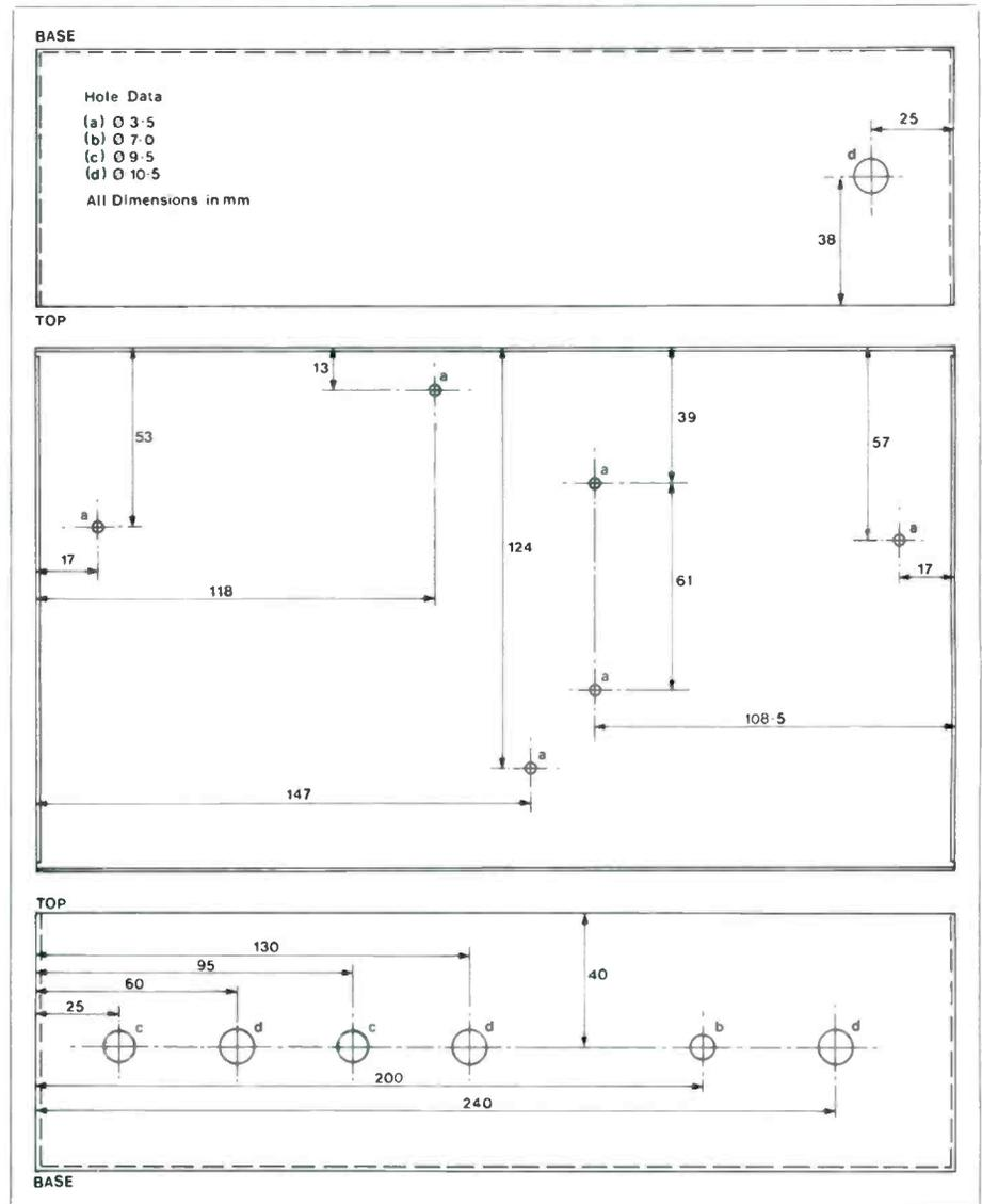
Figure 9. Box Drilling
