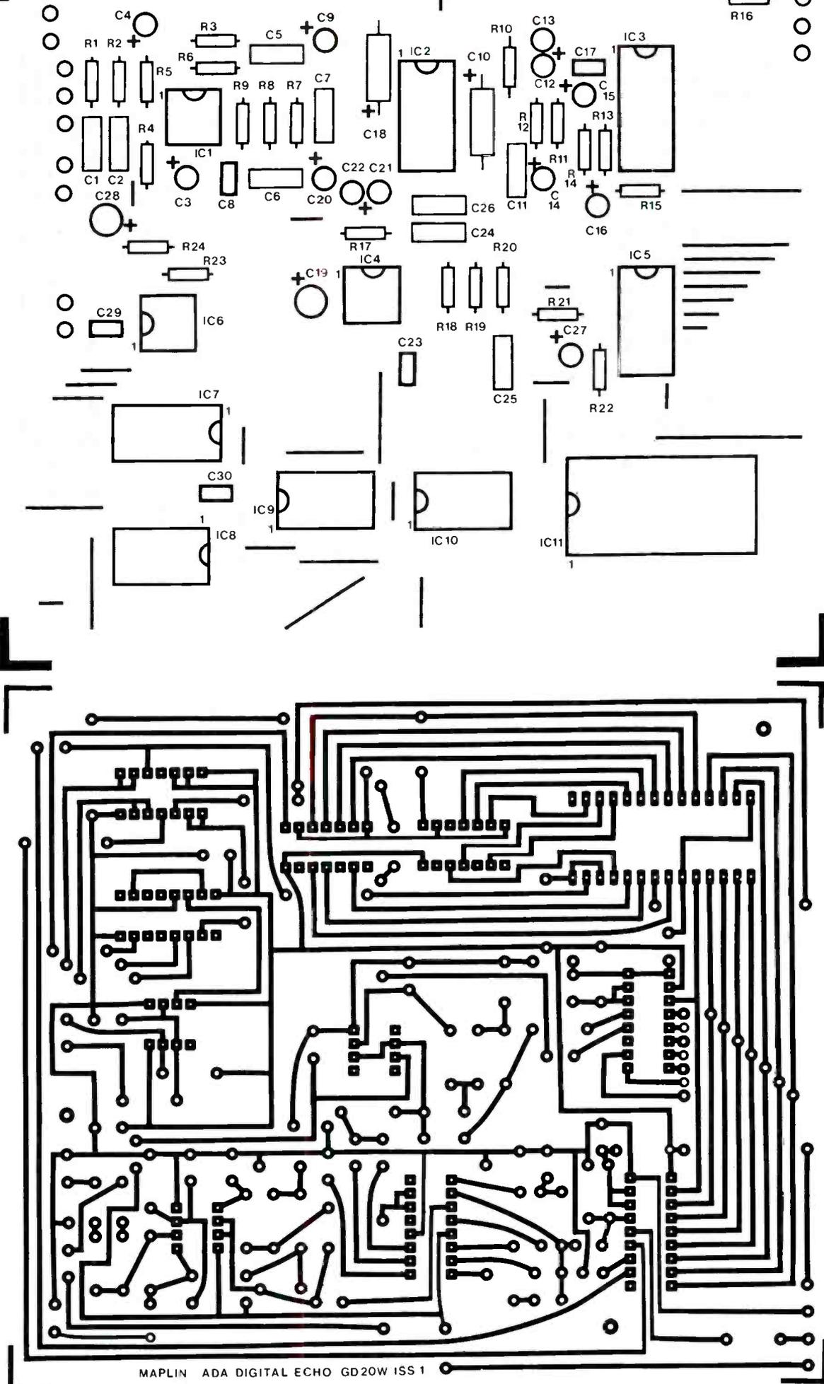
Figure 6. Main PCB Track and Overlay
