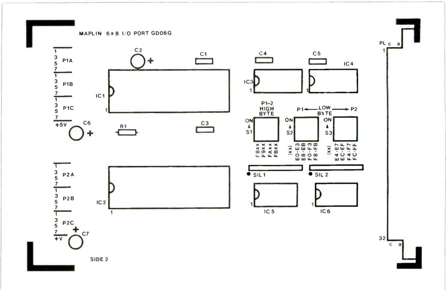
Figure 2. 6 x 8-bit Port PCB Overlay
