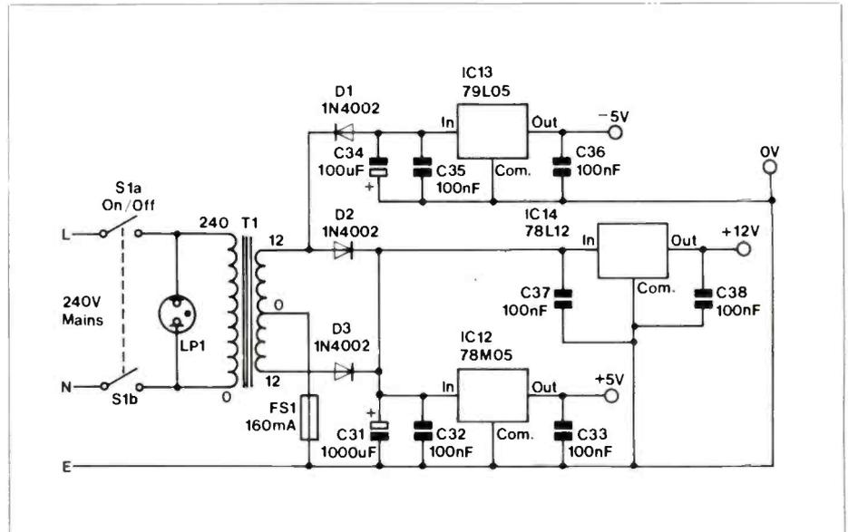
Figure 5. Power Supply Circuit
