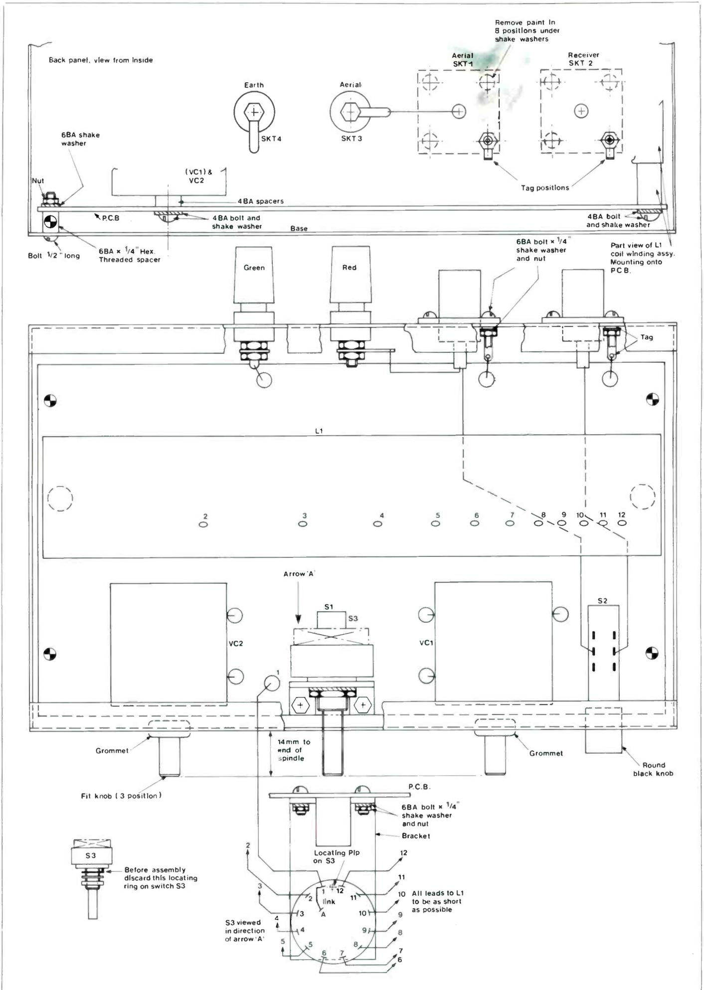
Figure 3. Wiring the Tuner
