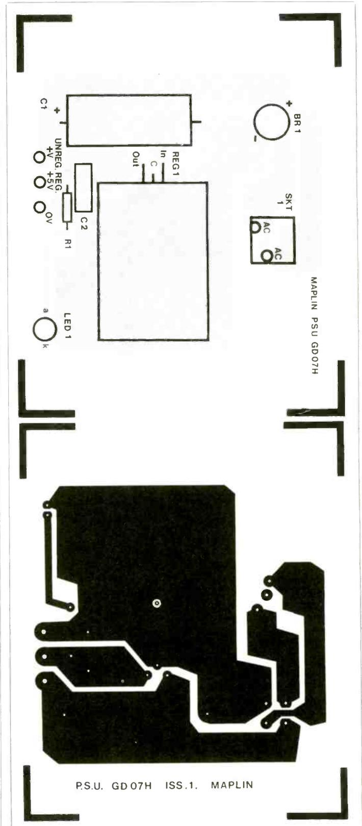
Figure 8. PSU PCB Track and Legend
