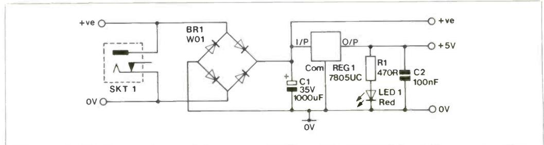
Figure 7. PSU Circuit
