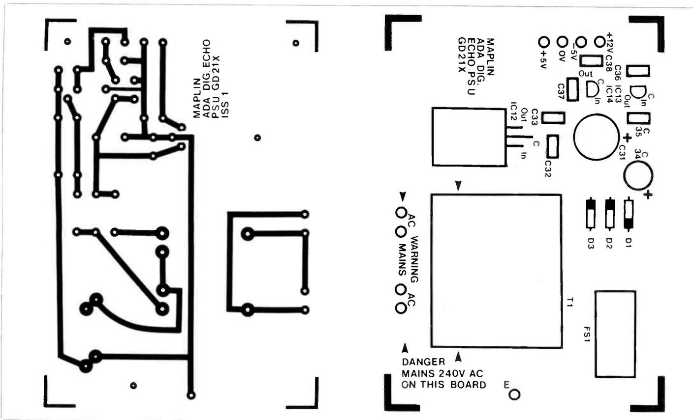
Figure 7. PSU PCB Track and Overlay
