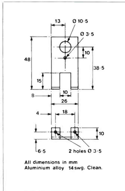
Figure 9. Tuner Bracket
