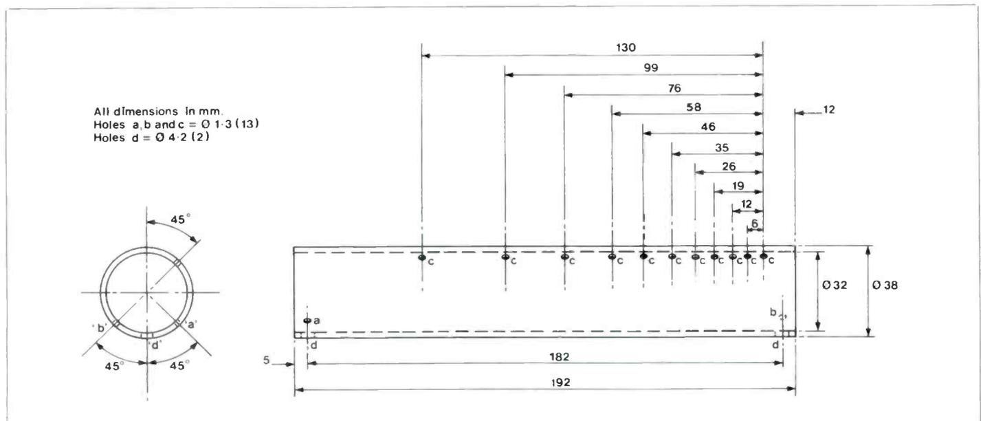
Figure 7. Coil Tube Drilling
