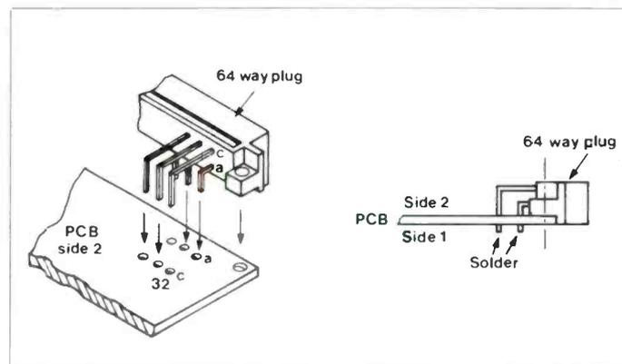
Figure 3. Fitting the 64-pin plug
