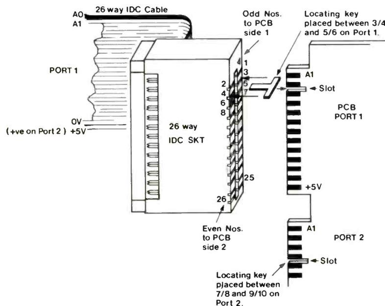
Figure 6. Connection to the 6 x 8-bit PCB
