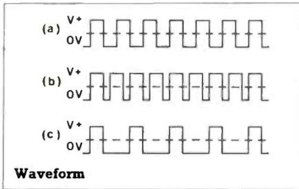
waveform diagram. If the input frequency is increased, the output pulse length remains the same, and the gap between the pulses narrows (as in (b)). With reduced input frequency the duration between output pulses increases, giving a waveform of the type shown in
