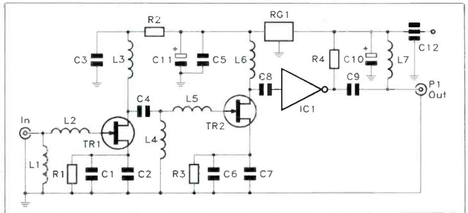
Figure 4. Pre-amplifier circuit.
