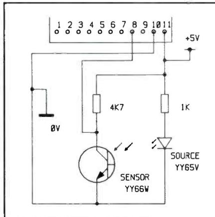
Figure 4. Opto-coupled input.
