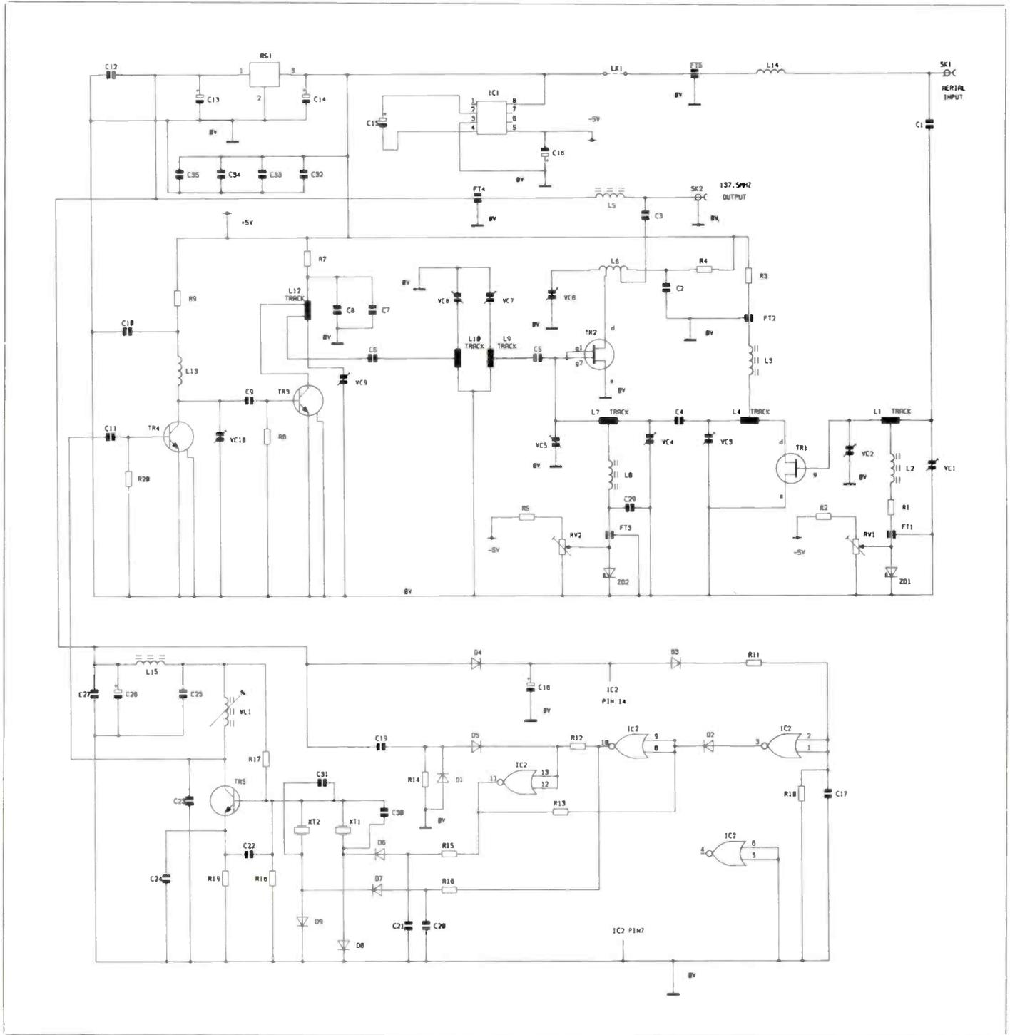
Figure 5. Down Converter circuit.
