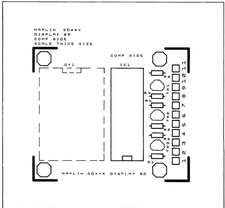
Figure 2. PCB layout.
