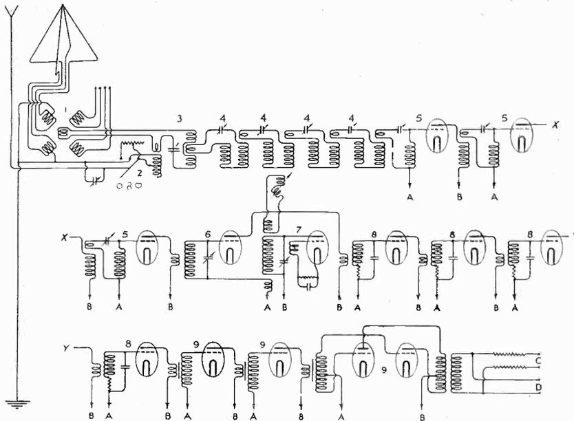
FIG. 2.—Simplified Diagram of Connections, Type R.C.6c Receiver.
