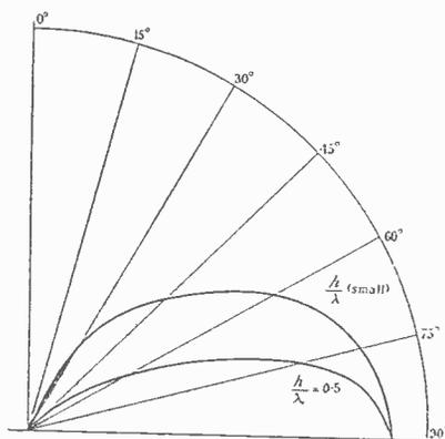
FIG. 1. — Vertical polar diagram of radiation for  $\frac{1}{2}\lambda$  and  $\frac{1}{4}\lambda$  (or less) aerials. Drawn for the same maximum radiation intensity in the horizontal plane.
