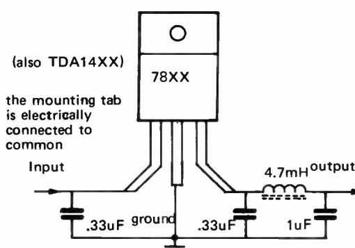
Three terminal voltage regulators are now well established as the leading means of achieving power regulation at fixed voltages. They are thermally protected and compensated - and apart from a tendency to produce RF noise, they are ideal for any application within their specification.
