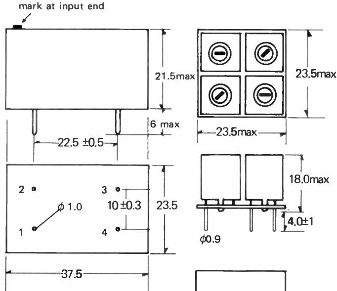
NB A DC path exists between input and output
