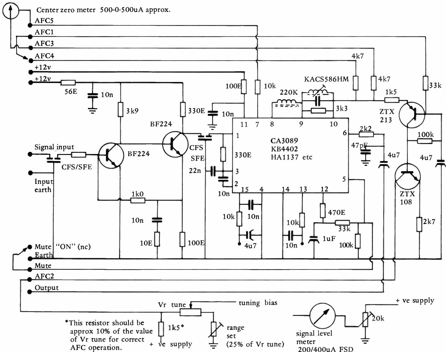
For AFC operation, connect AFC1 to AFC3.
