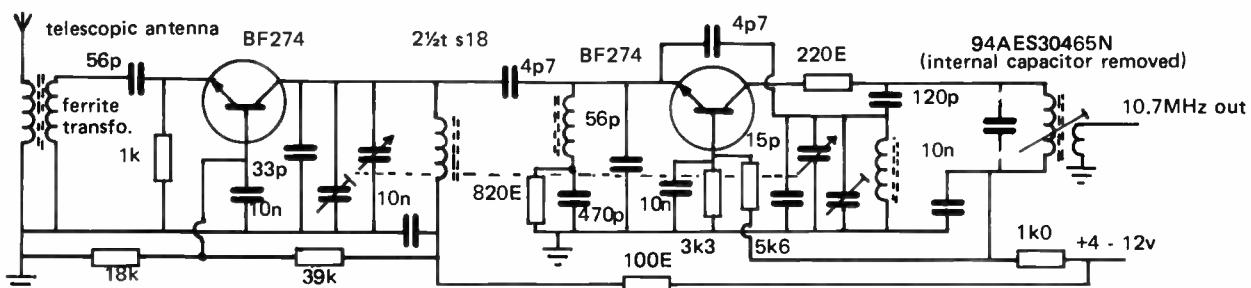
Tuning capacitor: 3.5 to 20pF per section ( or varicap)
