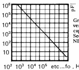
Graph of operating frequency,  $f_0$ , versus the value of the timing capacitor,  $C_0$ , for the 560, 1 & 2. See separate formula for the NE565 capacitor values.
