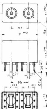
The 10K, and double 10K, are the standard choice for high stability FM and TV IFs. The construction is similar to the 7K: a spiral former, with fixed cup core, and adjustable slug. The maximum inductance for the single 10K is 50uH, with ferrites suitable for use from 2MHz to 100MHz. The double form is available with a maximum inductance of 25uH. In identical dimensions, a double 10E - the 10WA - is also available with a maximum inductance of 2mH per winding.
