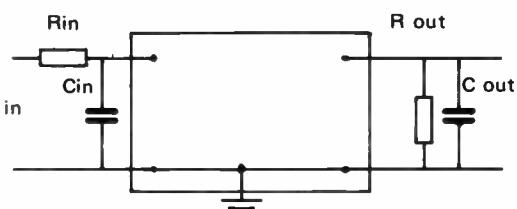
The input impedances given in the table above do not include the additional capacity required for a perfect match. The additional capacity must take into account all circuit strays.
