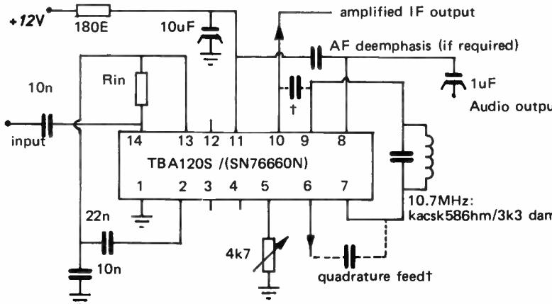
The capacitors marked † are not required at 6 and 10.7MHz in the TBA120S, as these are furnished internally.
