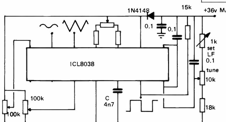
The circuit shown here represents a complete AF signal source. The outputs should be buffered in voltage followers, and provided with attenuators to suit the desired application
