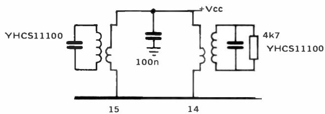
Figure 6: Detector arrangement for NBFM operation
