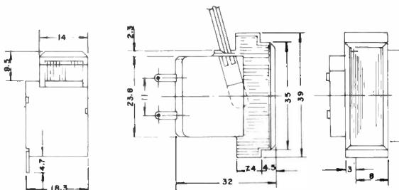
The HS12 is probably one of the most widely used basic styles in equipment today - like the others illustrated here, it is also widely copied by many other sources. Illumination may be provided by an internally mounted bulb (as illustration)
