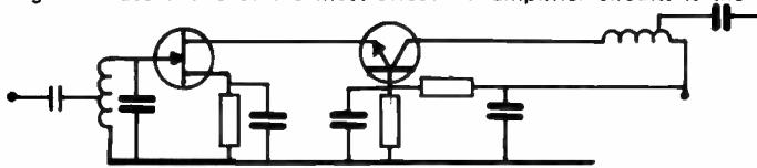
This configuration has very low feedback capacitance, hence good stability, combined with the gain of a common source stage and an excellent noise figure. Either reverse or forward AGC may be applied, with a Max gain at V agc approx. 0v. This type of circuit is well suited to 'preamp' and preselector circuits where gain control may be a manual function, since the AGC range is not as good as that of the standard dual gate MOSFET stage.
