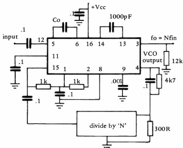
Figure 4. The NE565A as an FM demodulator for FSK, offering increased output over the 560/1/2, but at a lower frequency.
