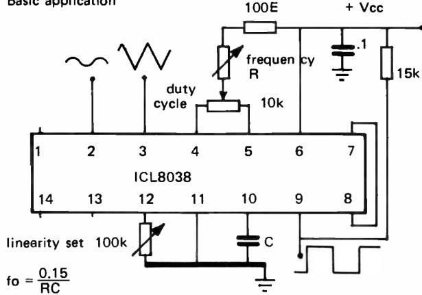
The 8038 is an exceptionally versatile waveform source for various applications in test equipment, musical sources, tone generation. Sine, square and triangle outputs are simultaneously available, with excellent amplitude stability.
