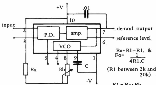
1000pF connected between pins 7 & 8 will eliminate the possibility of VCO instability
