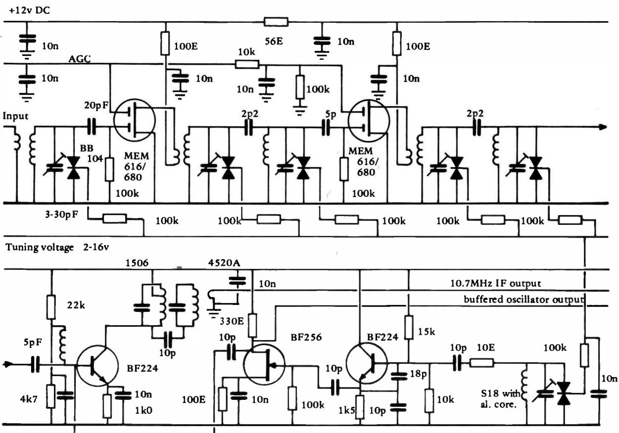
For optimum noise and gain performance, the source of the two input MOSFETs is taken to the nearest available earth point. Greater AGC range may be obtained by using a decoupled source resistor of approx. 100 ohms, but in most applications the gain is the important factor.
