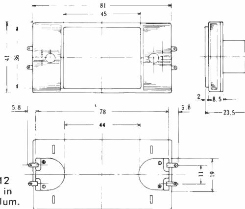
A very low priced double meter, with movement characteristics similar to the HS12. It is possible to combine a centre null function with a left/right biased movement in this style - for example as a combined tuning and signal level meter. OK for rear illum. Standard scales in leaflet 200uA FSD movement R 750 ohms
