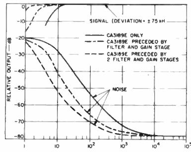
Fig. 8 - Typical limiting and noise characteristics.
