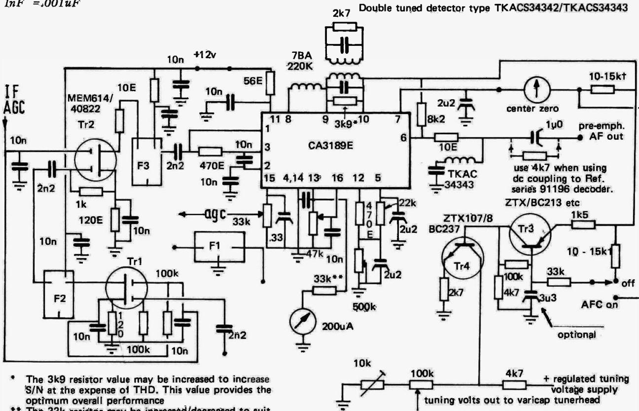
\* The 3k9 resistor value may be increased to increase S/N at the expense of THD. This value provides the optimum overall performance
