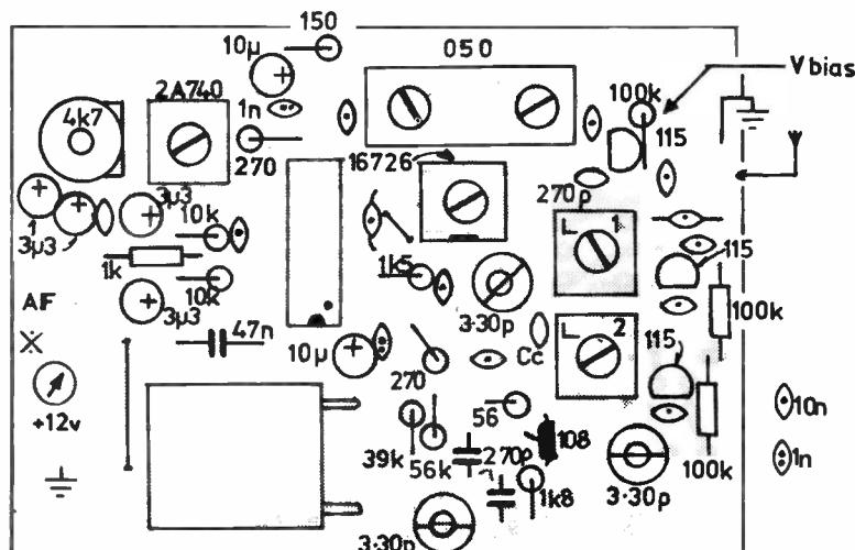
\*Cc The coupling capacitor for the input stage, values will vary with selected frequency range. Generally 8p2 will be suited to most applications to 7MHz. 7-14MHz use 4p7, above 14MHz 2p2. (Smaller values will increase selectivity at the expense of sensitivity.)
