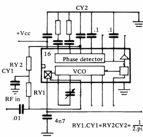
Figure two. The NE561B AM synchronous detector
