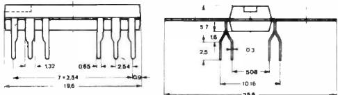
The TBA810AS and TCA940 are interchangeable audio power ICs - the only differences being the increased supply voltage capability of the TCA940, coupled with the increased output power of the TCA940
