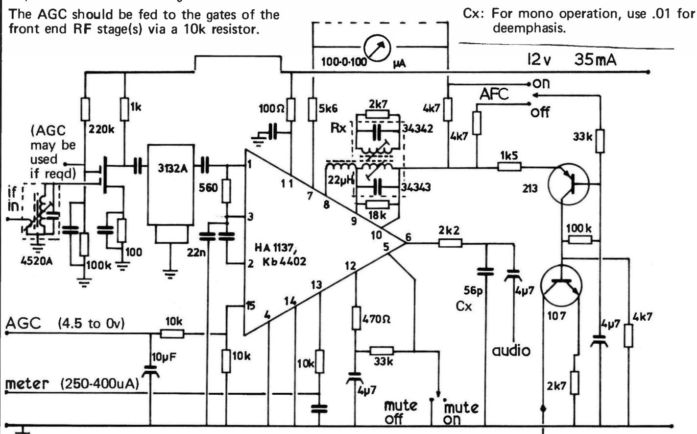
All unmarked capacitors are .01 disc ceramic
