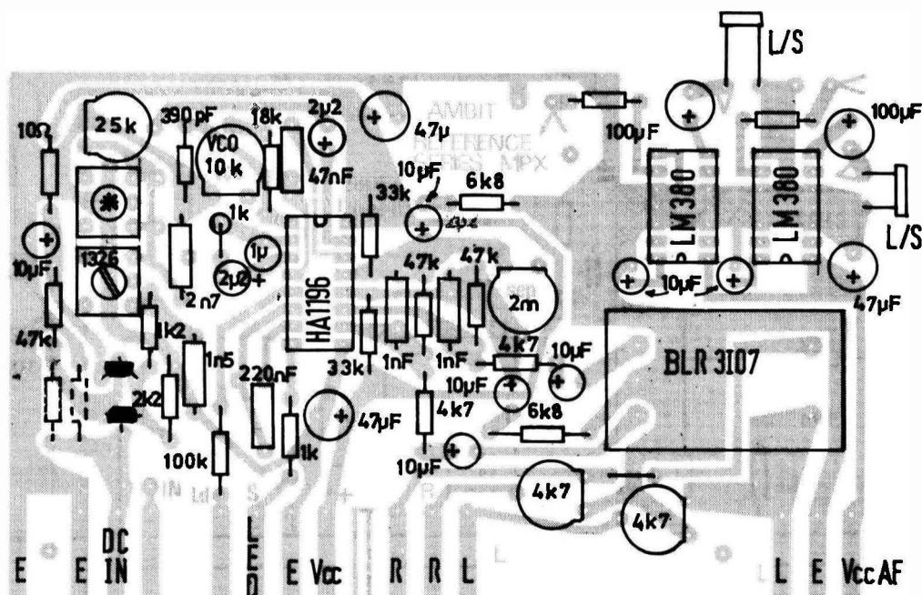
The resistors forming a PD at the base of the input stage are optional - since when this unit is used in conjunction with most IF/detector ICs (3089 etc) the output from the IF may be DC coupled to the base of the input stage, via 4k7.
