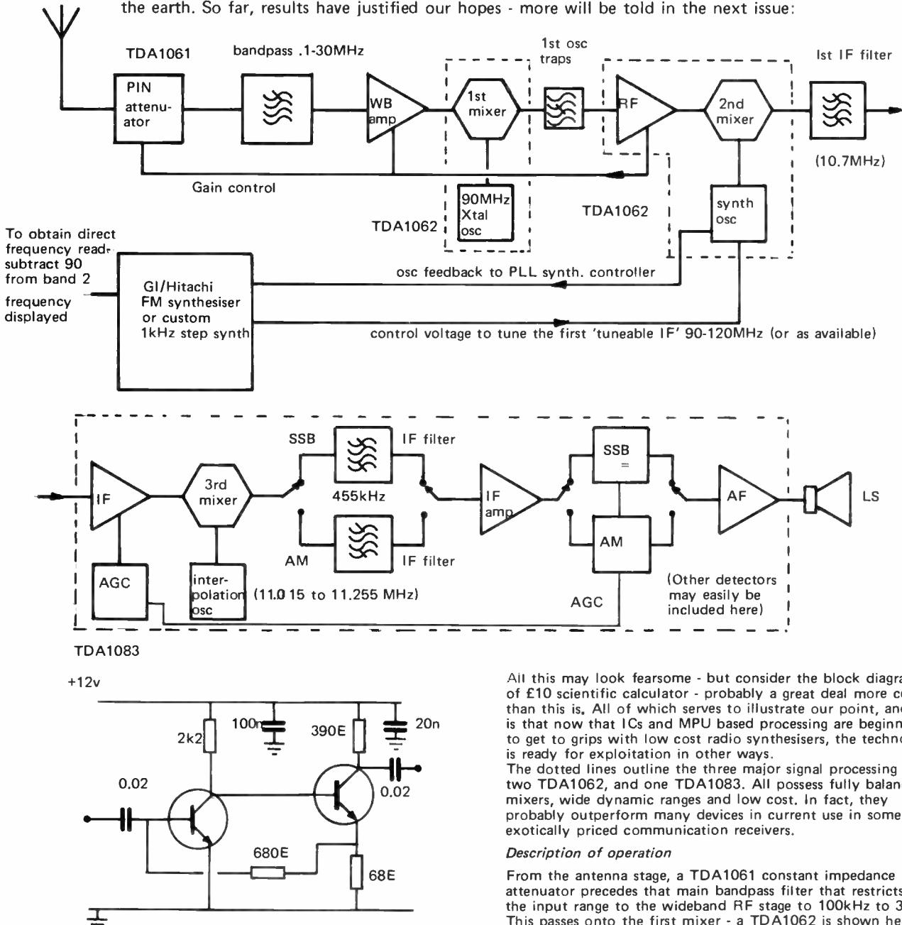
A wideband RF amplifier having a voltage gain of 24dB and a spot noise figure of 3.5dB at 100MHz. The upper -3dB point is 160MHz for 2N3570 transistors, largely dependant on component lead lengths. Use of new devices, such as the BF479 should result in superior results, with greatly reduced noise and improved gain. (Remember to invert the supply for PNP devices). In fact, the basic BF274 will be quite good enough for HF use.
