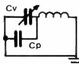
There are two basic approaches to the techniques of electrical bandspread - for a variety of reasons, the usual result is a combination of the two, since the impedance of the tuned circuit is very low with a high value of parallel capacity - and thus not suited to many oscillator applications - or very high with a large value of inductor, where the stray capacities inherent in PCBs and wiring limit the overall tuning range through a tight restriction on the factor ' $V$ ' (Capacitor ratio)
