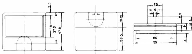
The HS13 series are widely used in recording and tuner applications with mounting either way up. The translucent back permits illumination of scale from behind.
