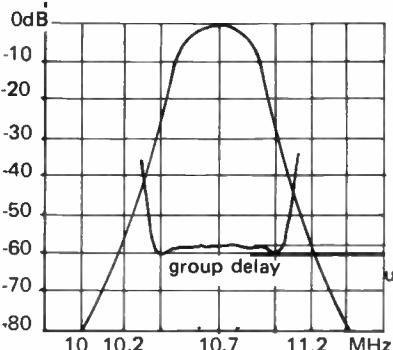
in most major parameters, and possess a far lower insertion loss - but all types of ceramic filter require an LC tuned circuit to precede their application, since an entirely ceramic filter would not possess adequate 'out-of-band' attenuation. Finally, the long filter is excellent, and the
