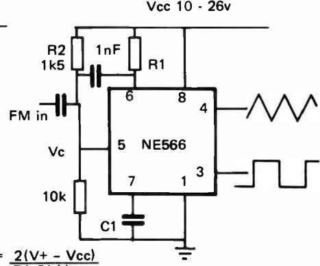
The NE566V is a wide range triangle/square wave function generator which can also be modulated over a ten to one range by a suitable choice of components.
