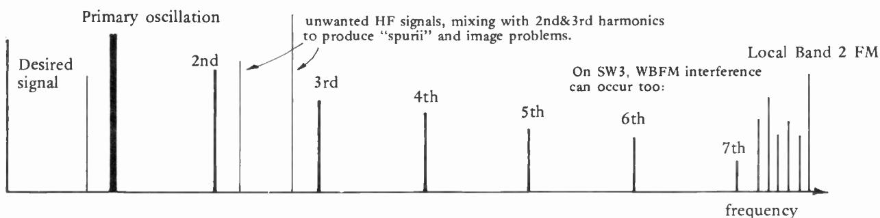
Figure four: A spectral consideration of SW mixing and spurii problems
