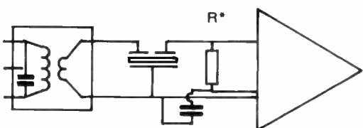
The CFSE filter is especially characterized for group delay consistent with good stereo reception. The CFS is more suitable in mono and 'rooftop' applications.
