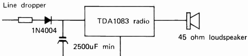
Figure three: The mains dropper system
