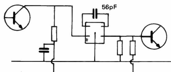
The SFD is a long established ceramic block filter for AM IFs. A 56pF external capacitor is required for neutralization, and coupling the two internal ceramic resonators.
