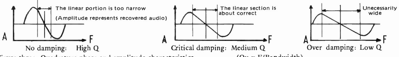
Figure three: Quadrature phase and amplitude characteristics
