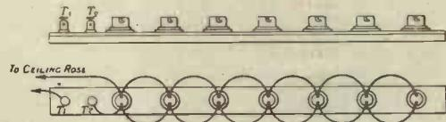
Fig. 2. Construction and wiring of the lamp resistance.
