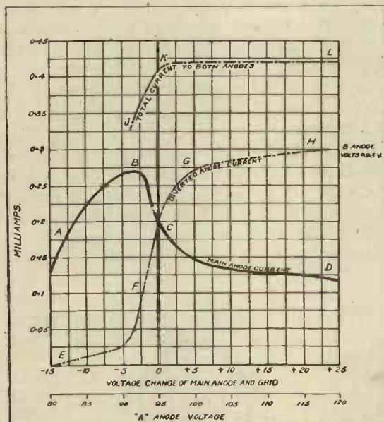
Fig. 3. Characteristic curves of the negatron, main anode and diversion anode currents being plotted against change in grid voltage.
