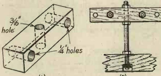
Fig. 7. Supports for the secondary.
