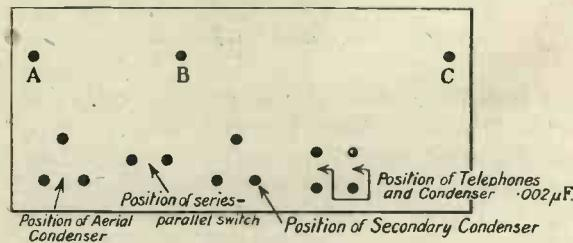
Fig. 6. Plan of the base-board.
