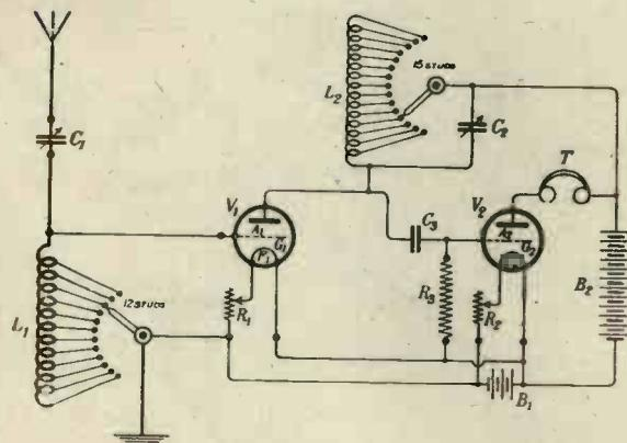
Fig. 3. Circuit of the two-valve receiver.
