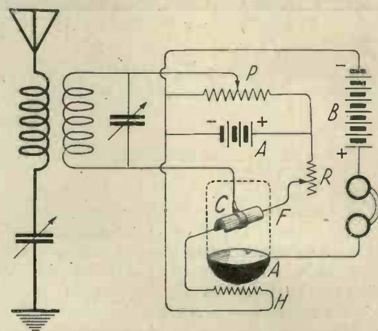
Fig. 2. Circuit of the new rectifier tube. Note the resistance in series with the filament. The current consumption is about the same as that of a standard tube.
