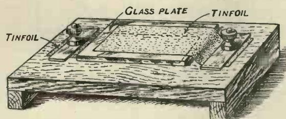
Fig. 8. Illustrating a home-made grid condenser.
