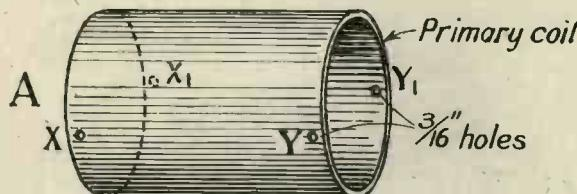
Fig. 4. Details of primary tube.
