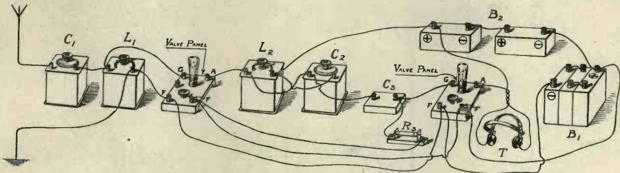
Fig. 2. Connections of the two-valve set.
