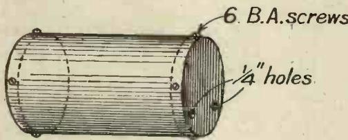
Fig. 1. Tube for secondary winding.
