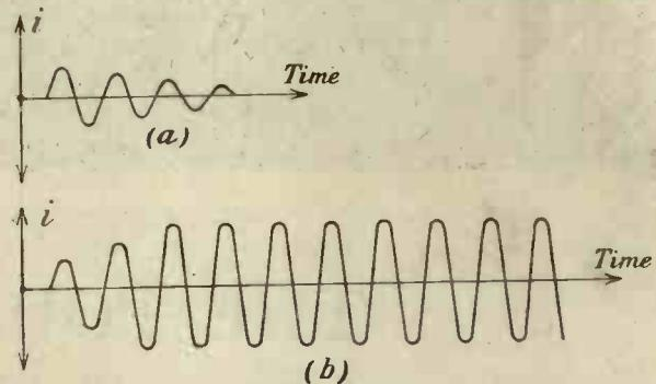
Fig. 4. The damped oscillatory discharge of a condenser.
