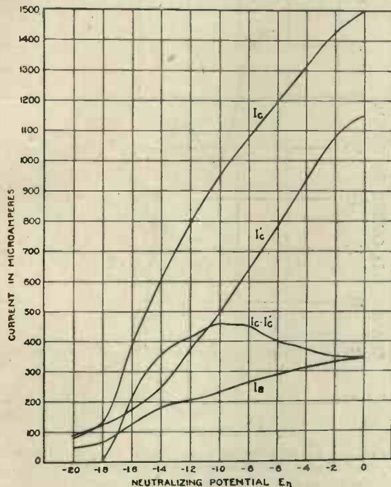
Fig. 3. Variation in anode and collector currents  $I_a$  and  $I_c$  with variation of neutralising potential  $E_n$ .
