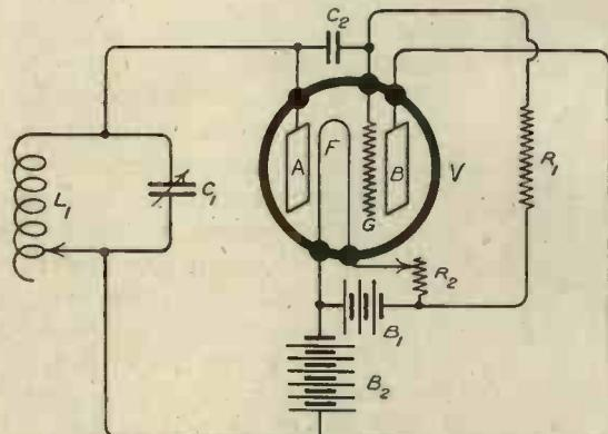
Fig. 4. The negatron employed as a generator.
