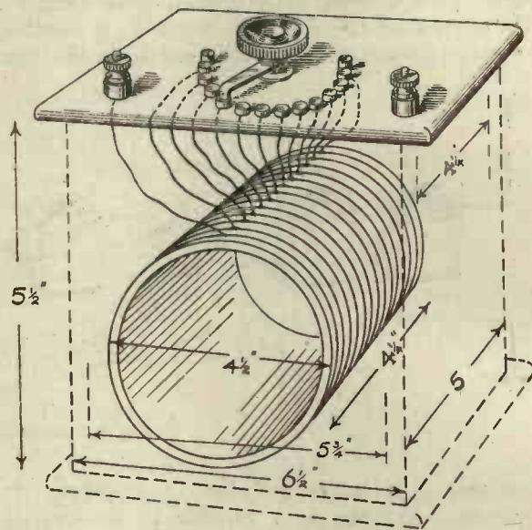
Fig. 6. The coil in position.
