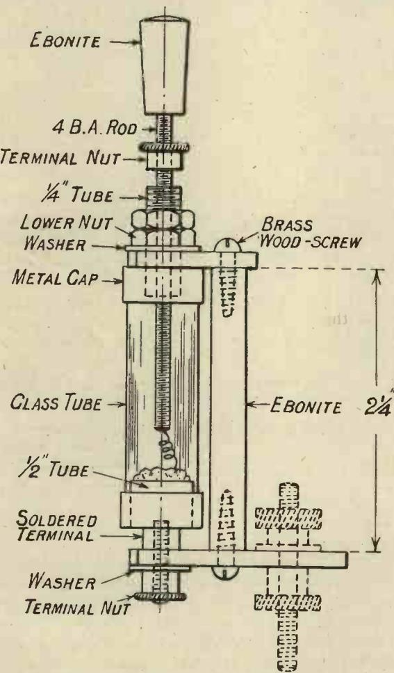
Fig. 1. General arrangement of detector.
