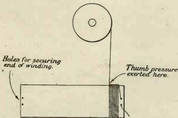
Fig. 1. Illustrating method of winding.
