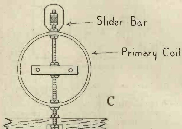
Fig. 9. Showing the position of the supports for the secondary within the primary.
