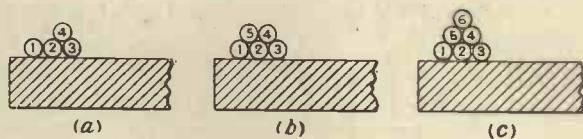
Fig. 5. Commencement of a three-pile winding.
