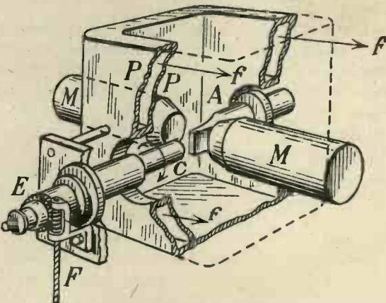
Fig. 7. A diagrammatic representation of the interior of an arc chamber.
