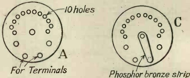
Fig. 2. Arrangement of secondary switch.
