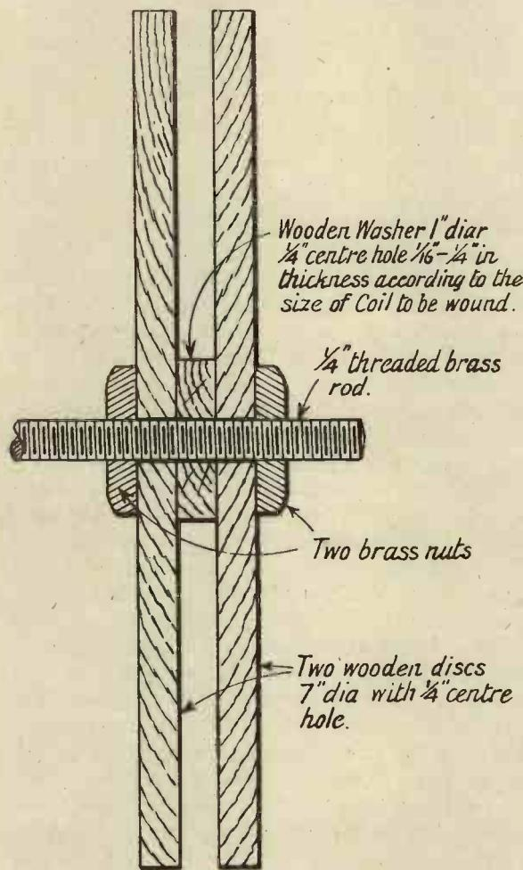
Fig. 1. Section of slab coil winder.
