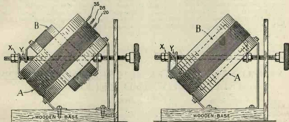
Figs. 1 and 2. Showing the general arrangement of the coupling device.
