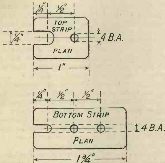
Fig. 2. Details of brass strips.
