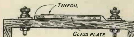
Fig. 9. Side view of the grid condenser.
