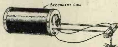
Fig. 5. Assembly of secondary coil.
