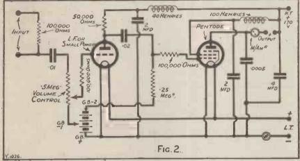
A very thorough system of de-coupling the various H.T. feed leads was found highly desirable.
