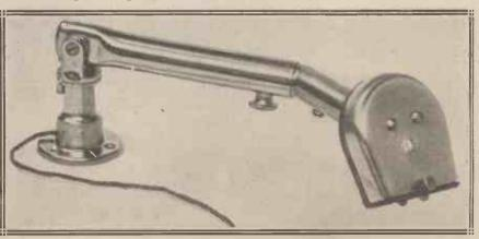
The pick-up and carrier-arm used during the test-the pick-up has since been redesigned by the makers and now has different characteristics from those shown overleaf. 516
