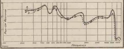
The curves obtained with and without the volume control in action across the pick-up. Note how closely they correspond.
