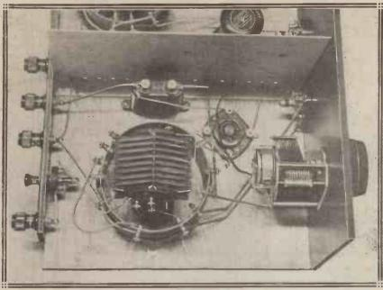
Note the special series condenser and shorting switch for the aerial circuit mounted on the terminal strip.
