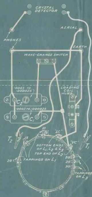
on 50 turns in all. This is the secondary coil  $L_2$ , and the end is joined to the terminal "V.C." on the coil former.
