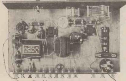
Most of the wiring is clearly shown in this photograph, which should be studied in conjunction with the diagram on the opposite page when building the set. The panel layout is simple and gives a workmanlike appearance to the set.
