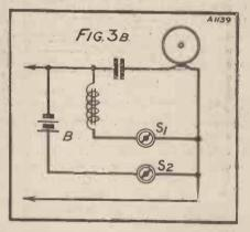
$S_2$  switches the set on and off. Across the loud-speaker extension leads at the set end are the additional items shown in Fig. 3A.
