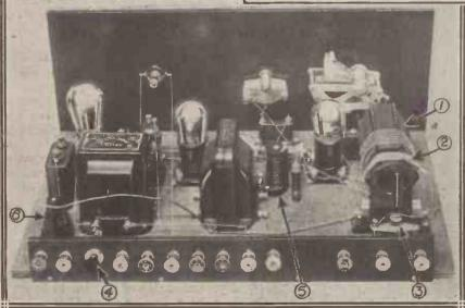
A general view of the set. (1) and (2) are the reaction and tuning coil, and the aerial coil respectively; (3) the series condenser  $C_3$ ; (4) the loud-speaker switch; (5) the reaction H.F. choke, and (6) is the output H.F. choke.
