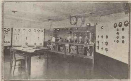
The transmitting apparatus at the Munich broadcasting station. This German station operates on a wave-length of 533 metres with a power of 1.5 kw. It can easily be received in this country on simple valve sets.
