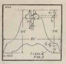
then be traced over with a wellpointed pencil, using a straight-edge where practicable, and taking care to trace the whole of a pattern once (and only once) before lifting the drawing from the wood.
