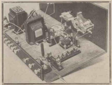
This photo shows how the coil holder and the aerial coupling condenser are placed and connected.
