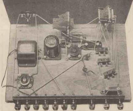
The two neatly-spiralled flex leads you see here are the connections to the tapping points on the two "X" coils. (The photographer coiled them up to make them more prominent.)
