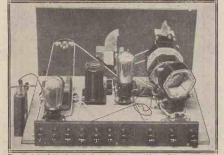
There is plenty of vacant space in the set for the accommodation of the small grid-bias battery required. The little unit illustrated, for example, could stand upon the baseboard beside the L.F. valve socket.
