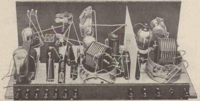
Be careful to arrange your coils in the way you see here. The best position was determined by test, and the screen completes the "separation" of the circuits quite effectively when the loading coils come at the angles shown.
