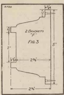
The dimensions for the brackets that support the cross-piece.
