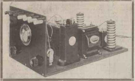
The special H.F. stopping filter is placed at the back of the unit. Note the heavy-duty H.F. chokes.
