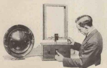
The "Universal" frame aerial fitted to the "Flat-Dweller's" Four, which was described in. "M.W." some months ago. coupled stage will give more amplification it requires careful screening for complete stability. If you use a pentode after the detector you will have a powerful three-valve combination, and if careful consideration is given to the efficient design of the frame aerial and to the choice of the H.F. coupling choke, the performance
