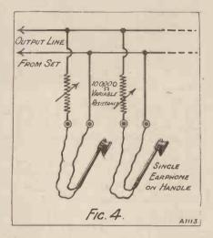
The output lines may be of the same wire as the microphone leads, and need not necessarily be lead-covered.
