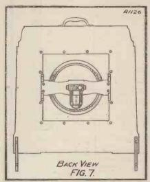
Note that the cross-piece is sunk into the brackets for strengthening.
