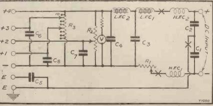
The circuit is a straightforward one, but capable of smoothing-out ripple from even very "rough" mains. If H.F. smoothing is not required the circuit can be simplified at the points marked X, as explained in the article.
