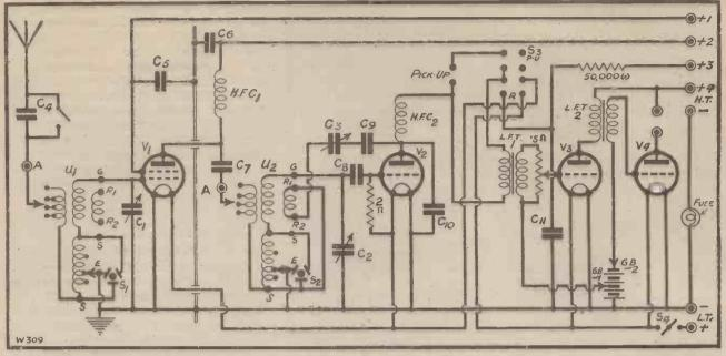
This is mounted upon the terminal strip in the usual position, and by pushing the knob inwards you have the series condenser in action, while by pulling it outwards the condenser is cut out of circuit. With the aid of this device and also the tappings on the low-wave primary winding and upon the long-wave loading coil, you can obtain a very wide control of selectivity and can suit greatly differing conditions.
