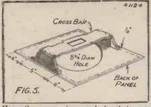
How the cross-piece and brackets are fitted together.
