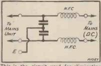
This is the circuit used for eliminating the interference.
