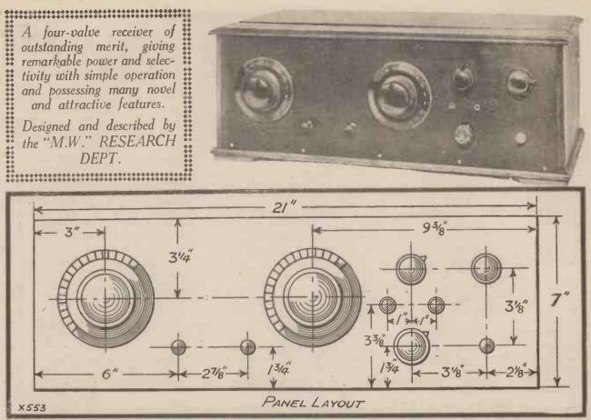
The set has a number of special refinements, and so there are quite a few knobs on the panel, but it is not complicated to operate. The wave-change switches are between the tuning dials, to the right and below are the reaction condenser and L.T. switch, above these are the radio-gramophone switch and the volume control.
