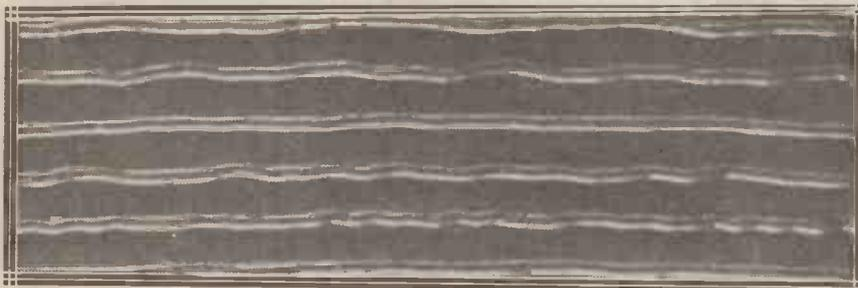
Fig. 3. A section of the same "band" record after the B.T.-H. pick-up has played it 50 times. Little trace of deformation of the grooves is visible. The polish of the record face is worn off, hence the dulness of some of the "crests."
