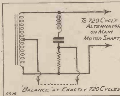
At a frequency of 720, therefore, the voltage across the dotted line shown (that is, between the junction point of the resistance and condenser-choke side, and the centre-point of
