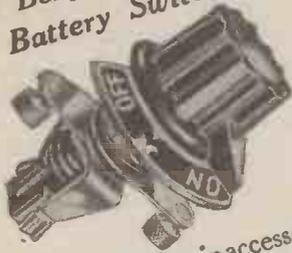
This is a new Benjamin accessory offering a pleasant alternative to the usual pull and push type of switch. It is all insulated and has an indicating "on" and "off" dial, pointer knob, terminals and double contact. It gives a quick and positive make and break action, and is suitable for use with panels up to 3/8 inch thickness. You will see this component featured on quite a number of sets this season—ask to see it at your dealers and you will realize why.
