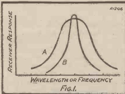
it leads to improved quality of reproduction, other things being equal. Before we can see how these effects are produced we must just run over a few elementary facts about the behaviour of tuned circuits to refresh our memories.
