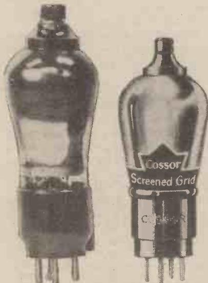
Two typical screened-grid valves—the Marconi and Cossor two-volters.
