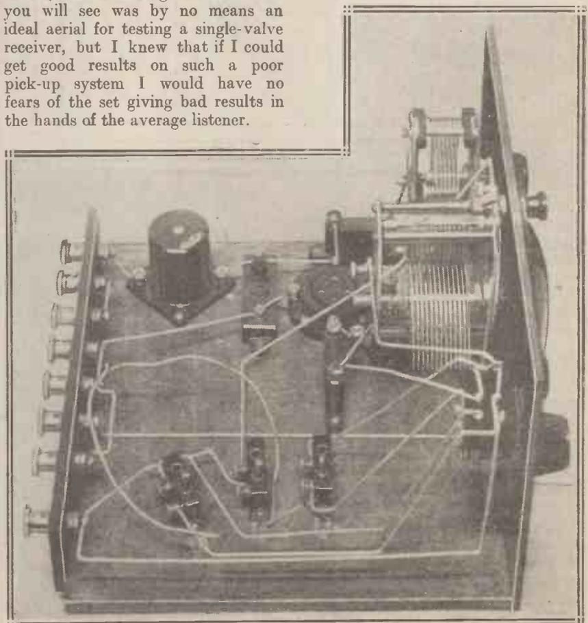
The two flexible leads in the foreground of this photograph are for the tapings on the two "X" coils. The centre coil holder is the supplementary reaction coil.
