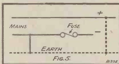
of the mains leads which will blow at nothing greater than, say, a third of an ampere. Do not make the mistake of using only the one fuse. We have said enough about mains, we hope, for you to have firmly grasped the idea that it might so happen that you inserted the fuse in a wire which happened to be grounded. Obviously this would do nothing to prevent damage arising through the other wire short-circuiting to earth.
