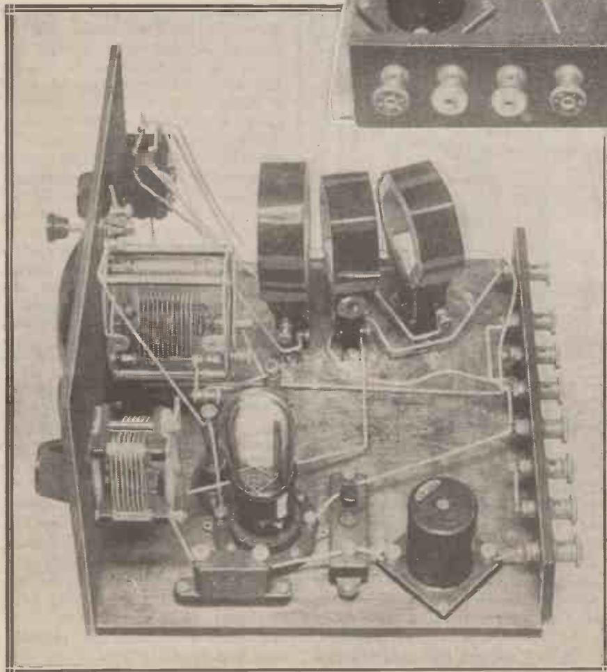
The orientation of the medium-wave coil holder (nearest the terminal strip) is very important, since it has a great bearing on the smoothness and efficiency of the reaction control.
