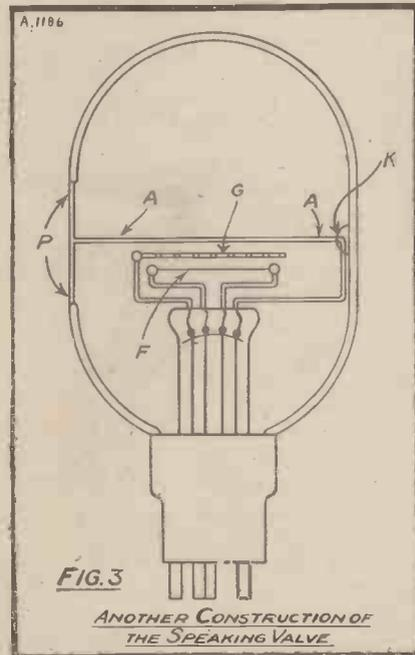
and flanges C are attached to the latter so as to form a partially enclosed air-space, which acts as a resonator to strengthen the sound. The grid G and filament F are arranged as shown.
