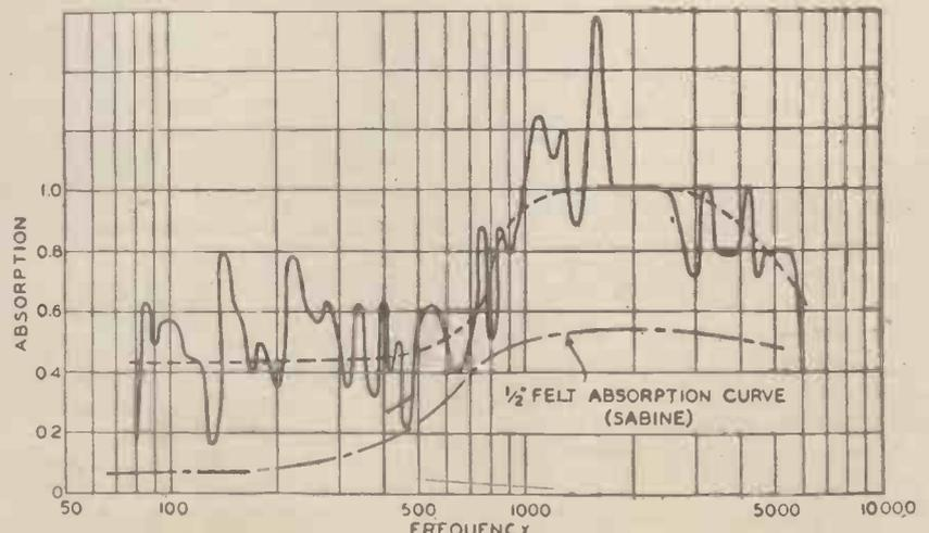
Fig. 8. Absorption-frequency characteristics in felt-lined room.
