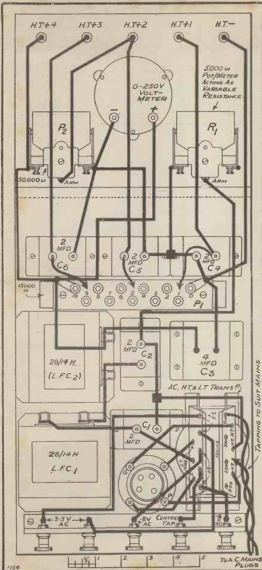
It is usually desirable in such cases to break into the wiring of the receiver and take out a separate H.T. supply lead for the first L.F. valve. This valve should then be run from H.T.+3 on the mains unit, the plug appropriate thereto being placed in the No. 8 or 9 socket of the tapped potential divider.
