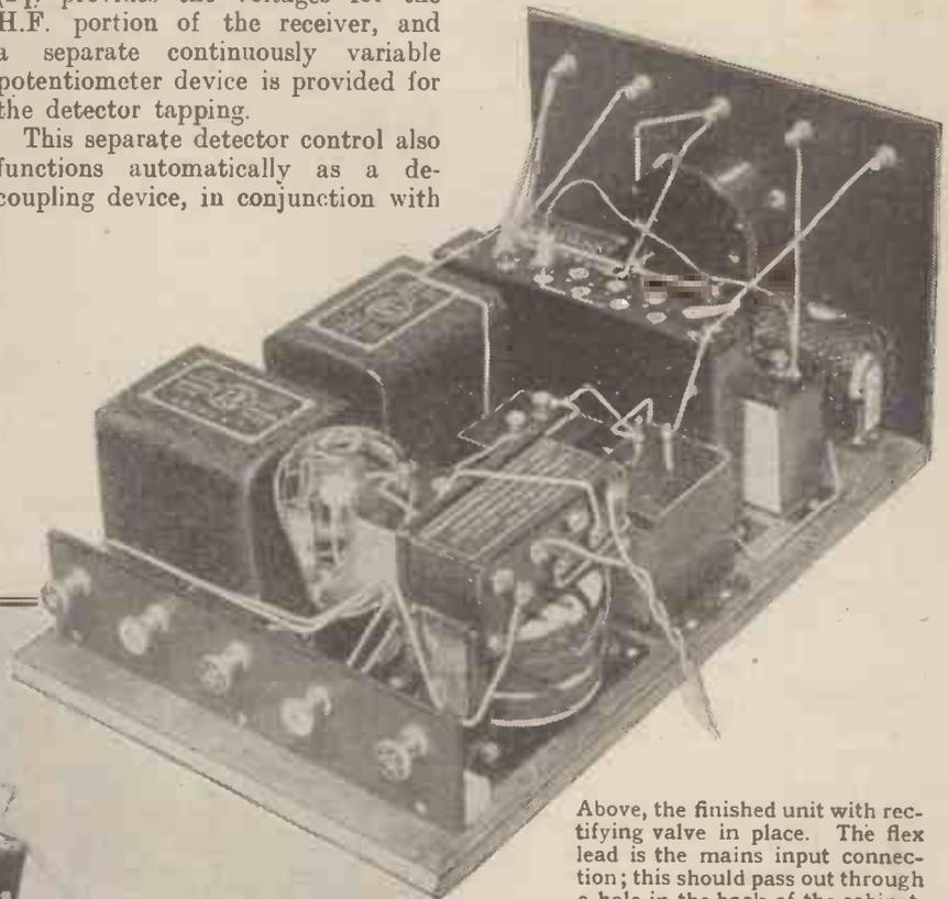
Above, the finished unit with rectifying valve in place. The flex lead is the mains input connection; this should pass out through a hole in the back of the cabinet. To the left you see the row of low-voltage A.C. output terminals.
