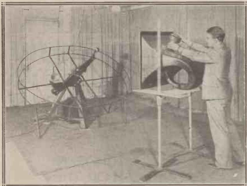
Fig. 6. The machine for rotating the condenser-transmitter to make indoor loud-speaker measurements.
