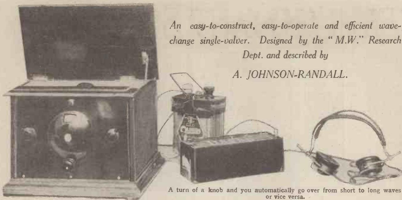
An easy-to-construct, easy-to-operate and efficient wave-change single-valver. Designed by the "M.W." Research Dept. and described by
