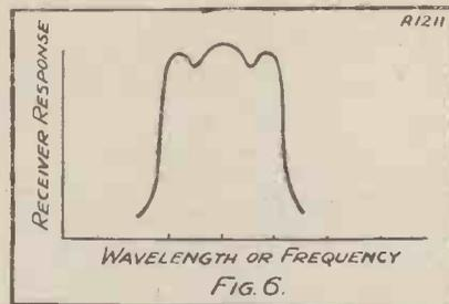
In the set in question,  $C_3$  was actually a small neutrodyne type of condenser, and with the particular capacity chosen a distinct broadening
