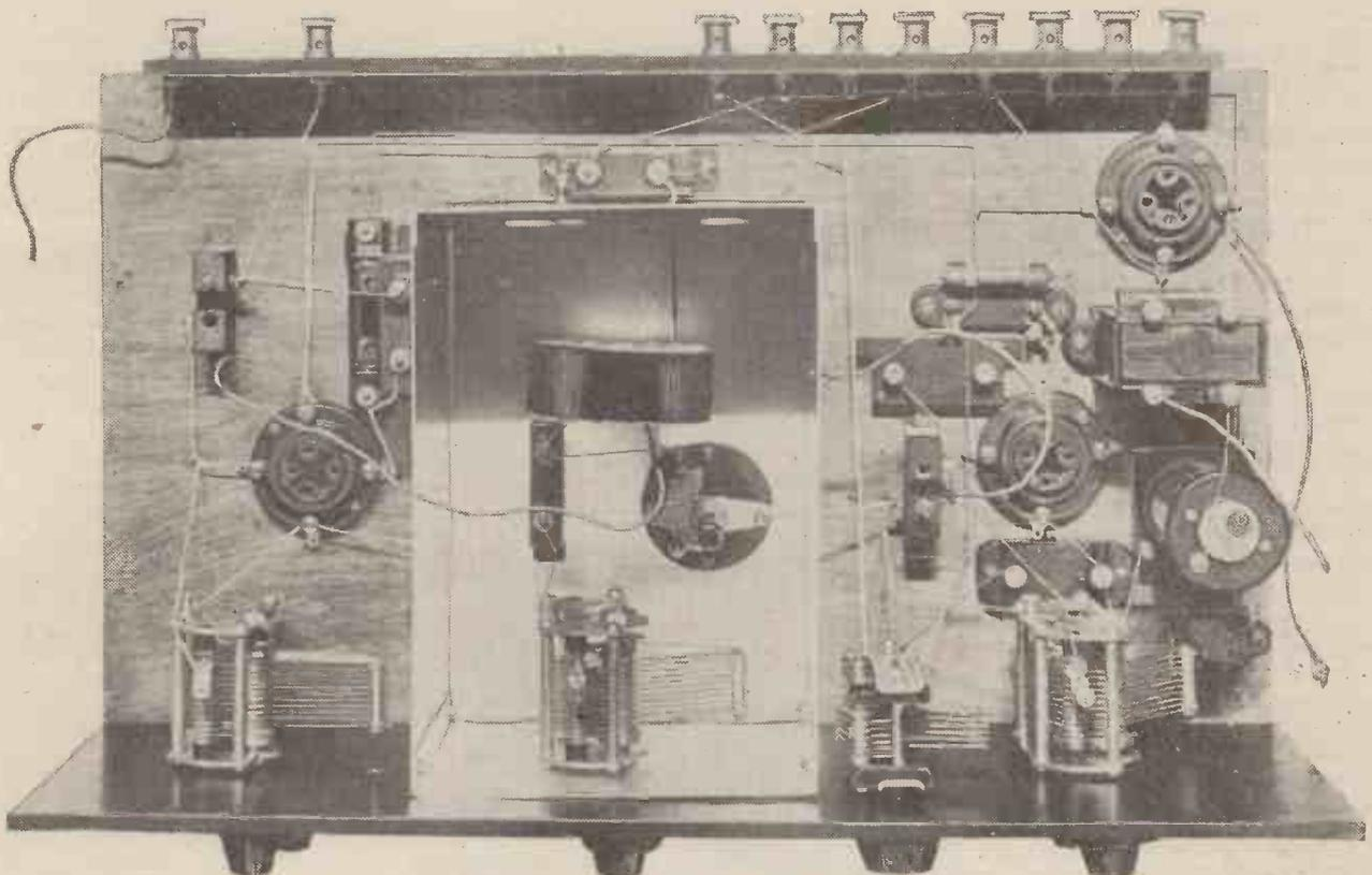
In the "Brookman's" Three the coupling between the two circuits forming the filter was adjustable by means of the neutrodyne type condenser inside the screening box.
