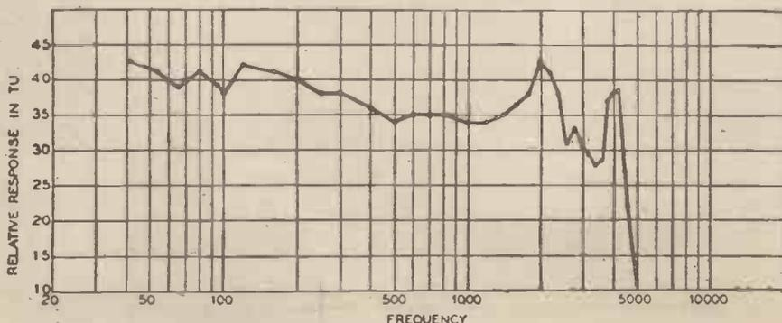
Fig. 1. The response curve of a pick-up, showing several resonance peaks.
