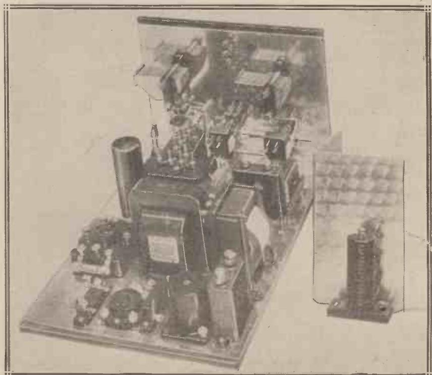
In building the set the last operation before wiring up is the attachment of the partition screen and the parallel-feed H.F. choke.
