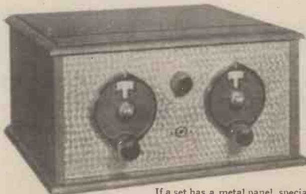
If a set has a metal panel, special precautions must be taken before a mains unit is used. Remember, it is possible for the whole panel to be "live."
