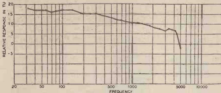
Fig. 2. This pick-up has good bass response though the treble is poorly reproduced.
