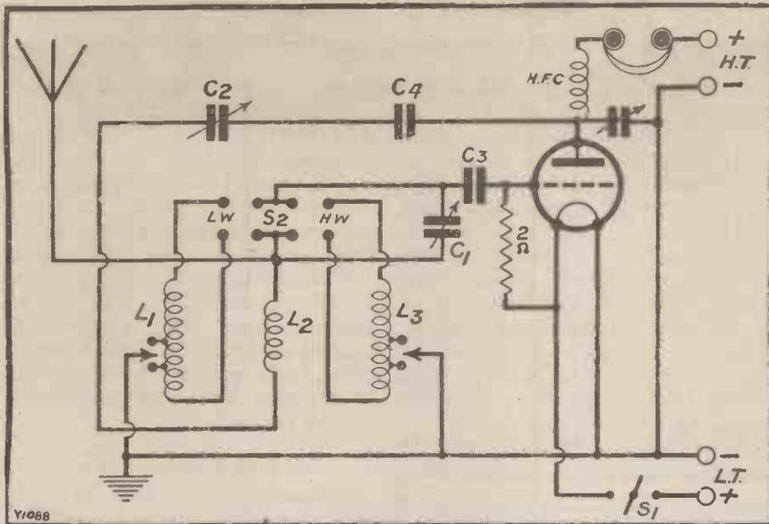
I connected up the aerial and earth leads and also the H.T. and L.T. batteries. In the valve holder I inserted a valve of the D.E.H. type, applying about 70 volts H.T.
