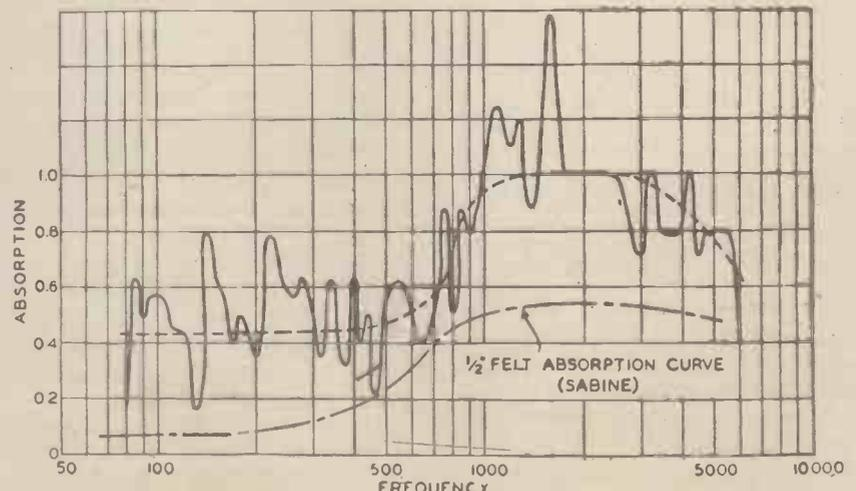
Fig. 8. Absorption-frequency characteristics in felt-lined room.
