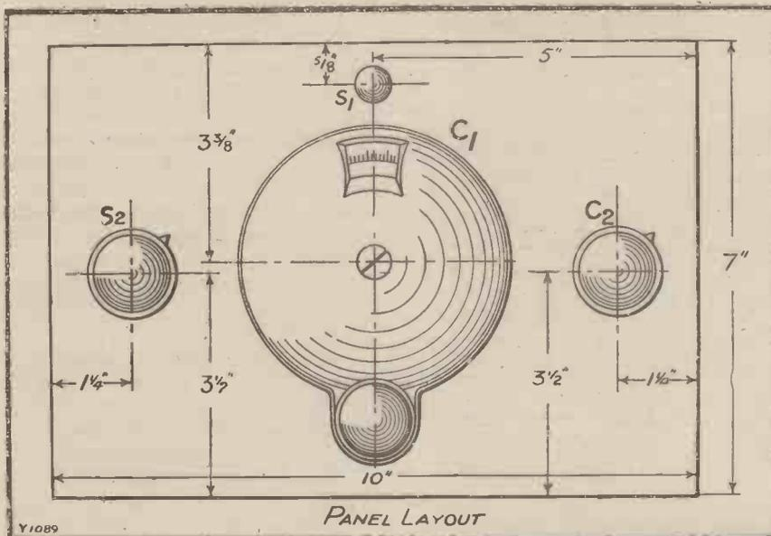
the set, the panel and baseboard layouts are quite straightforward. Drill the panel in accordance with the dimensions given in the diagram, and then place the various components in position on the baseboard. Note very carefully how the three-coil sockets are placed and arrange socket  $L_1$  so that it can be rotated to a certain extent in order to vary the distance between  $L_1$  and  $L_2$ . This is important.
