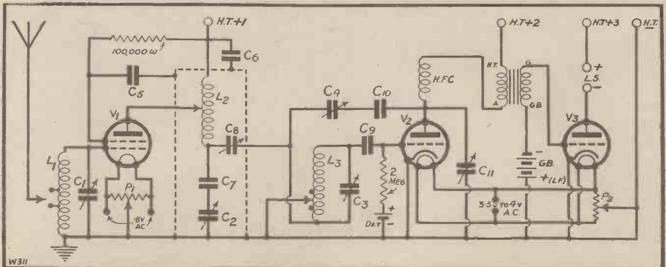
The circuit of the "Brookman's" Three after the various little modifications have been made for the use of A.C. valves.
