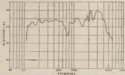
Fig. 4. Response-frequency characteristic of 115-cycle cut-off exponential horn. Measured outdoors on horn axis 2 in. from mouth.
