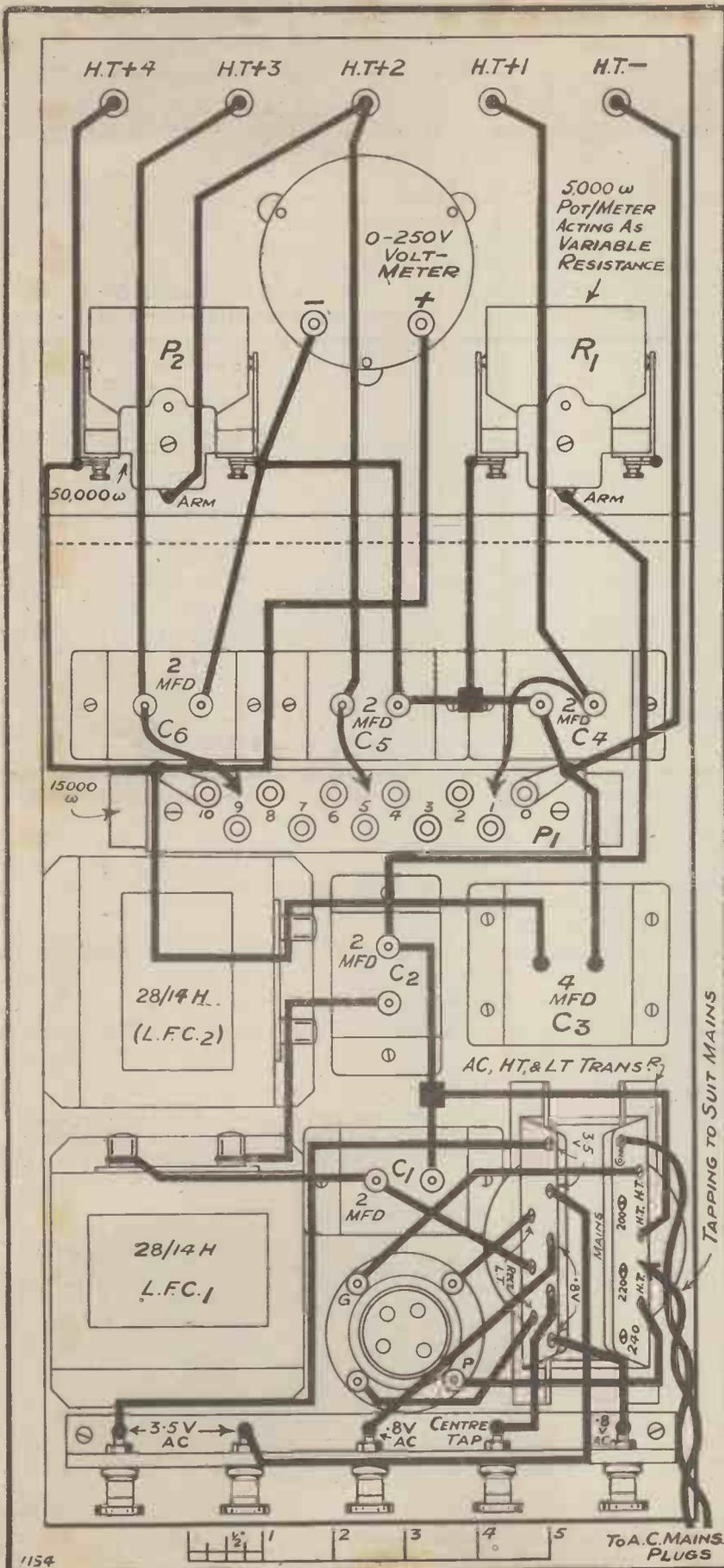
It is usually desirable in such cases to break into the wiring of the receiver and take out a separate H.T. supply lead for the first L.F. valve. This valve should then be run from H.T.+3 on the mains unit, the plug appropriate thereto being placed in the No. 8 or 9 socket of the tapped potential divider.
