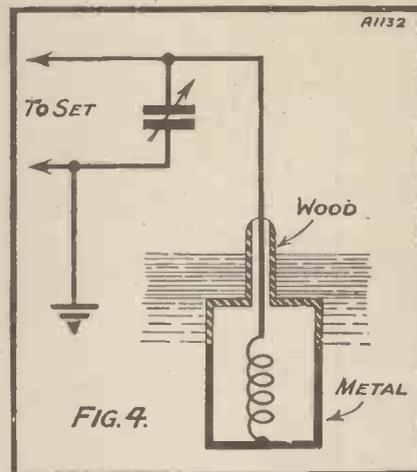
In the centre of the box is a coil wound to dimensions necessary to cover the wave-lengths required. One end of this coil is connected to the metal box. From the other end of the coil a lead runs up through the wooden tube to an ordinary aerial lead-in tube, and so on to the aerial terminal of the set.
