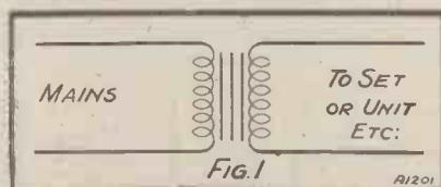
The effective voltage is 70 per cent of the maximum, and it is this that is given as the rating; so do not forget that if you have the A.C. mains you are up against a voltage much greater than that which is inscribed on your electric light bulbs and other devices. This greater voltage will not be taken into account in the ordinary
