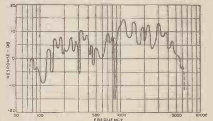
Fig. 5. Response-frequency characteristic of 3 1/2-in. piston-diaphragm loud speaker. Measured 12 ft. from diaphragm in highly absorbing room.
