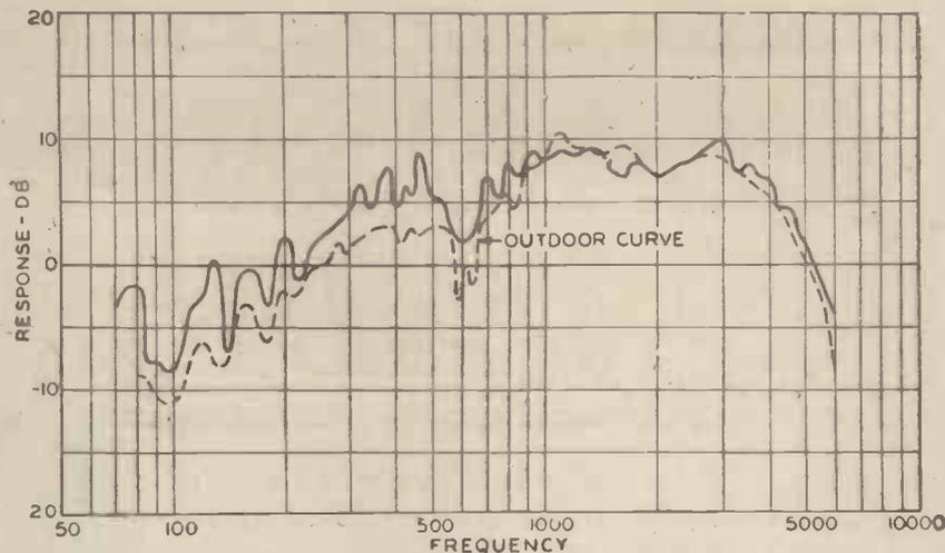
Fig. 7. Response-frequency characteristic of a 3 1/2-in. piston-diaphragm loud speaker. Measured in a highly absorbing room and averaged in small region 12 ft. from diaphragm.
