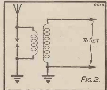
A water-pipe earth is used indoors for stability purposes. If a mains unit of any kind is employed, or the receiver itself is mains driven, the water-pipe connection is unnecessary, as the set will find its stabilising earth in the mains themselves.
