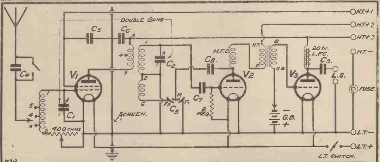
In this circuit diagram you can follow the special arrangements which make the "Eckersley" Three both a high-quality local set and a sensitive long-range outfit. The photo above shows the control for the series condenser C<sub>4</sub>.
