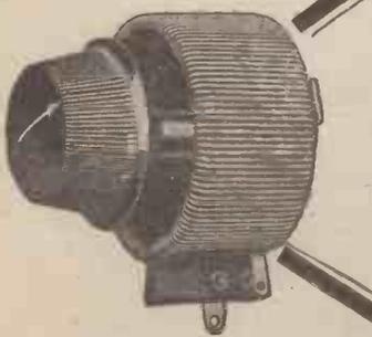
Small in diameter, but large in capacity, this rheostat is constructed of heat-resistant material throughout. The wire is wound on a metal core insulated with asbestos.
