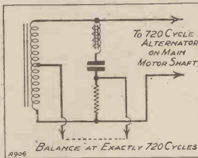
At a frequency of 720, therefore, the voltage across the dotted line shown (that is, between the junction point of the resistance and condenser-choke side, and the centre-point of
