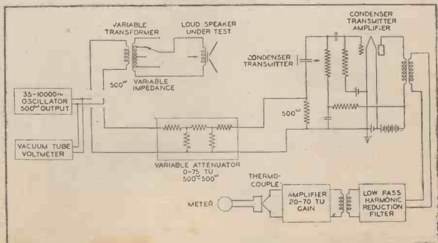
Fig. 1. The circuit of the loud-speaker response-measuring system.
