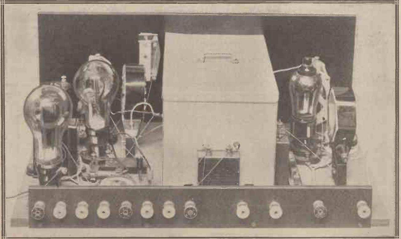
Two extra terminals are required for the 8-volt A.C. supply to the screened-grid-valve filament, and these are mounted just to the left of the earth terminal.
