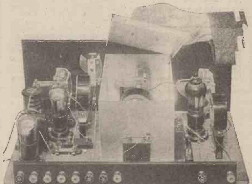
The "Brookman's" Three incorporated a form of band-pass filter in the intervalve coupling circuits. (This set was described in detail in the September issue.)
