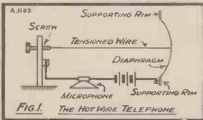
FIG.1. THE HOT WIRE TELEPHONE
