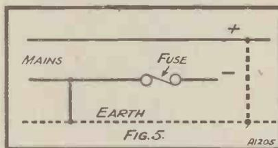
of the mains leads which will blow at nothing greater than, say, a third of an ampere. Do not make the mistake of using only the one fuse. We have said enough about mains, we hope, for you to have firmly grasped the idea that it might so happen that you inserted the fuse in a wire which happened to be grounded. Obviously this would do nothing to prevent damage arising through the other wire short-circuiting to earth.
