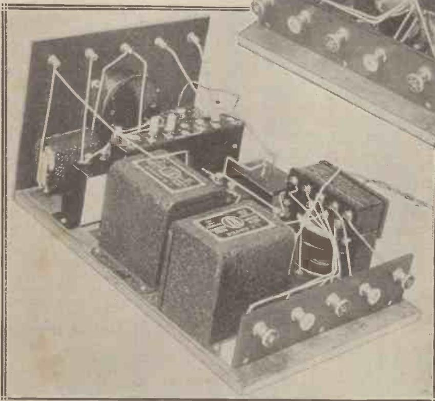
current which becomes the H.T. supply after rectification and smoothing. Both these windings are provided with a centre-tap, that on the filament winding constituting the positive side of the H.T. circuit, and the one on the other forming the negative.
