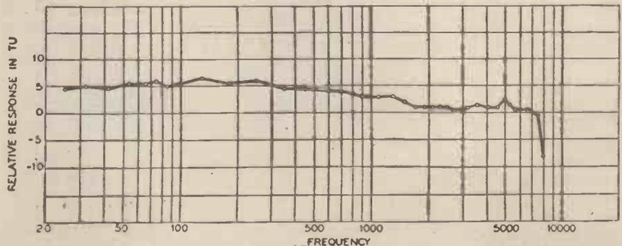
Fig. 3. A curve of a new type of pick-up which has greatly improved high note response.
