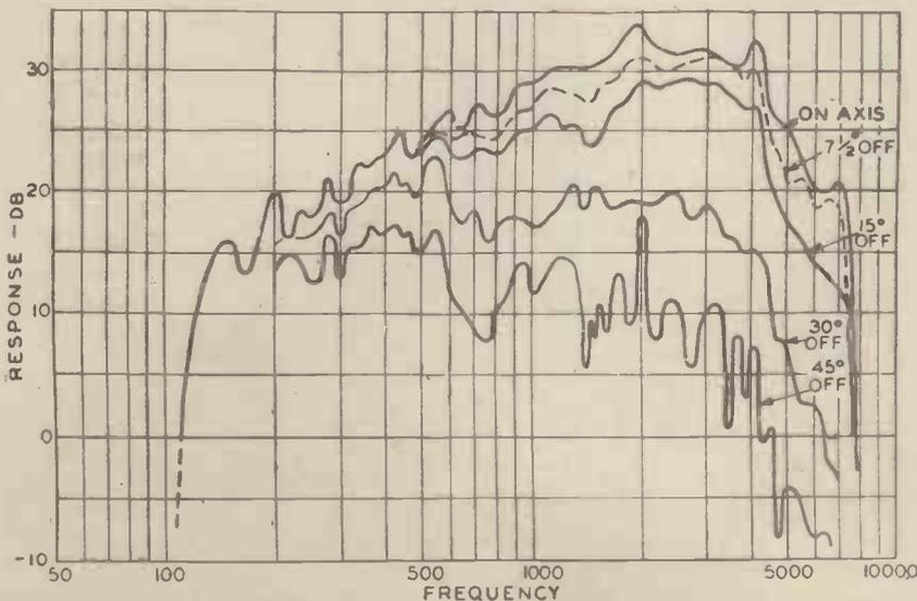
Fig. 2 The response-frequency characteristics of 115-cycle cut-off exponential horn with a moving-coil unit. Measured outdoors 12 ft. from mouth of horn at specified angles to horn axis.
