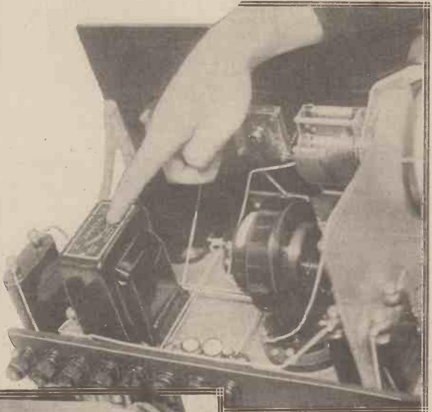
Above, the output filter choke, where low D.C. resistance is to be desired. Below, the "losser" resistance which enables you to flatten out your tuning for the best quality on the local programmes.
