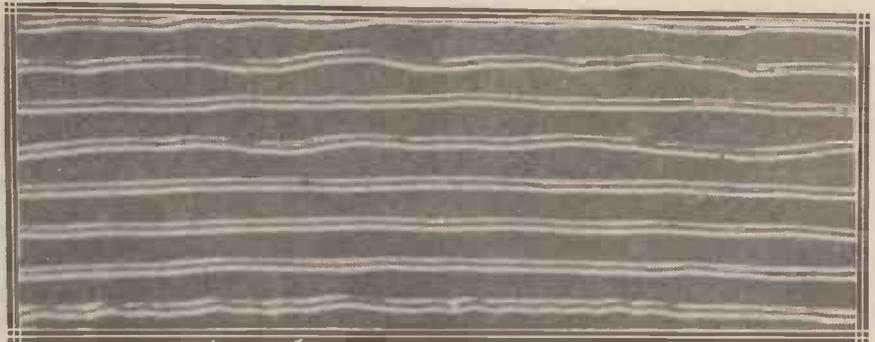
Fig. 4. After 50 times with the Lissen pick-up and a spear-point needle. The grooves show no trace of wear.
