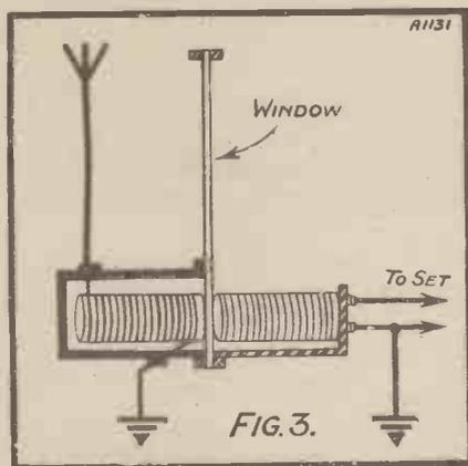
pieces of brass, one pointed, separated from each other only by the thickness of a piece of paper. Enough slack is allowed in the aerial and earth in order to permit the window to be opened.
