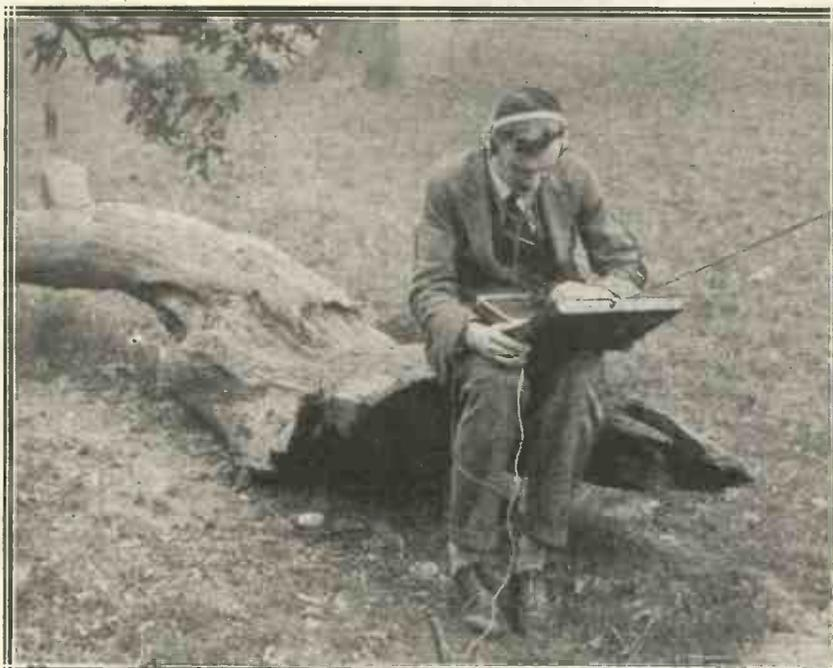
A little portable outfit that employs an improvised extended aerial. Greater selectivity is possible with a frame, although all frame-aerial sets are not necessarily sufficiently selective for modern conditions, as many set-owners have found!
