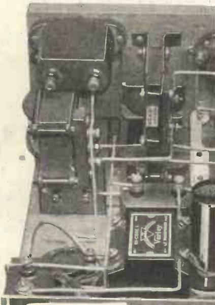
The running costs of a set that derives its power from A.C. mains are generally extremely low, and compare very favourably with those of an equivalent battery-driven receiver. Here is a section of the "Mains-Power" Three, described in the December, 1930, issue of "M.W."
