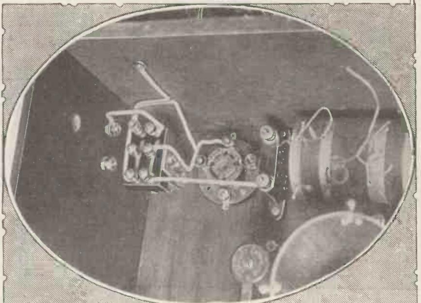
Fig. 4. The next step in the construction deals with the mounting and wiring of the control switch, illustrated above.
