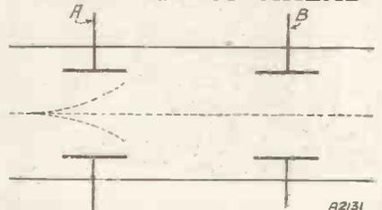
The sets of plates, A and B, are the starting and finishing lines in the high-speed course over which the electrons are timed. and a positive charge on the lower, or else the opposite might be the case
