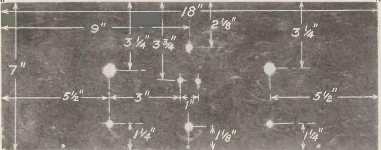
The exact positions of the holes in the panel are shown in the above illustration, which is a photograph of the original
