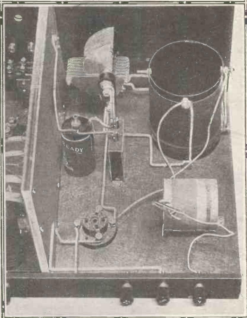
Fig. 3. Only the L.T. positive filament connection remains to be done on the H.F. side.
