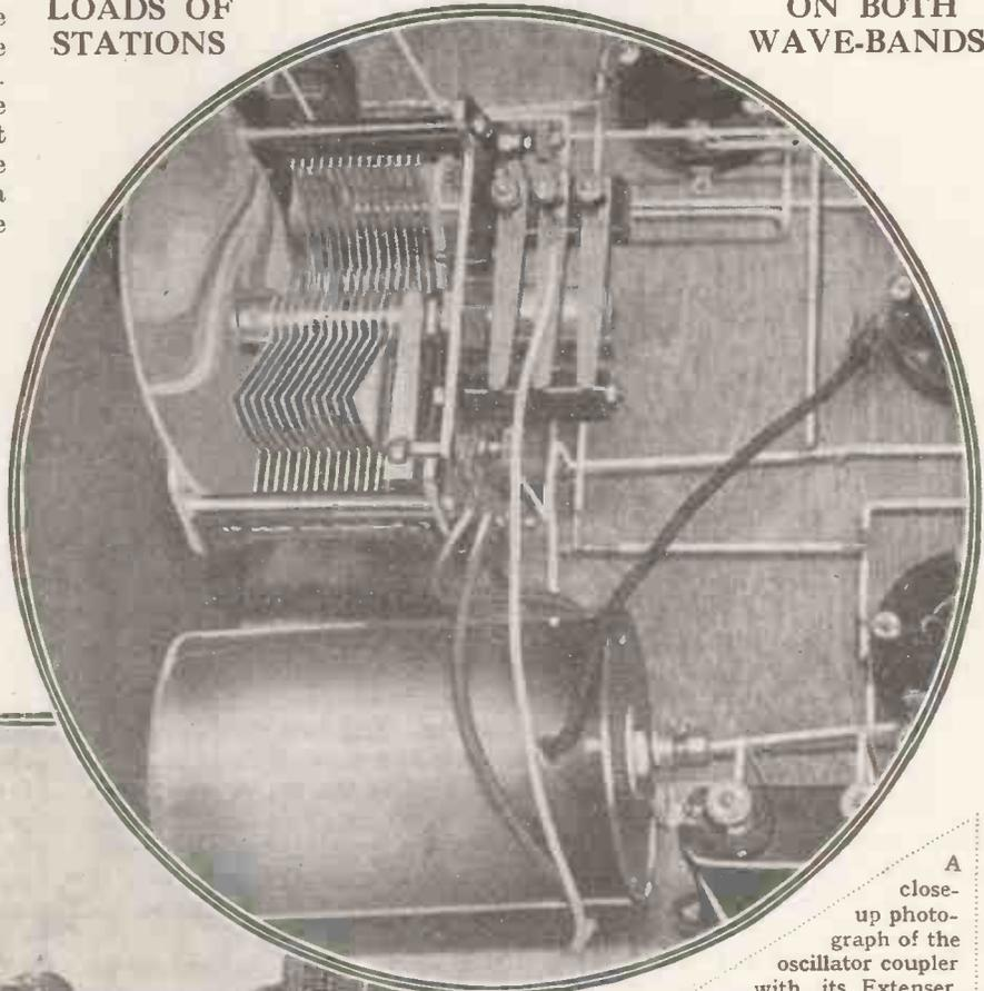
A close-up photograph of the oscillator coupler with its Extenser. Note the self-changer on the shaft end.
