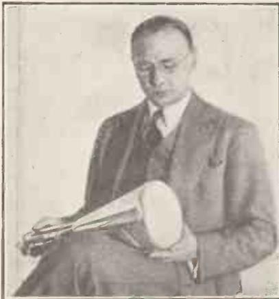
A cathode ray tube, which is really a powerful electron gun. One of these tubes is used in the apparatus described in this article.
