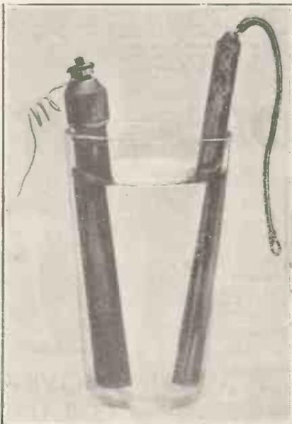
An elementary Léclanché cell formed by zinc and carbon rods immersed in a sal-ammoniac solution.
