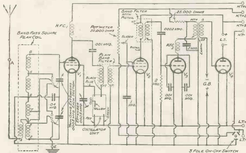
This is the circuit diagram of the “M.W.” “Super-Quad,” the world’s first “Extensered” super-het.
