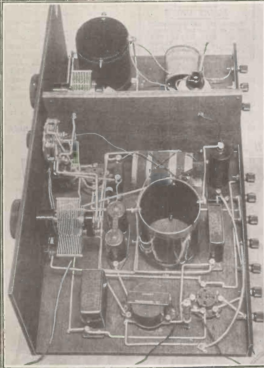
Fig. 10. "The last lap." The final connections have been made, and the wiring is now ready to be checked over before the set is tested.
