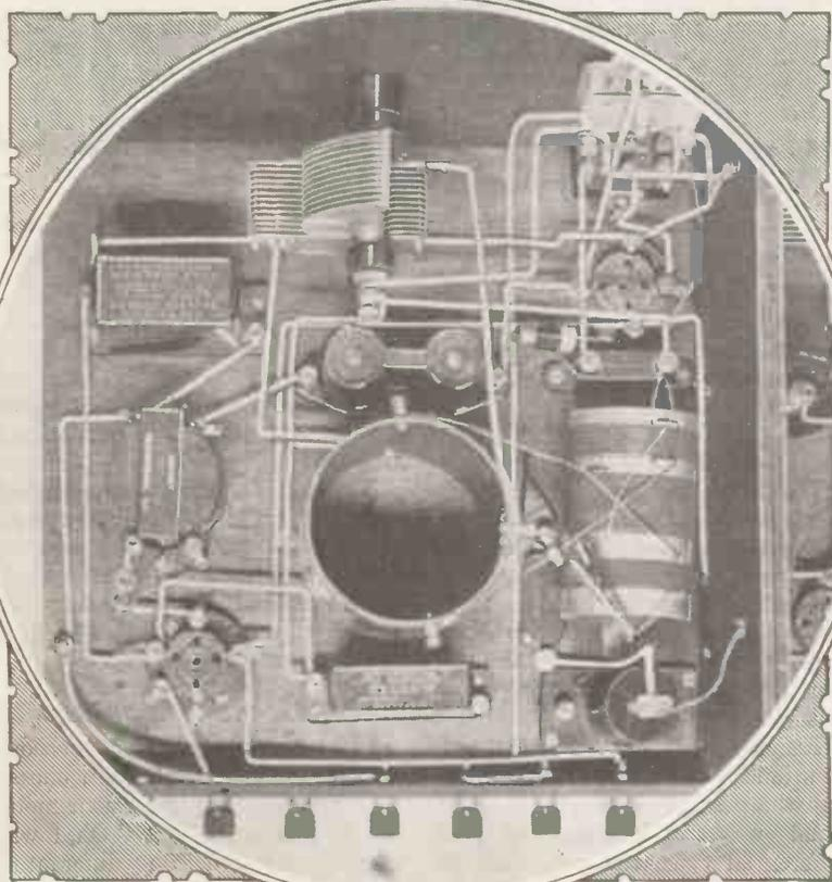
Fig. 9. With the exception of the G.B.—2 lead, the L.F. transformer has been wired up and the L.F. circuit from the detecto valve is now complete.
