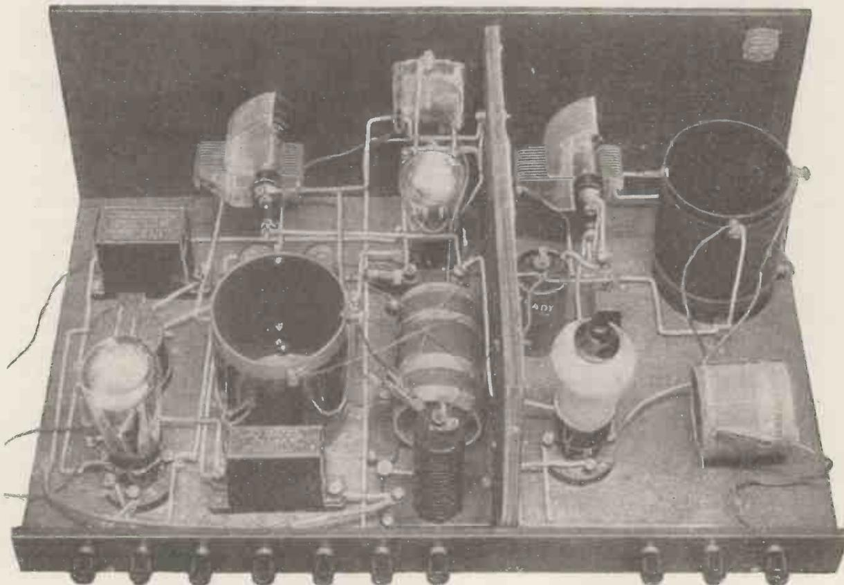
This general view shows the valves in position, the set being ready to connect up to aerial and earth, loud speaker and batteries. Note the metallised screen-grid valve, a feature that is very important.
