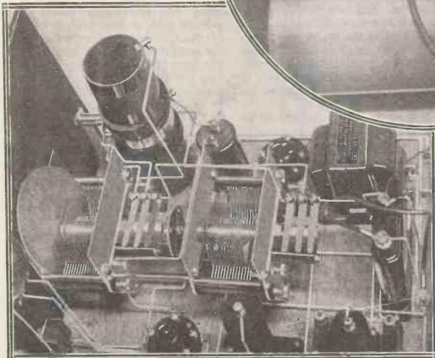
The ganged Extenser eliminates switches and enables the change-over from one band to the other to be carried out automatically.
