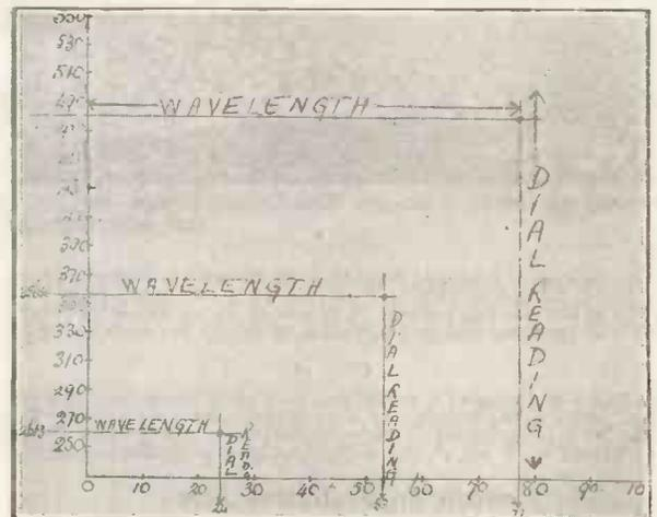
The first stages of a typical tuning-chart, with only three dial readings marked in.
