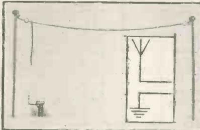
As the wireless waves pass a suspended wire aerial they induce electrical currents in it, just as would a moving magnetic field from a huge coil. This kind of aerial system demands a good contact with the earth—note the earth tube!
