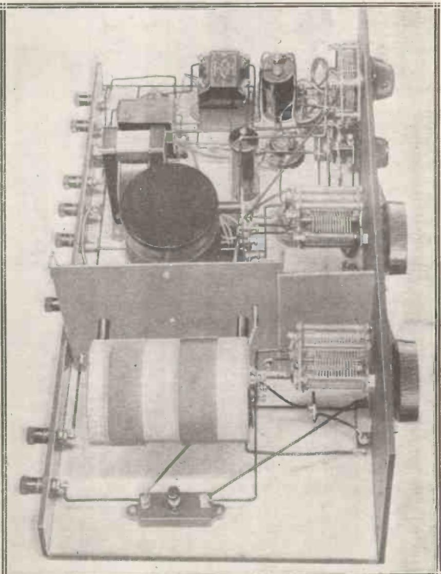
The two coils in the "Eckersley" Tuner are coupled by a resistance so that the tuning of the one does not tend to upset the tuning of the other.
