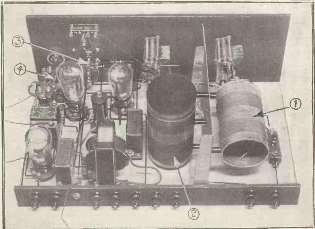
(1) and (2) are the two sections of the "Eckersley" Tuner. Working in conjunction with this at the L.F. end of the set is a special filter, the component parts of which are indicated at (3) and (4); (3) shows the fixed condensers, and (4) the Spaghetti resistances. The tuner and the filter together provide remarkable selectivity, and distant stations come in with extraordinary freedom from "mush."
