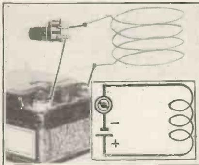
The inductance of a length of wire is considerably increased if the wire is wound into a coil.
