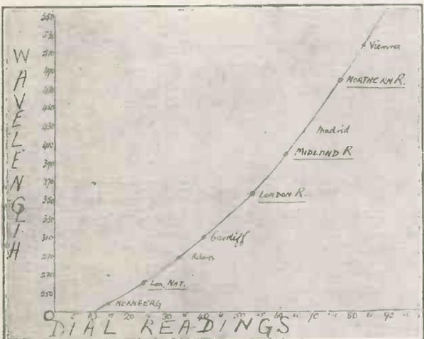
Here some other stations have shown us the general shape of the curve, with dial readings linked to wave-lengths.
