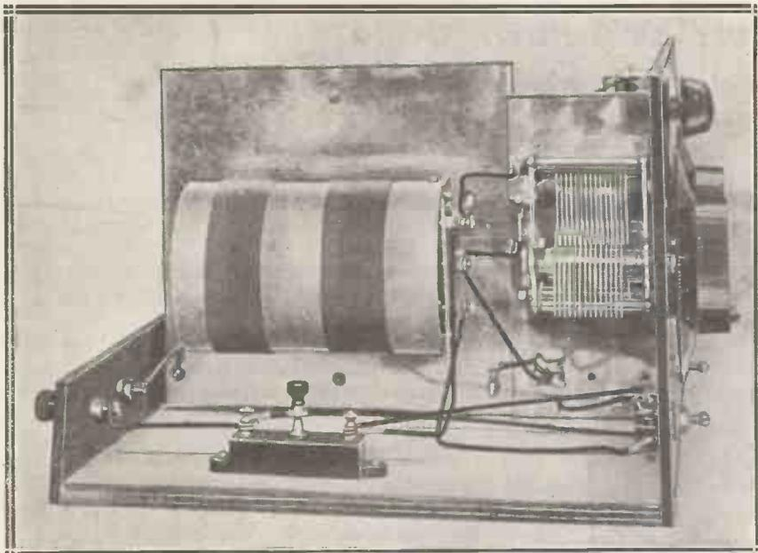
A small series condenser enables the set's aerial circuit to be exactly adjusted whatever the length of aerial used.
