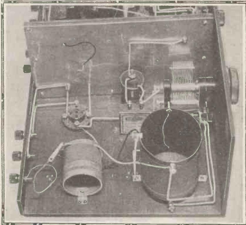
A further view of the H.F. end, showing the aerial tapping clip on the end of the red flex. Note the flex lead for the S.G. valve.
