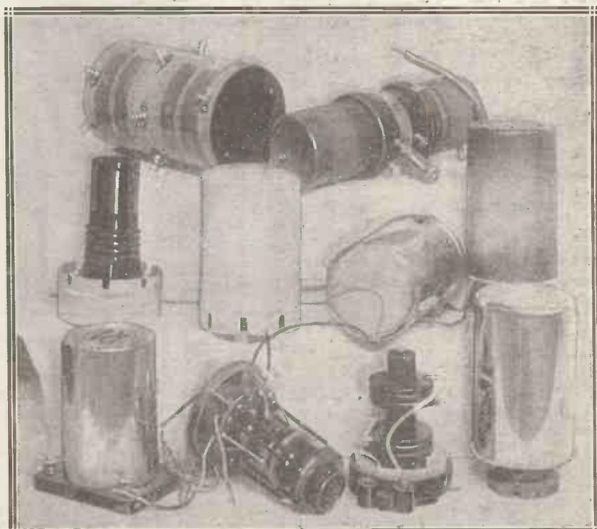
Here are some of the key components used in the "S.Q." series. You will recognise the R.I. Dual Astatic band-pass coil; the Varley Square Peak coil; the R.I. super-het coil; and the Colvern, Lewcos and Wearite intermediates, and oscillator coil units.
