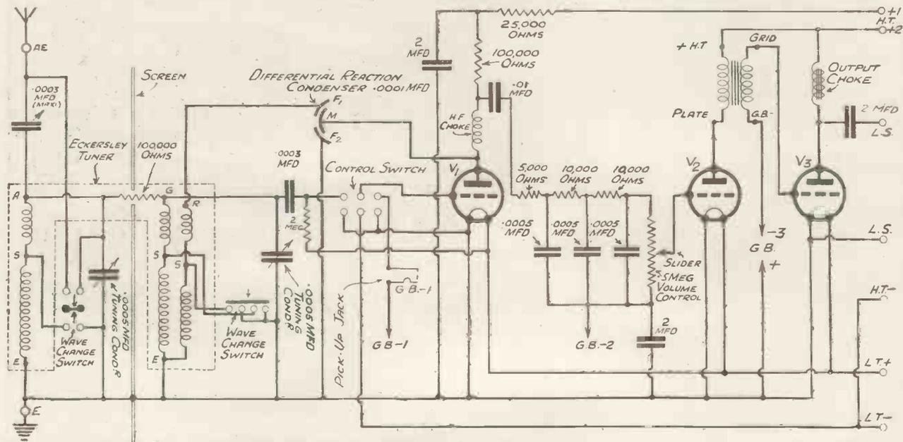
The almost perfect selectivity given by this circuit is due to the separately tuned aerial and grid circuits. All stray coupling effects are entirely absent, the only connection between the two coils being through the special coupling resistance.
