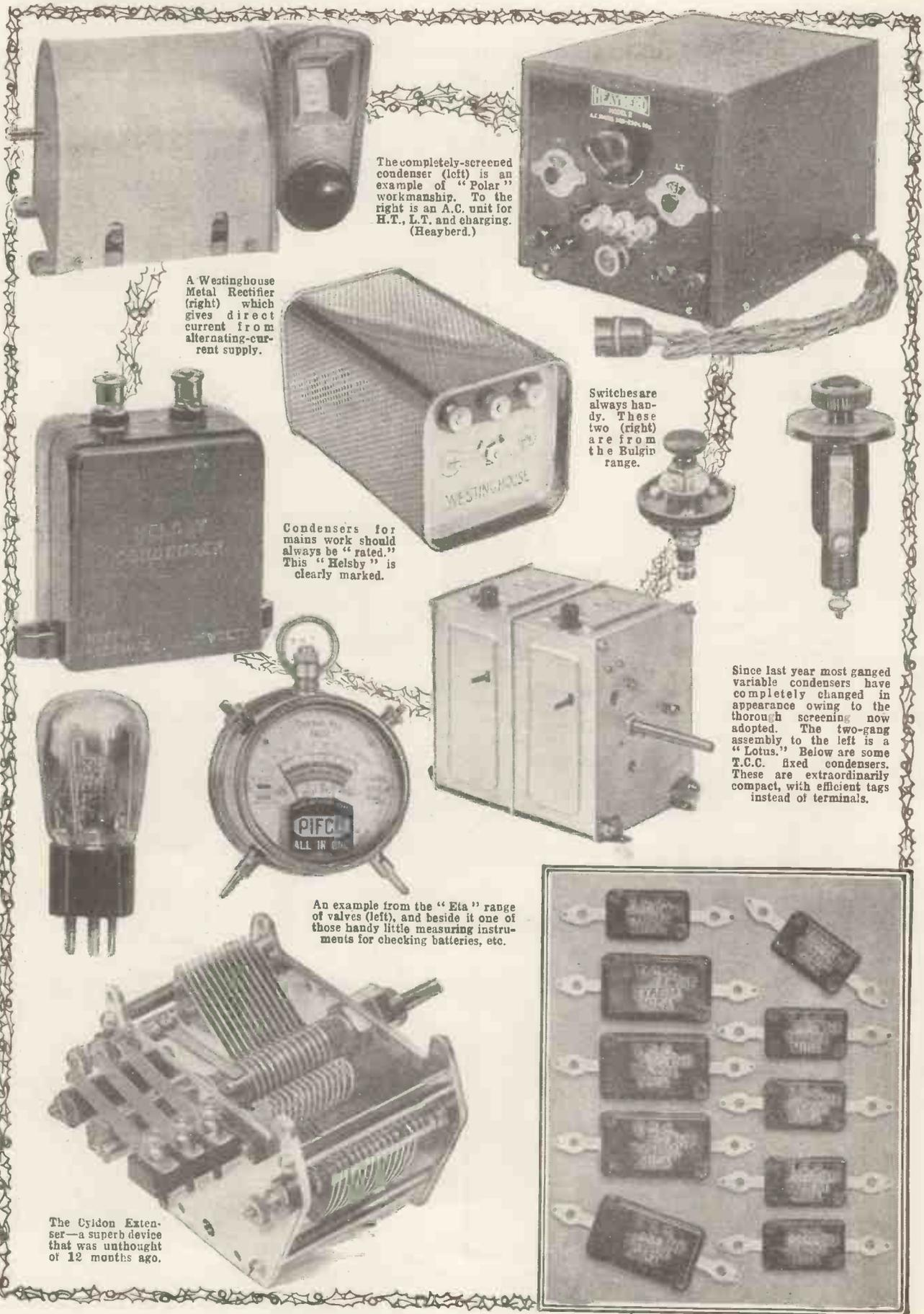
The completely-screened condenser (left) is an example of "Polar" workmanship. To the right is an A.C. unit for H.T., L.T. and charging. (Heayberd.)
