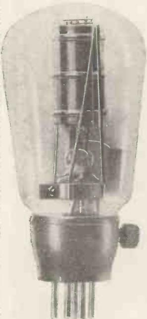
Above is a close-up revealing the structure of the Mazda A.C. Pentode.
