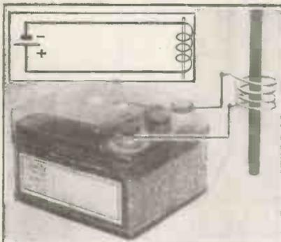
Inserting an iron core increases the inductance still further, for iron is a better conductor of magnetic lines of force than is air, so the iron core tends to cause a concentration of these, and that is the same as saying the intensity of the magnetic field immediately surrounding the coil is increased—which is also equivalent to an increase in inductance.
