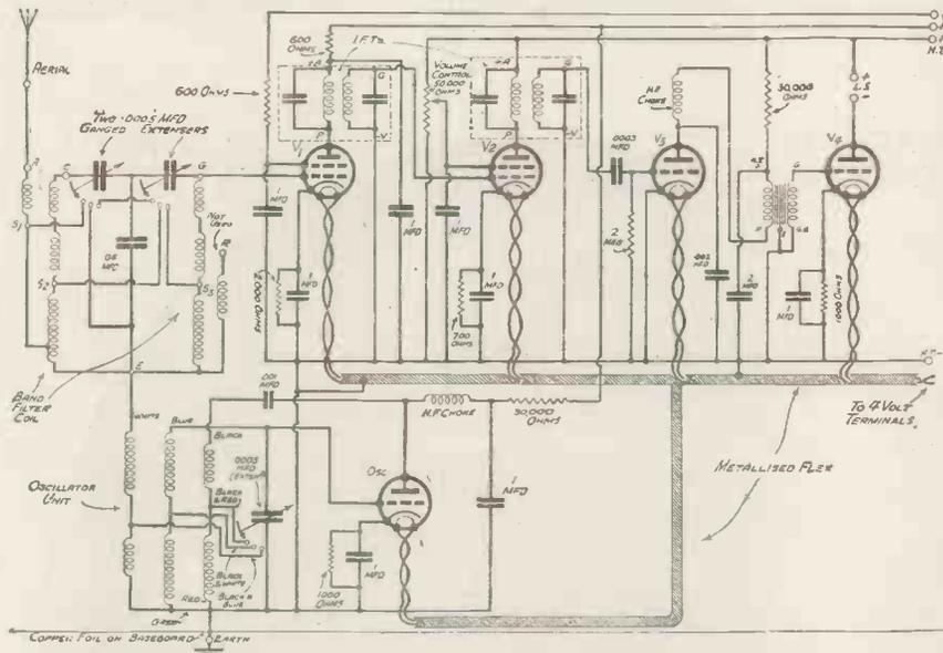
The A.C. version of the "Super-Quad" uses a separate oscillator valve, and is operated from a commercial mains unit.
