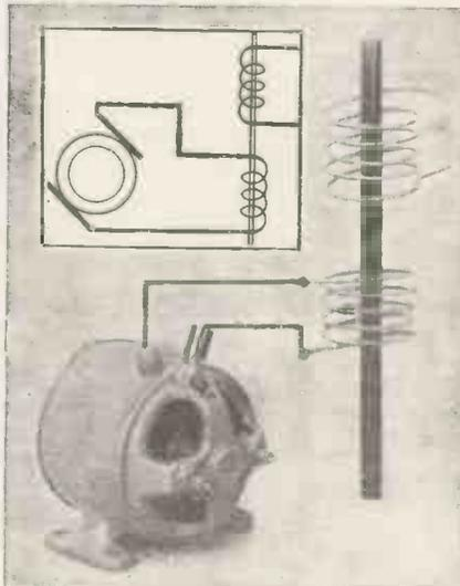
An alternating current dynamo produces current which alternates in its direction of flow and thus causes the magnetic field round the primary winding of the above primitive transformer to fluctuate and induce current in the secondary winding.
