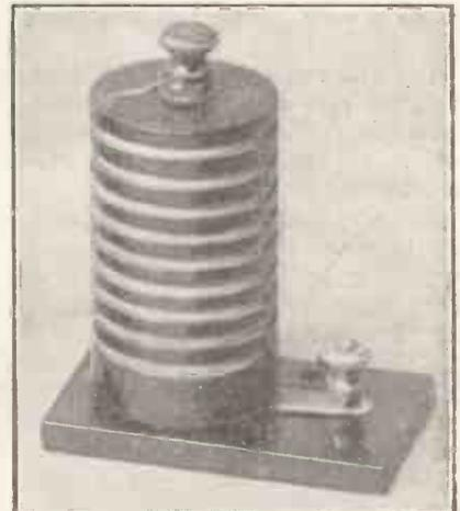
Modern circuits demand very high efficiency in the H.F. choke, and this (Paroussi) is a good example.
