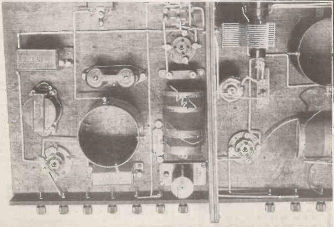
Fig. 5. The wiring is continued in this photograph to its fifth stage, when some of the components on the det. and L.F. side of the screen are connected.
