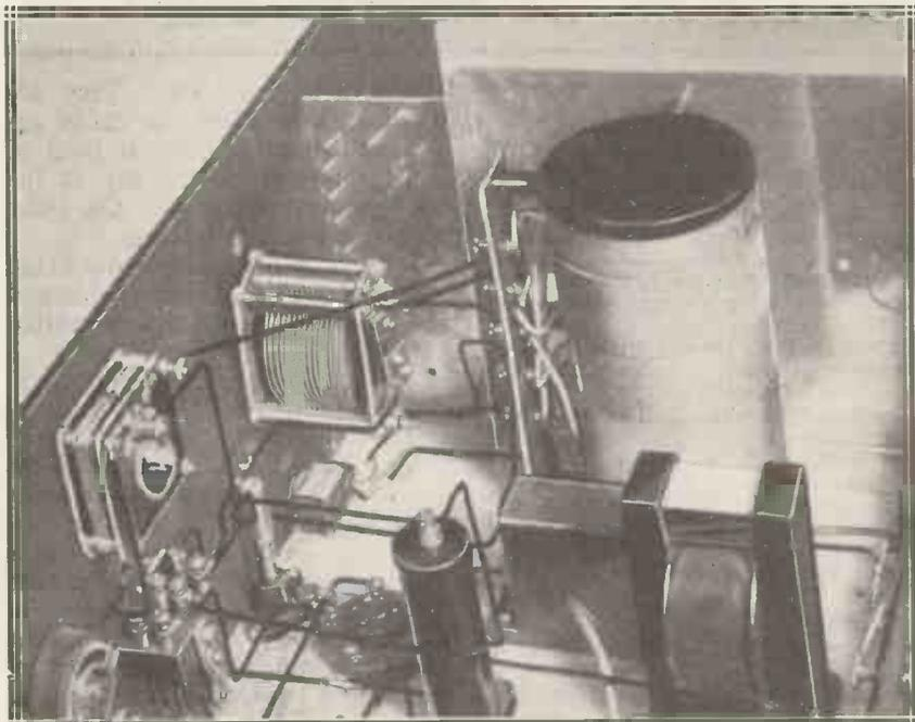
The windings of this coil are arranged so that the reaction is divided into two portions, which are placed at the top and bottom to assist the screen in eliminating capacitive and inductive coupling.
