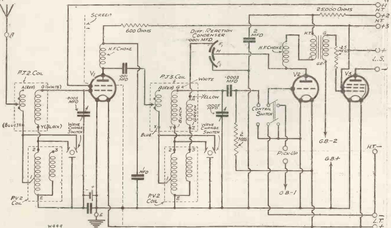
This is the theoretical circuit of the "M.W." Alpha, the pentode output being optional.
