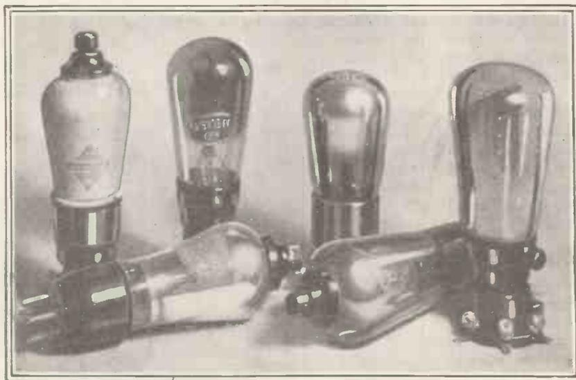
This photograph shows a group of highly efficient 2-volt valves. From left to right we have Cossor S.G., Osram HL2, Mullard P.M.1HL, and Mazda Pen.220, with Marconi and Eta S.G. valves in front.
