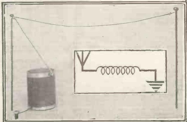
The coil completes the simple aerial circuit.
