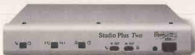
**STUDIO PLUS TWO**—Includes Modem and Printer "Thru" switches so you can keep your normal MIDI setup connected and still print or use your modem. A third switch lets you connect all 6 MIDI OUTs together. LEDs on the front panel display MIDI activity! It has 2 MIDI INs and 6 MIDI OUTs, and is available with cables for the Mac Plus or the Mac 512.
