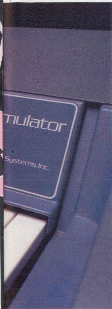
keyboard case (unlike the Fairlight with its four separate units including processing module, "piano" and QWERTY keyboards, and monitor), and despite weighing in at 30kg, the Emulator was the first of its kind: the portable keyboard sampler.
