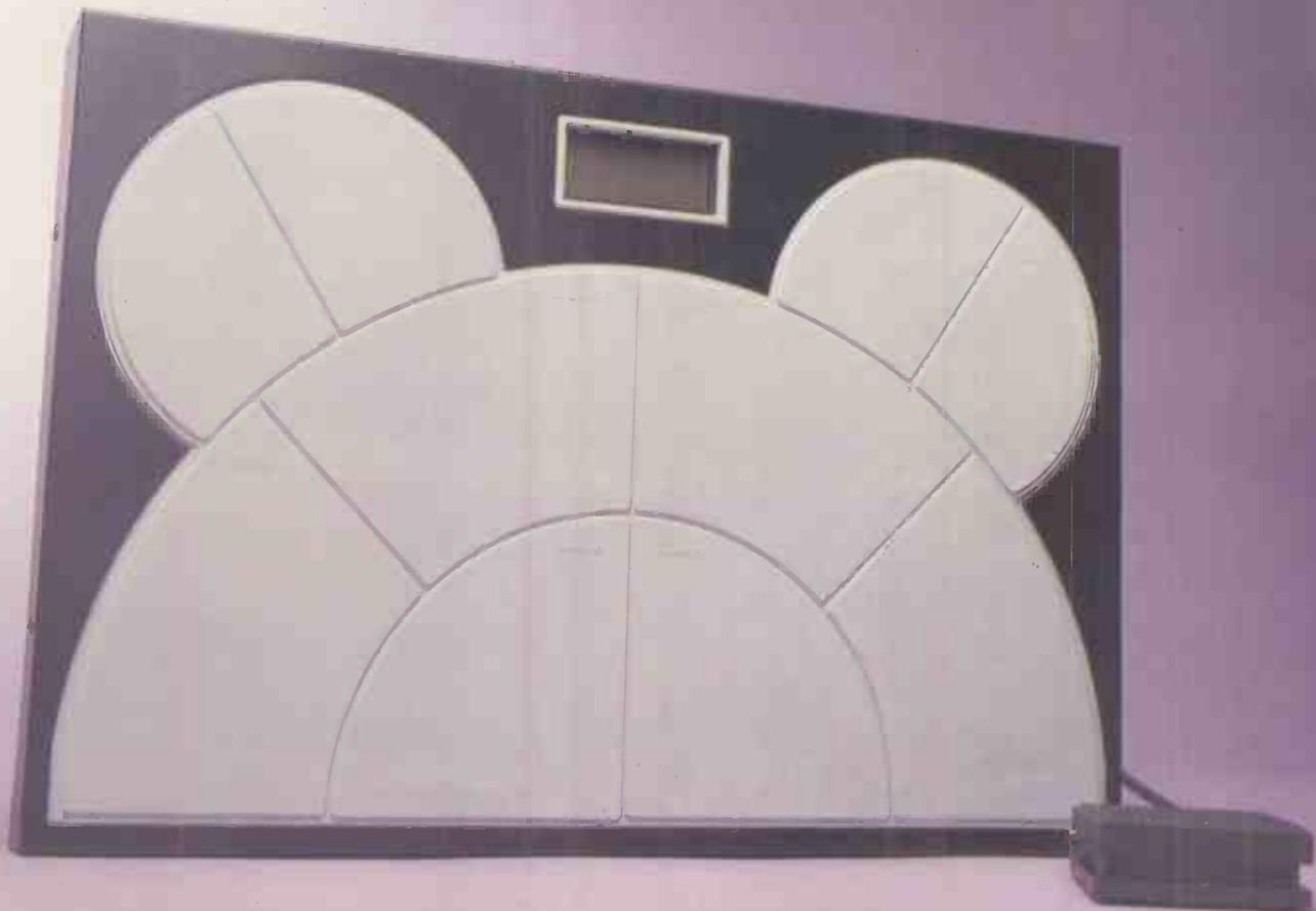
► combine these to form fewer, but larger, playing 'zones'. Much like a MIDI controller keyboard, the drumKat provides no sound of its own, but rather, generates MIDI information which can be used to trigger sounds from any MIDI source, of which the drum machine is only one example. In addition to the onboard pads, it is possible to connect up to nine further drum pads – or bugs attached to drums or other surfaces – and derive MIDI triggers from these.
