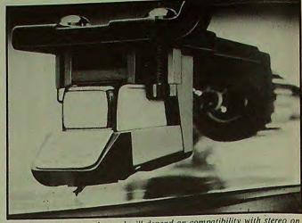
Acceptance of surround sound will depend on compatibility with stereo on discs. Pick-up cartridge by ADC.
