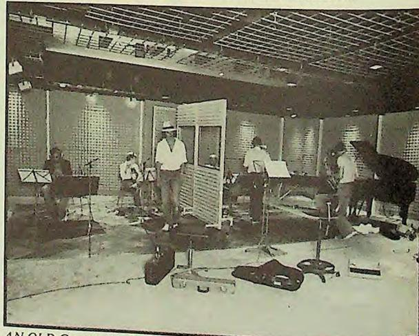
AN OLD Copenhagen warehouse, with the thick walls and 14-inch wooden beams which the builders of 1810 favoured, is now the home of a young recording studio. Sound Track has acoustic design by Eddie Veal, and is of generous proportions — the control room is 40 square meters and the studio is 100. Equipment includes a new Trident TSM 40-in, 32-out console, Lyric 24-track machine, and four JBL 4350s for monitoring. The
