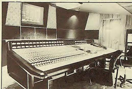
PICTURED ABOVE is the recently re-furbished re-mix room at Utopia Studios. It features 48 channel Series 6000 SSL with total recall, enabling post-production video, as well as music mixing, plus a Sony 50-inch screen projection TV.
