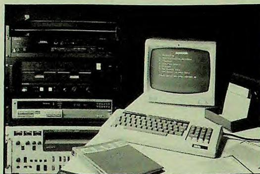
**CLUE**: A computer logging and editing system — is a package designed and developed by HHB that allows Sony's low-cost processors to be used as effective, professional mastering systems.
