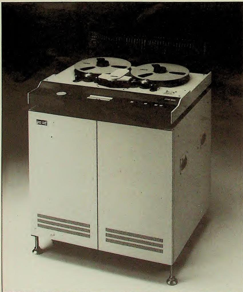
OTARI'S 32-track DTR-900 PD format recorder: about 10 PD multitracks are currently in use in the UK.
