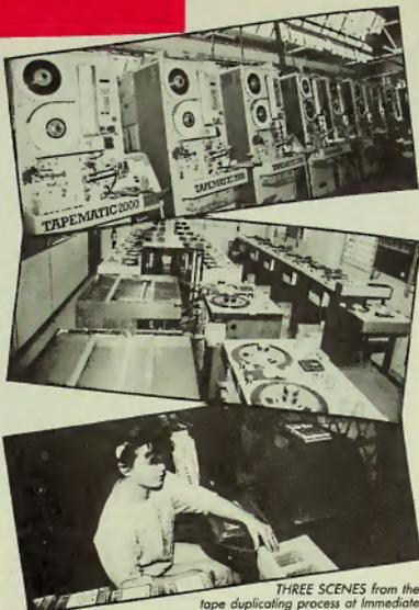
THREE SCENES from the tape duplicating process of Immediate Sound Services: the eight Tapematic loaders (high-speed cutting and winding machines); the fully-equipped duplicating room comprising Gauss Tapematic machines; and the in-house packaging department which offers a very wide service to its customers, especially with children's story tapes packaged with books.
