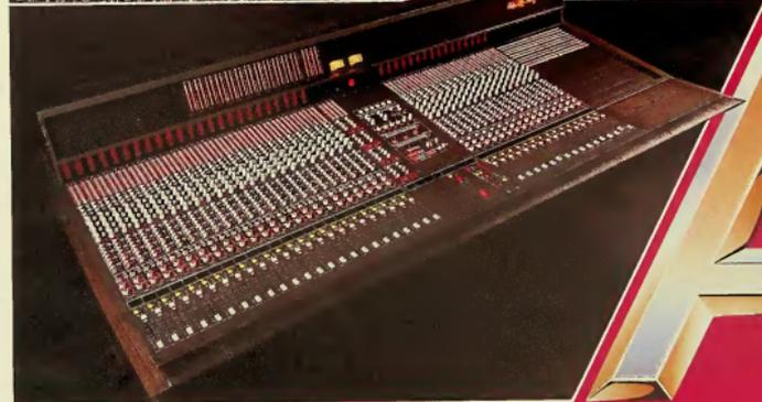
AMEK G2520 uses an advanced dual-signal path i/o module with phenomenal signal flow permutations. 40 and 56 input chassis are currently offered, with 24- or 48-track monitoring options in some versions. Master Status switching, 8 auxiliary sends, parametric equalization, correctly-designed balanced bussing, VCA faders equipped with digital subgrouping, and plasma meters are standard equipment. The Audio Kinetics 'Mastermix' computer can be directly interfaced.
