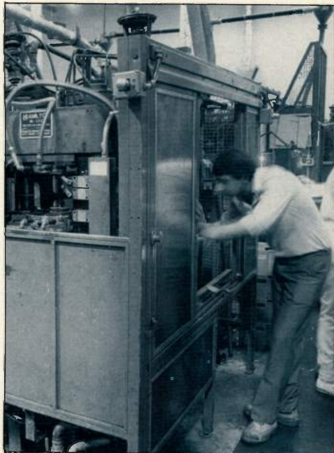
AUTOMATIC moulding presses can produce one 12 inch record every 22 seconds.
