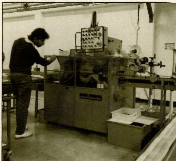
CBS PLANT: The Ilseman K7M4 machine puts inlays, library cases and cassettes together
