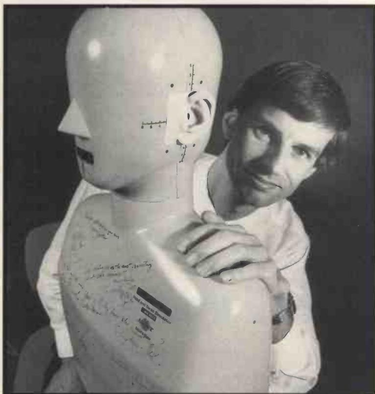
Thorn EMI's new 3-D sound system Sensaura records artists using an artificial human head and torso wired up with microphones. The dummy – pictured with product manager Richard Clemow – is then placed in a studio or live venue. Recordings can be made on any format and played on an ordinary stereo system.
