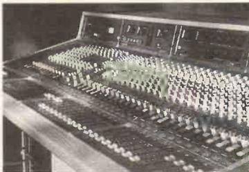
Singapore Broadcasting Corporation has taken delivery of a Producer console from Clyde Electronics via local agent Electro-Acoustics Systems Pte. Ltd. Configured as a 32/8/2, it has 26 mono inputs and six stereo with four stereo groups (with mono derived outputs) and independently controllable mono and stereo main outputs. Metering is PPM throughout with the addition of a phase correlation meter. The producer was custom designed
