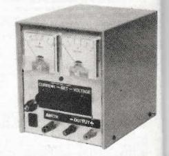
A superb design giving 0-25V and 0-2.5A. Twin par meters indicate Voltage and Current. Voltage is ve able from zero to 25V. Current-Limit control allows Constant Current cha-ing of NICAD batteries, and protects circuits from ovi load. A Toroidal transformer MOSFET power outp device, and Quad op-amp IC design give excellent pe formance formance
