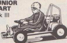
Assembled or DIY kit. New Honda 4-stroke, 144cc, automatic clutch, disc brake. Max speed 30 mph with lock to limit speed to any desired intermediate. Uses 2 star fuel. Safe, sturdy, good ground clearance. Build confidence & awareness for the driver of the future. Adjustable for 6 year old to adult size. 6 months parts & labour guarantee. SEND LARGE SAE FOR COLOUR LEAFLET TO:
