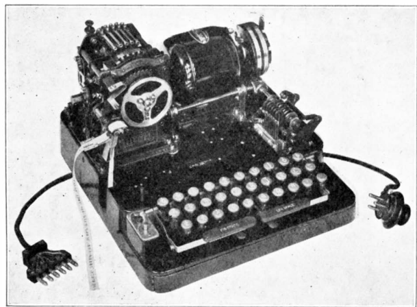
FIG. 2.—MORKRUM TELETYPE NO. 1A, WITH COVER OFF.
