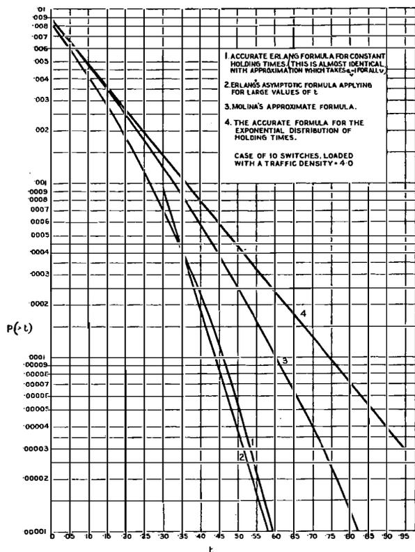
FIG. 2.—CURVES SHOWING THE PROBABILITIES FOR DELAYS, EXCEEDING VARIOUS SPECIFIED TIMES.
