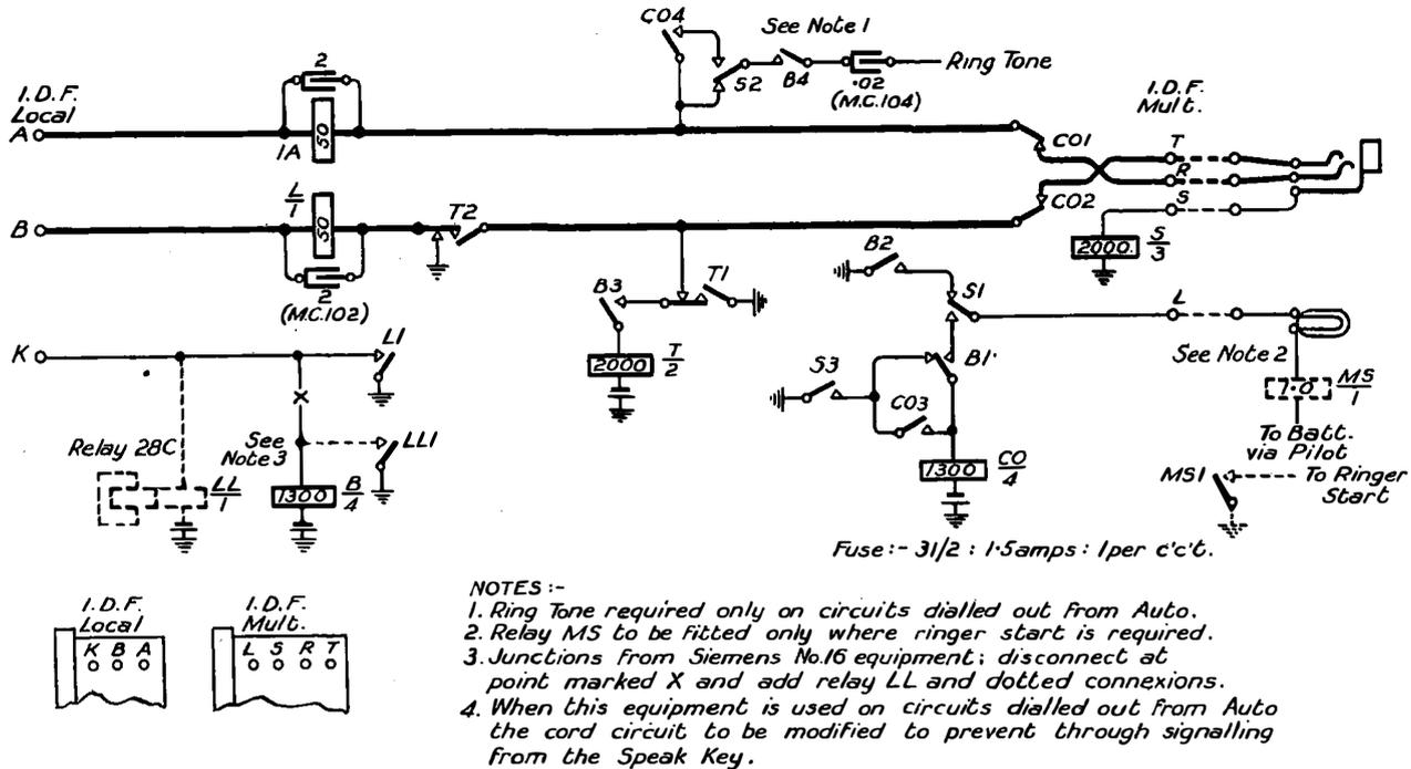
FIG. 2.—JACK-ENDED JUNCTION CIRCUIT WITH CALLING SIGNAL ARRANGED FOR FOLLOWING-ON CALL.
