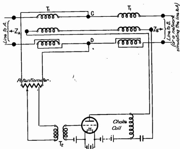
FIG. 48.—PRINCIPLE OF TWO-WAY ONE-ELEMENT "REPEATER" (2-1 TYPE).
