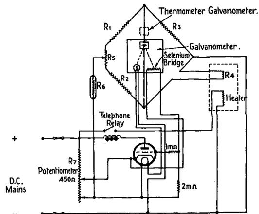
FIG. 2.—CONNEXIONS OF THERMOSTAT WORKED FROM D.C. MAINS.
