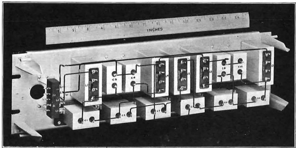
FIG. 4.—RECEIVING-END FILTER.
