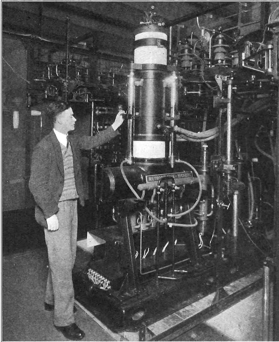
FIG. 1.—500 KILOWATT DEMOUNTABLE VALVE.
