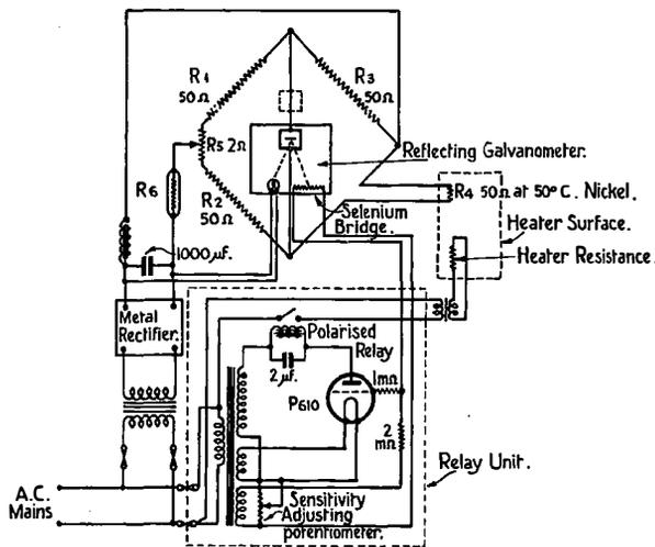
FIG. 1.—CONNEXIONS OF THERMOSTAT WORKED FROM A.C. MAINS.
