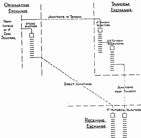
FIG. 4.—APPARATUS REQUIRED FOR DIRECT AND TANDEM-ROUTED TRAFFIC.
