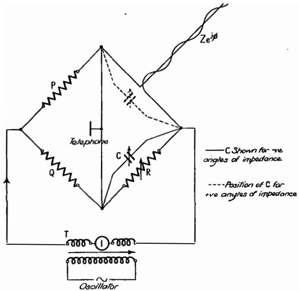
FIG. 52.—A.C. BRIDGE FOR LINE IMPEDANCE MEASUREMENT.
