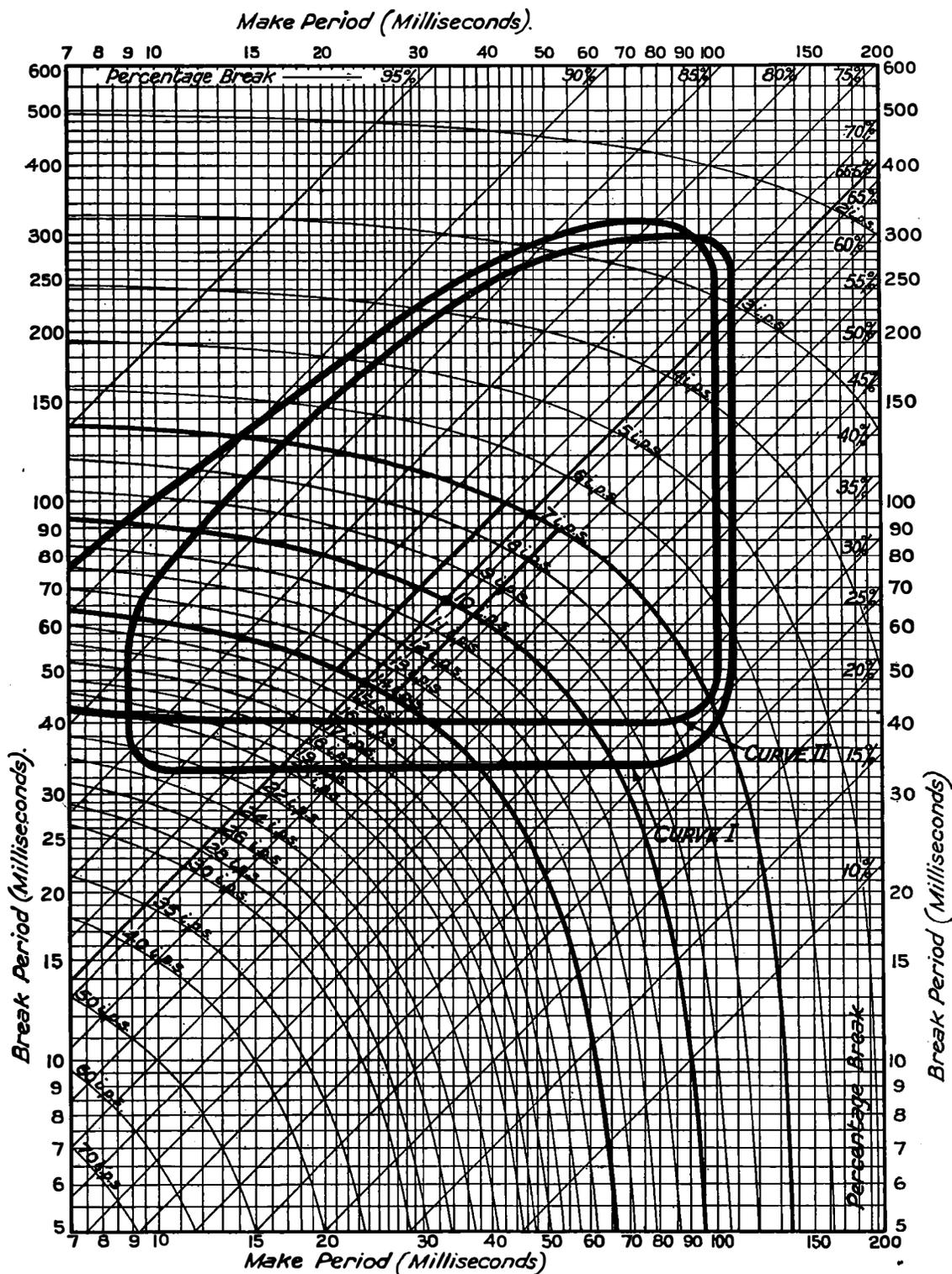
CURVE I . Line Resistance 1800.Ω, Leak ∞, 46 Volts.
