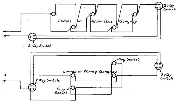
FIG. 10.—WIRING OF GROUP OF THREE PARALLEL SUITES.
