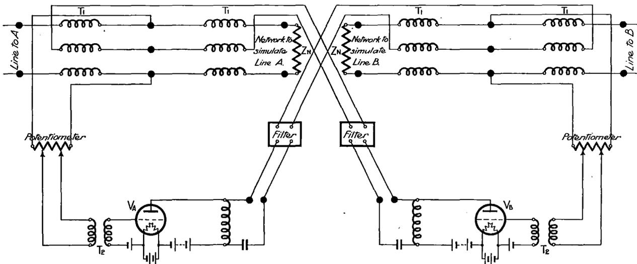
FIG. 49.—PRINCIPLE OF TWO-WAY TWO-ELEMENT "REPEATER" (2-2 TYPE).
