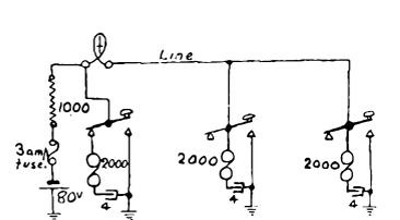
(b). The coils of sounders used for secondary cell working are of 1,000 ohms resistance and are shunted by 9,000 ohms, giving a joint resistance of 900 ohms. They are operated from the 24-volt battery and have a figure of merit of 11 mA.
