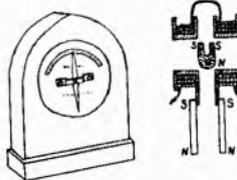
also carries the pointer which moves over a centre-zero scale graduated in degrees. The coils, needle, and magnets are enclosed in a wooden case; the coils are terminated upon four connexion screws fitted on the back of the case. A circular glass cover protects the pointer and scale from damage.
