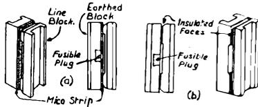
The 2-unit protector (sketch b) consists of two blocks of moulded carbon having flat active surfaces which are sprayed with a fusible gum varnish. The carbon blocks are coated at each end with a thin layer of insulating varnish which dries nail hard and is non-hygroscopic. The air gap is 3 to 6 mils and the break down voltage 500 to 750 volts D.C.
