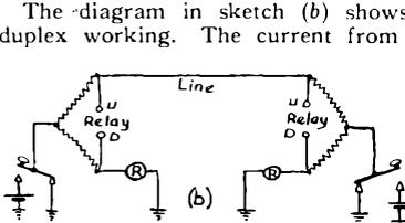
To obtain a resistance balance on a double current duplex circuit, the 40-ohm arm of the rheostat is reduced to zero and the 400-ohm arm set to any value in excess of the resistance of the circuit. The key is then depressed and the galvanometer deflection observed. The 400-ohm arm is reduced step by step until the depression of the key gives a deflection in the opposite direction to that previously observed. The 40-ohm arm is then increased step by step until balance is obtained.
