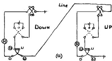
When one key is depressed while the other is at rest, the reversal of the battery causes the line current to fall to zero, because the batteries at each end now oppose one another through the line. The effect of the current in the compensation circuit is to record a space at one end and a mark at the other.
