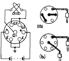
To make a sectional localization of an earth fault on a single-wire telegraph circuit, the furthest testing point, at which the circuit is led in for testing, is asked to disconnect the circuit. The line is then tested and, if proved clear, the testing point is asked to restore the circuit and the penultimate testing point is asked to disconnect the circuit.
