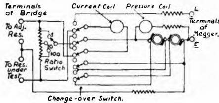
the switch to "megger." The handle is turned until the clutch is felt to slip, when the value of the insulation resistance is measured directly from the scale.
