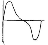
The oscillogram required is shown in the sketch. Any complex wave form can be resolved into a fundamental wave and a number of harmonic waves of increasing frequency. For the faithful reproduction of a complex speech wave, it is necessary that the fundamental and harmonics comprising the wave shall be transmitted without distortion either in phase or amplitude.
