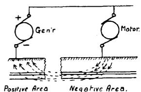
It is in positive areas that electrolytic damage occurs to cable sheaths; the current leaving the sheath sets up electrolytic action which causes the lead composing the cable sheath to be decomposed and deposited in the surrounding earth.
