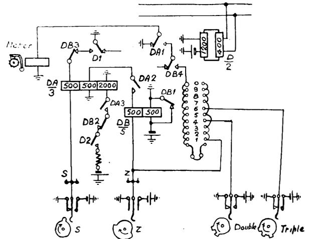
and 0 are used for single metering, level 4 for double metering and level 6 for triple metering. Thus calls to the second unit fee area are routed over level 4 and calls to the third unit fee area over level 6.
