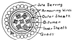
ound. The cable is served with jute to form a bedding for 25 No. 4 S.W.G. and 3 No. 12 S.W.G. stranded armouring wires. A jute serving overall completes the cable.
