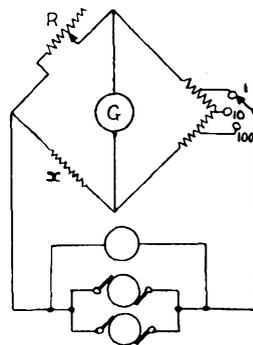
With the change-over switch at "bridge," the ratio switch is brought into circuit and the two 125-volt generators are connected in parallel. Four terminals at the back of the instrument are used, two being connected to the resistance under test and two to an adjustable resistance. The connexions in these conditions are shown in the sketch. The pressure coil is used as the control coil and holds the needle
