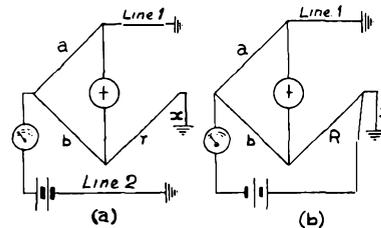
Pomeroy's test for the resistance of an earth connexion is shown in sketches (a) and (b). In the first test, two lines earthed at the distant end are connected as shown. It is necessary that the value of the current flowing at
