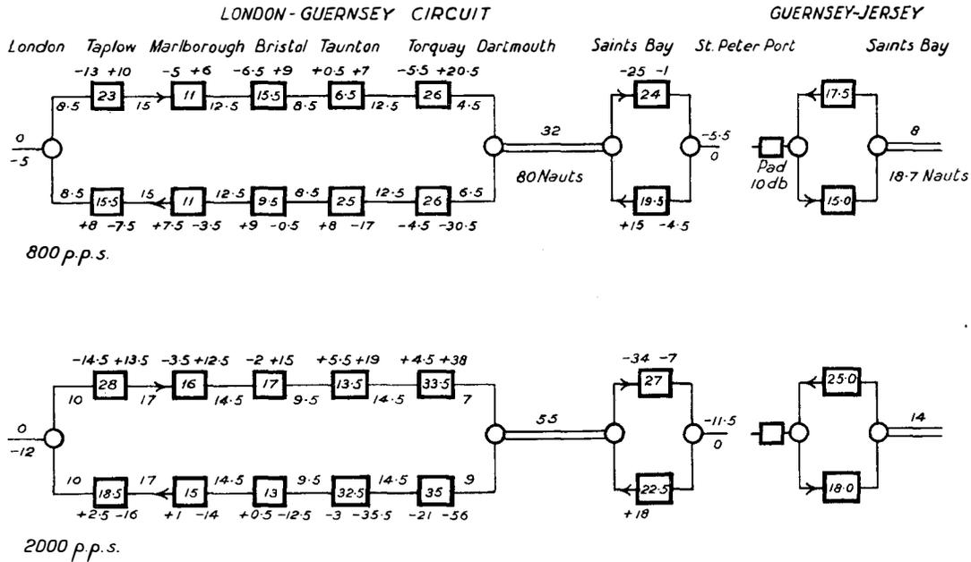
FIG. 4.—ATTENUATIONS AND LEVELS AT 800 P.P.S. AND 2,000 P.P.S.
