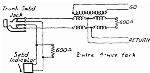
FIG. 1.—600-OHM CIRCUIT TERMINATION.
