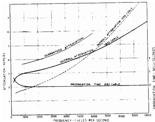
FIG. 10.—ATTENUATION AND PROPAGATION TIME FOR OVERALL LENGTH.
