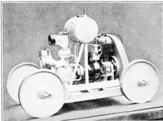
FIG. 2.—PUMP WITH WHEELS AND AXLES IN POSITION.
