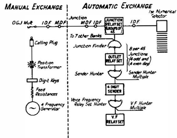
FIG. 4.—FOUR-DIGIT A.C. KEYSENDING OVER STRAIGHT-FORWARD JUNCTION SYSTEM.
