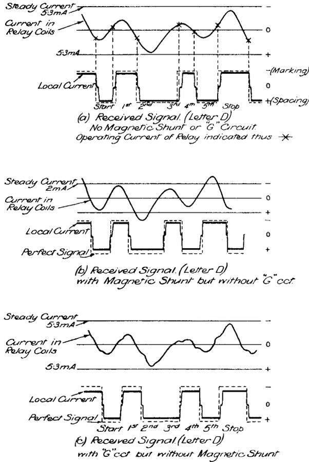
FIG. 5.—OPERATION OF RECEIVING RELAY FOR DISTORTED TELEPRINTER SIGNALS.
