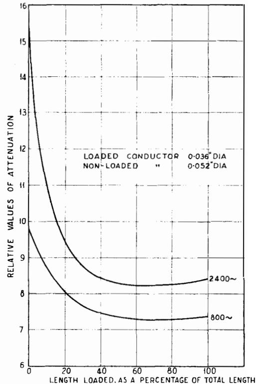
FIG. 5.—VARIATION OF ATTENUATION WITH PERCENTAGE OF LOADING.
