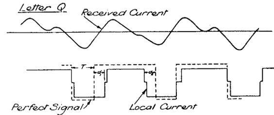
FIG. 6.—EXAMPLE OF BADLY DISTORTED TELEPRINTER SIGNALS.
