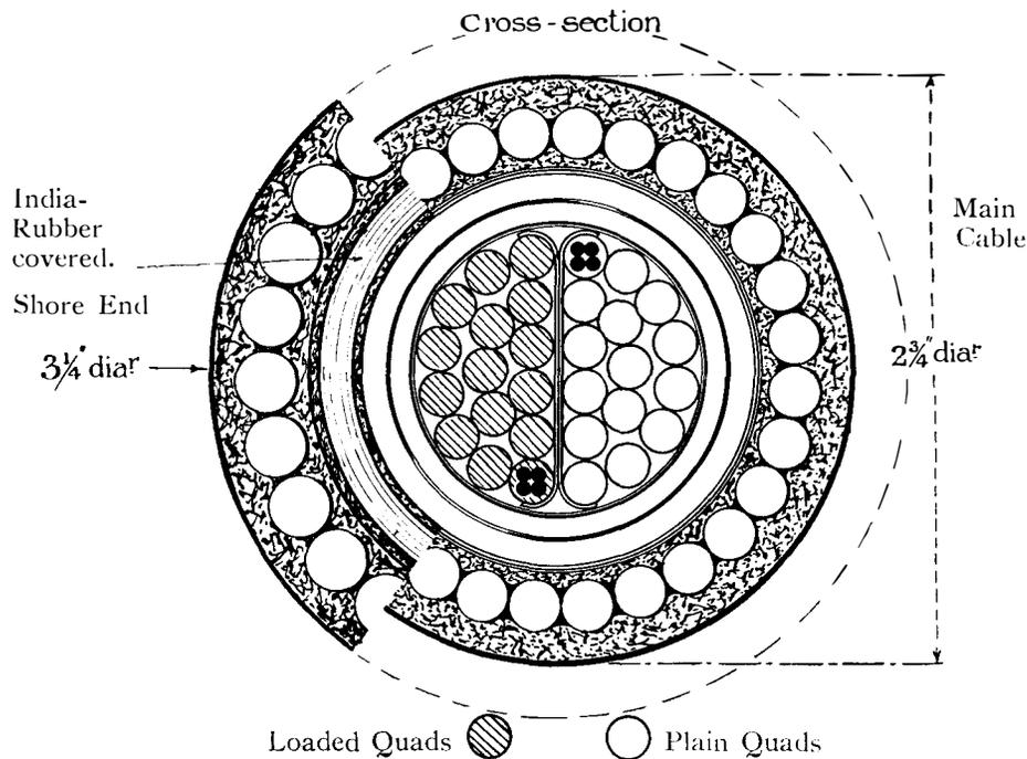
FIG. 7.—CROSS-SECTION OF MAIN CABLE AND ENGLISH SHORE-END.
