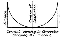
flows in the skin or, at least, penetrates only a small distance, it is usual to employ copper tube, strip or stranded wire, thus increasing the percentage of the copper cross-section carrying current. Stranded wire or litzendraht consists of a large number of strands of fine wire 30-38 s.w.g. frequently stranded  $3 \times 3 \times 3$ , each strand being enamel and silk insulated.
