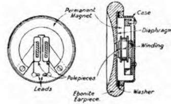
The diaphragm is being continuously pulled towards the pole faces by the permanent magnet, but if an audio frequency current is passed through the winding it will vary the magnetic flux and hence the tension on the diaphragm thus setting up mechanical vibrations, i.e., sound, at a frequency equal to that of the current and proportional to its amplitude.
