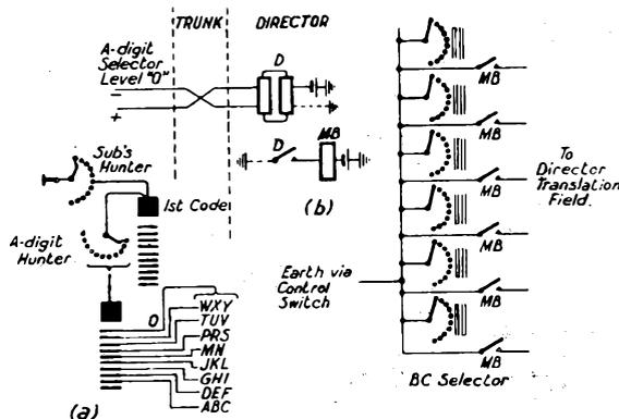
features of the modification; the +ve and -ve wires of the trunk outgoing from the o level are reversed and, when a
