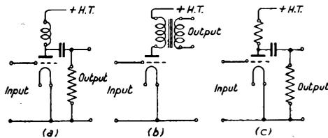
placed in the anode circuit of a valve and an A.C. input is applied to the grid then the anode current will vary in accordance with the grid input. This variation in anode current will set up an A.C. voltage across the anode circuit impedance and this voltage can be coupled to a succeeding stage through a condenser C as in (a) and (c) or through the transformer as in (b).
