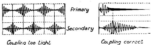
The quenched gap, a large number of small gaps in series with large cooling surfaces, quenches the spark or deionises the gap in this manner and enables a closer coupling and hence greater efficiency to be obtained.
