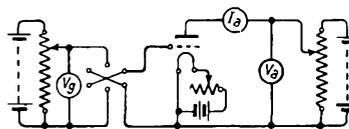
A reversing switch is inserted in the grid supply to enable readings to be taken for both +ve and -ve values of grid voltage. The meter  $I_a$  enables the anode current to be read. The procedure would be as follows:—With the anode voltage set to a particular value and maintained constant readings of anode current would be taken for various values of grid voltage. The readings would then be repeated for other values of anode voltage. The values would then be plotted to form a series of curves.
