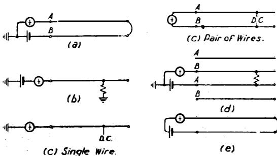
a test for current should be made before a test for earth (low insulation resistance). Otherwise, the presence of an undetected extraneous earth current would give the appearance of low insulation on the line. Next, tests for loop and disconnection are made and, finally, the line is tested for freedom from contact.
