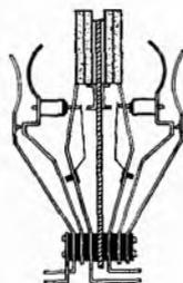
arrangement of the heat coils, protectors, and test jack required for one line; by inserting a plug into the jack, formed by the two outer pairs of springs, testing or other apparatus may be inserted in the line. This equipment is mounted on
