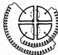
An electrostatic voltmeter could be used as an ammeter in conjunction with a shunt of fairly high resistance, say 200 ohms. In the majority of cases, however, the insertion of this resistance in the circuit would materially affect the current flowing and the method could only be used where the resistance of the circuit was large compared with that of the shunt.
