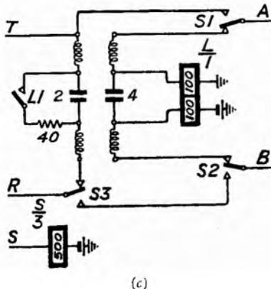
P.B.X. and an ordinary C.B. telephone is fitted at the extension point. The circuit is arranged so that the equipment may be cut out of circuit when the extension line is extended to an exchange line, so that the extension point may be fed with transmitter current from the exchange, instead of from the auxiliary equipment.
