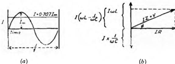
the voltage across the inductance is represented by the line  $\omega L$  which, due to the effect of the inductive reactance, is lagging  $90^\circ$  behind the vector  $IR$ ; the voltage across the capacitance is equal to  $1/\omega C$ , and leads the vector  $IR$  by  $90^\circ$  due to the effect of the capacitive reactance. The resultant of these three vectors is the applied voltage  $I Z = V$ , where
