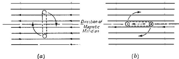
cut, no E.M.F. is generated. When the plane of the coil is in the magnetic meridian, as in sketch (b), the conductors are cutting the earth's field at right angles and a maximum E.M.F. is generated. By this means it is possible to locate the direction of the magnetic meridian if the position of the coil corresponding to a maximum deflection of the galvano-
