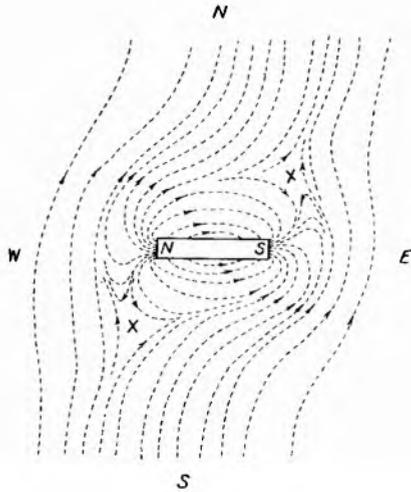
to the earth and the bar magnet are opposite in direction and equal in magnitude. A compass needle placed in one of these positions is not subject to a magnetic force and will therefore come to rest in any direction.
