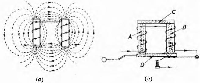
With the magnetomotive force of the coils and the reluctance of the magnetic circuit fixed by design, the number of lines of force in the air gaps can be calculated. The total number of lines of force at any point in the circuit is referred to as the "flux" at that point. The flux depends directly upon the magnetomotive force and inversely upon the reluctance, i.e.,
