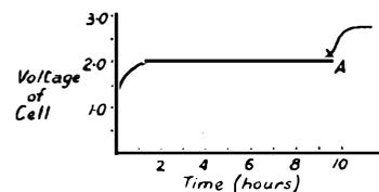
to about 2.0 volts during the first hour of the charge, and then remains steady for some hours. As the cell approaches the fully-charged condition, the voltage again rises and about the point marked "A" in the sketch, gassing commences.
