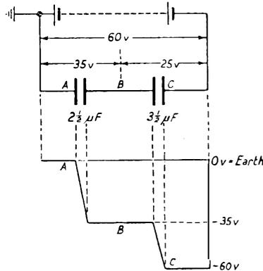
With the connexions as shown in the sketch and considering the earth potential as zero, the potentials of the points marked are: A = 0, B = - 35 volts, and C = - 60 volts.
