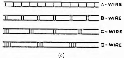
of lines in, say, one yard length of paper, is the same for each of the four wires; by this means, it is ensured that the dielectric formed by the insulating paper and its markings shall be uniform for either pair of wires.
