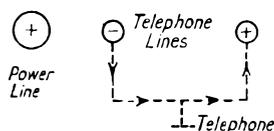
at both ends. The left end of B has now a negative potential as compared with the space immediately surrounding it. Similarly, the right end of B has an apparent positive charge compared with the field strength at that end.
