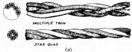
the two types. The star quad consists of four wires revolving around a common axis, whilst the multiple twin quad consists of two twisted pairs twisted together. The A, B, C, and D wires of a star quad are marked by groups of 1, 2, 3, and 4 ink lines on the insulating paper at intervals, as shown in sketch (b). The groups of lines are so spaced that the number
