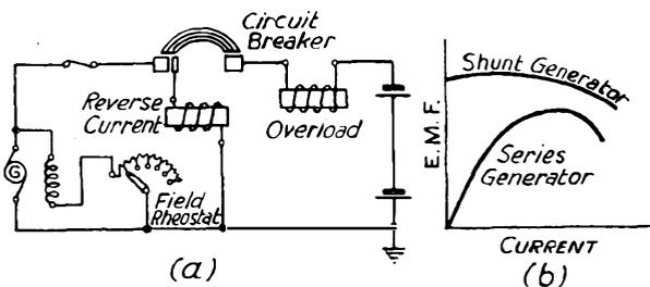
If such a generator were to be used for charging secondary cells, there would be a difficulty in running the machine up to the voltage required. Further, the increase in the E.M.F. of the cells during charge would reduce the terminal E.M.F. of the generator down to the point where it would fail to excite.
