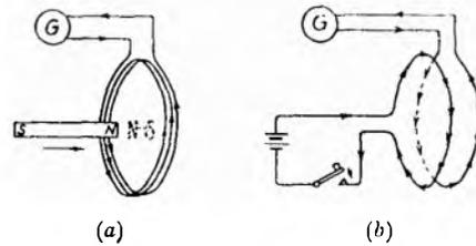
4. Place the two coils of wire close together with their planes parallel. Connect up the battery to the second coil and a deflection of the galvanometer will occur at the moment of switching on. This verifies experiment No. 1, since an E.M.F. is generated only when the magnetic field is building up round the second coil and in so doing cuts across the conductors of the first coil.
