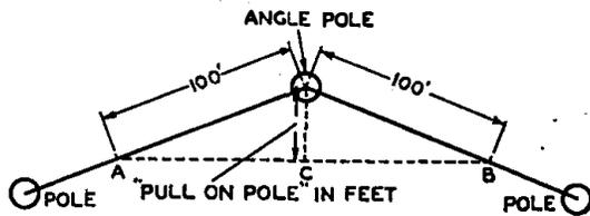
FIG. 2.—"PULL-ON-POLE" MEASUREMENT.
