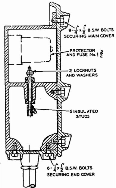
FIG. 7. PROTECTOR AND FUSE UNIT.
