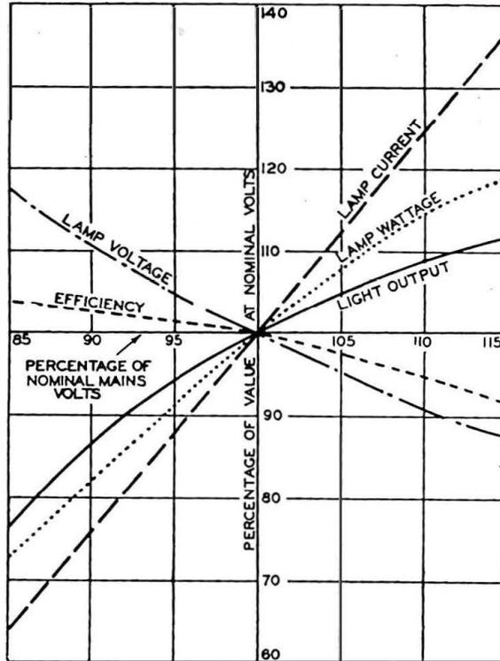
FIG. 7.—GRAPH ILLUSTRATING EFFECT OF SUPPLY VOLTAGE VARIATIONS.
