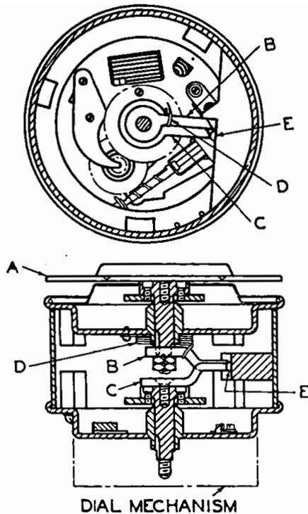
FIG. 5.—DIAL MECHANISM FITTED WITH SLIPPING CLUTCH DEVICE.
