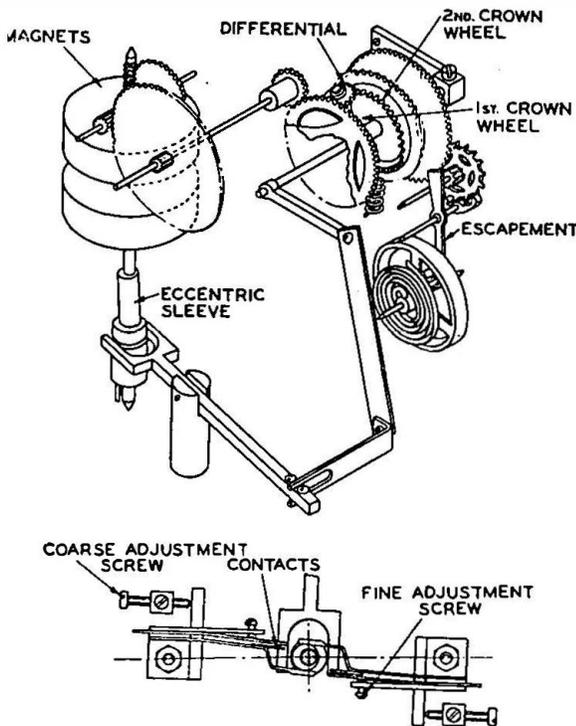
FIG. 6.—CONSTRUCTIONAL DETAILS OF EXPERIMENTAL MOTOR.
