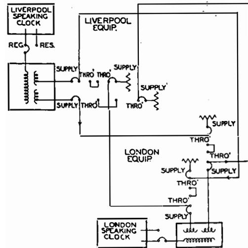
FIG. 2.—OMNIBUS TRUNK CIRCUIT CONNECTIONS AT REPEATER STATIONS.
