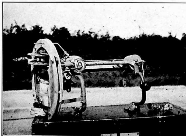
FIG. 2. THE NEALE SPINNER (SHOWING TENSIONING WHEELS).
