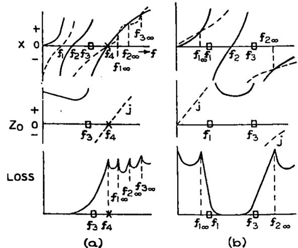
FIG. 7.—LOW PASS AND BAND PASS FILTER CURVES.
