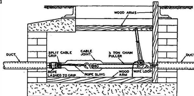
Men were posted to watch the intermediate joints, and the two chains were operated simultaneously. The movement of the cable was slow and steady and the cable was gradually restored to its original position. It should be mentioned that the cable was jointed straight across the intermediate joint boxes, and that the duct track follows a straight line.
