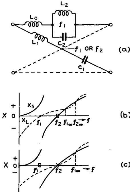
FIG. 5.—Low Pass Filter with Alternative Characteristics.
