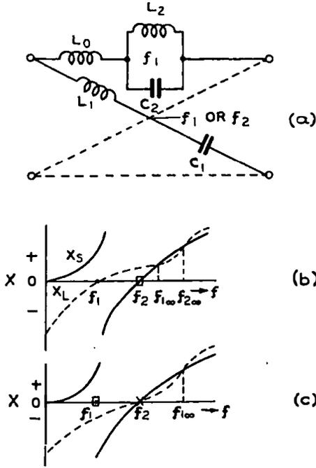
FIG. 5.—LOW PASS FILTER WITH ALTERNATIVE CHARACTERISTICS.
