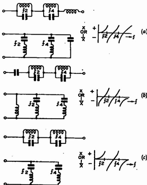
FIG. 3.—REACTANCE AND SUSCEPTANCE CURVES OF VARIOUS CIRCUITS
