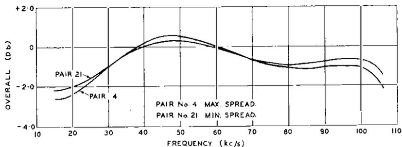
FIG. 5.—MAXIMUM AND MINIMUM VARIATIONS OF LEVEL WITH FREQUENCY ON LONDON-LEICESTER SECTION OF LONDON-DERBY NO. 2 CABLE.
