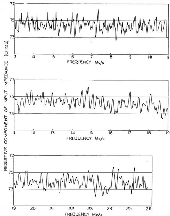
FIG. 8.—VARIATION OF RESISTIVE COMPONENT OF INPUT IMPEDANCE WITH FREQUENCY FOR 3-MILE LENGTH OF 0.975 INCH TUBE.
