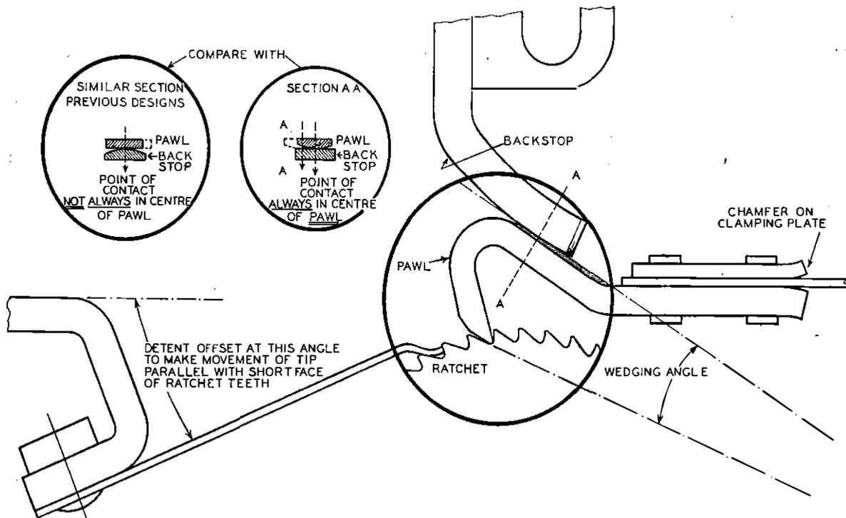
FIG. 5.—MAIN FEATURES OF DRIVING MECHANISM.
