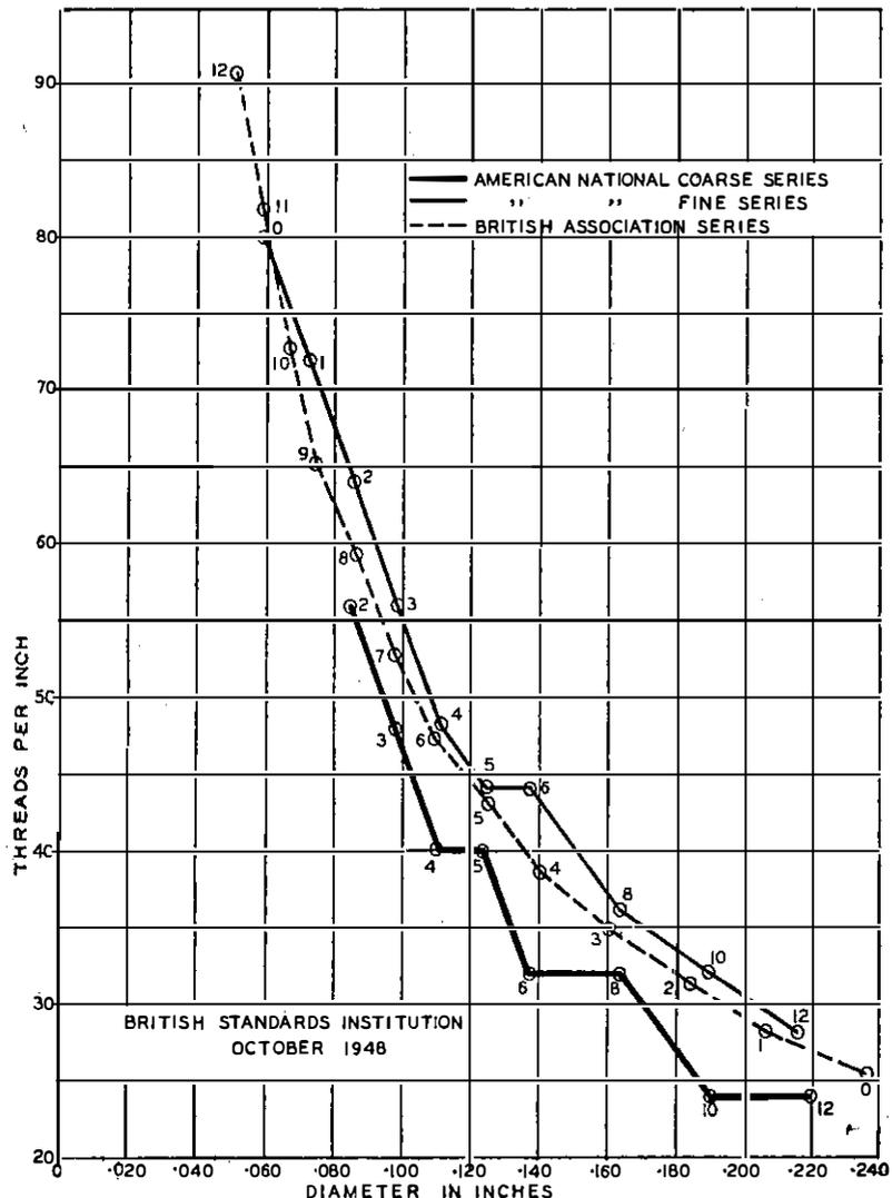
FIG. 3.—COMPARISON BETWEEN BRITISH AND AMERICAN STANDARD SIZES FOR THREADS IN THE RANGE BELOW  $\frac{1}{4}$  INCH.
