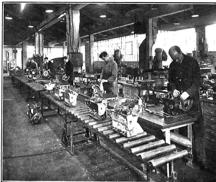
FIG. 5.—ENGINE ASSEMBLY LINE.
