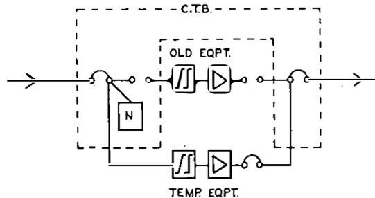
FIG. 3.—EXISTING EQUIPMENT REPLACED BY TEMPORARY EQUIPMENT.
