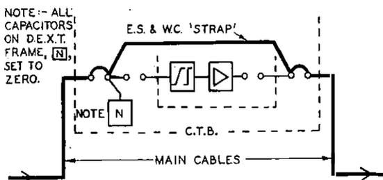
FIG. 1.—MAIN CABLE CONNECTIONS AT NEW STATION BEFORE EQUIPMENT IS CUT IN.
