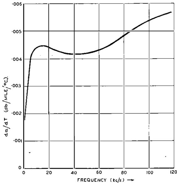
FIG. 6.—CABLE P.C.Q. CARRIER 12-QUAD 40-LB. SIDE CIRCUIT. VARIATION OF ATTENUATION ( $\alpha$ ) WITH TEMPERATURE ( $T$ ) (DB./MILE/°C) V. FREQUENCY.
