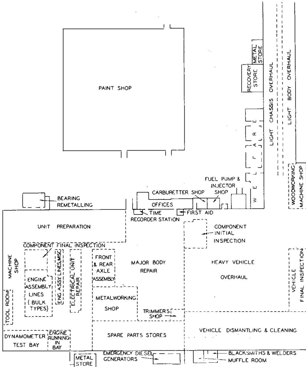
FIG. 1.—LAYOUT OF YEADING REPAIR DEPOT.
