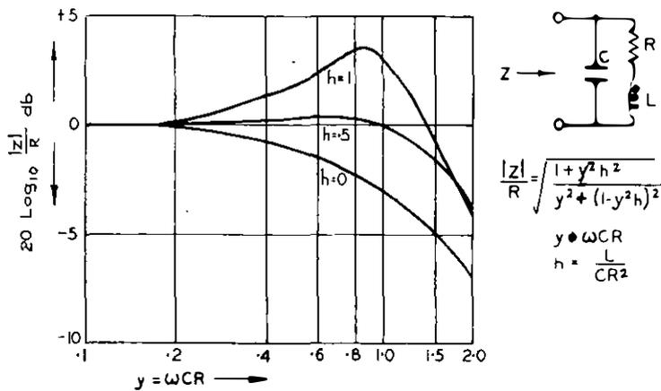
FIG. 4.—ANODE LOAD INCLUDING REACTANCES.
