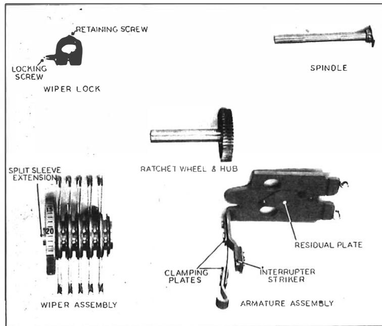
FIG. 6.—PARTS OF UNISELECTOR TYPE 2.
