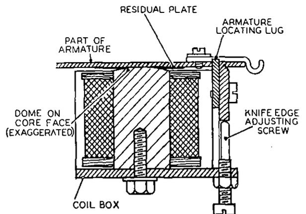
FIG. 4.—CROSS-SECTION OF COIL BOX AND ARMATURE.
