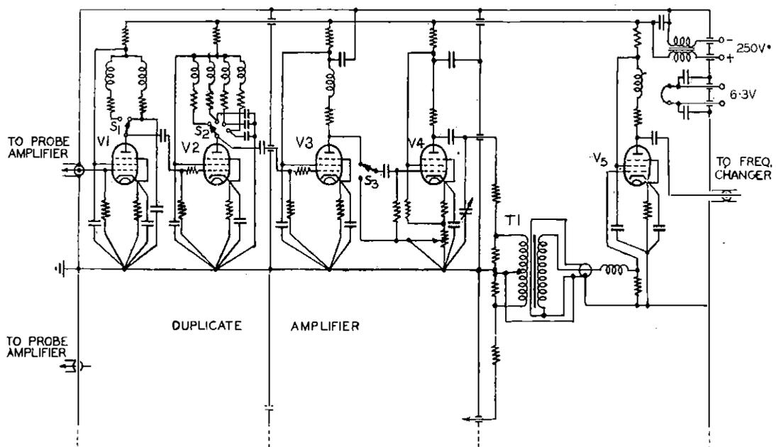
FIG. 3.—"TWIN" AMPLIFIERS CIRCUIT.
