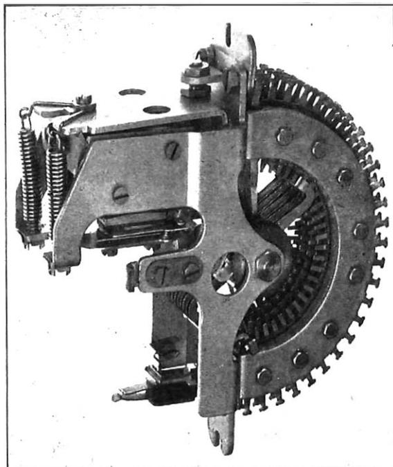
FIG. 1.—P.O. UNISELECTOR TYPE 2—5 LEVEL.
