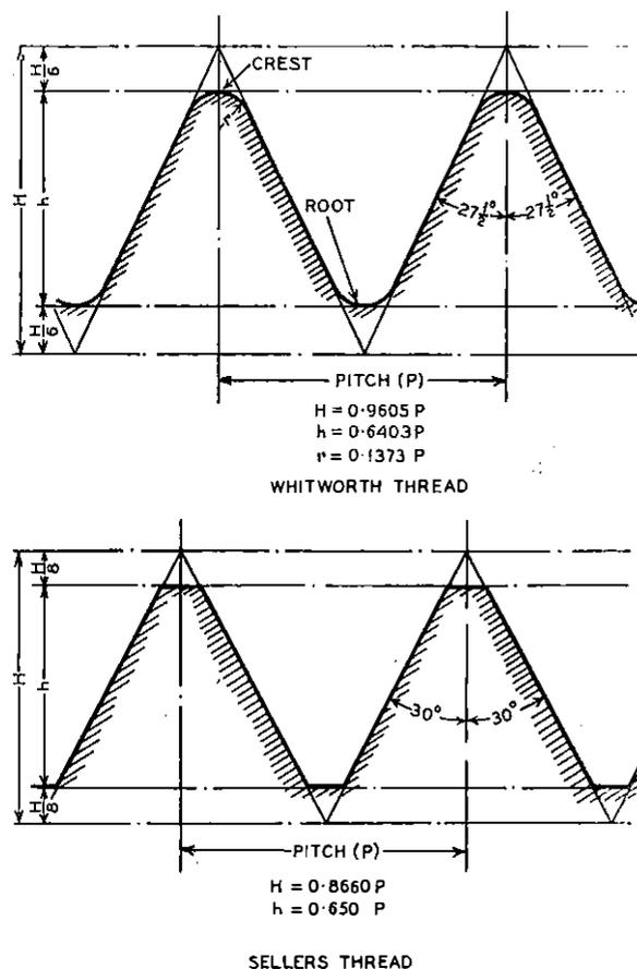
FIG. 1.—COMPARATIVE SHAPES OF WHITWORTH AND SELLERS THREADS.
