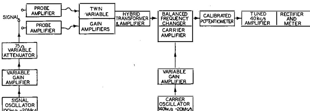
FIG. 1.—BLOCK SCHEMATIC DIAGRAM OF PHASE METER.
