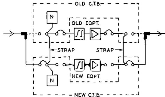
FIG. 2.—CONNECTIONS AT EXISTING STATION BEFORE NEW EQUIPMENT IS CUT IN.
