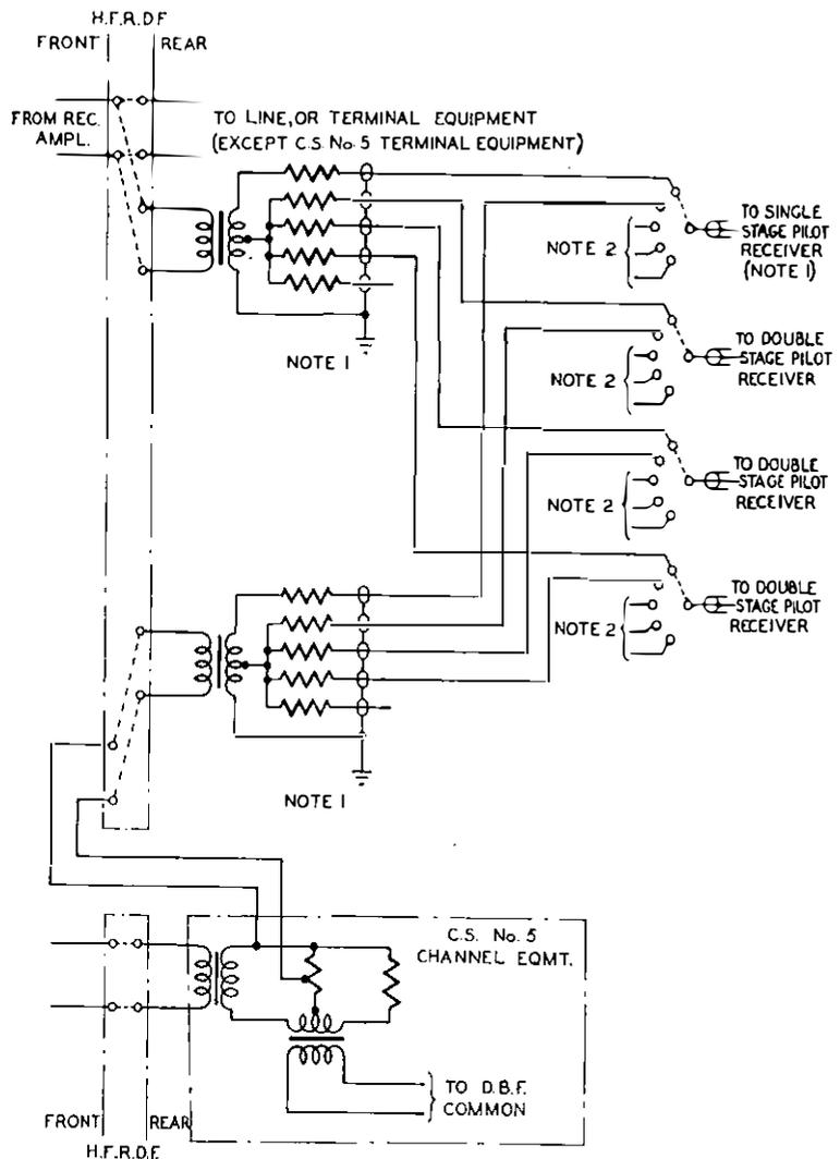
**Note 1.**—Depending upon the output connections, each transformer unit caters for either one single-stage pilot receiver and three double-stage pilot receivers, or four double-stage pilot receivers.
