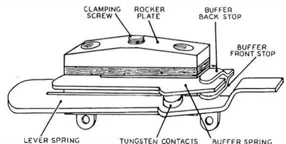
FIG. 7.—INTERRUPTER OF UNISELECTOR TYPE 2.
