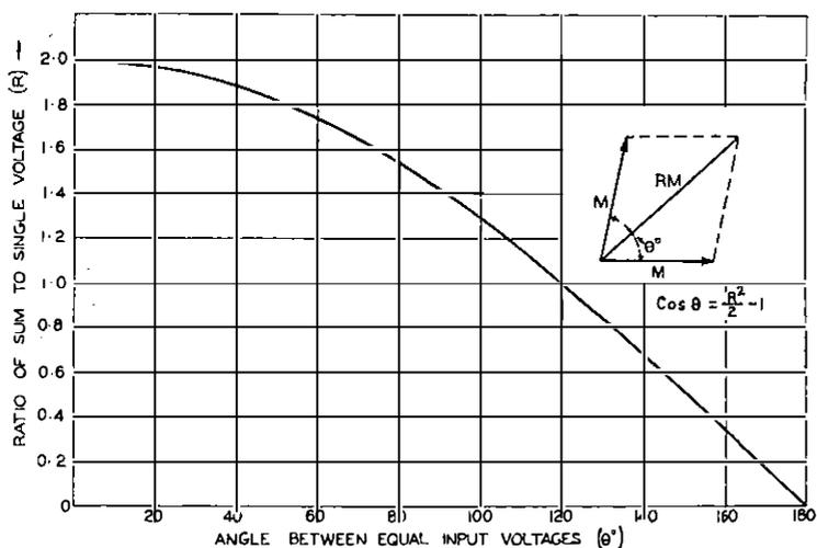
FIG. 2.—RATIO OF MAGNITUDE OF SUM OF TWO EQUAL VOLTAGES AT ANGLE  $\theta^\circ$ , TO MAGNITUDE OF A SINGLE VOLTAGE.
