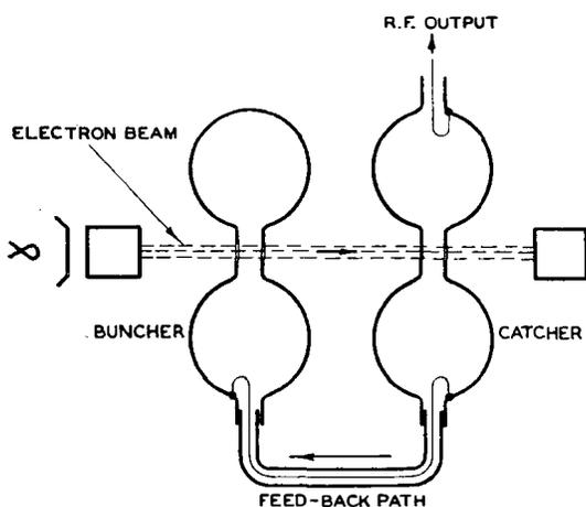
FIG. 8.—SIMPLIFIED SKETCH OF DOUBLE-RESONATOR KLYSTRON OSCILLATOR.
