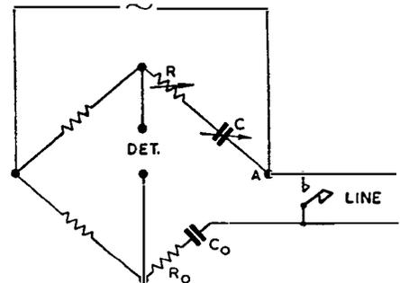
FIG. 1.—SIMPLIFIED CIRCUIT OF SERIES ARTIFICE BRIDGE.
