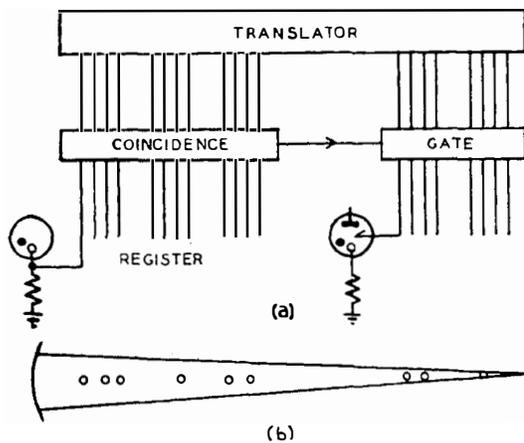
FIG. 7.—THE ELEMENTS OF A STATIC REGISTER-PULSE TRANSLATOR.
