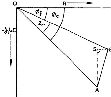
FIG. 2.—VECTORIAL REPRESENTATION OF OPEN AND CLOSED IMPEDANCES.
