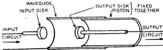
FIG. 1.—BASIC FEATURES OF AN  $E_{0,1}$  PISTON ATTENUATOR.
