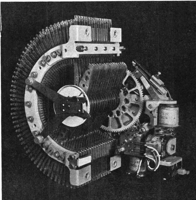
For their Trunk Mechanization Scheme the British Post Office has adopted the High-Speed Motor Uniselector illustrated above.
