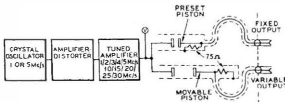
FIG. 3.—BLOCK SCHEMATIC DIAGRAM OF PISTON ATTENUATOR CONTROLLED SIGNAL GENERATOR.
