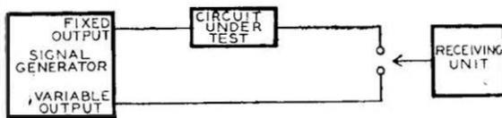
FIG. 2.—ARRANGEMENT FOR MEASURING INSERTION LOSS.
