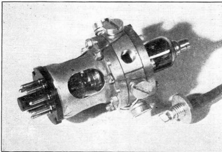
FIG. 10.—REFLEX KLYSTRON OSCILLATOR, VX 5026.
