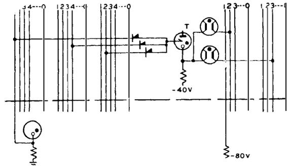
FIG. 6.—THE ELEMENTS OF A STATIC REGISTER-STATIC TRANSLATOR.
