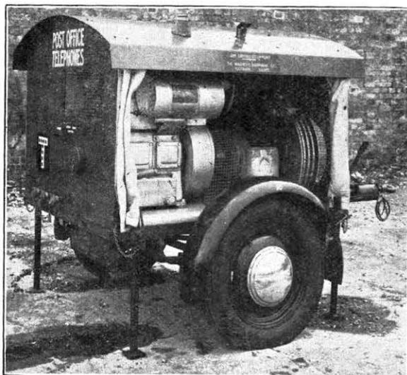
FIG. 2.—ENGINE AND COMPRESSOR SIDE OF THE DESICCATOR.
