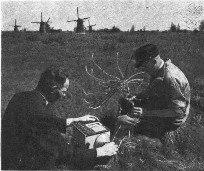
HOLLAND. "Megger" Testers are used by the Dutch Post Office. This photograph shows Dutch P.O. engineers using a 500 volt Bridge-Megger Varley Testing Set to test a faulty line of a telephone cable in a polder-dike.
