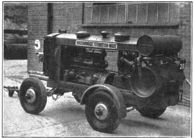
FIG. 5.—TWO-TOOL TRAILER AIR-COMPRESSOR WITH SIDE PANELS REMOVED.
