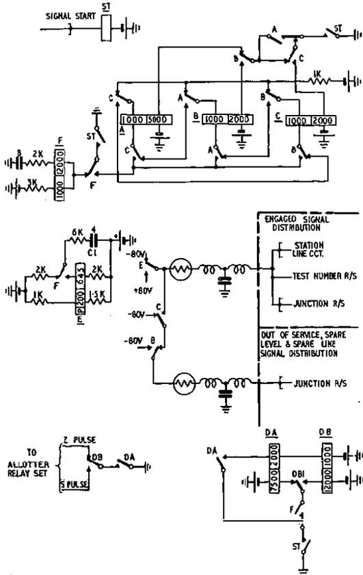
FIG. 7.—CIRCUIT ELEMENTS OF SIGNAL GENERATOR RELAY SET.
