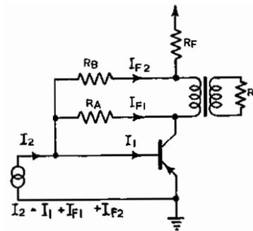
FIG. 28.—MIXED FEEDBACK APPLIED TO A GROUNDED-EMITTER CIRCUIT.
