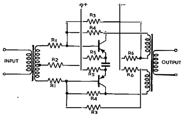
FIG. 29.—EXPERIMENTAL AUDIO-FREQUENCY LINE AMPLIFIER USING JUNCTION TRANSISTORS.
