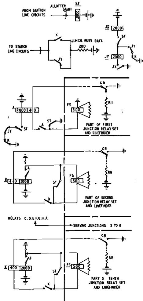
FIG. 5.—ELEMENTS OF THE ALLOTTER RELAY SET CIRCUIT.
