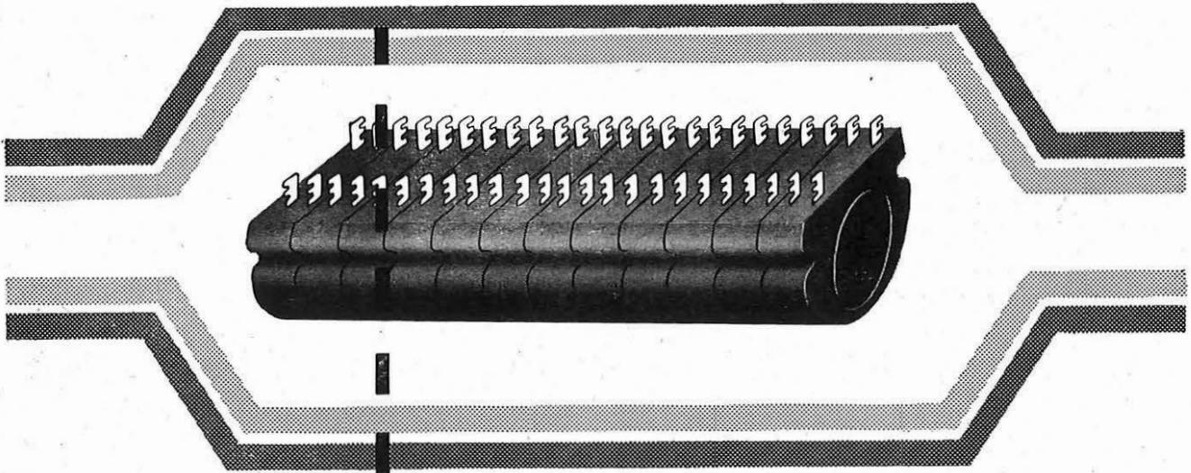
The advantages of the splice loading technique are particularly marked in the loading of small cables of up to 74 pairs. The coils can be included in a jointing sleeve or unit of only slightly larger diameter than would normally be used.
