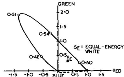
FIG. 4.—RED-GREEN CHROMATICITY DIAGRAM FOR C.I.E. SPECTRAL PRIMARIES.
