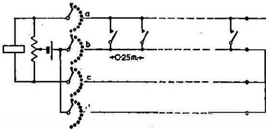
FIG. 6.—BRIDGE CONNECTIONS OF TEST QUAD AND CONTACTORS.
