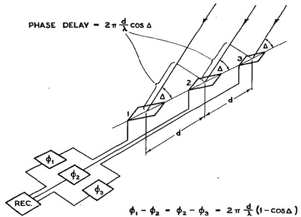
FIG. 17.—MULTIPLE UNIT STEERABLE ANTENNA SYSTEM. (Principle of Operation.)
