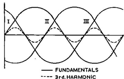
FIG. 2.—PHASE RELATIONSHIPS IN A 3-PHASE POWER LINE.
