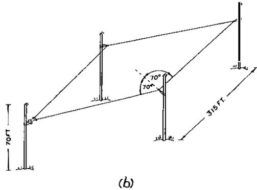
FIG. 10.—PRINCIPLE OF OPERATION AND PICTORIAL VIEW OF RHOMBIC AERIAL.
