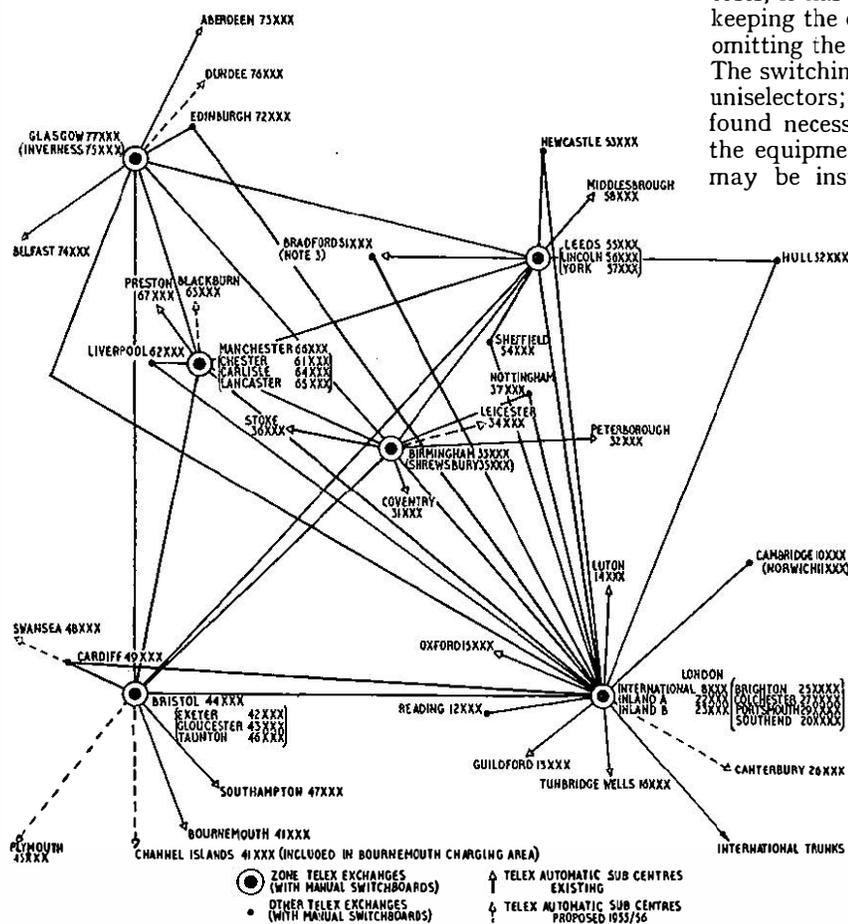
FIG. 1.—THE U.K. TELEX NETWORK AT SPRING, 1955.
