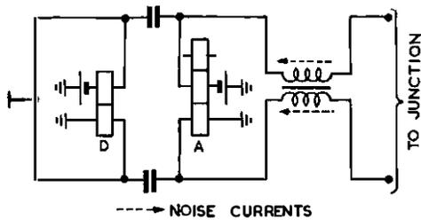
FIG. 7.—USE OF AN INDUCTOR TO SUPPRESS NOISE.
