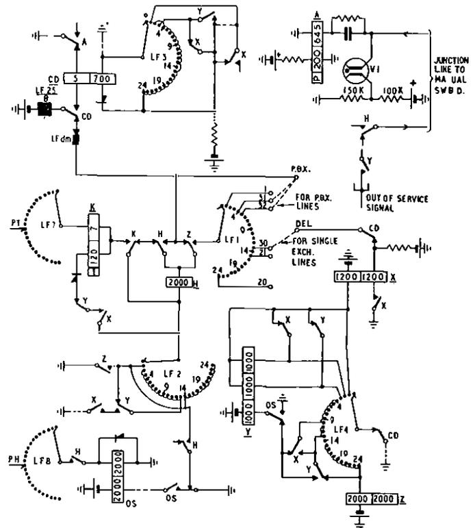
FIG. 6.—THE JUNCTION RELAY SET CIRCUIT ELEMENTS USED FOR CONTROLLING THE UNISELECTOR BY DIAL PULSES ON INCOMING CALLS.
