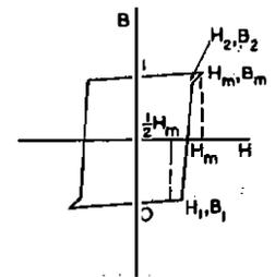
FIG. 9.—SIMPLIFIED HYSTERESIS LOOP FOR THE CORE OF A MATRIX-STORE INDUCTOR.
