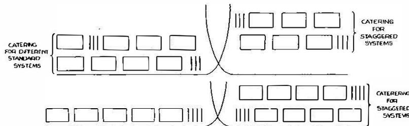
The signalling channels placed in an otherwise wasted part of the frequency band, as illustrated.
