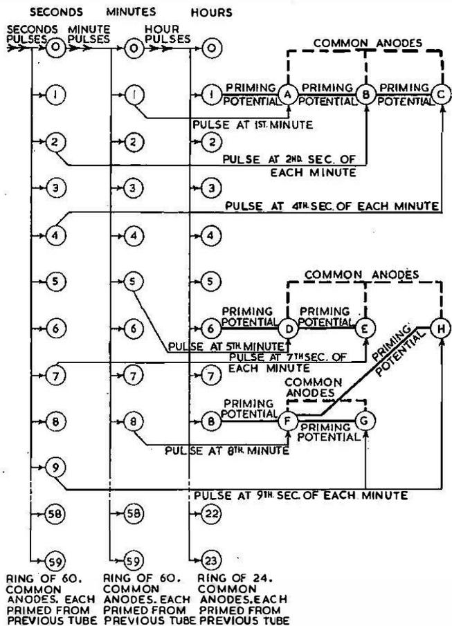
FIG. 2.—SCHEMATIC DIAGRAM OF AN ELECTRONIC PROGRAMME CLOCK.
