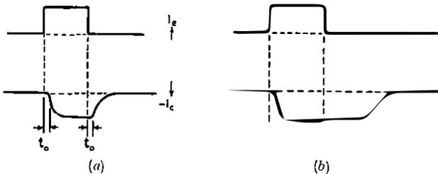
FIG. 23.—THE TRANSIENT RESPONSES OF TYPICAL TRANSISTORS FOR (a) A SMALL OUTPUT SIGNAL; AND (b) A LARGE OUTPUT SIGNAL.
