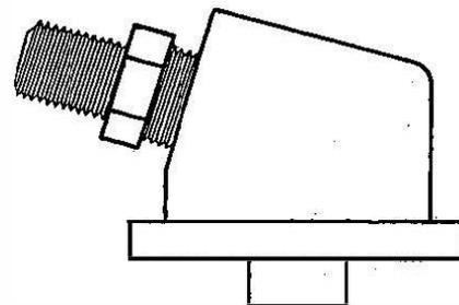
FIG. 8.—SCHRADER VALVE ASSEMBLY.
