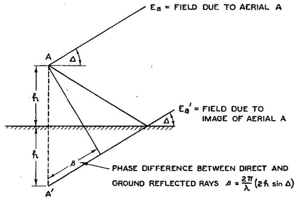
FIG. 15.—DERIVATION OF HEIGHT FUNCTION.
