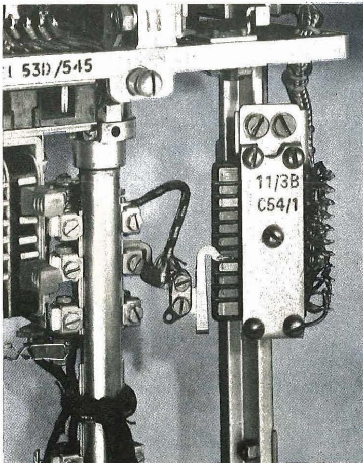
Interesting features in Strowger exchanges by G.E.C. using the SE50 as a 200-outlet linefinder:
