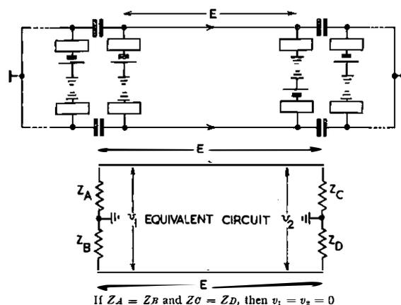
FIG. 4.—A TYPICAL TELEPHONE CIRCUIT AND ITS EQUIVALENT, SHOWING INDUCED VOLTAGES.
