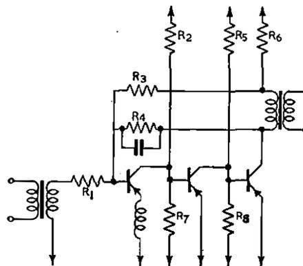
FIG. 30.—EXPERIMENTAL THREE-STAGE LINE AMPLIFIER USING JUNCTION TRANSISTORS.
