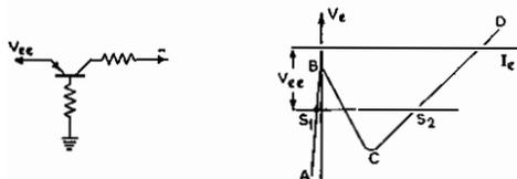
FIG. 35.—A BI-STABLE CIRCUIT USING A POINT-CONTACT TRANSISTOR.
