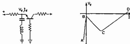
FIG. 33.—A TWO-TERMINAL OSCILLATOR USING A POINT-CONTACT TRANSISTOR.
