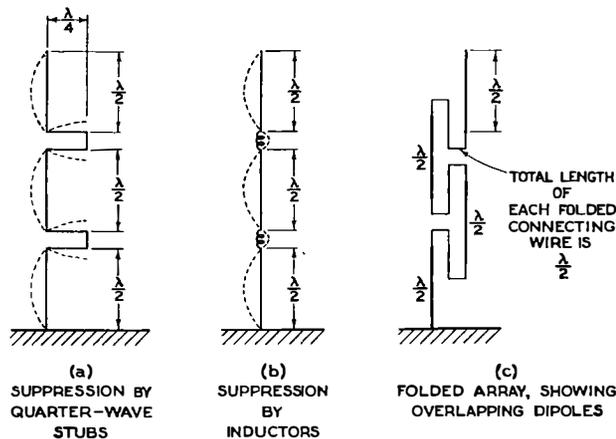
FIG. 14.—PRINCIPLE OF FRANKLIN ARRAYS.
